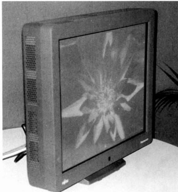
Fujitsu's prototype gas-plasma display.
