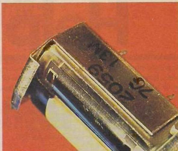
Fig. 4: A worn head. The step or groove is visible near the top edge of the audio head insert.
