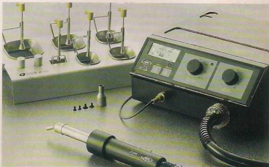
The JBC JT6040 hot-air desoldering station, which is available from Willow Vale, will deal with all types of surface-mounted devices. The control unit has an 800W heater.
