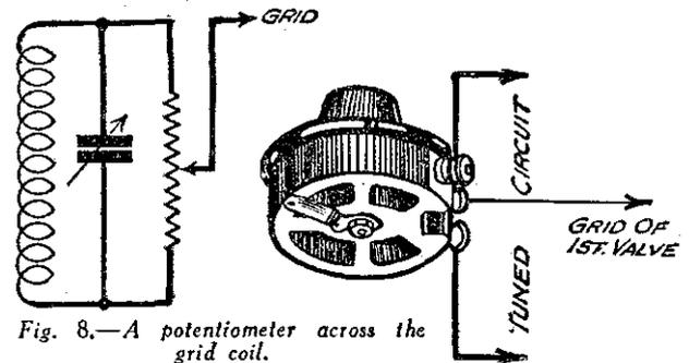
Fig. 8.—A potentiometer across the grid coil.
