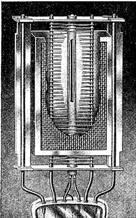
The employment of Mica Bridge Mounting in Cossor Valves ensures microscopic accuracy in the assembly of the electrode system. As a result the characteristics of every valve are identical with those of the original design developed in the laboratory. Variation is impossible. The performance of each valve is therefore safeguarded—the Mica Bridge is a virtual guarantee of performance and reliability.
