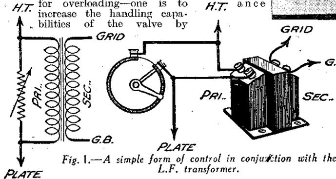
Fig. 1.—A simple form of control in conjunction with the L.F. transformer.
