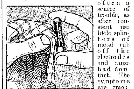
Fig. 2.—To dust the grid leak remove it from the clips. Also dust between the clips before replacing it.
