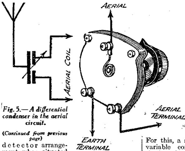
Fig. 5.—A differential condenser in the aerial circuit.
