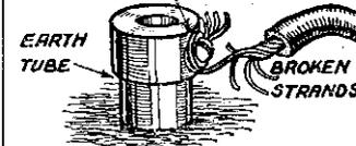
Fig. 7.—Some likely causes of a poor earth.
