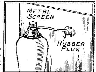
Fig. 4.—Where the wire from the plate of a screen grid valve passes through a metal screen, capacity losses may be minimised by adopting the idea shown here.
