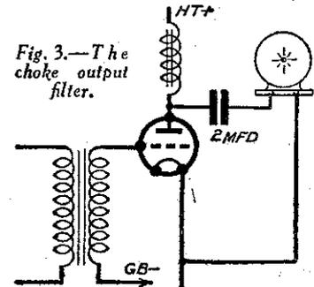
Fig. 3.—The choke output filter.
