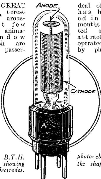
The B.T.H. cell showing the electrodes.
