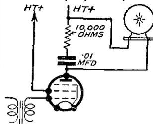
Fig. 5.—The corrector circuit.
