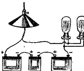
By adopting the simple arrangement shown here, accumulators can be charged at home if your electric supply is D.C. The two lamps on the right are 60-watt lamps and are used as a resistance.
