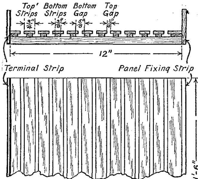
Fig. 2.—Part plan and section of the baseboard.
