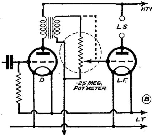
Fig. 2 (and opposite).—Two forms of post-detector control.
