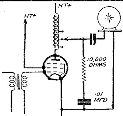
Fig. 7.—Tapped output choke and tone corrector.
