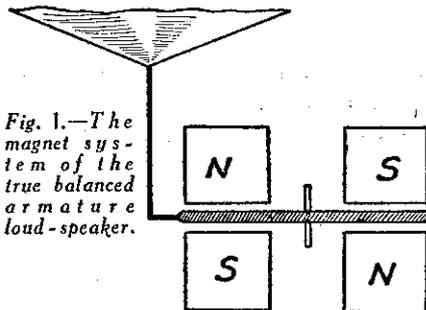
Fig. 1.—The magnet system of the true balanced armature loud-speaker.
