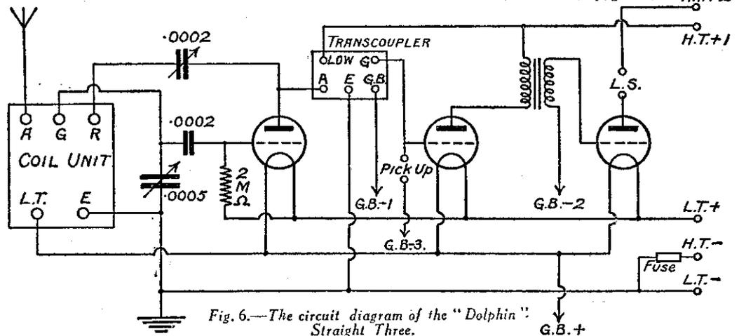
Fig. 6.—The circuit diagram of the "Dolphin" Straight Three.
