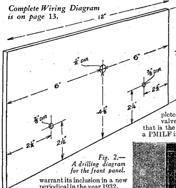
Fig. 2.—A drilling diagram for the front panel.
