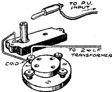
When using a pick-up in conjunction with two L.F. stages, the usual panel switch or jack arrangement for bringing the pick-up into circuit generally involves a long grid lead and return. This can be obviated by using two old plug-in coil-holders as shown.
