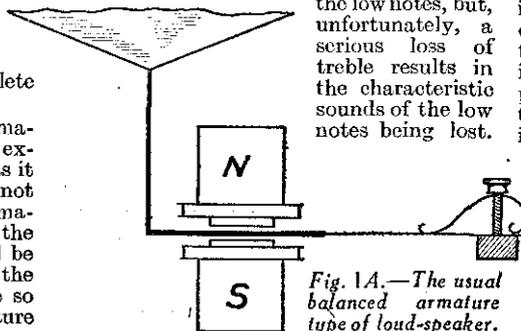
Fig. 1A.—The usual balanced armature type of loud-speaker.
