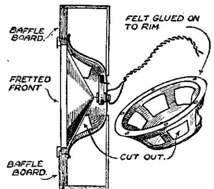
A reasonably good speaker—unit chassis can be made from an ordinary tin or enamel basin measuring 12in. or 18in. in diameter.
