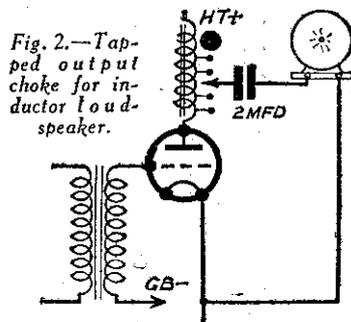
Fig. 2.—Tapped output choke for inductor loud-speaker.
