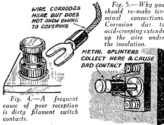
Fig. 4.—A frequent cause of poor reception is dirty filament switch contacts.
