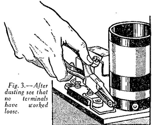
Fig. 3.—After dusting see that no terminals have worked loose.
