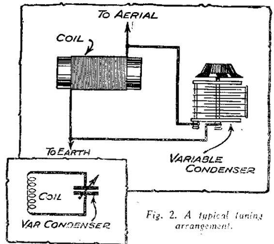
Fig. 2. A typical tuning arrangement.
