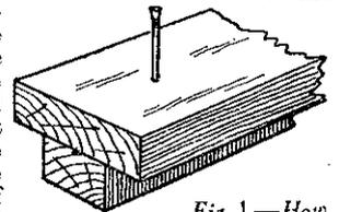
Fig. 1.—How to assemble the T-pieces.
