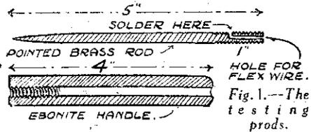
Fig. 1.—The testing prods.
