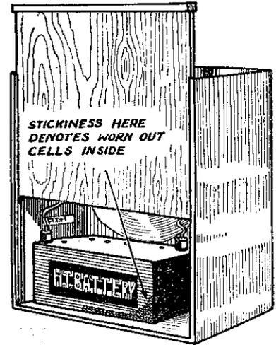
Fig. 8.—Stickiness on the outside of the H.T. battery means deterioration and will cause harm if left in your set in such condition.
