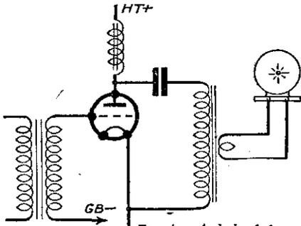
Fig. 4.—A choke-fed transformer for a moving-coil speaker.
