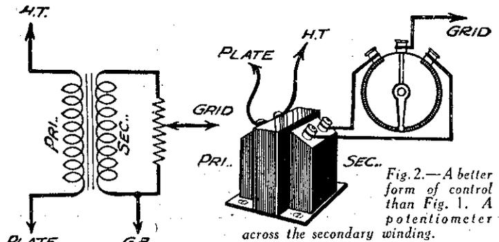
Fig. 2.—A better form of control than Fig. 1. A potentiometer across the secondary winding.
