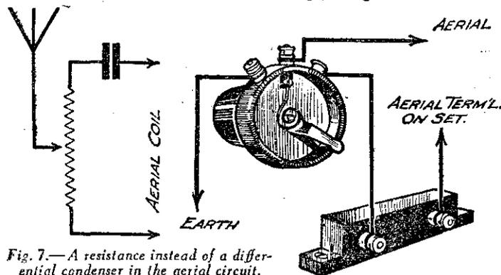
Fig. 7.—A resistance instead of a differential condenser in the aerial circuit.
