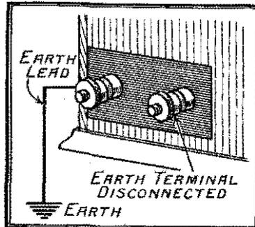
Fig. 2.—Utilising the earth lead as an aerial.
