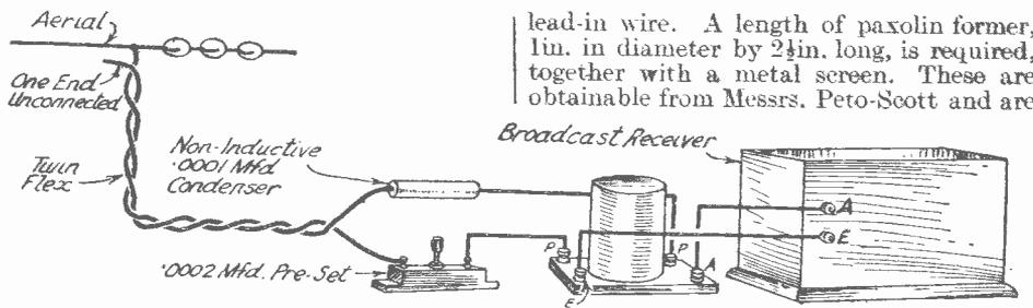
Fig. 5.—Connections for anti-interference device.
