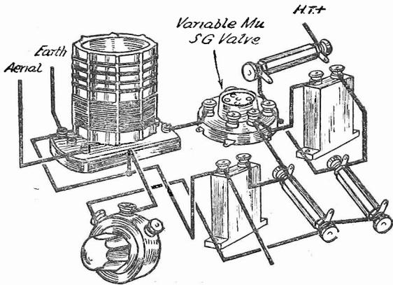
Fig. 5.—Gain control by variable-mu S.G. valve in a mains set.
