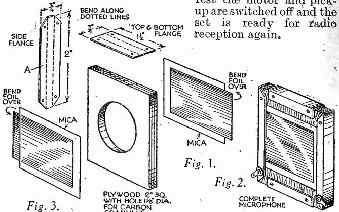
*Constructional details for an easily made microphone.*
