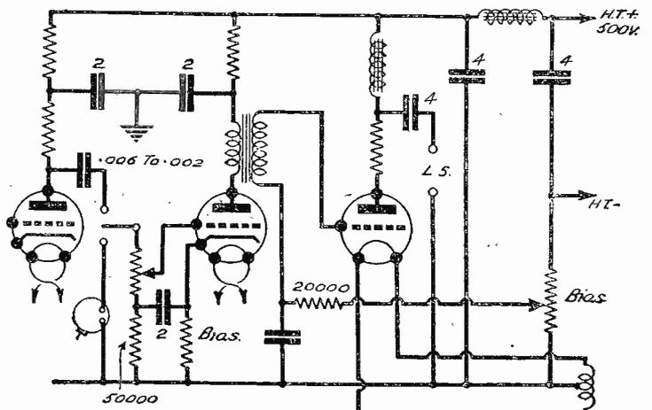
Fig. 9.—A suggested arrangement for the L.F. side of a quality receiver.
