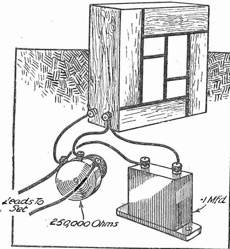
Fig. 1.—A simple system of effecting remote control of volume.
