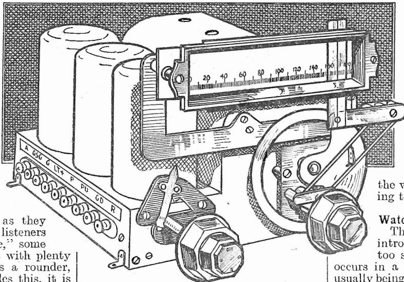
Fig. 1.—Illustration of modern H.F. tuning pack.
