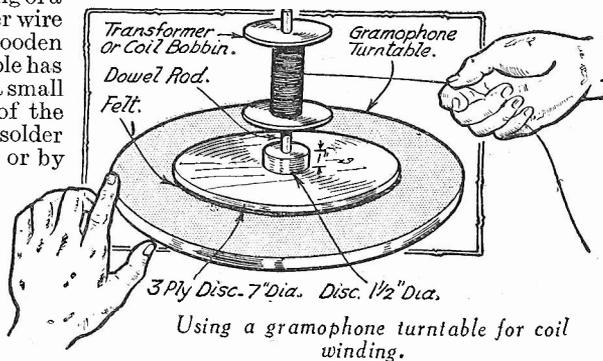
*Using a gramophone turntable for coil winding.*
