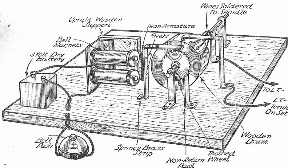
Fig. 6.—A relay by means of which the receiver can be switched on and off from a remote point.
