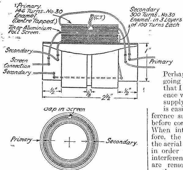
Fig. 3.—Details of the transformer.
