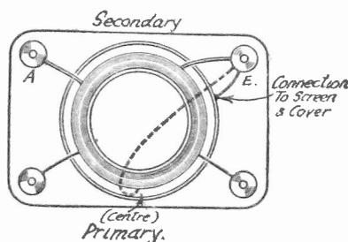
Fig. 4.—Wiring of transformer
