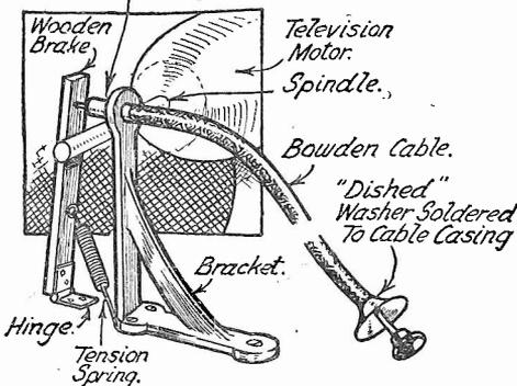
*Simple speed regulator for a television motor.*
