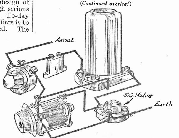
Fig. 2.—A pre-H.F. volume control using a potentiometer.
