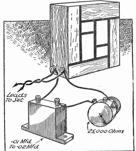
Fig. 4.—A simple and effective remote-control for varying the tone of reproduction. The .01 mfd condenser is not always necessary, but is generally desirable.
