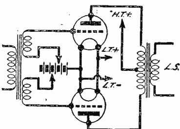
Fig. 8.—A battery operated push-pull stage.
