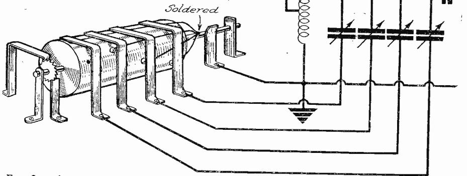
Fig. 8.—A remote tuning scheme which makes use of a relay similar to that shown in Fig. 6. This works in conjunction with a number of pre-set condensers.
