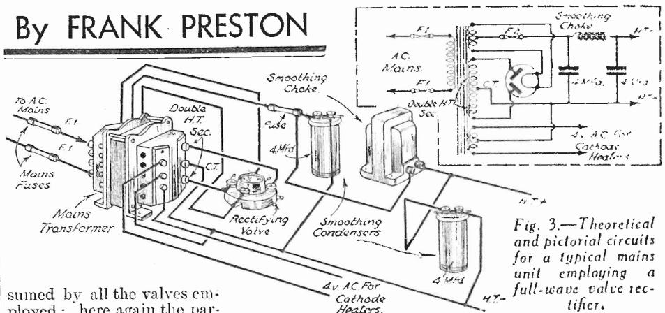
Fig. 3.—Theoretical and pictorial circuits for a typical mains unit employing a full-wave valve rectifier.
