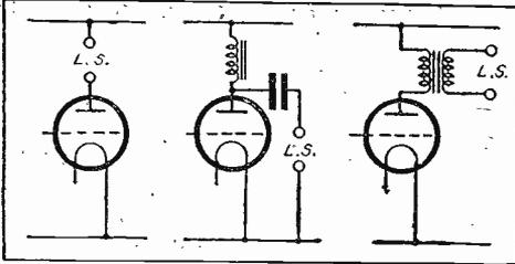
Figs. 3, 4, and 5.—Various methods of coupling the speaker to the output valve.
