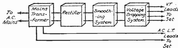
Fig. 1.—This diagram shows the principal parts of a mains unit arranged in their correct sequence. The last section—for voltage dropping—generally forms a part of the receiver.
