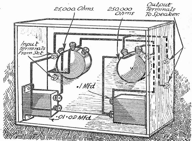
Fig. 5.—A neat unit which combines a tone control and volume control. The unit is connected between the receiver and speaker.
