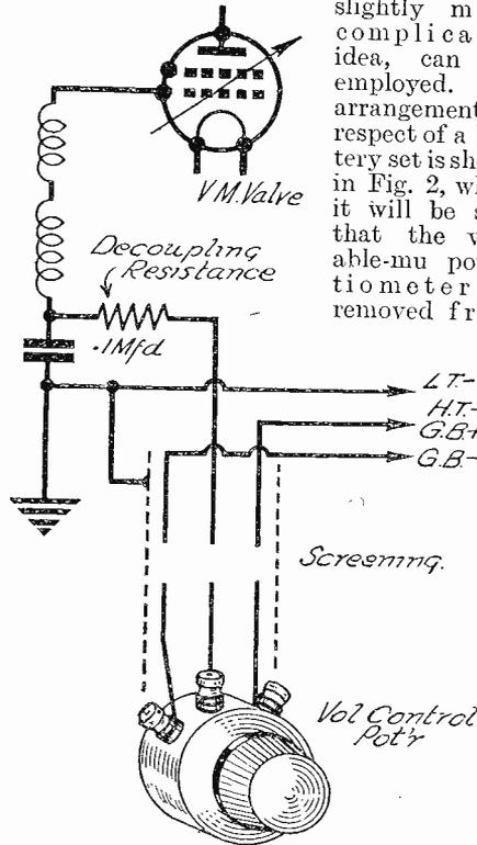
Fig. 2.—Remote volume control is easily arranged in the case of a set having a variable-mu amplifier. The connections shown above refer to a battery-operated set.
