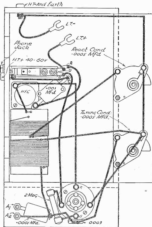
Fig. 2.—Wiring diagram for this neat little receiver.
