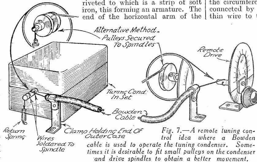
Fig. 7.—A remote tuning control idea where a Bowden cable is used to operate the tuning condenser. Sometimes it is desirable to fit small pulleys on the condenser and drive spindles to obtain a better movement.
