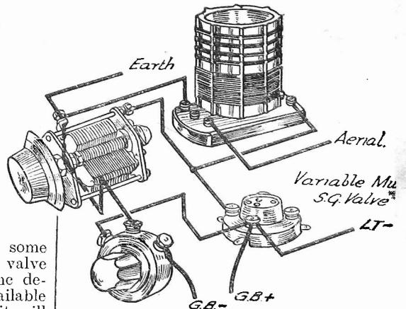
Fig. 4.—Gain control by variable-mu S.G. valve in battery set.
