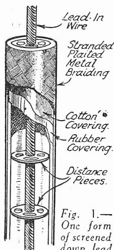
Fig. 1.—One form of screened down lead having a low self-capacity.
