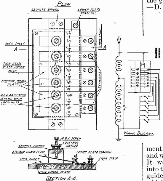
A simple method of making a bank of pre-set condensers.
