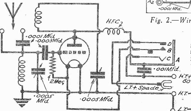
Fig. 3.—Theoretical circuit of the Pocket Portable.
