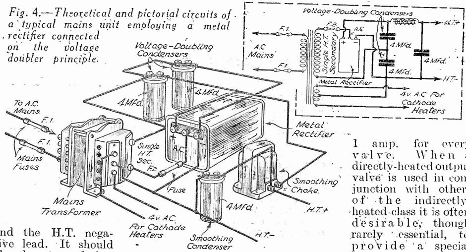
and the H.T. negative lead. It should also be stressed that the choke has a good deal of effect upon the maximum rectifier output; increasing its value tends to increase the voltage output, whilst reducing it produces the opposite effect. As a matter of fact, a 4 mfd. condenser is in nearly every case assumed by the makers in stating the output of any particular rectifier.
