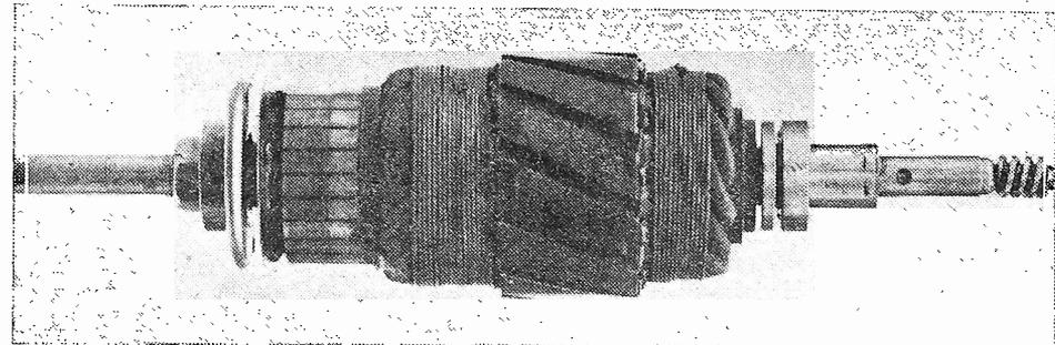
Fig. 5.—"Skewing" or inclining the armature slots of a television motor is sound practice.
