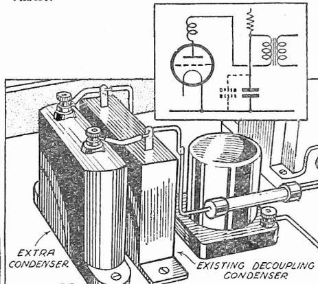
Fig. 2.—Improving the decoupling by increasing the capacity of the by-pass condenser.
