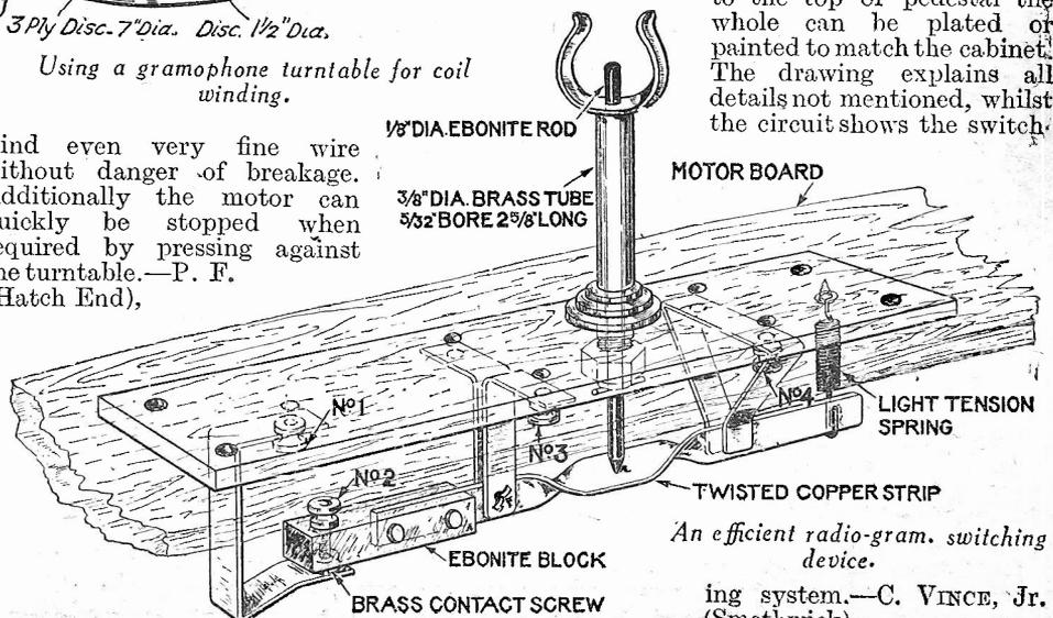
*An efficient radio-gram. switching device.*
