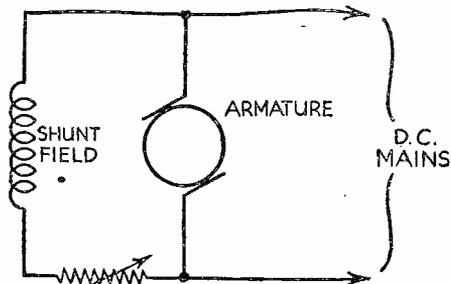
Fig. 6.—Speed control of shunt motors is effected by using a variable resistance in series with the field winding.
