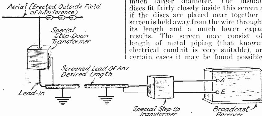
Fig. 2.—Diagram explaining the method of erecting an anti-interference aerial system employing special transformers.
