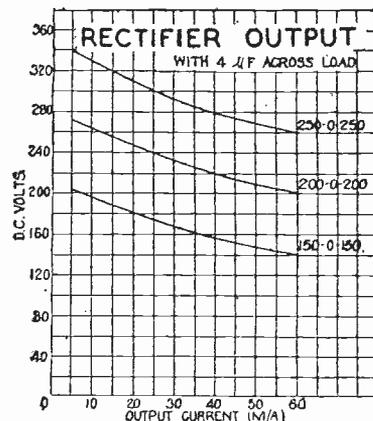
Fig. 2.—Regulation, or output curves for a typical Class A rectifying valve. These are referred to in the text.
