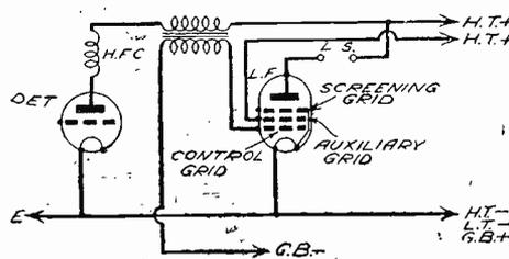
Fig. 4.—This shows the simplest connections for a pentode, as well as the corresponding connections for five-pin and base terminal valves.
