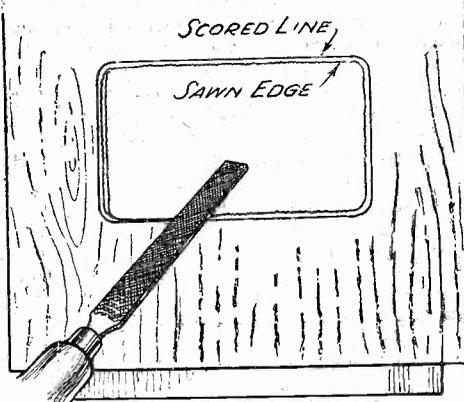
Fig. 4.—How the opening in the cabinet is finished off. The file is inclined.
