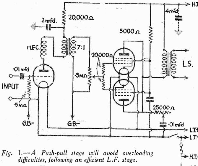
Fig. 1.—A Push-pull stage will avoid overloading difficulties, following an efficient L.F. stage.
