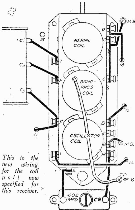
is not required, as the coils incorporate a special coupling winding and therefore hole number 13 is not used.
