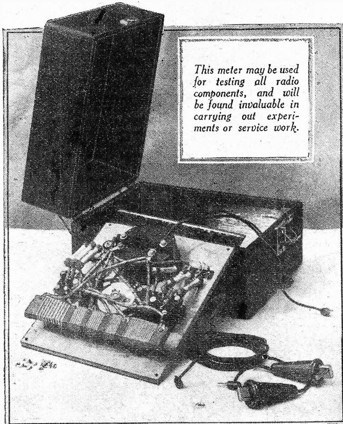
This meter may be used for testing all radio components, and will be found invaluable in carrying out experiments or service work.
