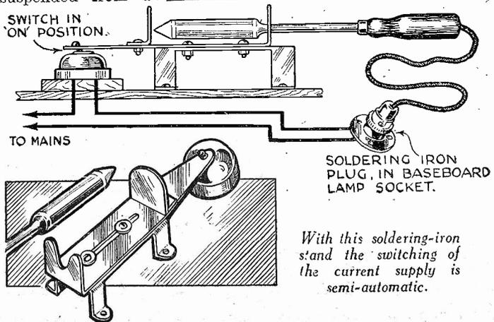
With this soldering-iron stand the switching of the current supply is semi-automatic.
