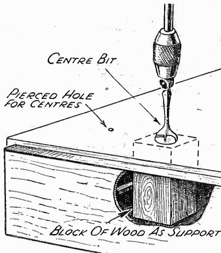
Fig. 2.—After making small centre holes from the inside of the cabinet full size holes should be traced out on the front, using a centre bit.
