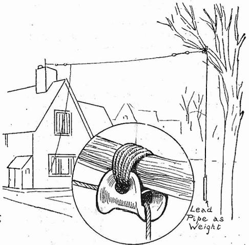
A method of suspending an aerial to allow for automatic adjustment.
