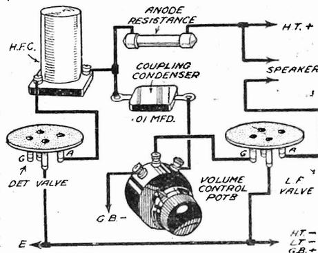
Fig. 3.—L.F. volume control in an R.C.C. or choke-capacity coupled amplifier. The potentiometer volume control replaces the grid leak and should be of similar value.
