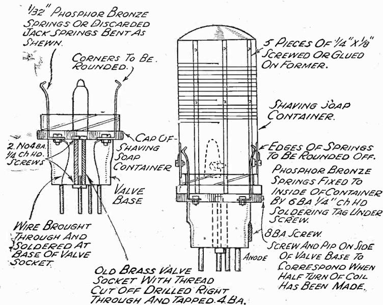
The diagrams explain clearly the idea mentioned by Mr. R. W. Horne for the construction of an easily-changed short-wave coil.
