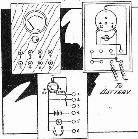
Plan view and wiring diagrams of a simple multi-purpose testing unit.
