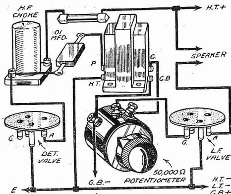
Fig. 2.—Connections for an L.F. volume control when using transformer or resistance-fed transformer coupling.
