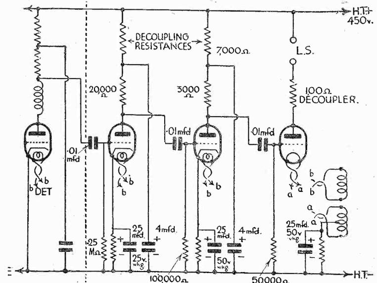
Fig. 2.—Where a succession of L.F. stages is employed, an efficient triode output valve should be used, and one with a large grid swing is necessary to avoid overloading.
