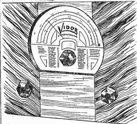
A full-vision scale as fitted to the Vidor receivers.
