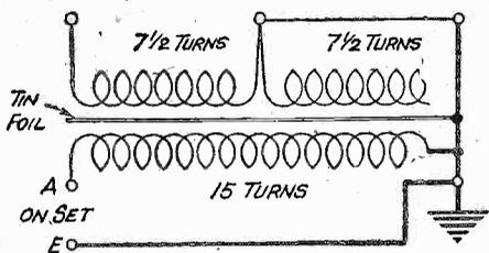
These two diagrams show Mr. Leigh's aerial arrangements; the upper diagram depicting the transformer, and the lower, the arrangement of the aerial wires.
