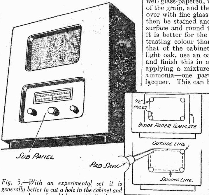
Fig. 5.—With an experimental set it is generally better to cut a hole in the cabinet and use a sub-panel—which can easily be replaced. Methods of making the hole are shown inset.
