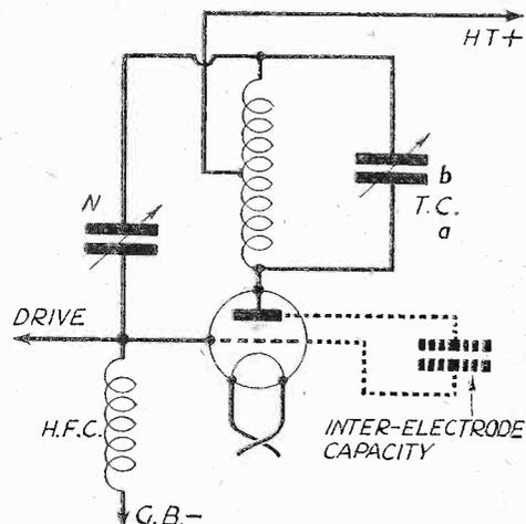
Fig. 3.—Showing how a neutralising condenser is fitted to nullify the inter-electrode capacity.
