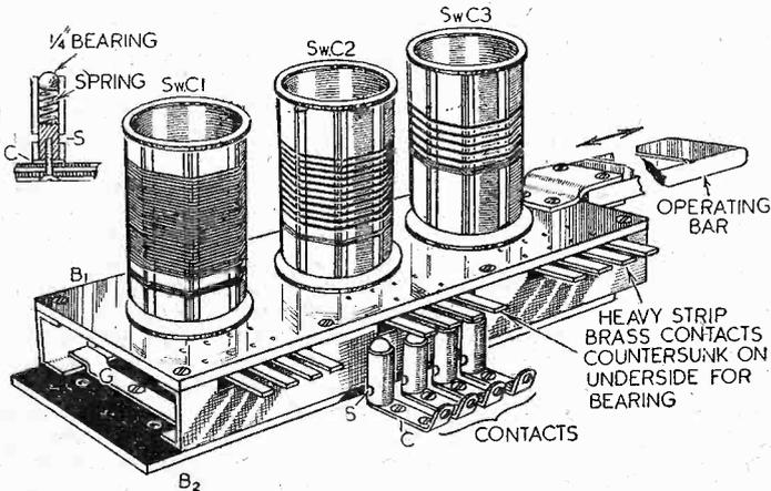
A coil switching unit to avoid coil changing.
