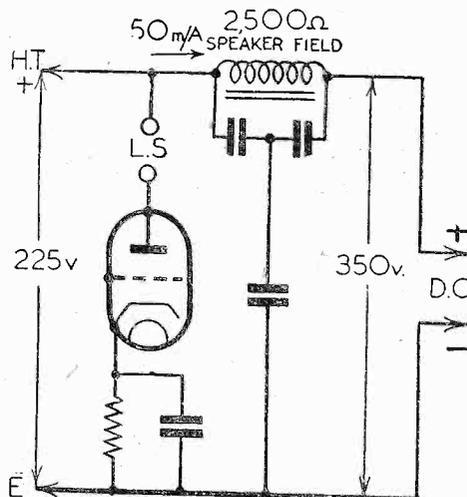
Fig. 6.—A speaker field winding produces a pronounced voltage drop.
