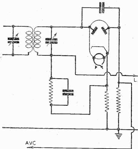
Fig. 2.—The basic form of delayed A.V.C.
