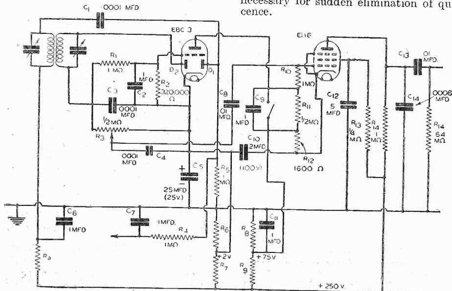
Fig. 5.—An elaborate A.V.C. circuit built round Mullard Type E valves.
