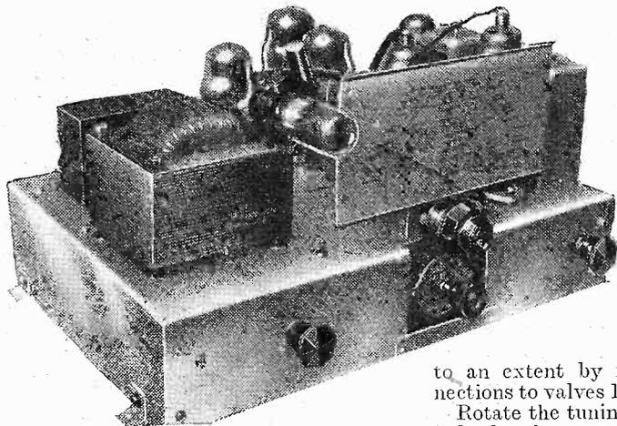
medium-wave station and use as small an aerial as possible. Adjust the trimmers on the top of the I.F. transformers to the loudest setting. Adjust them one at a time, starting from the rear. Note the reading on the dial. If it is not correct, rotate the tuning condenser nearer to its correct setting, but do not entirely lose the station, and again adjust the I.F. transformer trimmers, and repeat this until the dial reading is correct.
