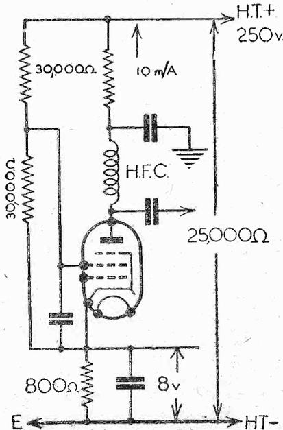
Fig. 2.—Many problems are introduced when an attempt is made to calculate the exact S.G. voltage supplied by a potentiometer, as shown here.
