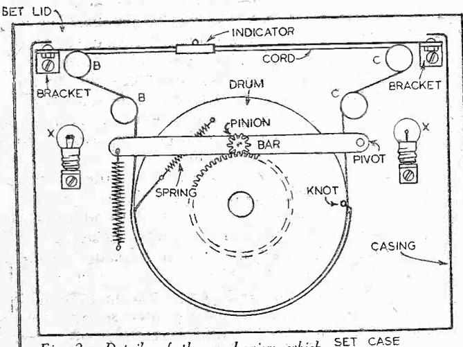
cut about  $\frac{3}{16}$  in. wide. The open end of the drum is towards the outside, and has a gear wheel, about  $\frac{1}{16}$  in. diameter, fixed on the same centre, but about  $\frac{1}{16}$  in. from the drum. This is illustrated clearly in Fig. 3.
