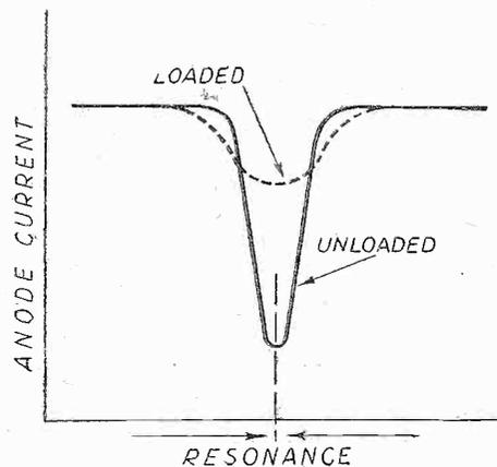
Fig. 2.—A typical anode current curve of a P.A. Note variation when load is applied.
