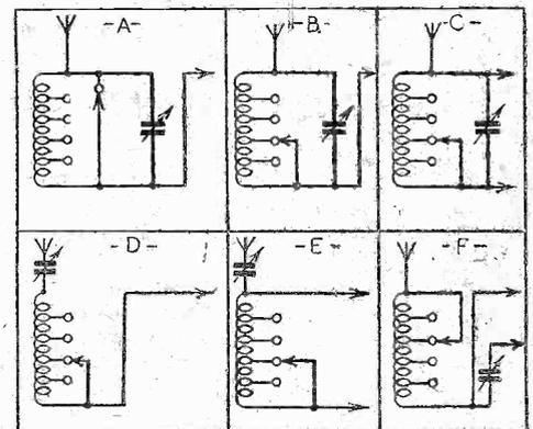
Connections and circuit combinations which are possible with Mr. Marchant's 6-in-1 wave-trap suggestion.
