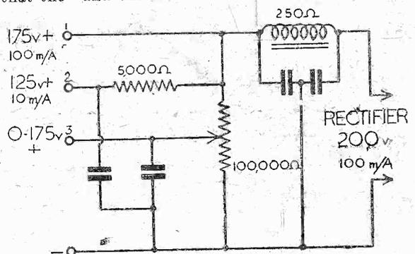
Fig. 3.—The output from different tappings of a mains H.T. unit varies according to the load applied to all of the tappings.
