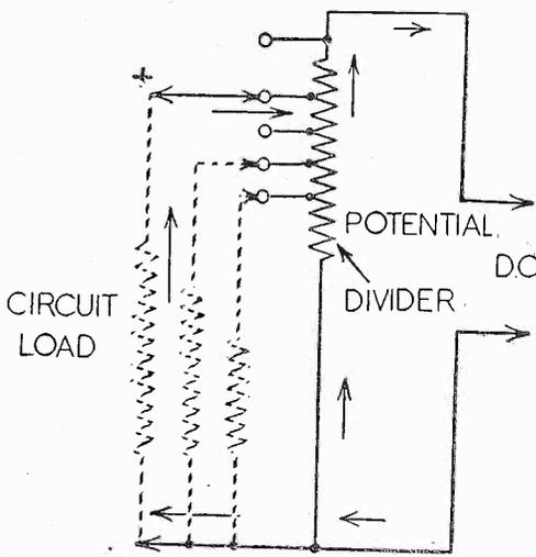
Fig. 4.—When a potential divider is used we have, in effect, a number of resistors in parallel with each other and with parts of the divider resistor.
