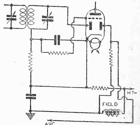
Fig. 4.—This shows one form of amplified and delayed A.V.C.
