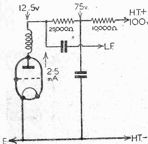
Fig. 1.—A typical R.C.C. coupling, and a decoupling arrangement in the anode circuit of a detector valve.
