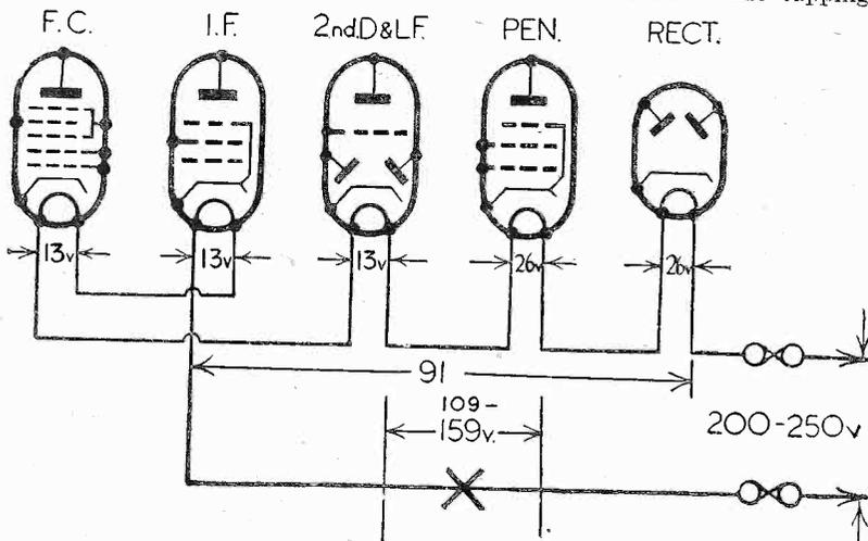
Fig. 5.—The allocation of voltages between the heaters of the valves in an A.C./D.C. circuit.
