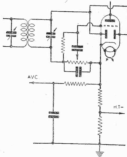
Fig. 3.—Amplified A.V.C. using a double-diode-triode.
