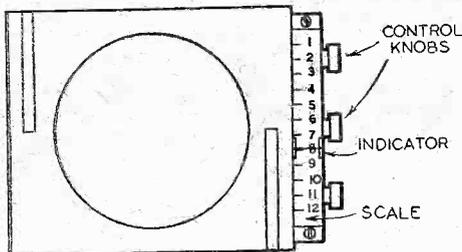
Fig. 1.—Showing the application of the direct control arrangement to a car-radio.
