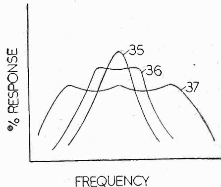
Fig. 2 (left) and Fig. 3 (right).—Curves showing the effects of the variable selectivity device on tuning.
