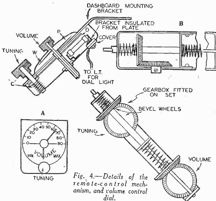
Fig. 4.—Details of the remote-control mechanism, and volume control dial.
