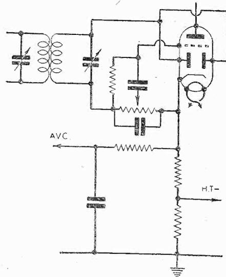
Fig. 3.—Amplified A.V.C. using a double-diode-triode.
