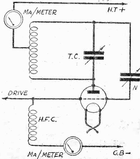
Fig. 1.—A normal neutralised P.A. stage showing where meters should be fitted for preliminary tuning.
