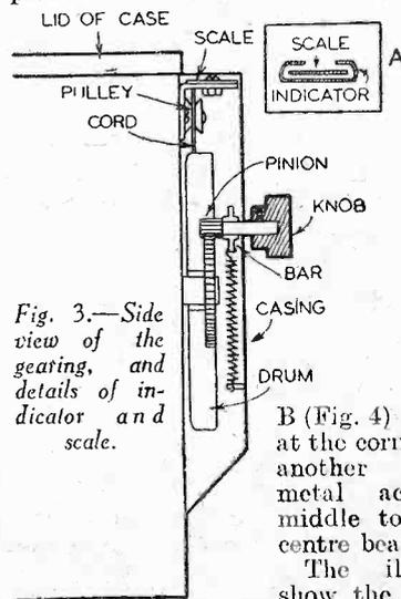
Fig. 3.—Side view of the gearing, and details of indicator and scale.
