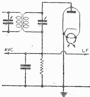
Fig. 1.—The basic circuit for automatic volume control, using a diode.
