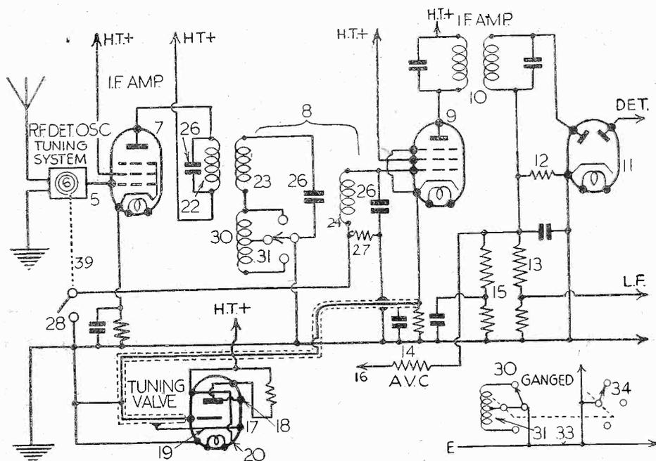
Fig. 1 (above).—Main circuit details incorporating the selectivity scheme mentioned in this article, and Fig. 4 (right) a modification for switching purposes.
