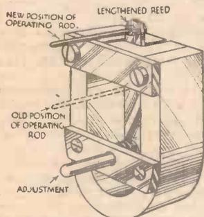
reed below, instead of above, the bobbin and pole pieces. This gave me twice the distance from the pivot and correspondingly greater movement of cone, resulting in a vast improvement in bass re-
