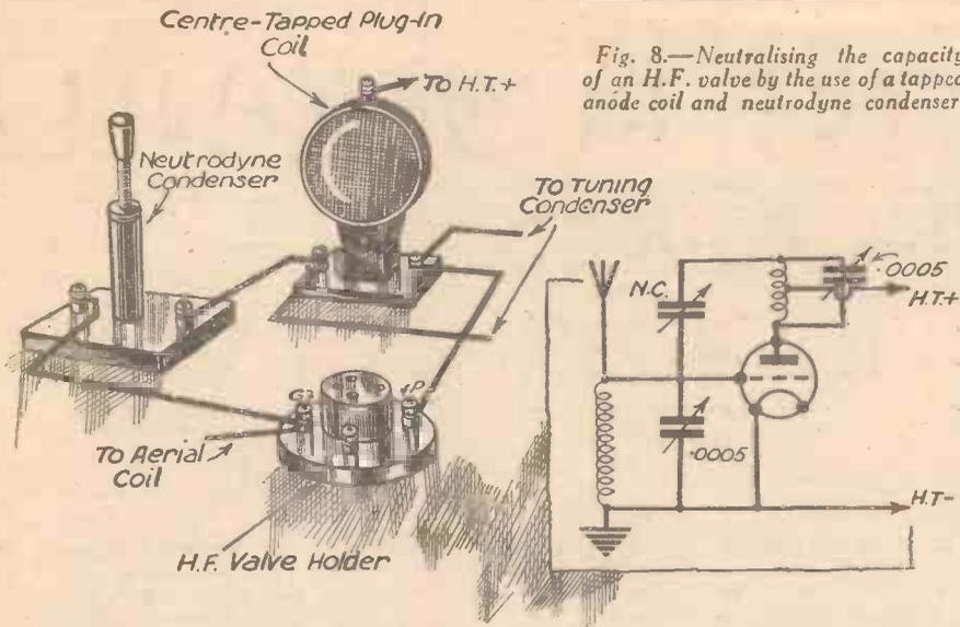
Fig. 8.—Neutralising the capacity of an H.F. valve by the use of a tapped anode coil and neutrodyne condenser.
