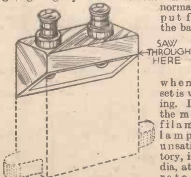
By cutting the top off a fixed condenser as shown it will make a useful terminal block.
