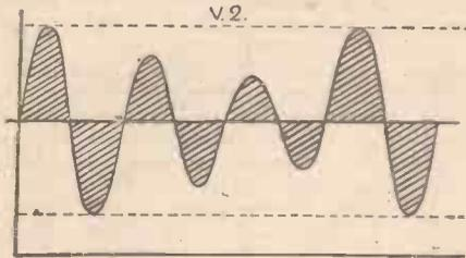
Fig. 6.—One half of an output signal in a push-pull stage.
