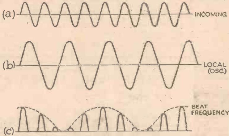
Fig. 3.—A graphic representation of the separate oscillations making up the signal.
