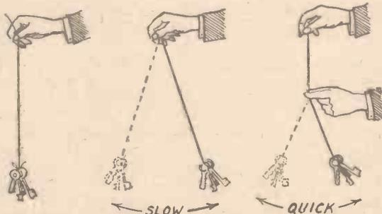
Fig. 8.—A quick way of verifying one of the laws of the pendulum.
