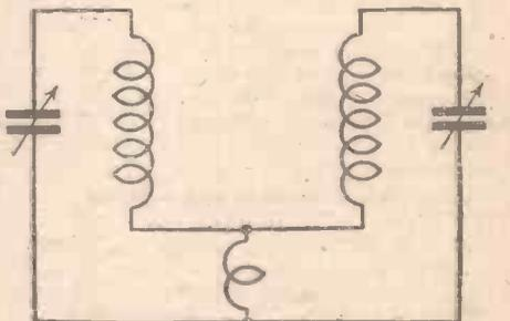
Fig. 4.—Inductive coupling between circuits.
