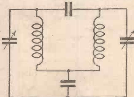
Fig. 2.—Still another method of providing coupling.
