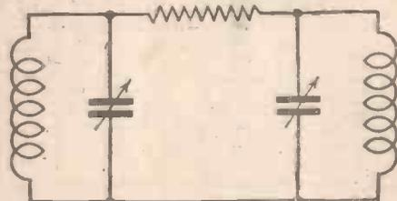
Fig. 3.—Using a resistance for coupling purposes.
