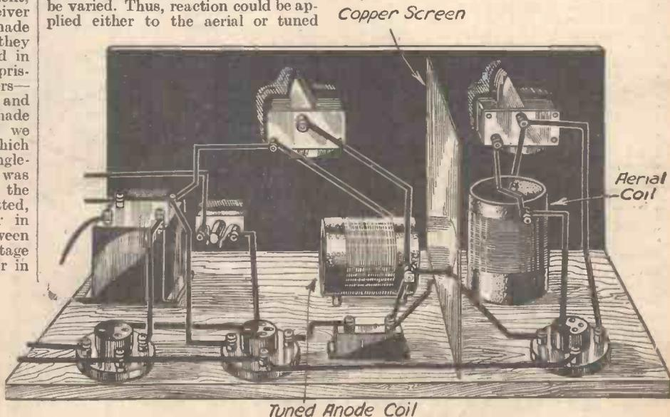
Fig. 11.—The kind of screening first used between large tuning coils of the solenoid type.
