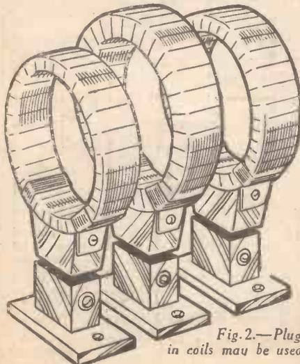
Fig. 2.—Plug-in coils may be used.
