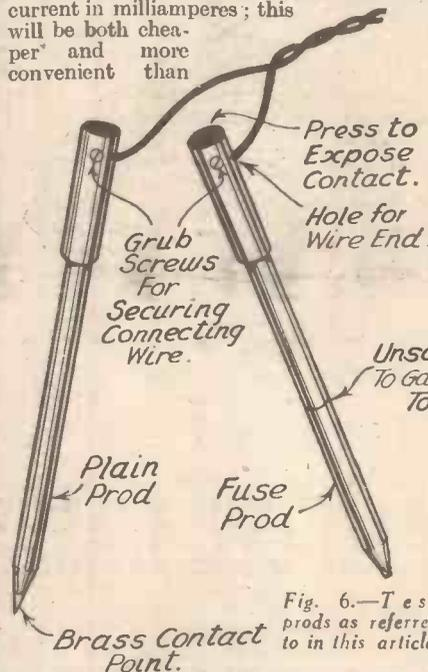
Fig. 6.—Test prods as referred to in this article.
