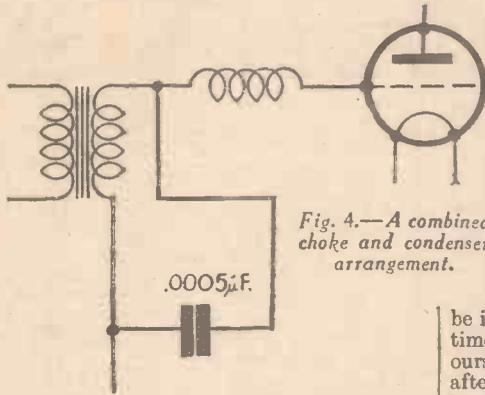
Fig. 4.—A combined choke and condenser arrangement.
