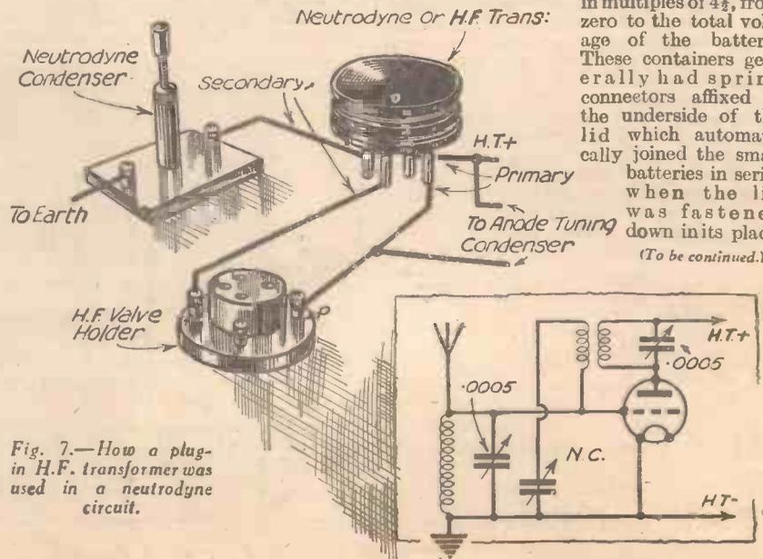
Fig. 7.—How a plug-in H.F. transformer was used in a neutrodyne circuit.
