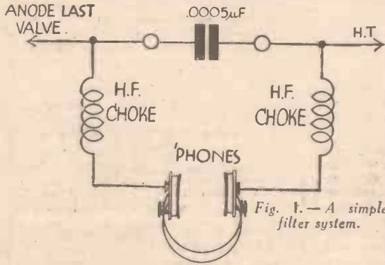
Fig. 1.—A simple filter system.
