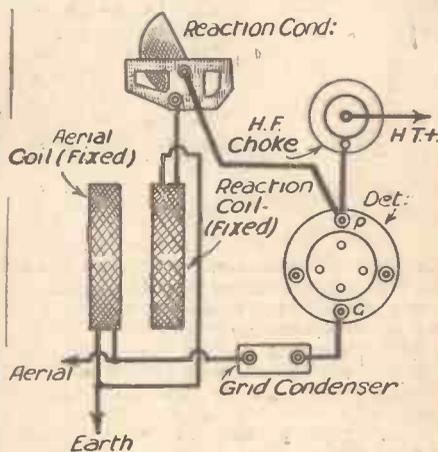
Fig. 10.—Connections for Reinartz or capacity-controlled reaction.
