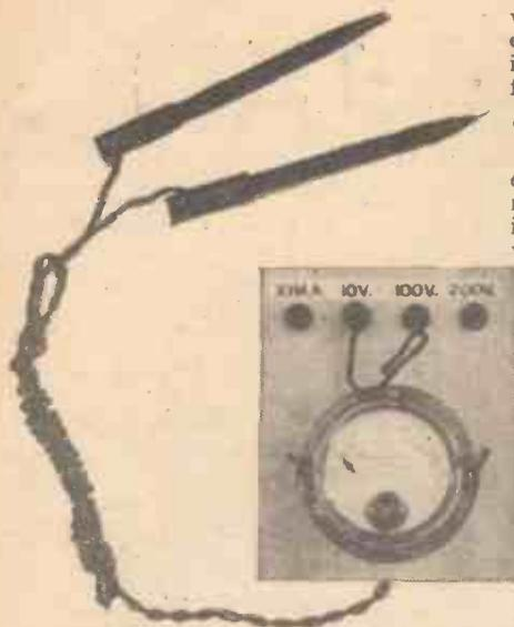
Fig. 3.—A useful home-made four-range meter.
