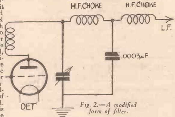
Fig. 2.—A modified form of filter.
