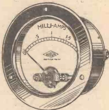
Fig. 1.—A commercial milliammeter.
