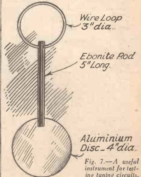
Fig. 7.—A useful instrument for testing tuning circuits.
