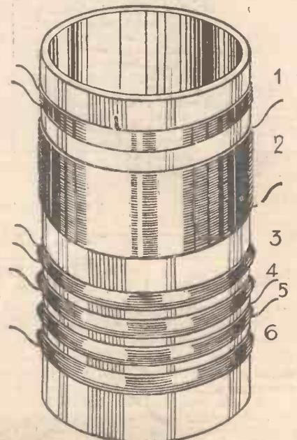
Fig. 3.—A finished dual-range coil as shown in Fig. 6.
