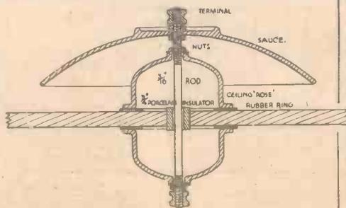
nuts; two terminals; two discs of rubber; a saucer; and a porcelain insulator. These parts are assembled as shown in the drawing. I use this type of lead-in for transmitting work and it will stand a very high voltage test.—R. G. (Swansea).
