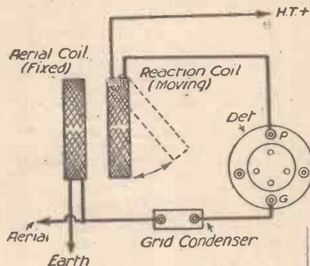
Fig. 9.—Connections for a swinging coil reaction circuit.
