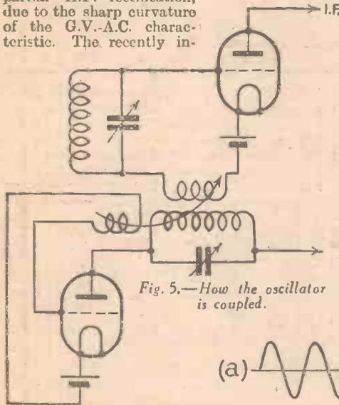
Fig. 5.—How the oscillator is coupled.
