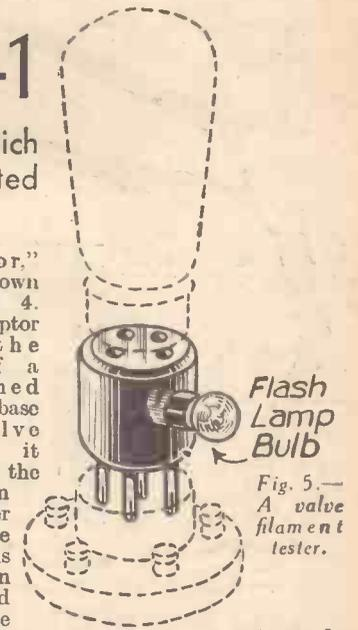
Fig. 5.—A valve filament tester.
