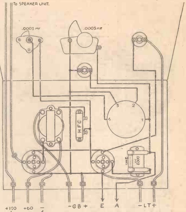
Fig. 4.—Wiring diagram of the Stand-by Two.
