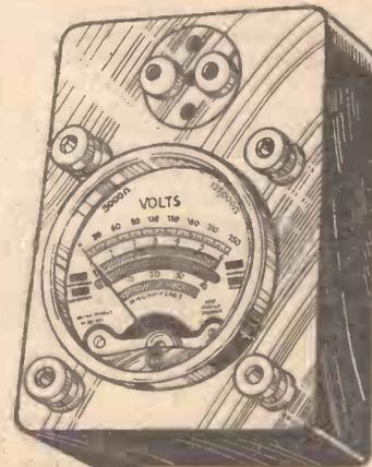
Fig. 2.—A commercial multi-range test-meter.
