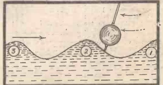
Fig. 6.—The pendulum swinging back in time to meet the second wave.
