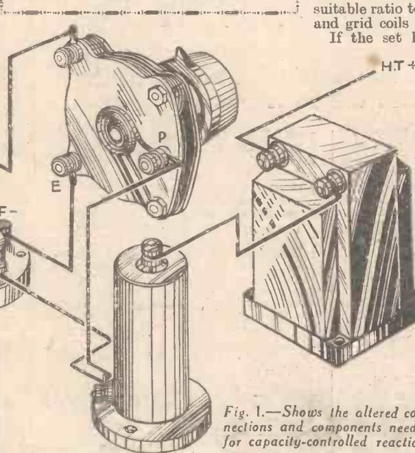
Fig. 1.—Shows the altered connections and components needed for capacity-controlled reaction.
