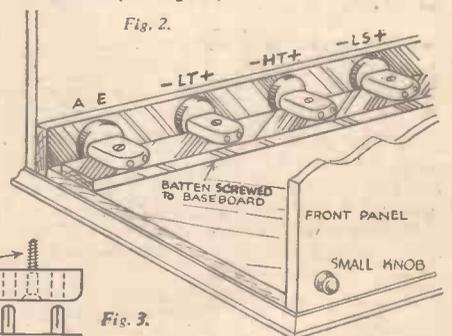
Showing how plug and socket connectors can be used for eliminating terminals.
