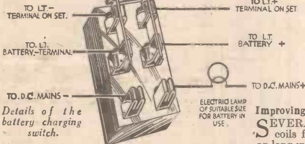
Details of the battery charging switch.
