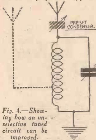
Fig. 4.—Showing how an unselective tuned circuit can be improved.
