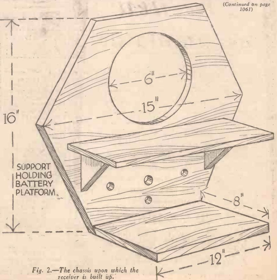
Fig. 2.—The chassis upon which the receiver is built up.
