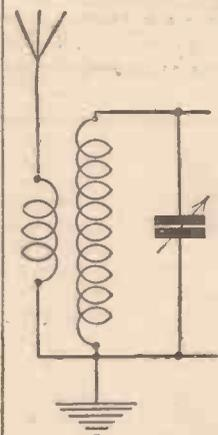
Fig. 5.—A better arrangement for improving an unselective tuned circuit.
