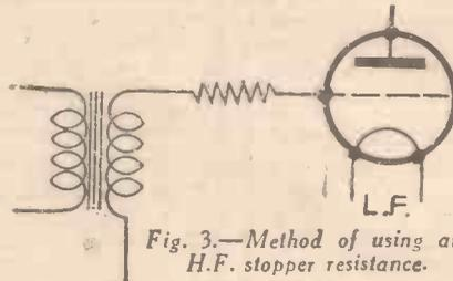
Fig. 3.—Method of using an H.F. stopper resistance.
