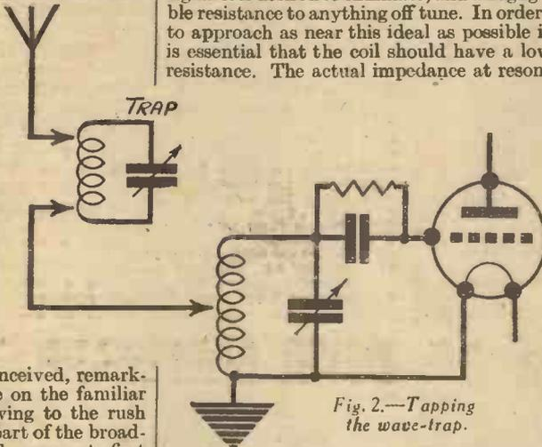
Fig. 2.—Tapping the wave-trap.
