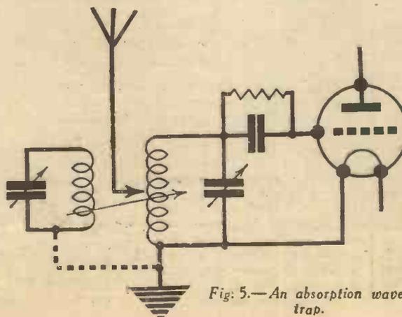
Fig. 5.—An absorption wave-trap.
