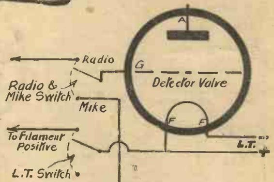
Fig. 4.—Fitting a 2 pole switch for switching in mike and switching out L.T. current of H.F. valve.
