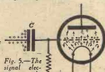
Fig. 5.—The signal electrons on the grid and grid condenser.
