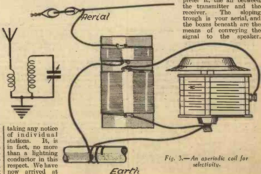
Fig. 3.—An aperiodic coil for selectivity.
