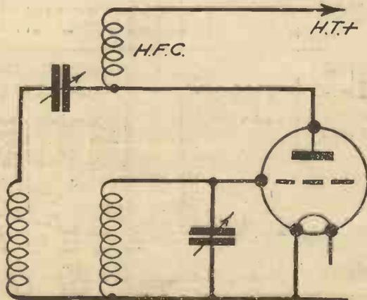
Fig. 2.—A typical reaction circuit.
