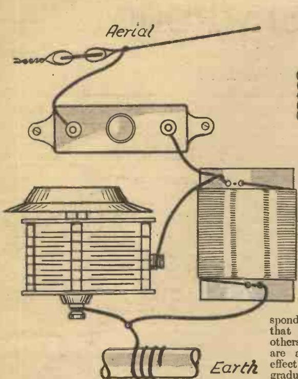
Fig. 4.—A series condenser used to improve selectivity.
