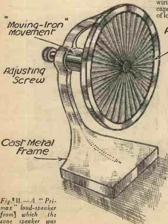
Fig. 11.—A "Primax" loud-speaker from which the cone speaker evolved.
