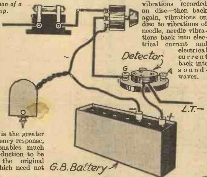
Fig. 2.—Wiring the pick-up into the grid circuit.
