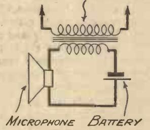
Fig. 2.—The microphone circuit.
