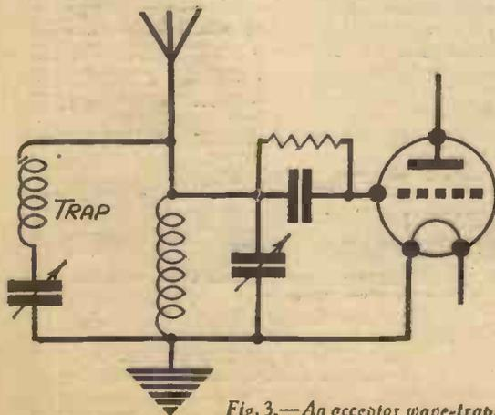
Fig. 3.—An acceptor wave-trap.
