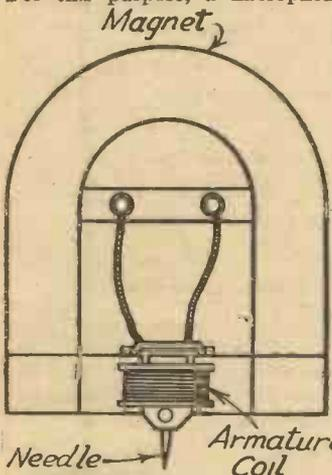
Fig. 1.—The construction of a gramophone pick-up.
