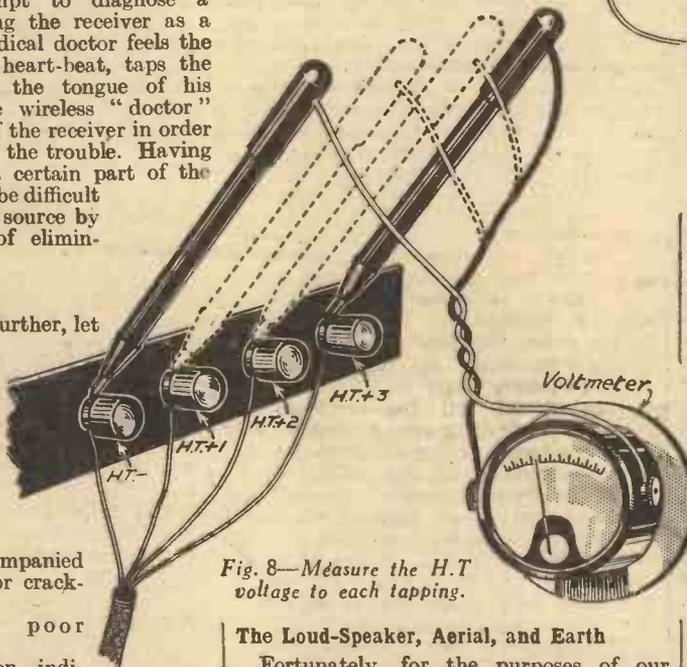
Fig. 8—Measure the H.T. voltage to each tapping.
