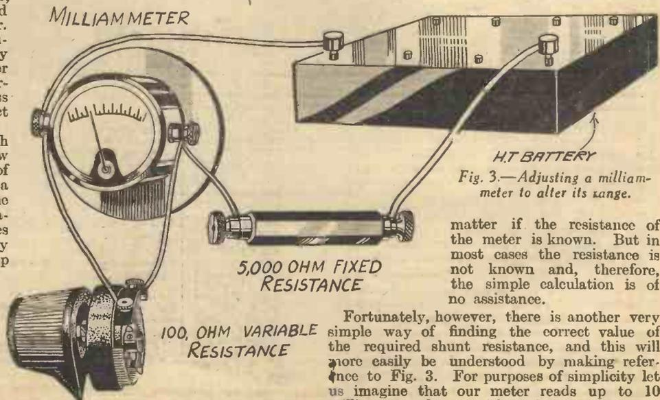
Fig. 3.—Adjusting a milliammeter to alter its range.
