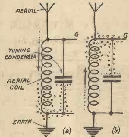
Fig. 3 (a) and (b).—Diagram illustrating the flow of electric currents in the aerial circuit of a receiver.
