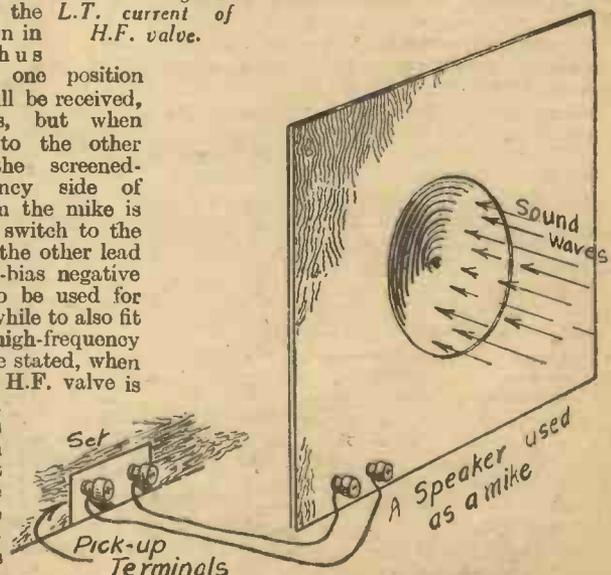
Fig. 2.—Connecting the loud-speaker microphone.
