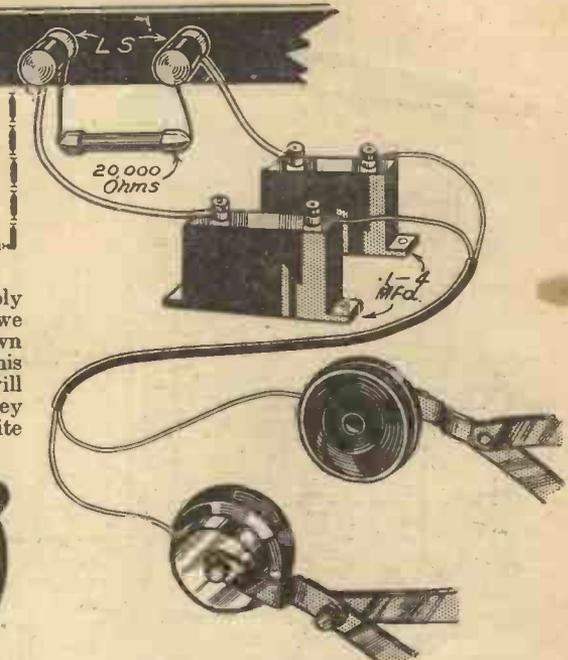
Fig. 7.—The method of connecting a pair of 'phones to the loud-speaker terminals of a powerful set operated from the mains.
