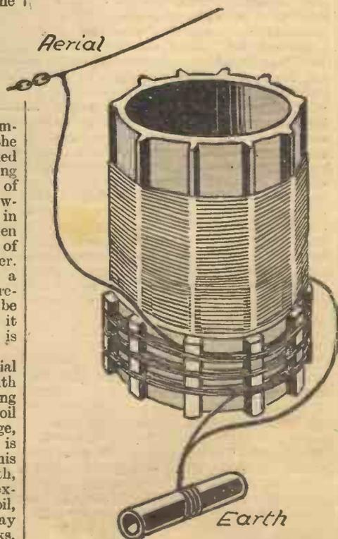
Fig. 5.—Adapting a ready-made coil to improve selectivity.
