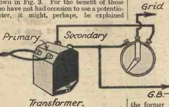
Fig. 5.—Using a transformer to isolate the pick-up.
