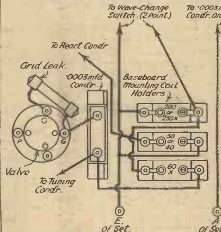
A method of wave-changing with plug-in coils.
