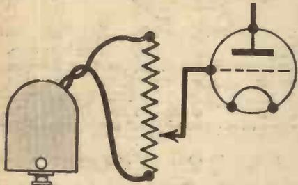
Fig. 4.—Theoretical circuit of pick-up with volume control.
