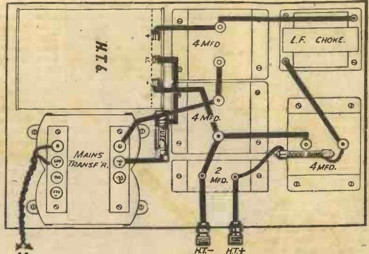
The Westinghouse A.C. Power Unit for operating the Battery Fury Four from A.C. mains. Sets of parts for building this power unit are available from the company mentioned.
