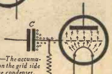
Fig. 6.—The accumulation on the grid side of the condenser.
