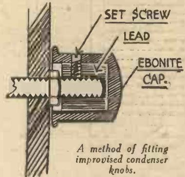
A method of fitting improvised condenser knobs.
