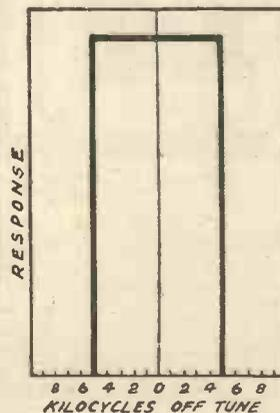
Fig. 2.—Ideal "curve" for a band-pass tuner.
