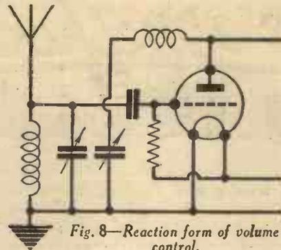
Fig. 8—Reaction form of volume control.
