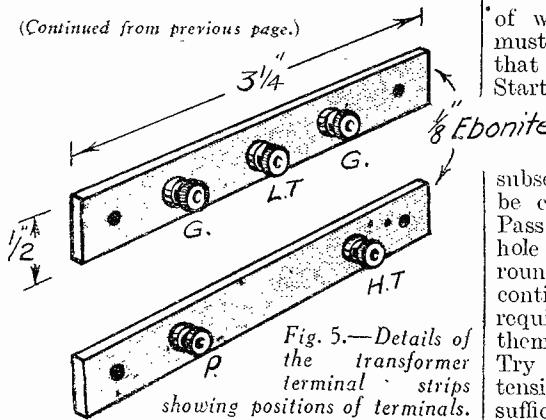
Fig. 5.—Details of the transformer terminal strips showing positions of terminals.
