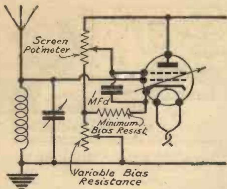
Fig. 7—Connections for A.C. variable mu valve.
