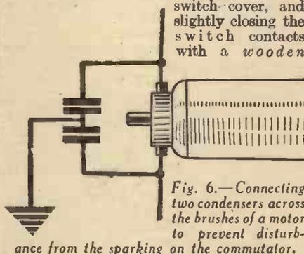
Fig. 6.—Connecting two condensers across the brushes of a motor to prevent disturbance from the sparking on the commutator.
