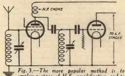
Fig. 3.—The more popular method is to employ a stage of H.F. amplification and to use the second circuit as the coupling between the S.G. valve and the detector.
