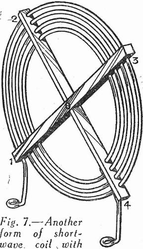
Fig. 7.—Another form of short-wave coil with dimensions of fixing strips.
