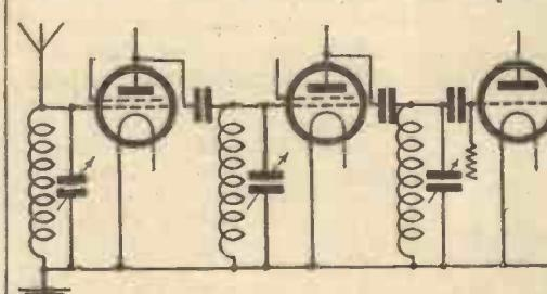
Figs. 4 and 5.—Optional arrangements for three tuned circuits.
