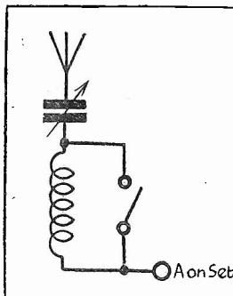
*Fig. 2.—An arrangement for preventing the medium wave station breaking through on long waves.*
