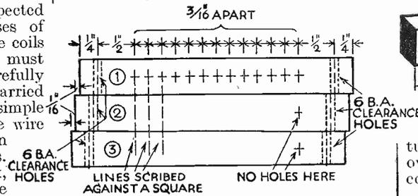
Fig. 2.—How to mark out and cut the coil supports.
