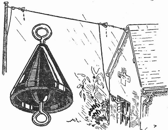
Fig. 1.—Cowl insulator showing method of use.
