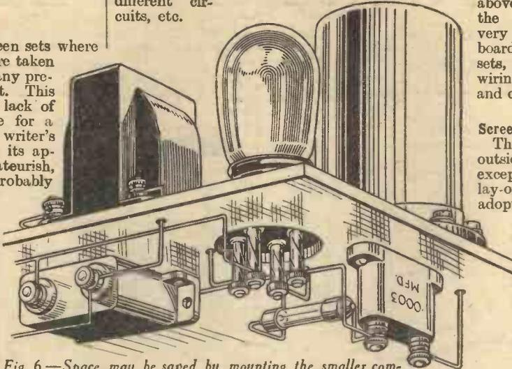
Fig. 6.—Space may be saved by mounting the smaller components "below deck."
