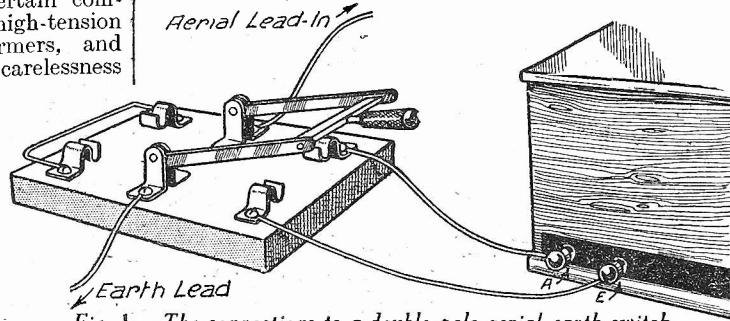
Fig. 1.—The connections to a double-pole aerial-earth switch.
