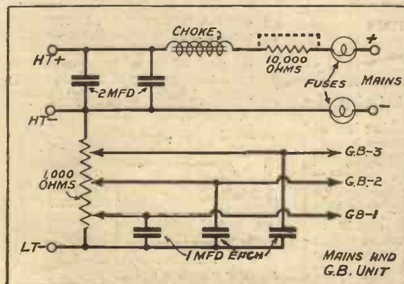
Fig. 3.—The mains and grid bias arrangement.
