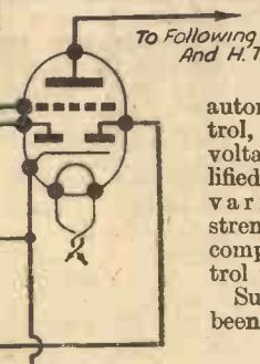
Fig. 6.—Fundamental circuit for using double-diode-triode as full-wave amplifier. For the sake of clearness all decoupling components have been omitted.
