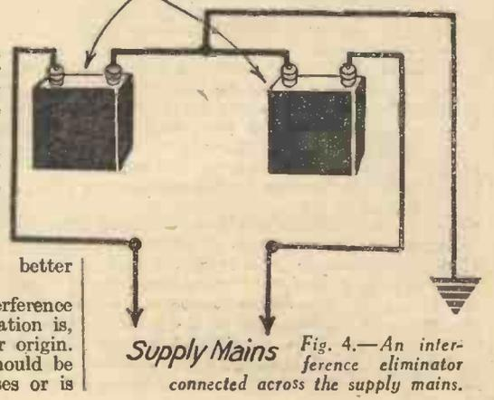
Fig. 4.—An interference eliminator connected across the supply mains.
