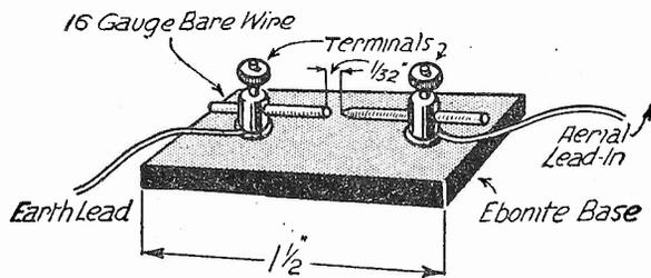
Fig. 3.—A simply made spark gap for connecting between the aerial and earth.
