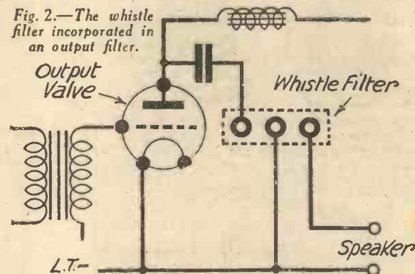
Fig. 2.—The whistle filter incorporated in an output filter.
