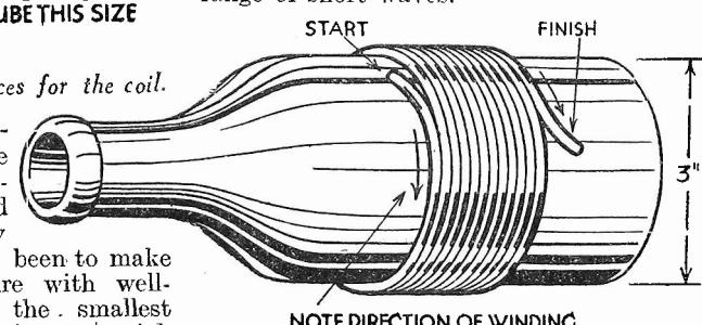
Fig. 4.—Winding the coil round a bottle.
