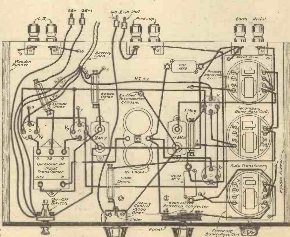
Top and sub-baseboard wiring of the Ferrocant Q.P.-P. Hi-mag Three.
