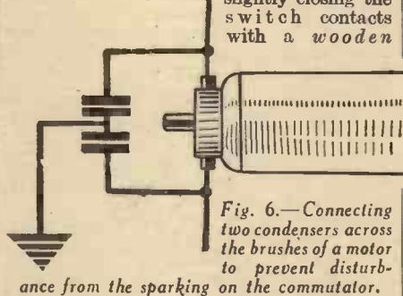
Fig. 6.—Connecting two condensers across the brushes of a motor to prevent disturbance from the sparking on the commutator.
