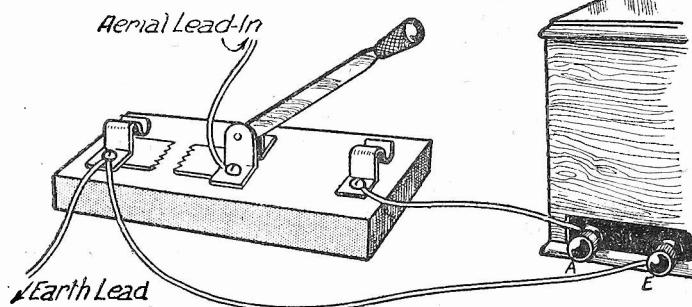
Fig. 4.—A single-pole aerial-earth switch fitted with a spark gap.
