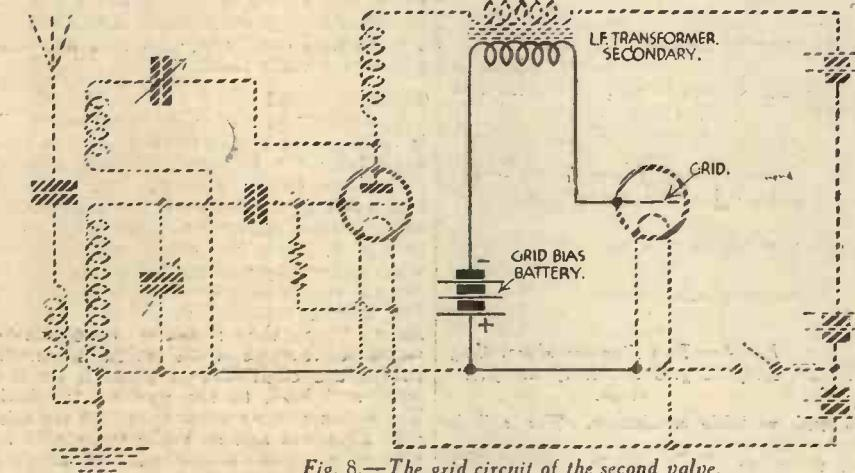
Fig. 8.—The grid circuit of the second valve.
