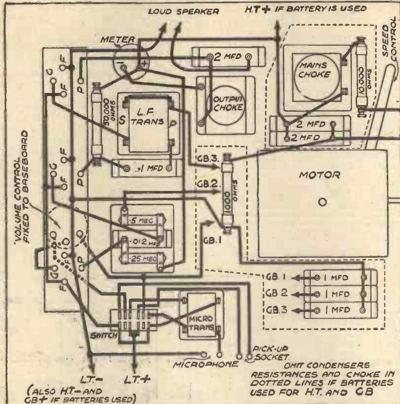
Fig. 6.—Wiring diagram of the outfit.
