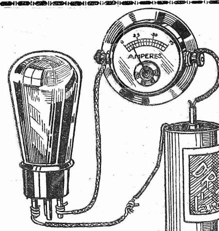
Fig. 6—An ammeter is used to measure current. The illustration shows a valve under test.
