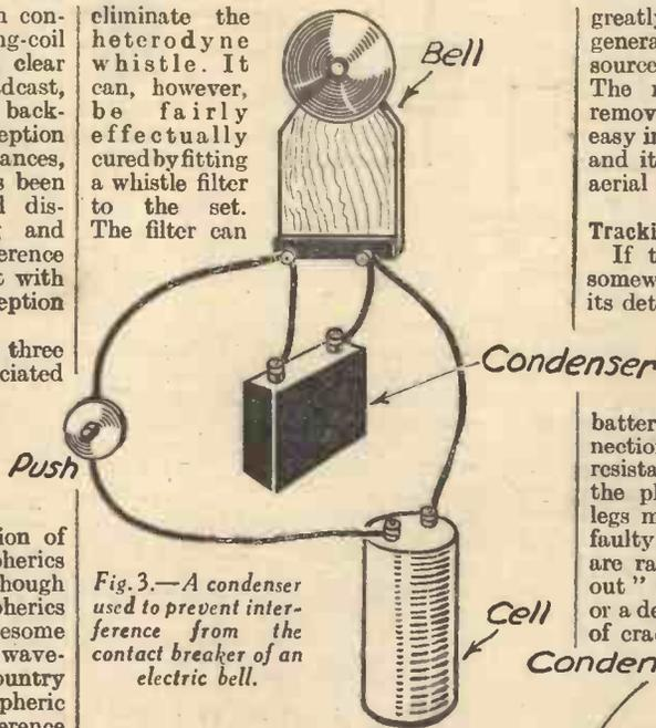
Fig. 3.—A condenser used to prevent interference from the contact breaker of an electric bell.
