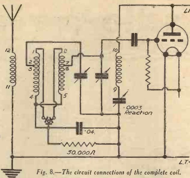
Fig. 8.—The circuit connections of the complete coil.
