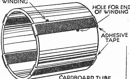
Fig. 8.—The former and adhesive strips for holding another form of coil.
