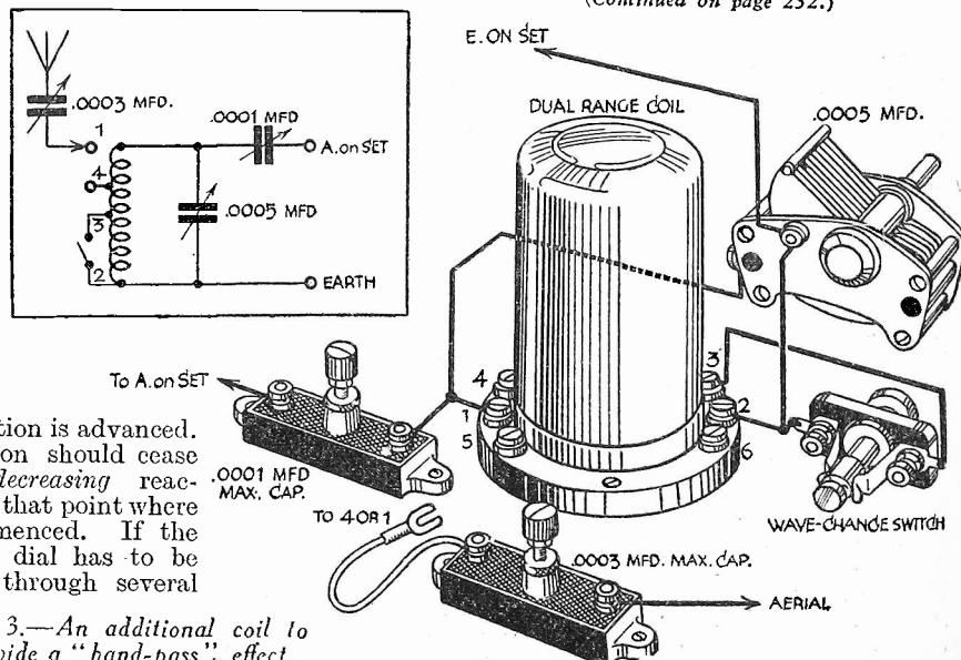
Fig. 3.—An additional coil to provide a "band-pass" effect.
