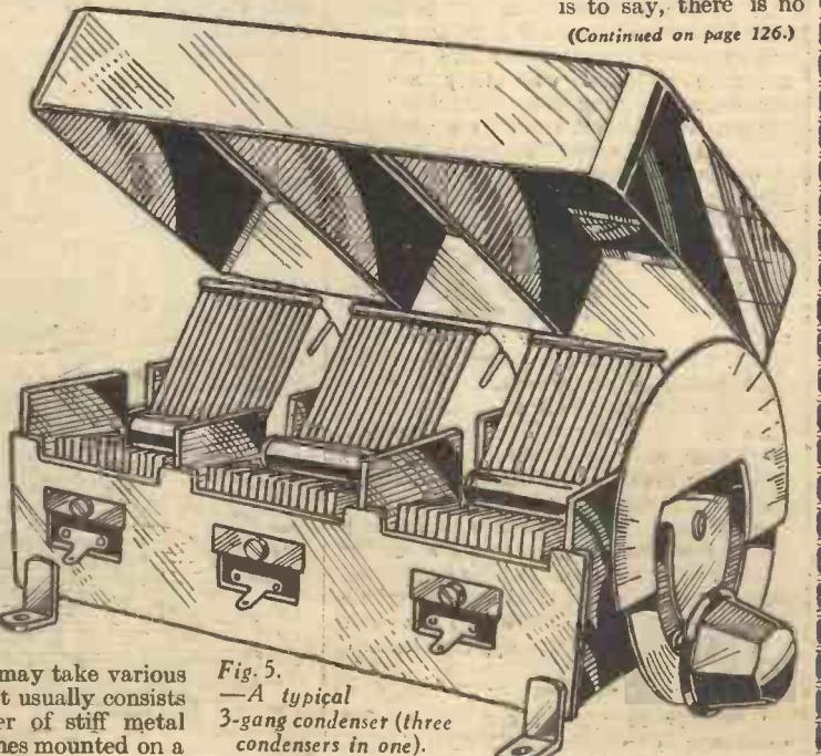
Fig. 5.—A typical 3-gang condenser (three condensers in one).
