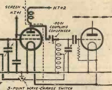
Fig. 2.—Circuit showing how to add an S.G. valve.
