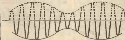
Fig. 3.—The result of half-wave rectification—the "negative" half-cycles have been suppressed.
