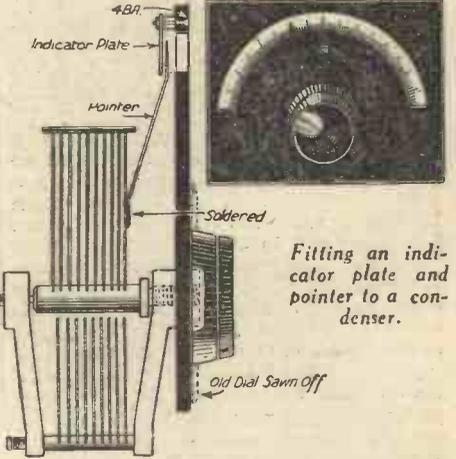
Fitting an indicator plate and pointer to a condenser.
