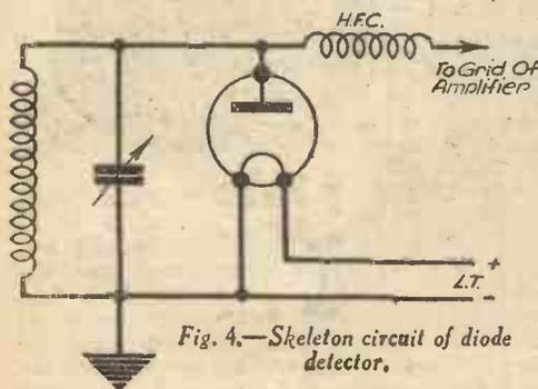
Fig. 4.—Skeleton circuit of diode detector.
