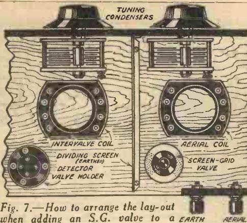
Fig. 7.—How to arrange the lay-out when adding an S.G. valve to a EARTH receiver.
