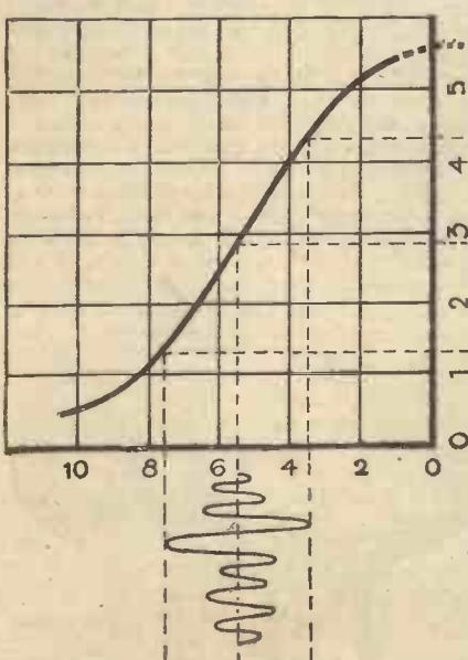
Fig. 1.—The curve of a valve biased to give even amplification. The lower line gives grid volts, and the right-hand line gives anode current.
