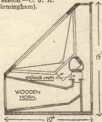
Fig. 2.—Sectional view of speaker.
