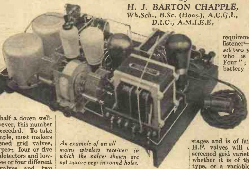
An example of an all mains wireless receiver in which the valves shown are not square pegs in round holes.
