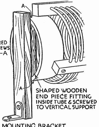
Fig. 6.—The coil supports and method of attaching the coil.
