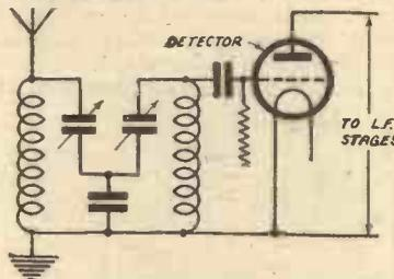
Fig. 2.—One way to employ two tuned circuits is to place them both before the detector.
