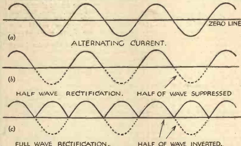
Fig. 1.—(a) The method of showing alternating current.
