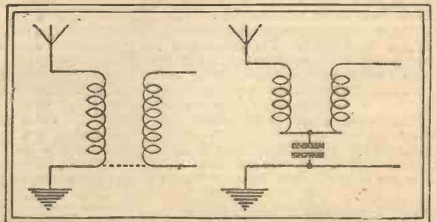
Fig. 6—Diagrams showing inductive coupling (left) and capacitive coupling (right).
