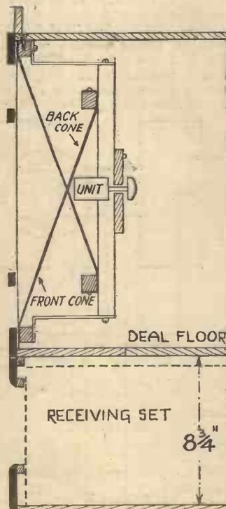
Fig. 4.—Section through set and speaker.
