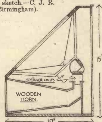
Fig. 2.—Sectional view of speaker.
