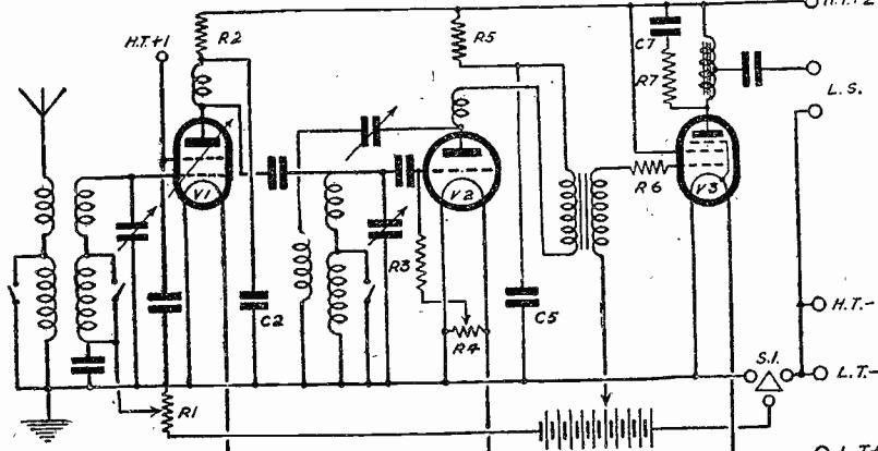
Fig. 1.—A typical battery operated three-valve set showing the various resistances used.
