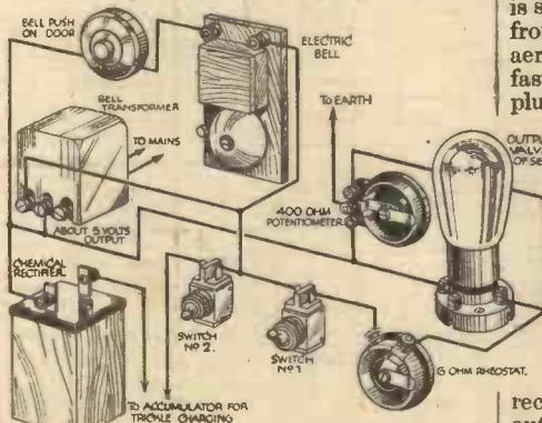
A novel way of using a bell transformer.
