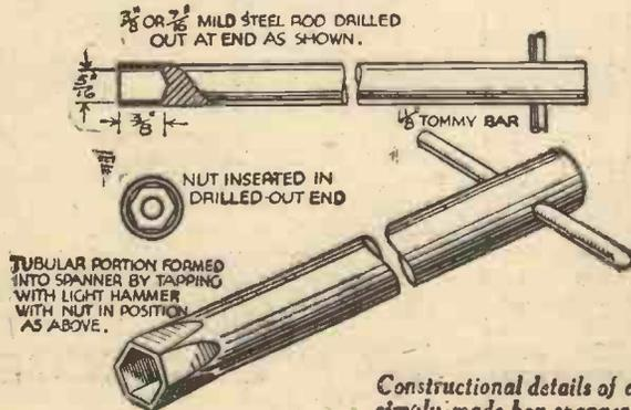
Constructional details of a simply-made box spanner.
