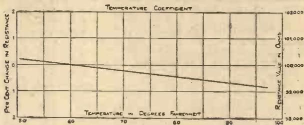
For every one degree centigrade rise in temperature the change in resistance value of a Dubilier resistance is only .04%. The small effect of this change in the resistance value under normal working conditions is emphasised by the curve shown herewith, the right-hand scale of which gives the actual resistance values of a 100,000 ohm resistance at various temperatures; while the left-hand scale gives the average percentage changes.
