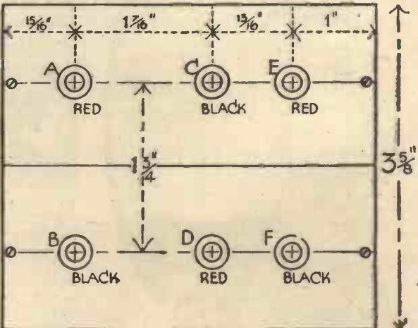
Fig. 2.—Drilling dimensions for the ebonite top.
