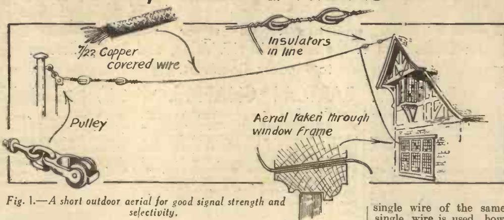
Fig. 1.—A short outdoor aerial for good signal strength and selectivity.
