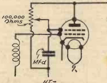
Fig. 5—Variation of screen voltage mains connections.
