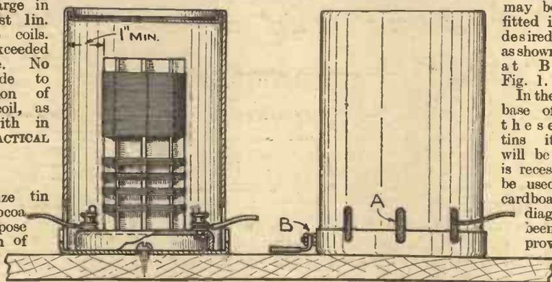
Fig. 1.—Section and elevation of the home-made coil screens.
