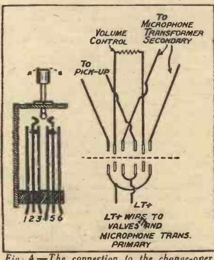
Fig. 4.—The connection to the change-over switch.
