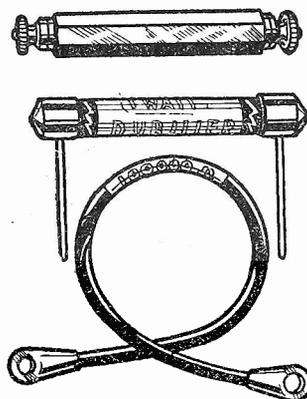
Fig. 3.—Three types of resistances suitable for decoupling purposes in the early stages of a battery set.
