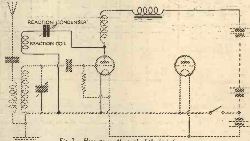
Fig. 7.—Here we see the path of the high-frequency currents which provide reaction.
