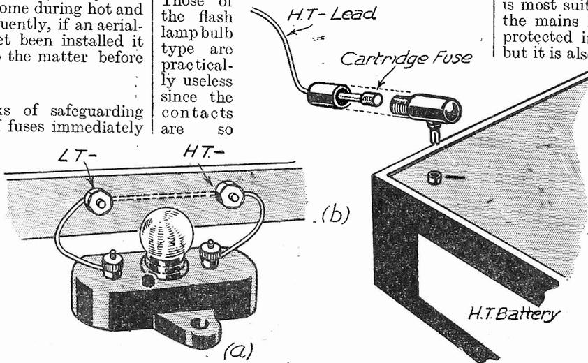
Fig. 7. Two ways of fitting a fuse to a battery set.
