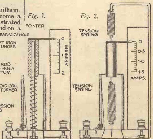
Two home-made high-reading ammeters.
