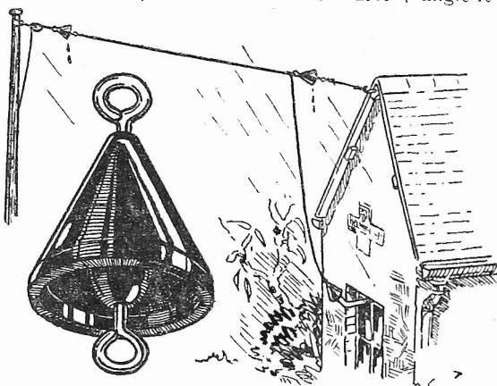
Fig. 1.—Cowl insulator showing method of use.
