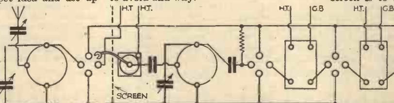
Fig. 3.—Shows the chain of essential components in a 4-valve S.G. receiver, arranged and connected in the simplest possible manner.
