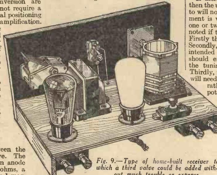
Fig. 9.—Type of home-built receiver to which a third valve could be added without much trouble or expense.
