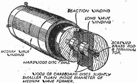
A neat method of making a dual-wave coil.
