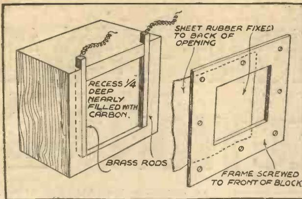
Fig. 10.—A simple carbon microphone.
