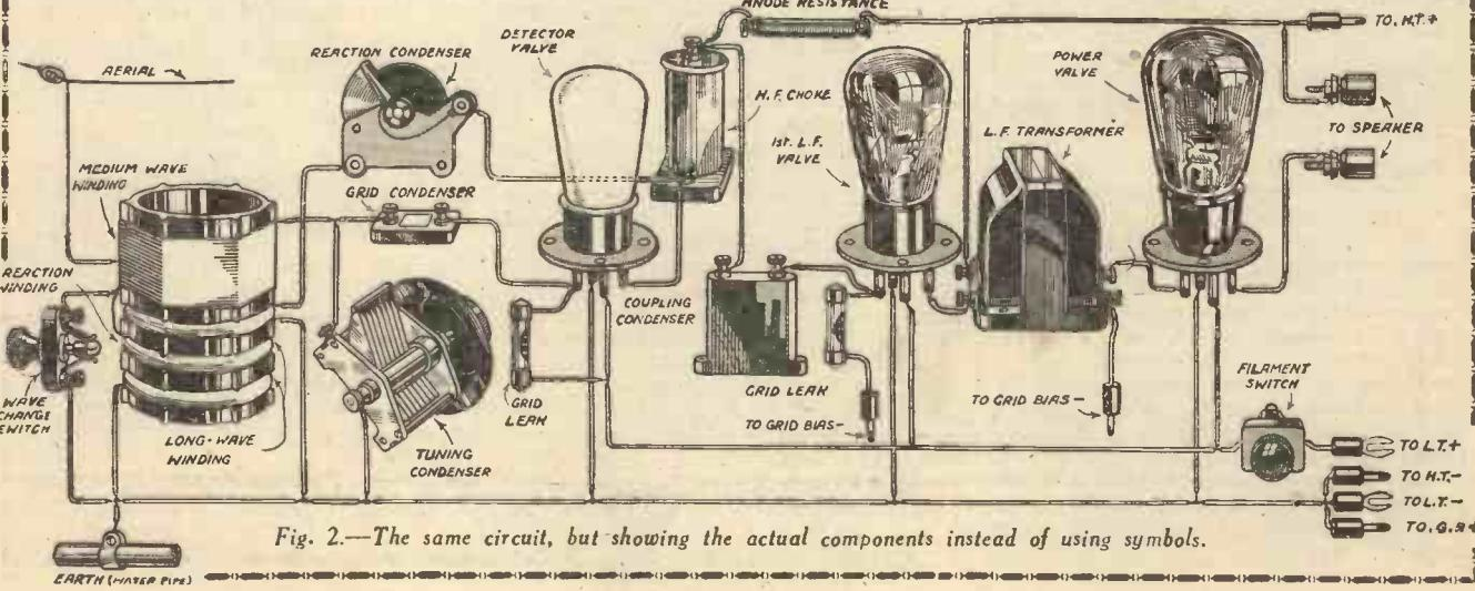
Fig. 2.—The same circuit, but showing the actual components instead of using symbols.
