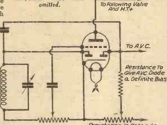
Fig. 7.—Fundamental circuit for using double-diode-triode as half-wave rectifier, L.F. amplifier and delayed automatic volume control valve.
