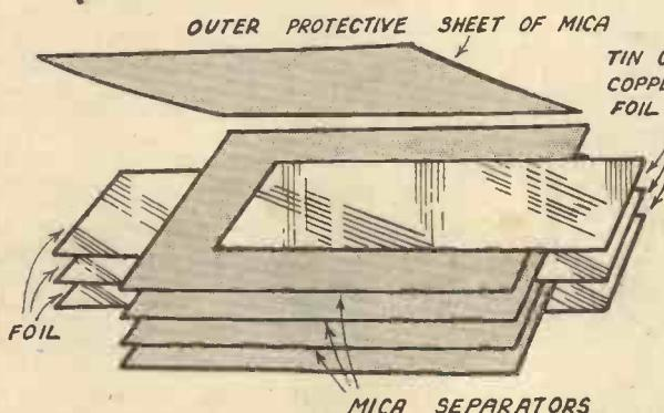
Fig. 1.—How a fixed condenser is built up.
