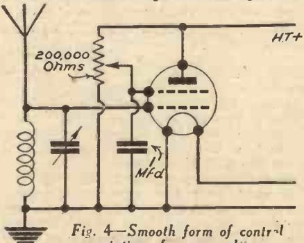
Fig. 4—Smooth form of control variation of screen voltage.
