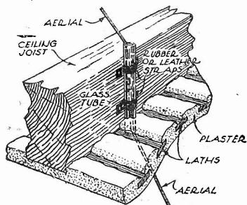
Method of taking a down lead through a ceiling.
