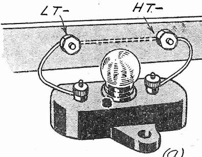
Fig. 7. Two ways of fitting a fuse to a battery set.
