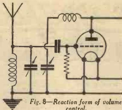
Fig. 8—Reaction form of volume control.
