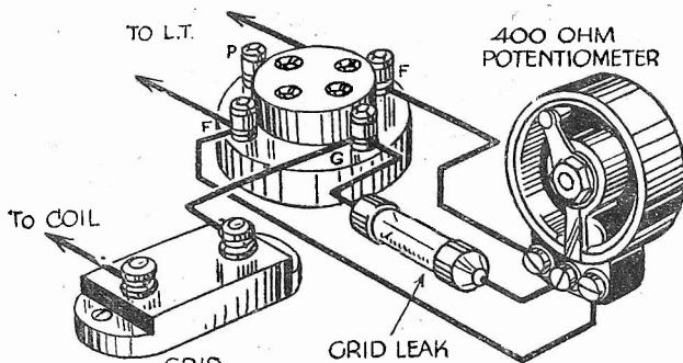
*Fig. 1.—Obtaining smooth reaction.*
