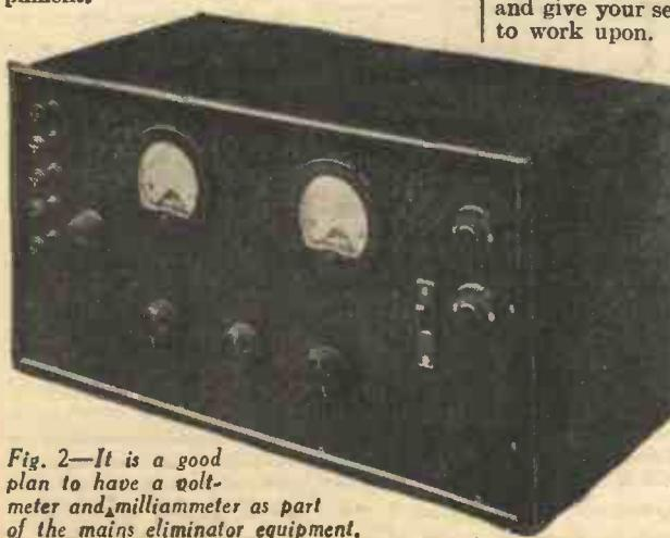
Fig. 2.—It is a good plan to have a voltmeter and milliammeter as part of the mains eliminator equipment.
