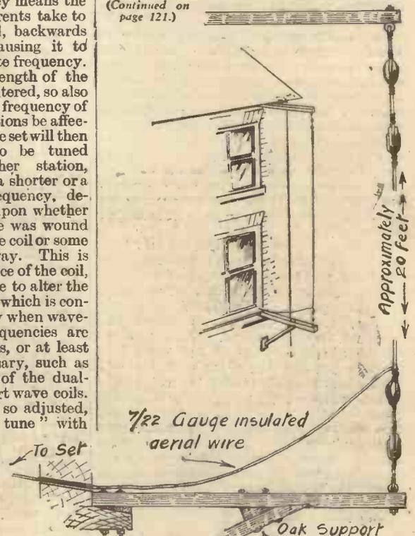
Fig. 2.—A vertical aerial held well away from the wall approximately 20 ft. high, will give very good results.
