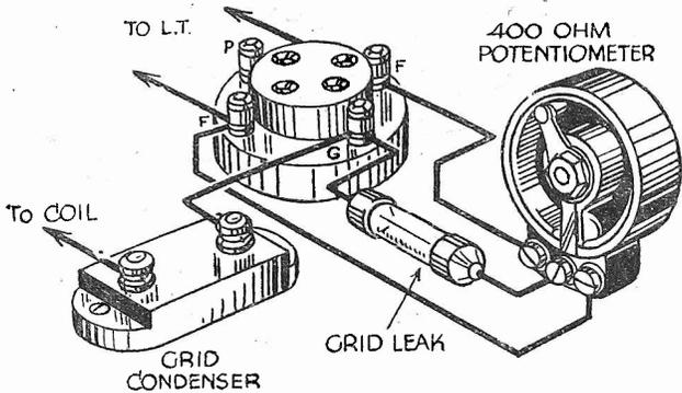
Fig. 1.—Obtaining smooth reaction.
