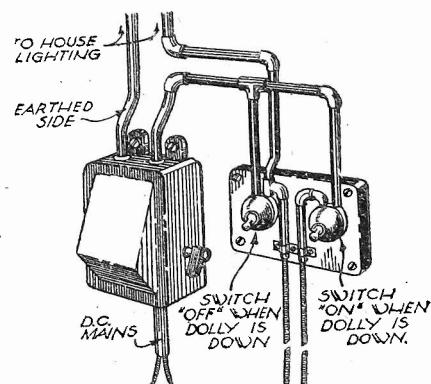
A handy accumulator switching arrangement. ACCUMULATOR.
