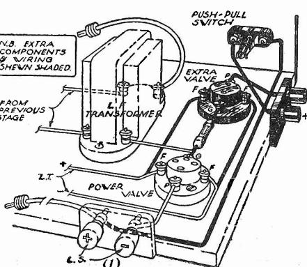
Connecting output valves in series-parallel.
