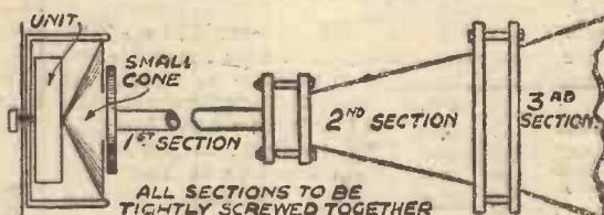
Fig. 8.—Method of building up the loud-speaker.
