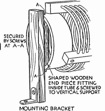
Fig. 6.—The coil supports and method of attaching the coil.
