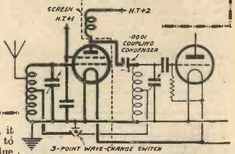
Fig. 2.—Circuit showing how to add an S.G. valve.
