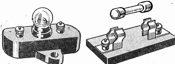
Figs. 5 & 6. Two types of fuses and holders : (5) a flash-lamp bulb fuse and (6) a cartridge fuse
