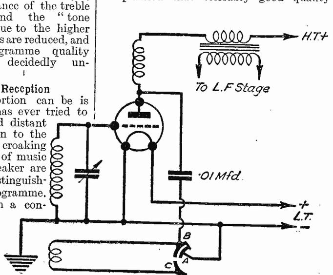
Fig. 3.—Simple connections for an automatic tone balance circuit.
