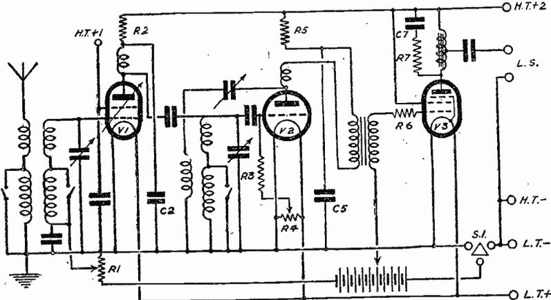
Fig. 1.—A typical battery operated three-valve set showing the various resistances used.
