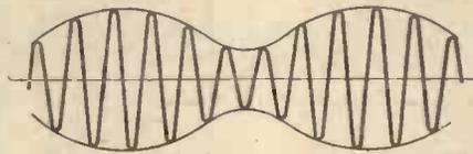
Fig. 1.—Modulated H.F. signal.
