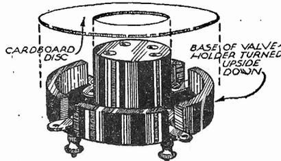
Adapting an ordinary valve-holder for chassis mounting.
