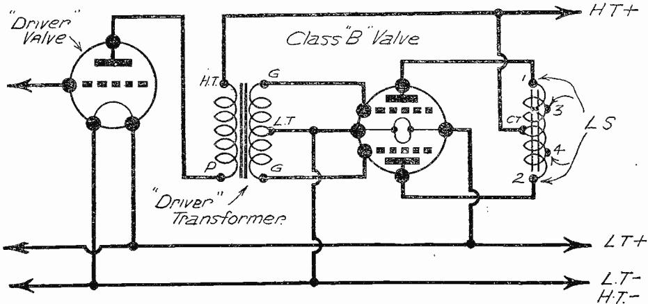
Fig. 1.—Circuit diagram of Class "B" amplifier.
