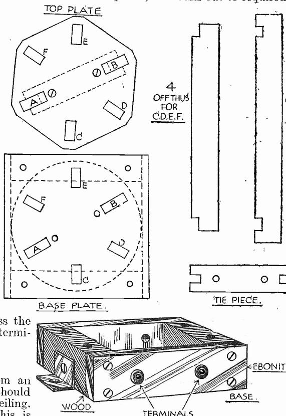
Details of a coil former made from scrap ebonite.
