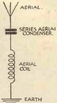
Fig. 2.—The aerial-earth circuit.
