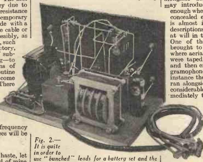
Fig. 2.—It is quite in order to use "bunched" leads for a battery set and the neat effect is shown here.
