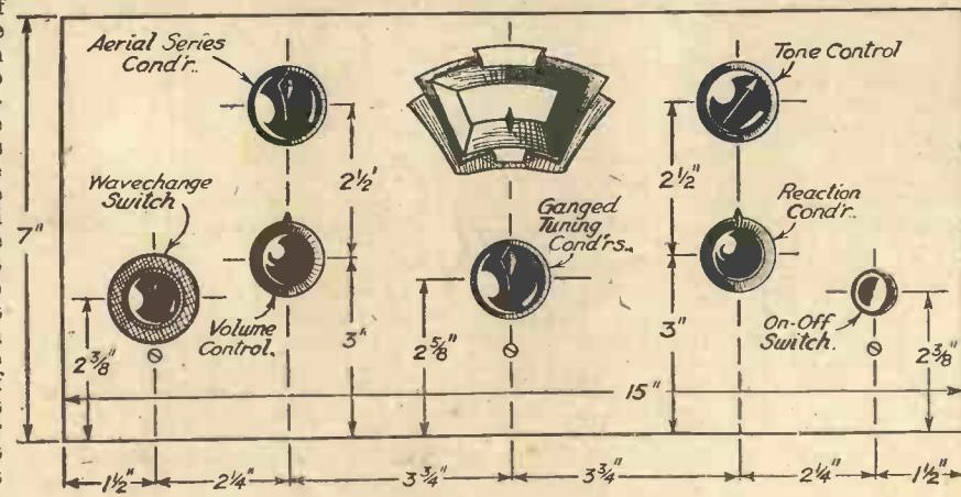
Fig. 2.—Panel-drilling dimensions.
