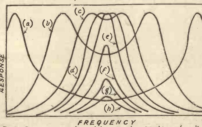
Fig. 1.—Resonance curves of a coupled circuit with various degrees of coupling.
