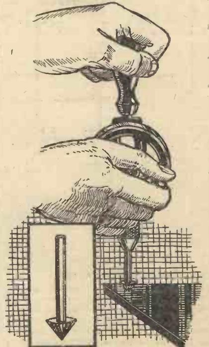
Fig. 2.—Countersinking an ebonite panel. Inset, countersink drill.
