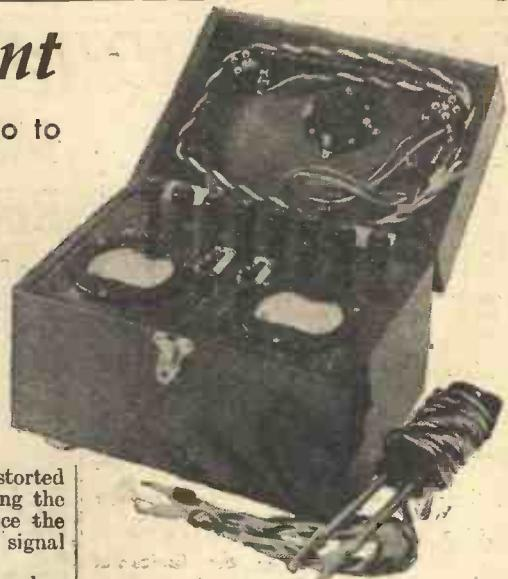
Fig. 1.—A good multi-purpose test set for carrying out measurements on a set to ensure absence of distortion.
