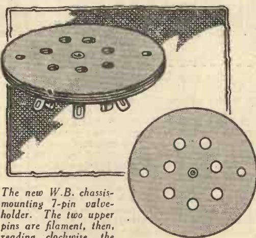
The new W.B. chassis-mounting 7-pin valve-holder. The two upper pins are filament, then, reading clockwise, the others are the anode, grid, grid, anode, and a blank.
