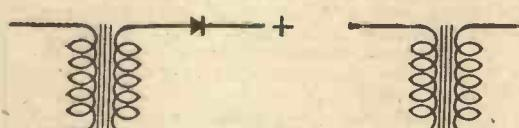
Fig. 2.—Circuit diagram of a half-wave rectifier, and a full-wave rectifier.
