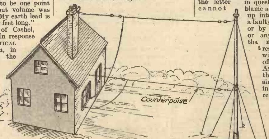
Fig. 2.—A counterpoise earth is often useful in reducing electrical interference.
