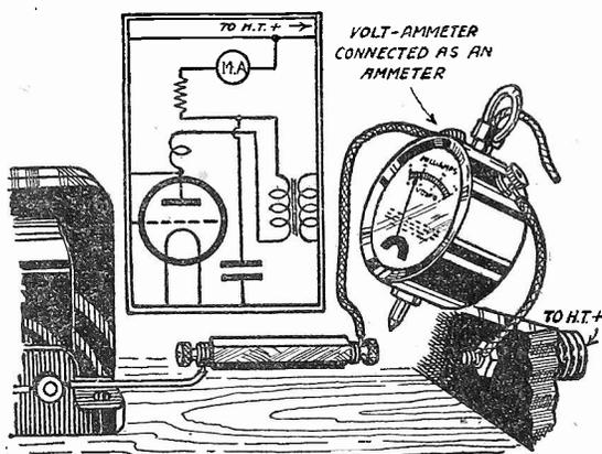
Fig. 4.—Testing the current passing through a resistance in the anode circuit of a valve.
