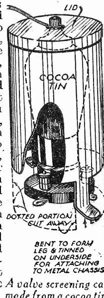
A valve screening can be made from a cocoa tin.
