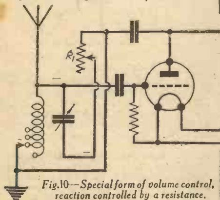
Fig. 10—Special form of volume control, reaction controlled by a resistance.
