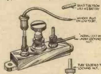
Using a plug and socket to cut out a condenser.
