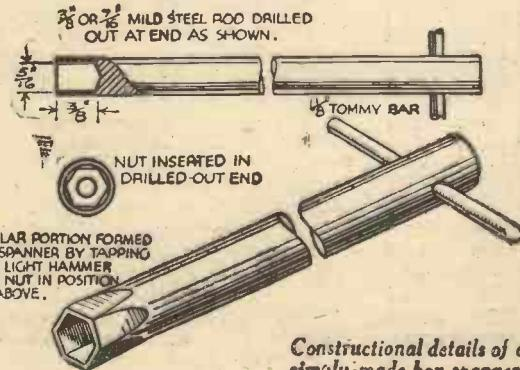
Constructional details of a simply-made box spanner.
