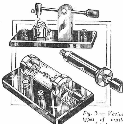
Fig. 3 — Various types of crystal detector.
