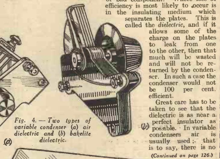
Fig. 4.—Two types of variable condenser (a) air dielectric and (b) bakelite dielectric.
