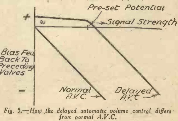
Fig. 5.—How the delayed automatic volume control differs from normal A.V.C.
