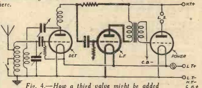
Fig. 4.—How a third valve might be added to the two-valver of Fig. 3.
