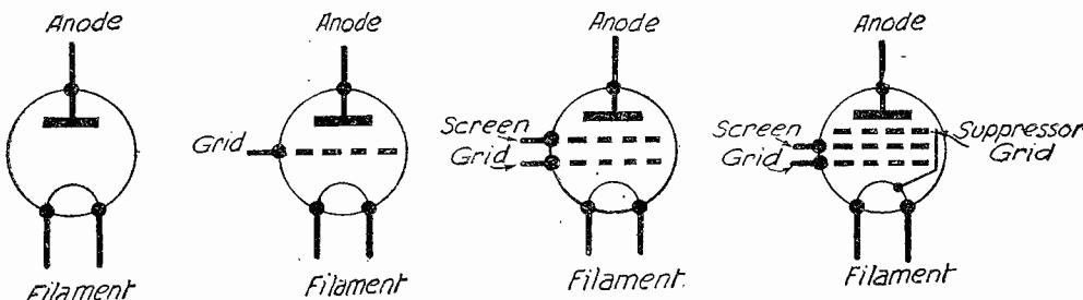
Fig. 1.—The evolution of the pentode valve.
