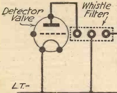
Fig. 1.—Including a whistle filter in the L.F. stage before a coupling device.
