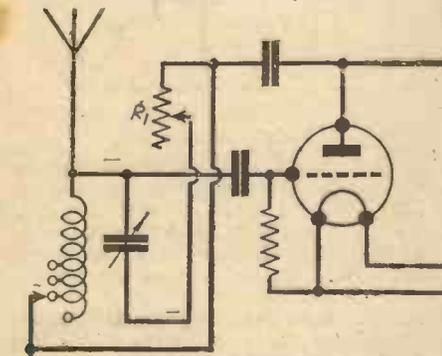
Fig. 10—Special form of volume control, reaction controlled by a resistance.
