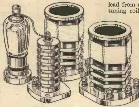
Fig. 2.—Unscreened coils and chokes should not be mounted near one another.
