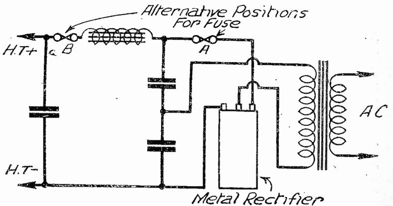
Fig. 9.—Fitting a fuse in a mains unit.
