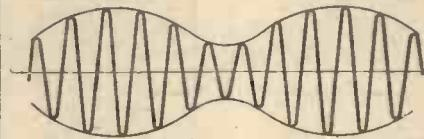
Fig. 1.—Modulated H.F. signal.
