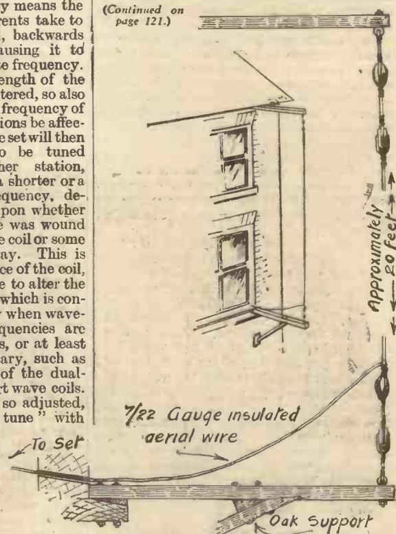
Fig. 2.—A vertical aerial held well away from the wall approximately 20 ft. high, will give very good results.
