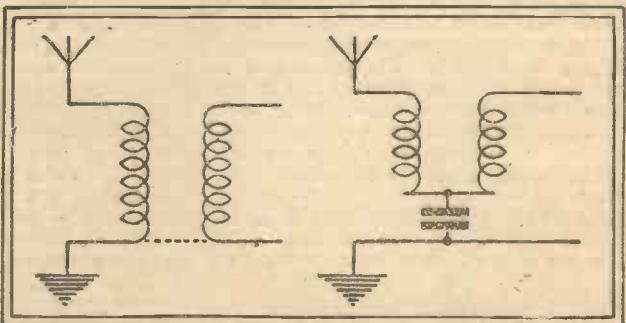
Fig. 6.—Diagrams showing inductive coupling (left) and capacitative coupling (right).
