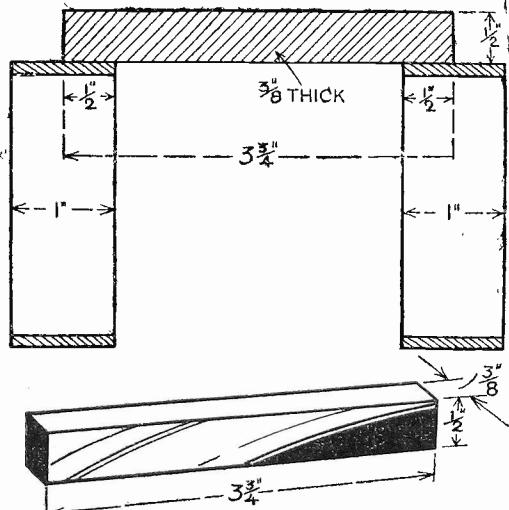
Fig. 5.—The supports, and method of fixing to the end pieces.
