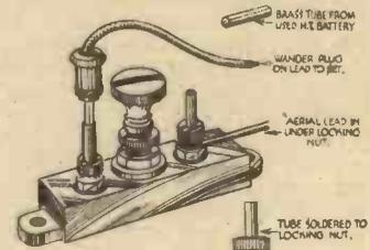
Using a plug and socket to cut out a condenser.
