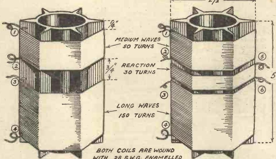
Fig. 3.—Details of suitable coils for a WIRE THROUGHOUT home-made band-pass tuner.
