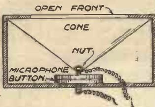
Fig. 5.—A simple cone microphone.
