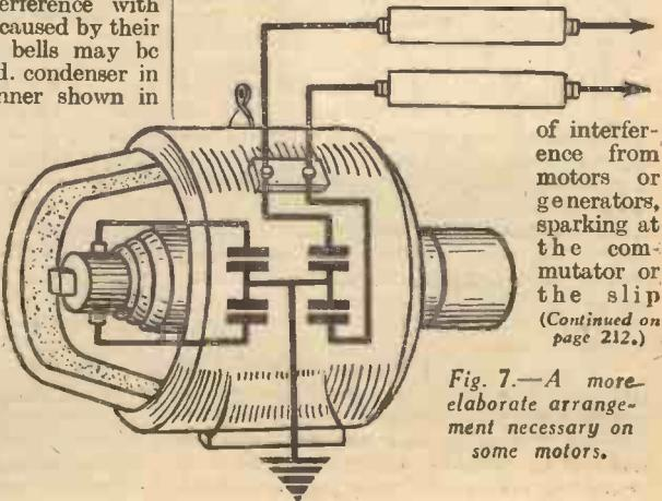
Fig. 7.—A more elaborate arrangement necessary on some motors.
