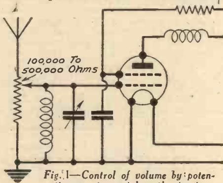
Fig. 1—Control of volume by potentiometer in aerial-earth circuit.
