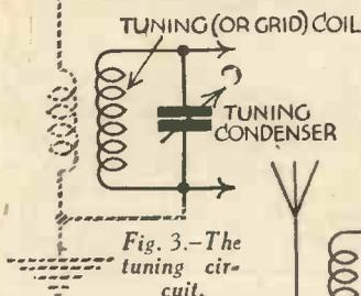
Fig. 3.—The tuning circuit.
