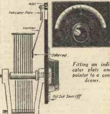
Fitting an indicator plate and pointer to a condenser.
