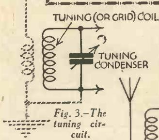
Fig. 3.—The tuning circuit.
