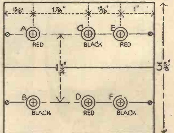
Fig. 2.—Drilling dimensions for the ebonite top.
