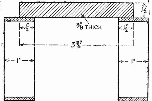
Fig. 5.—The supports, and method of fixing to the end pieces.
