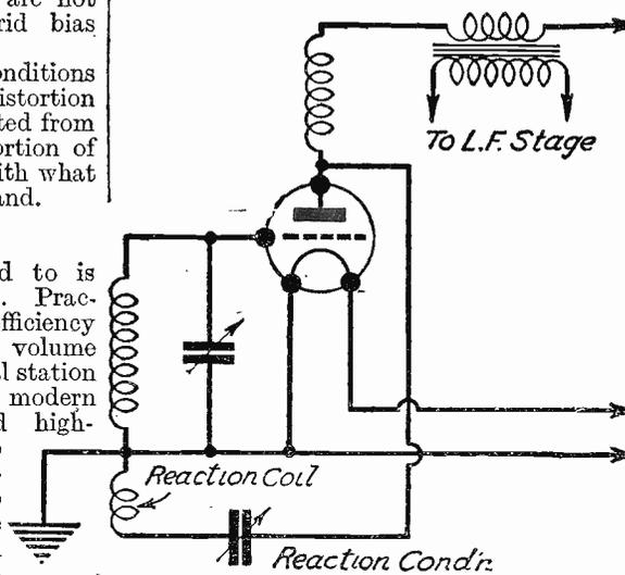
Fig. 1.—The conventional form of capacity reaction control.
