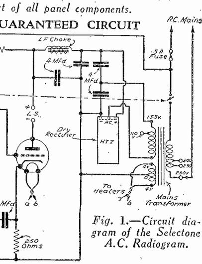
Fig. 1.—Circuit diagram of the Selectone A.C. Radiogram.
