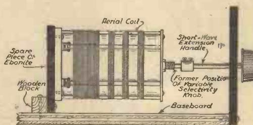
and removed the bakelite knob from the top. Then by boring a hole in the front panel and attaching a short-wave extension handle to the condenser spindle, I was able to re-attach the knob on to the extension handle, so that the selectivity could be controlled from the panel. This arrangement also helps to eliminate hand-capacity, when tuning in some of the weaker foreigners.—R. G. RENTON (Harlesden).
