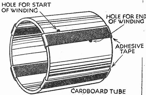
Fig. 8.—The former and adhesive strips for holding another form of coil.
