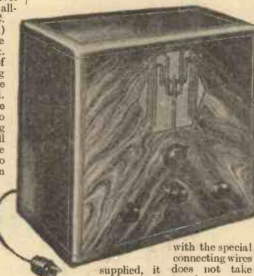
with the special connecting wires supplied, it does not take long to make up the receiver. The mains unit is bolted to the chassis after the principal assembly is completed. An interesting point in the wiring is that you are told how long to cut the wires, and a rule is printed on one edge of the chart. It would appear, therefore, that everything has been thought of to assist the constructor in putting this receiver together in the easiest and most efficient manner possible.
