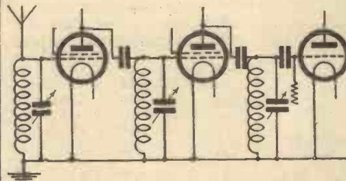
Figs. 4 and 5.—Optional arrangements for three tuned circuits.
