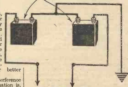
Fig. 4.—An interference eliminator connected across the supply mains.
