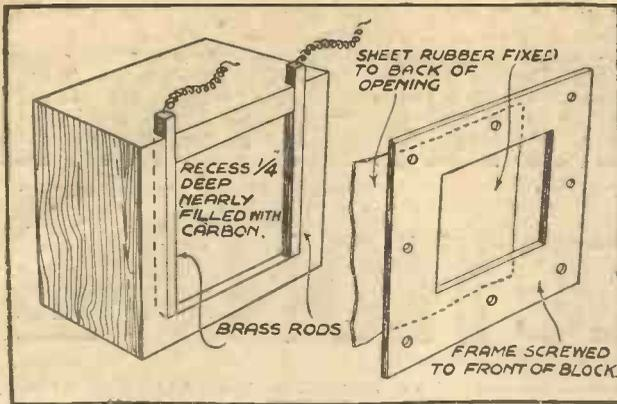
Fig. 10.—A simple carbon microphone.
