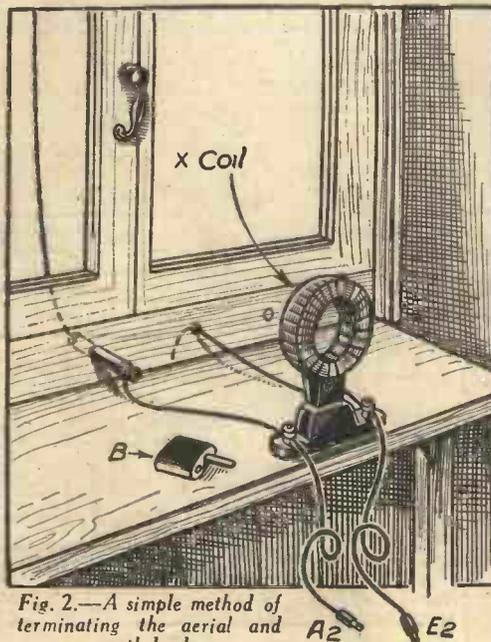
Fig. 2.—A simple method of terminating the aerial and earth leads.
