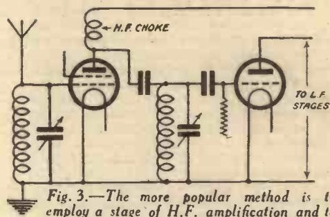
Fig. 3.—The more popular method is to employ a stage of H.F. amplification and to use the second circuit as the coupling between the S.G. valve and the detector.
