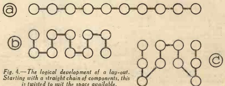
Fig. 4.—The logical development of a lay-out. Starting with a straight chain of components, this is twisted to suit the space available.
