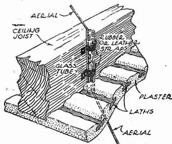
Method of taking a down lead through a ceiling.
