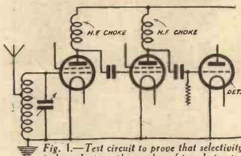
Fig. 1.—Test circuit to prove that selectivity is dependent on the number of tuned circuits.
