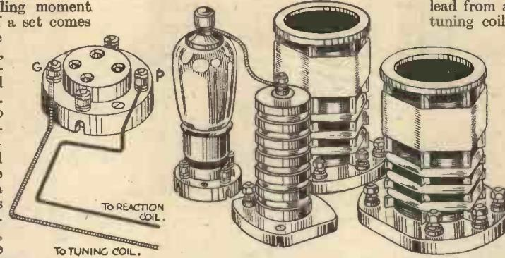
Fig. 1.—Do not run H.F. wires close together.
