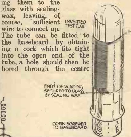
Method of mounting a simple short-wave choke.
