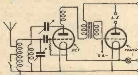
Fig. 3.—A typical two-valve circuit.
