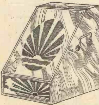
Fig. 1.—General view of a dual-unit speaker.
