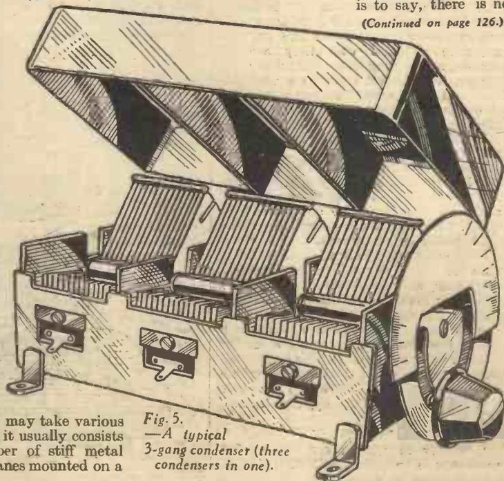
Fig. 5.—A typical 3-gang condenser (three condensers in one).
