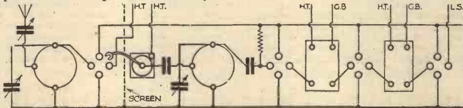
Fig. 3.—Shows the chain of essential components in a 4-valve S.G. receiver, arranged and connected in the simplest possible manner.
