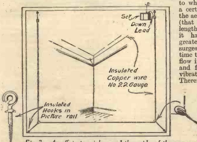
Fig. 3.—An efficient aerial around three sides of the room hung from its picture rail at a distance of 1 foot.
