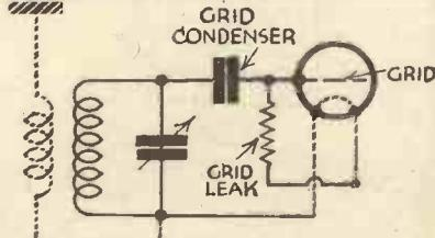
Fig. 4.—This diagram shows the complete grid circuit of the first valve.
