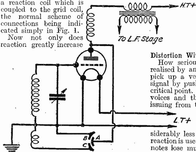
Fig. 2.—The slightly different connections when using a differential reaction condenser.
