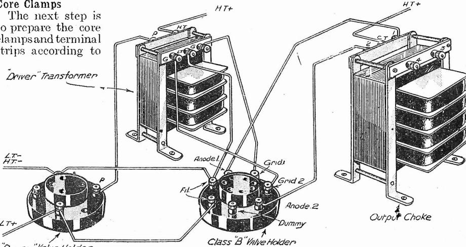
Fig. 8.—This sketch shows how the home-made components are connected up.
