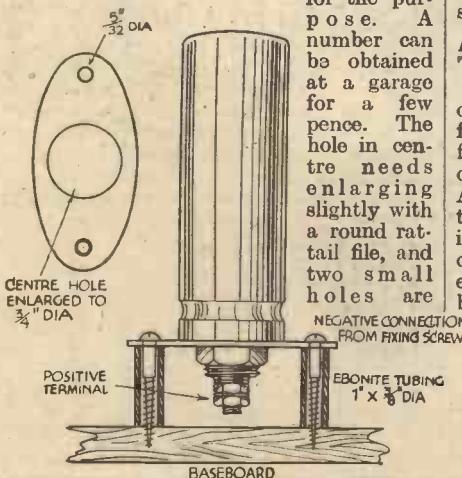
A neat mounting device for electrolytic condensers.
