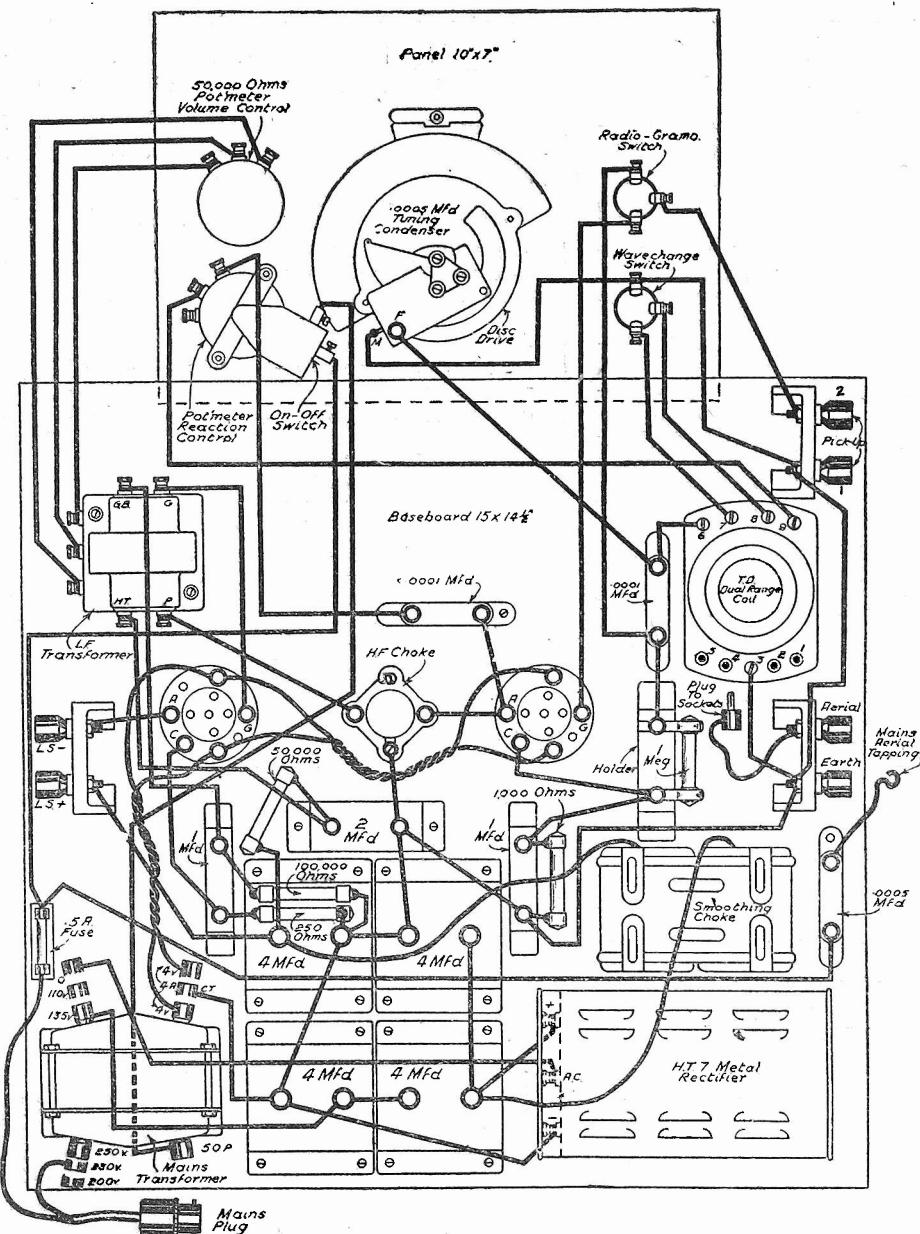
Fig. 3.—Wiring diagram of the Selectone A.C. Radiogram.
