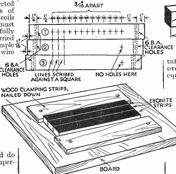
Fig. 2.—How to mark out and cut the coil supports.
