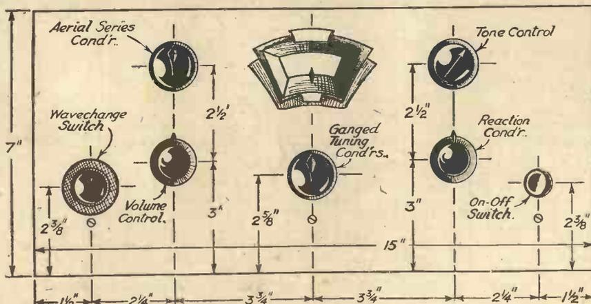
Fig. 2.—Panel-drilling dimensions.
