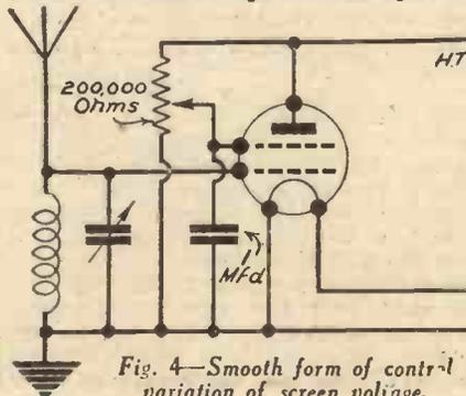
Fig. 4—Smooth form of control variation of screen voltage.
