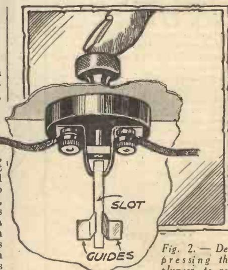
Fig. 2.—Depressing the plunger to release coin and break the circuit.
