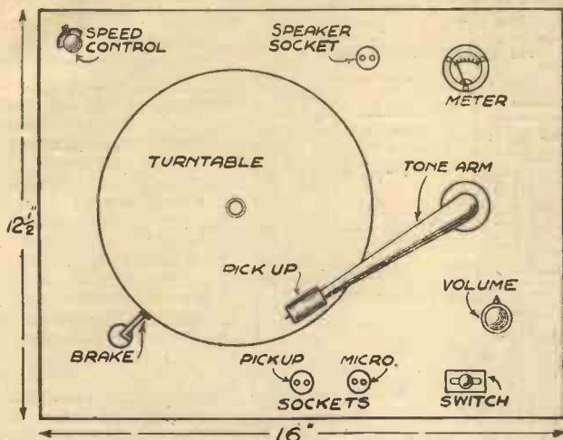
Fig. 1.—The lay-out of the motor-board.
