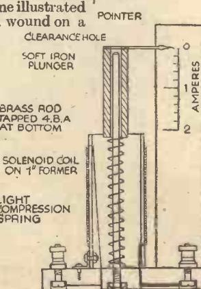
*Two home-made high-reading ammeters.*
