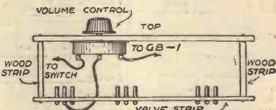
Fig. 7.—Connection to the volume control.
