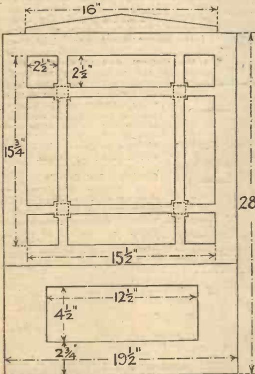
Fig. 2.—Front of cabinet with all necessary dimensions for making up.
