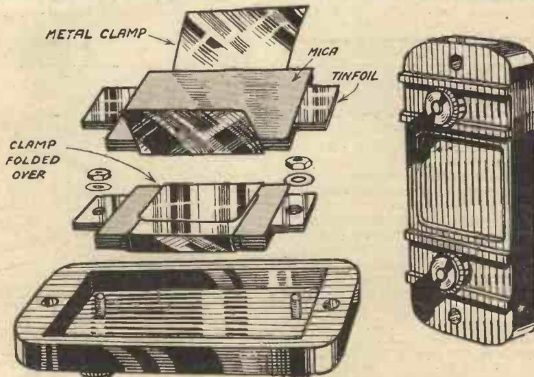
Fig. 2.—Three stages in the construction of a mica condenser.
