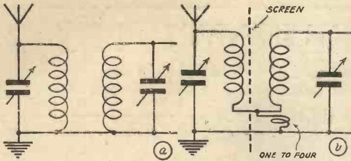
Fig. 4.—Two methods of inductively coupling two circuits.
