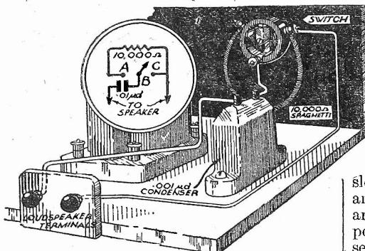
Simple device for controlling frequency response.
