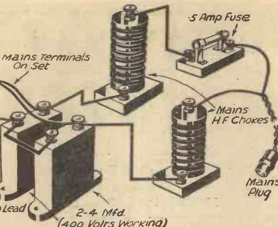
Fig. 3.—A rather elaborate filter circuit which is useful in cases of serious electrical interference of the kind introduced by the mains leads.
