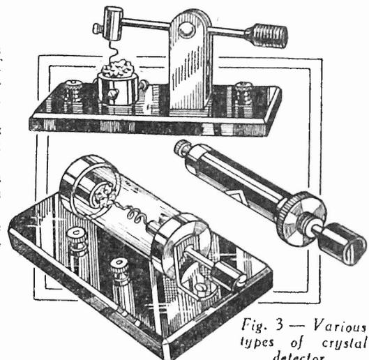
Fig. 3—Various types of crystal detector.
