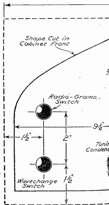
Fig. 2.—This drawing shows the shape cut in the cabinet front. A "PRACTICAL WIRELESS"
