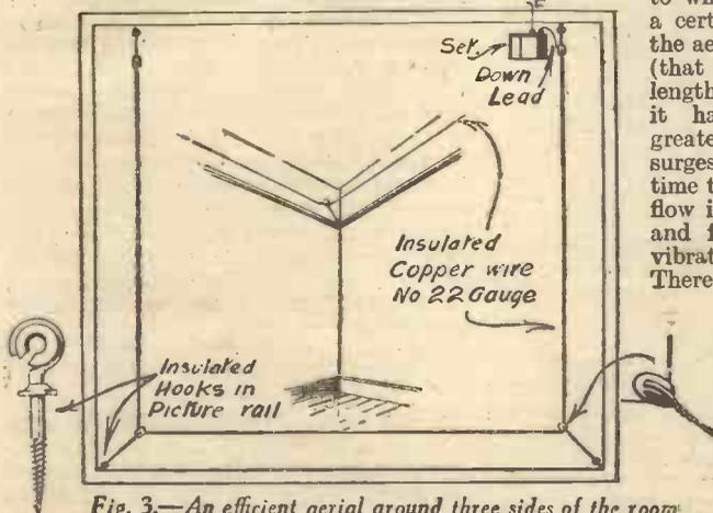
Fig. 3.—An efficient aerial around three sides of the room hung from its picture rail at a distance of 1 foot.
