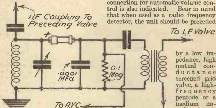
Fig. 2.—A Westecator arranged as an R.F. detector.
