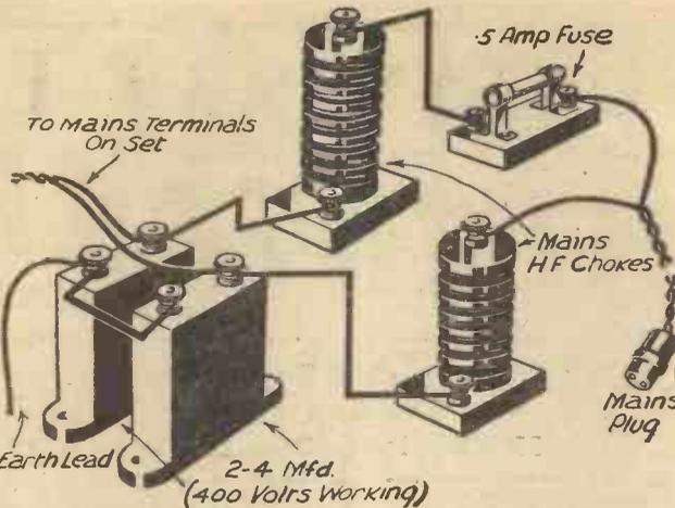
Fig. 3.—A rather elaborate filter circuit which is useful in cases of serious electrical interference of the kind introduced by the mains leads.
