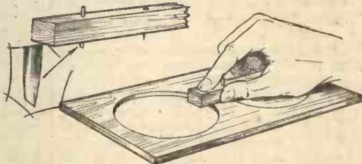
*Cutting large circular holes in a baffle board. the expansion type.—J. P. SAVAGE (Liverpool).*
