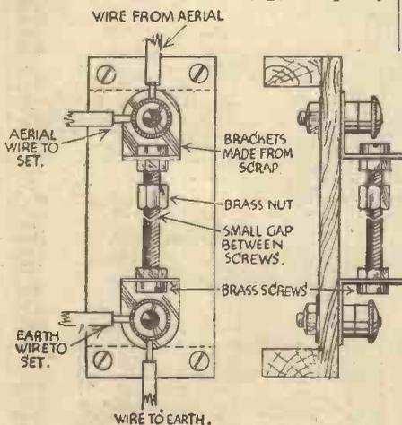
An aerial earthing device made from odds and ends.
