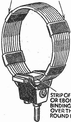
Fig. 9.—The coil wound on former shown in Fig. 8, and method of mounting.
