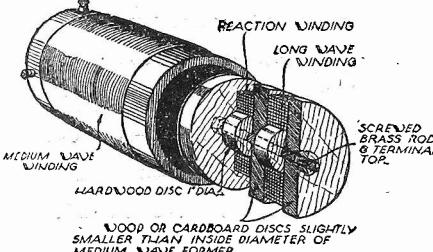
A neat method of making a dual-wave coil.
