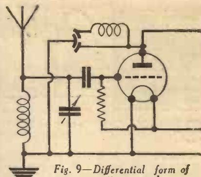
Fig. 9—Differential form of reaction control.
