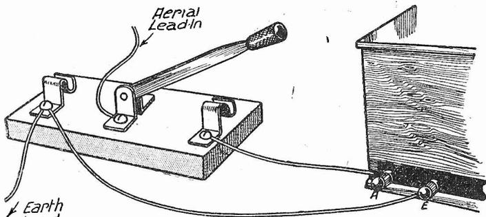
Fig. 2.—The connections to a single-pole aerial-earth switch.
