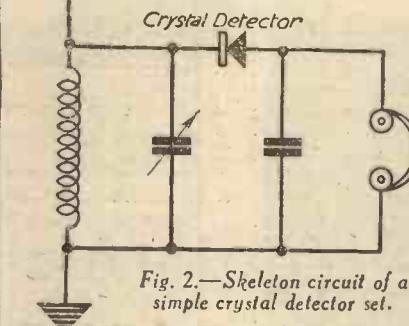
Fig. 2.—Skeleton circuit of a simple crystal detector set.
