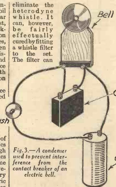
Fig. 3.—A condenser used to prevent interference from the contact breaker of an electric bell.
