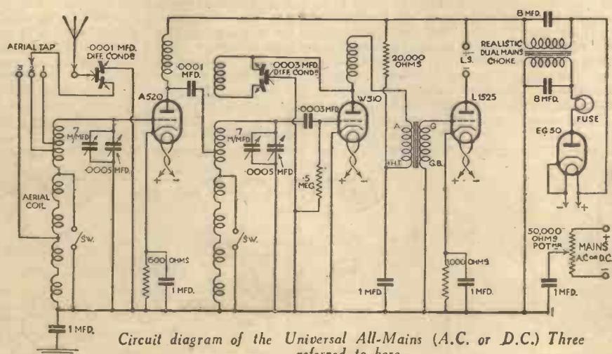
Circuit diagram of the Universal All-Mains (A.C. or D.C.) Three referred to here.
