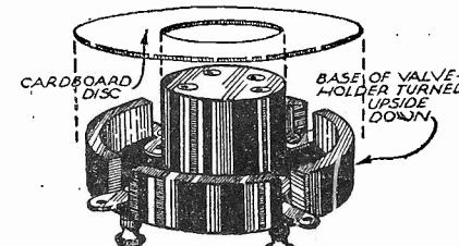
Adapting an ordinary valve-holder for chassis mounting.
