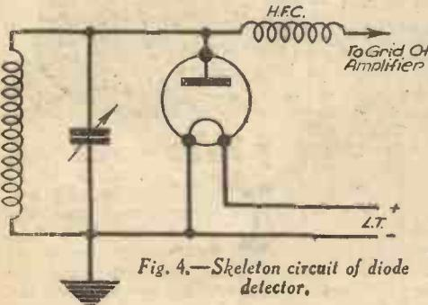
Fig. 4.—Skeleton circuit of diode detector.
