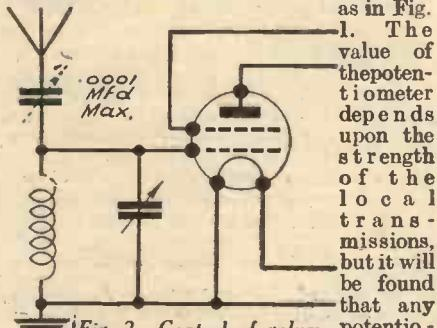
Fig. 2—Control of volume by pre-set condenser in the aerial circuit.
