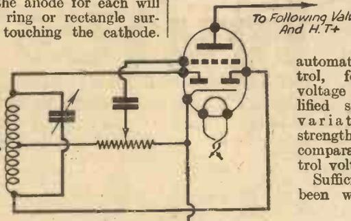
Fig. 6.—Fundamental circuit for using double-diode-triode as full-wave detector and L.F. amplifier. For the sake of clearness all decoupling components have been omitted.
