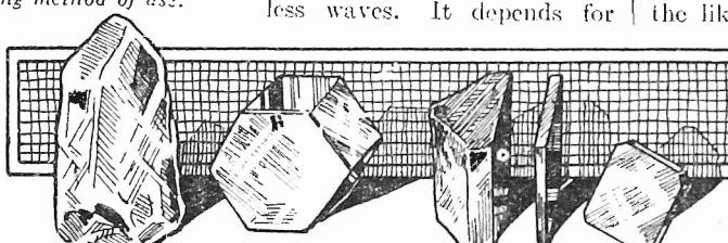
Fig. 2.—Stages in the cutting of quartz crystals as used for crystal control.
