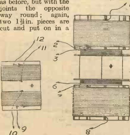
Fig. 5.—The long-wave coil.
