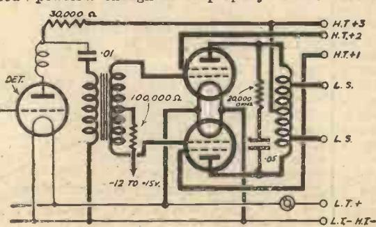
Fig. 5.—Circuit for pentodes in push-pull.
