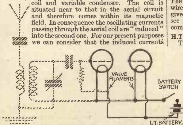
Fig. 5.—The filament circuit.
