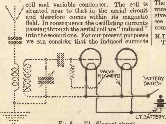
Fig. 5.—The filament circuit.
