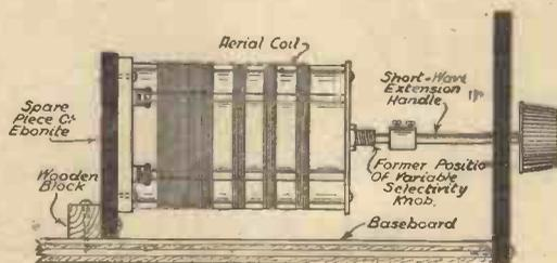
and removed the bakelite knob from the top. Then by boring a hole in the front panel and attaching a short-wave extension handle to the condenser spindle, I was able to re-attach the knob on to the extension handle, so that the selectivity could be controlled from the panel. This arrangement also helps to eliminate hand-capacity, when tuning in some of the weaker foreigners. —R. G. RENTON (Harlesden).
