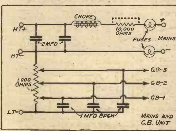
Fig. 3.—The mains and grid bias arrangement.
