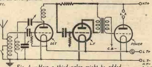
Fig. 4.—How a third valve might be added to the two-valver of Fig. 3.
