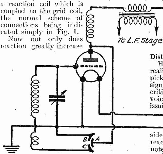
Fig. 2.—The slightly different connections when using a differential reaction condenser.
