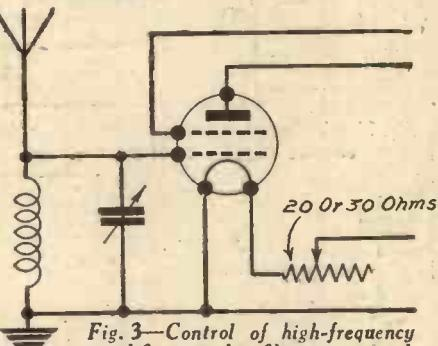
Fig. 3—Control of high-frequency amplification by filament control.
