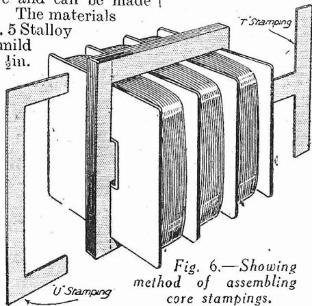
Fig. 6.—Showing method of assembling core stampings.
