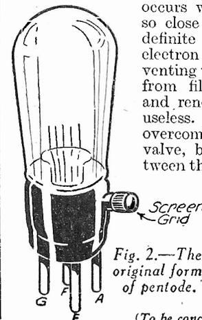
Fig. 2.—The original form of pentode.
