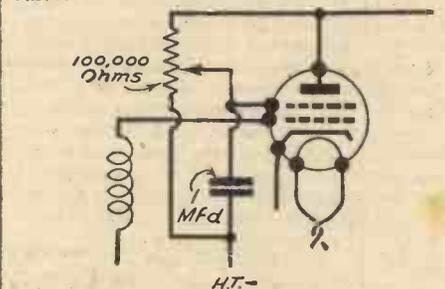
Fig. 5—Variation of screen voltage mains connections.
