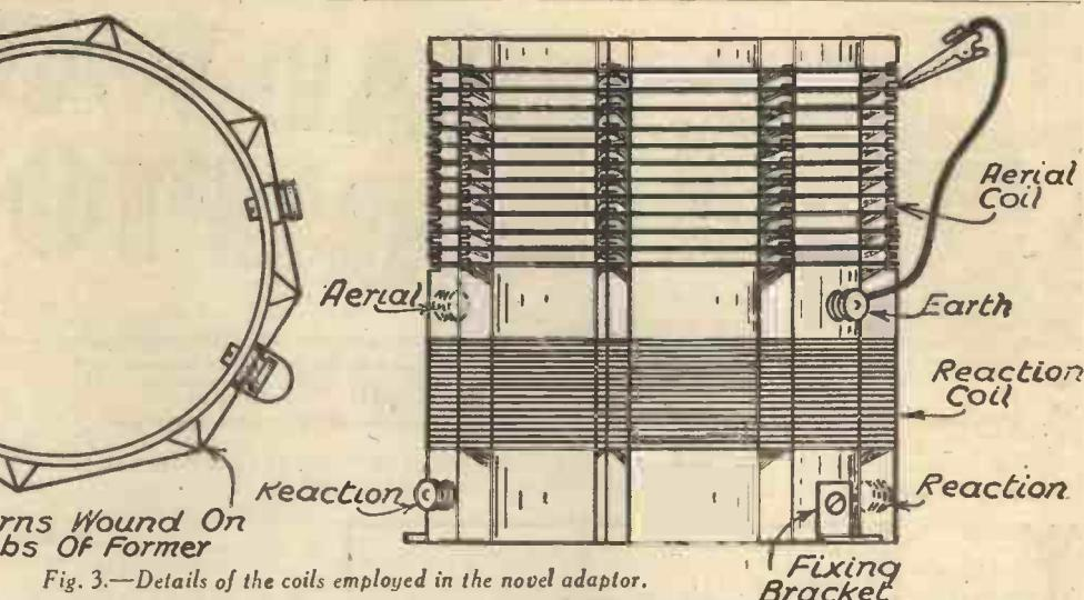
Fig. 3.—Details of the coils employed in the novel adaptor.
