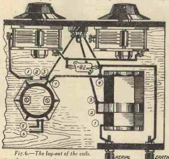
Fig. 6.—The lay-out of the coils.
