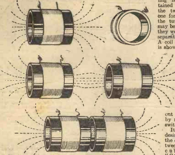
Fig. 3—Illustrating various degrees of coupling between two coils.
