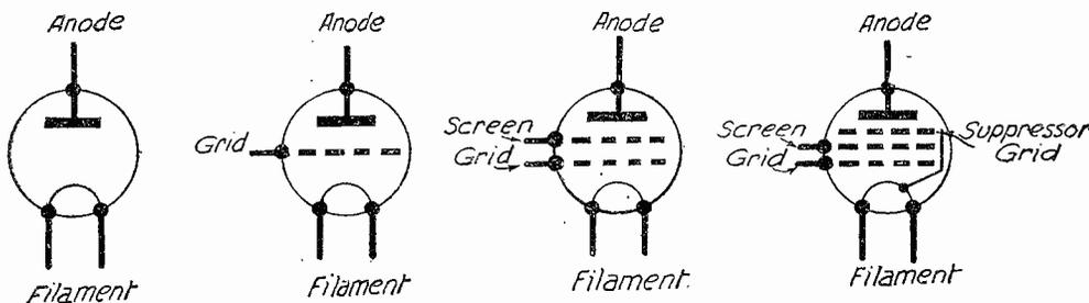
Fig. 1.—The evolution of the pentode valve.
