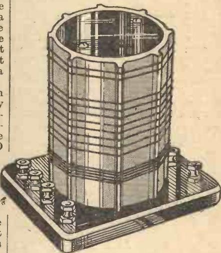
Fig. 4.—Shows three windings on the same former. The coupling here is fairly tight.
