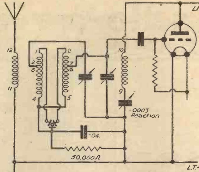
Fig. 8.—The circuit connections of the complete coil.
