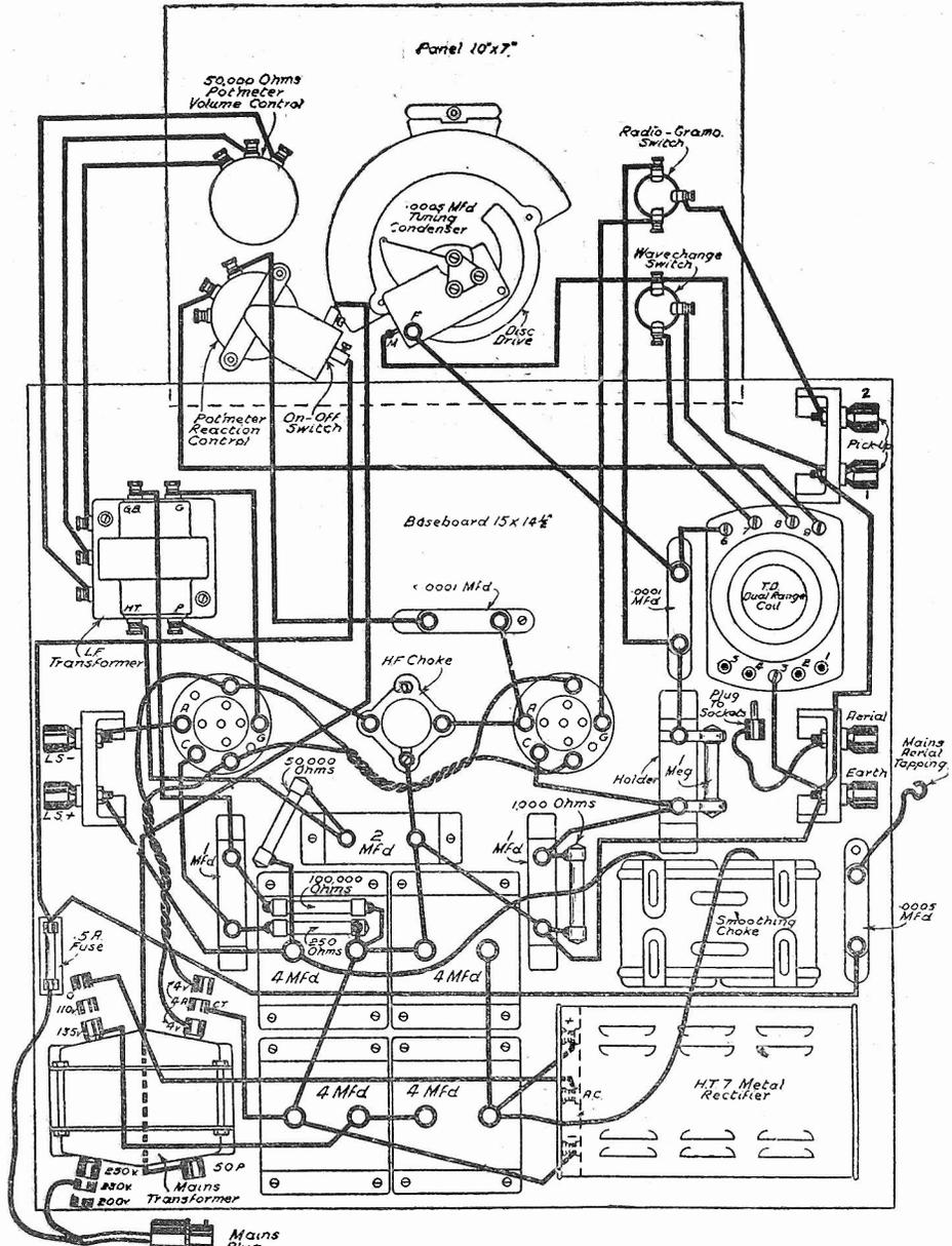
Fig. 3.—Wiring diagram of the Selectone A.C. Radiogram.
