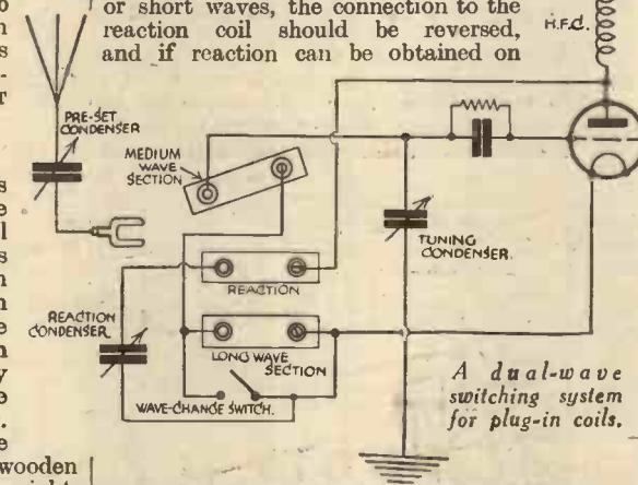
one wave but not on the other, reverse the connections to the coil which fails to oscillate. It might be noted that a very efficient arrangement can be set up as described, as the better makes of plug-in coils are good by modern standards, being wound with thick wire and have little solid dielectric.—P. TAYLOR (Penzance).
