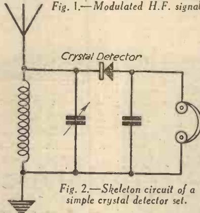
Fig. 2.—Skeleton circuit of a simple crystal detector set.
