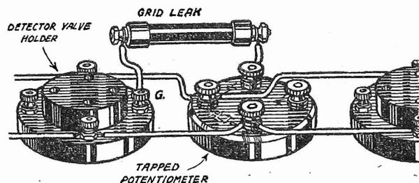
Fig. 5.—Using a tapped potentiometer in the filament leads.
