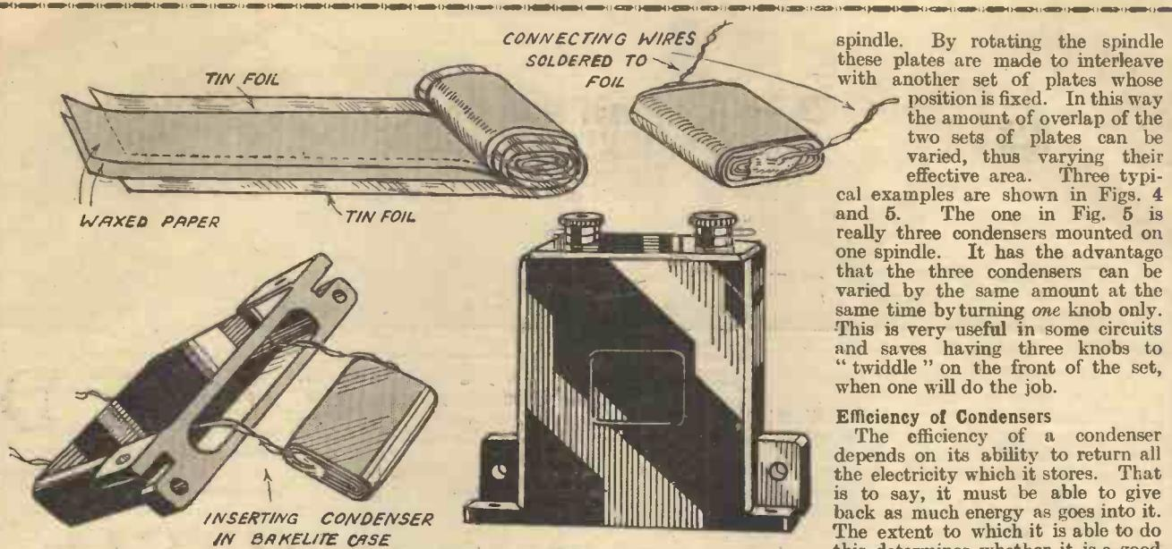
Fig. 3.—How a paper condenser is made.
