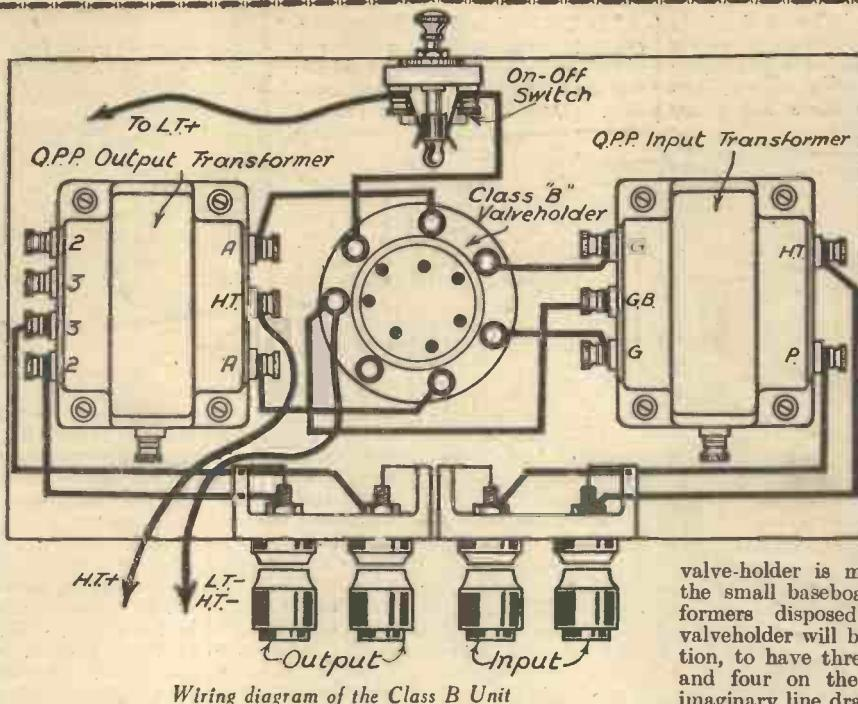
Wiring diagram of the Class B Unit
