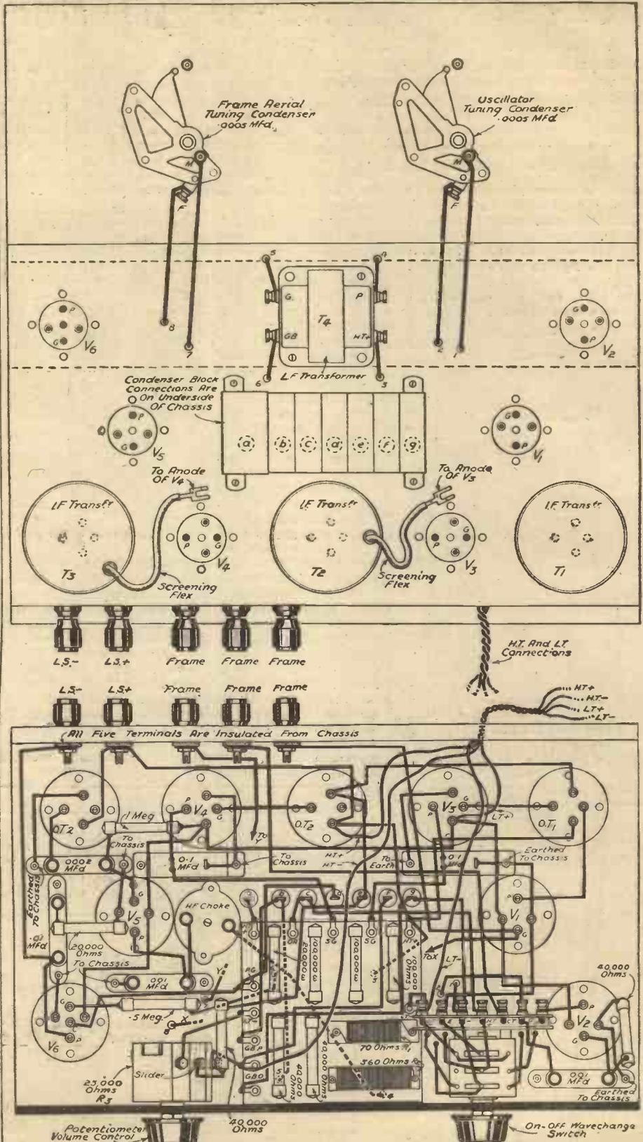
Above- and sub-baseboard wiring diagrams of the Supersonic Six.
