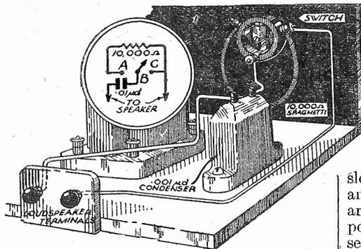
Simple device for controlling frequency response.
