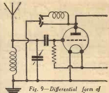
Fig. 9—Differential form of reaction control.
