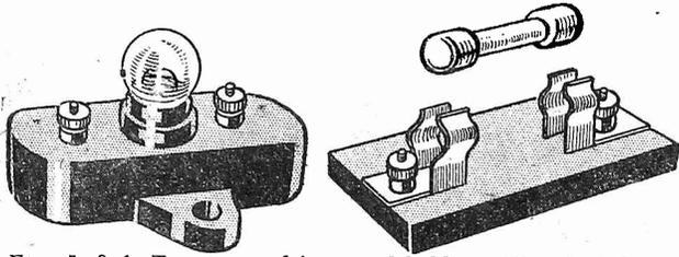
Figs. 5 & 6. Two types of fuses and holders: (5) a flash-lamp-bulb fuse and (6) a cartridge fuse
