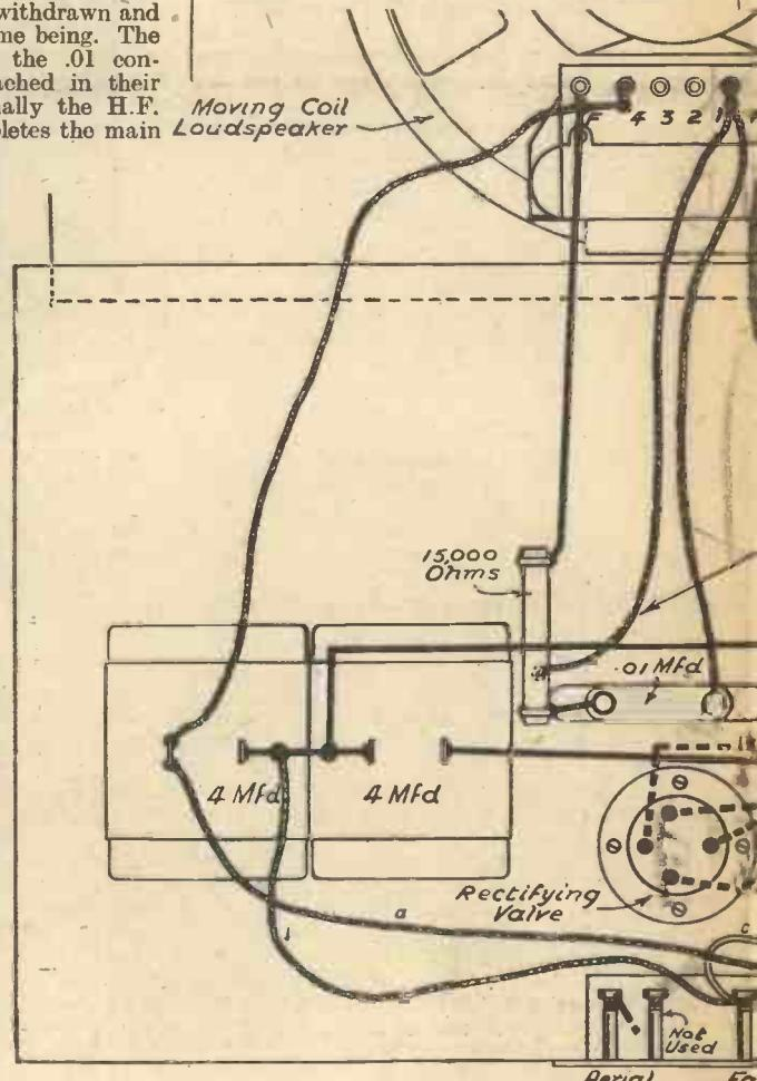
Wiring diagram of the power section of the A.C.T.Y. receiver.
