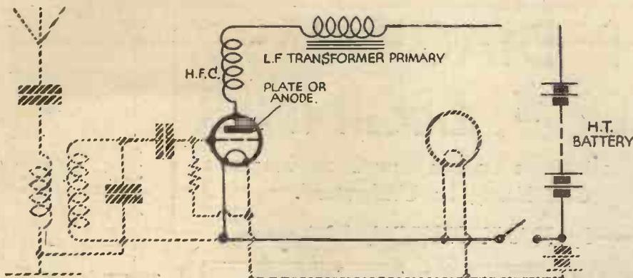
Fig. 6.—The anode and H.F. circuits of the detector valve; notice that the H.T. circuit "overlaps" the filament circuit.
