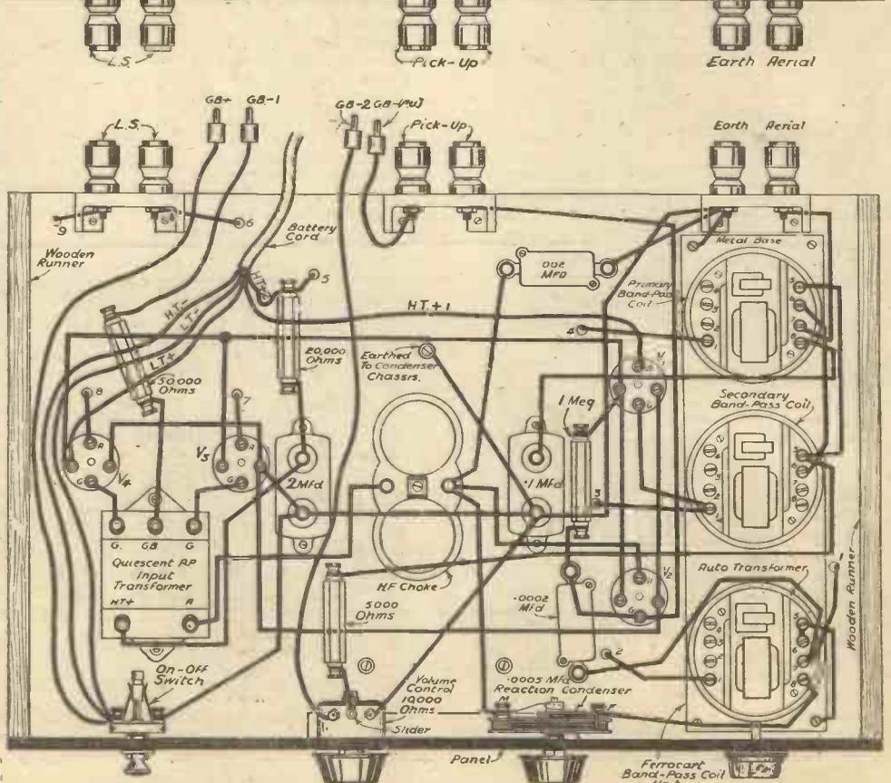
Top and sub-baseboard wiring of the Ferrocart Q.P.-P. Hi-mag Three.
