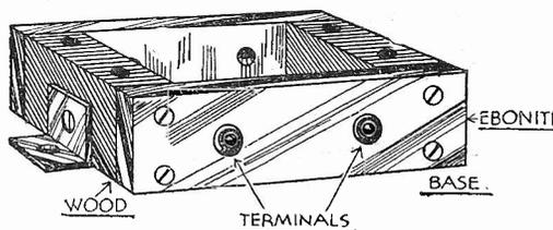
Details of a coil former made from scrap ebonite.
