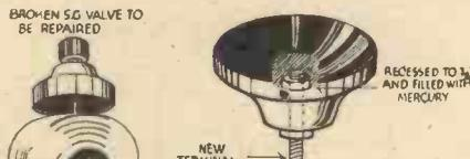
Repairing the terminal top of a screen-grid valve.
