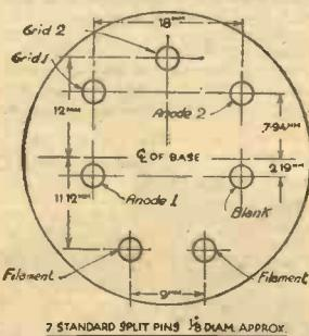
This diagram gives dimensions of the new valve-holders for 7-pin (Class B) valves. The diagram is a top view.
