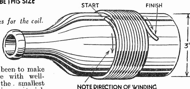
Fig. 4.—Winding the coil round a bottle.
