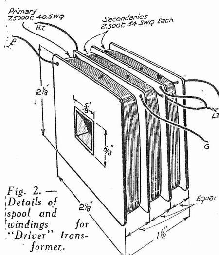
Fig. 2.—Details of spool and windings for "Driver" transformer.
