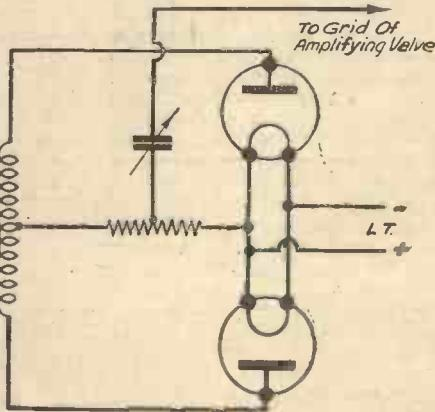
Fig. 5.—Push-pull diode detection. Instead of two diodes two triodes may be used, their grids being employed as the diode anodes and their anodes left disconnected.
