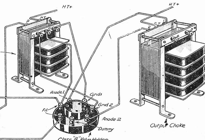
Fig. 8.—This sketch shows how the home-made components are connected up.
