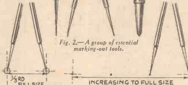
Fig. 3.—How to "scale off" with the dividers.
