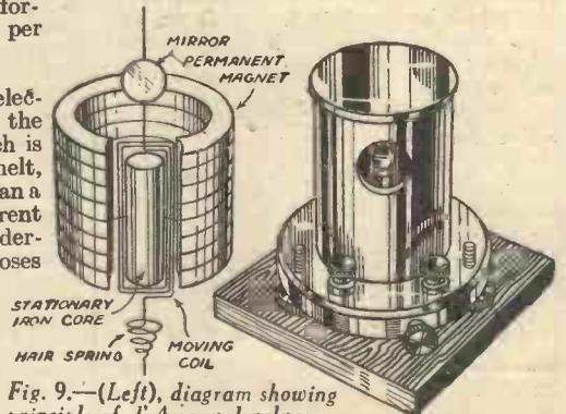
Fig. 9.—(Left), diagram showing principle of d'Arsonval galvanometer. (Right), the complete instrument.
