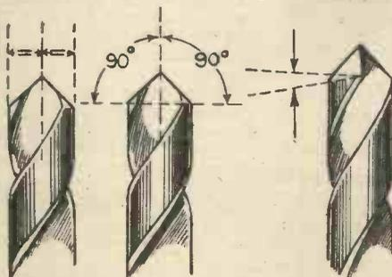
Figs. 2 and 3.—Make certain, after grinding, that the backing off and angles are equal
