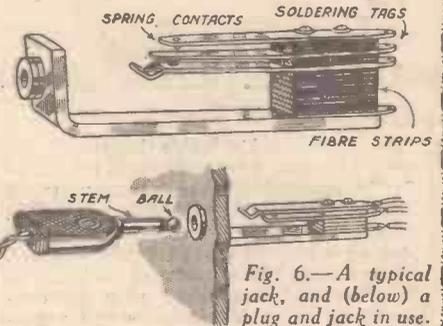
Fig. 6.—A typical jack, and (below) a plug and jack in use.
