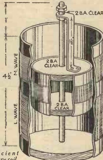
An efficient dual-wave coil.
