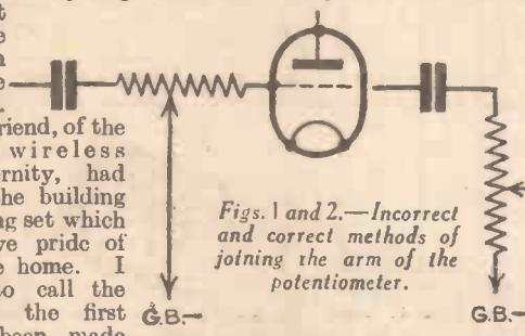
Figs. 1 and 2.—Incorrect and correct methods of joining the arm of the potentiometer.
