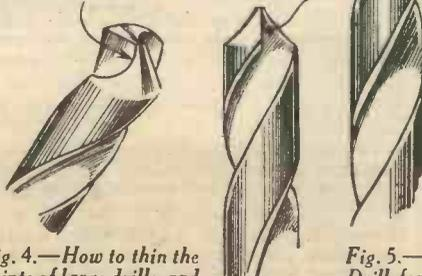
Fig. 4.—How to thin the points of large drills and how to avoid "greediness" when drilling soft metals.
