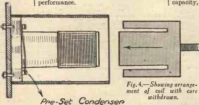
Fig. 4.—Showing arrangement of coil with core withdrawn.
