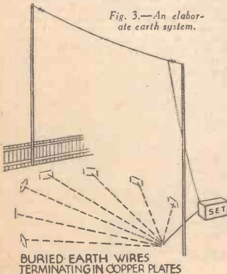
BURIED EARTH WIRES TERMINATING IN COPPER PLATES
