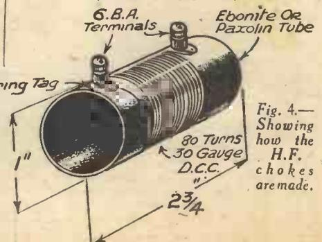
Fig. 4.—Showing how the H.F. chokes are made.
