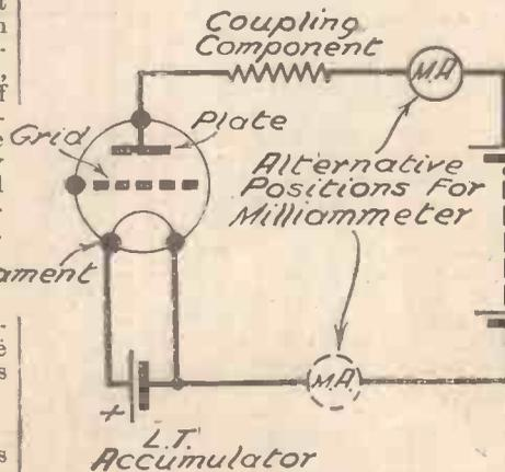
Fig. 2.—The current flowing from the filament to plate of a valve can be measured by inserting a milliammeter in series with the H.T. battery.
