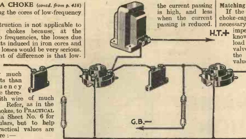
Fig. 3.—Showing the connections for choke-capacity L.F. coupling.
