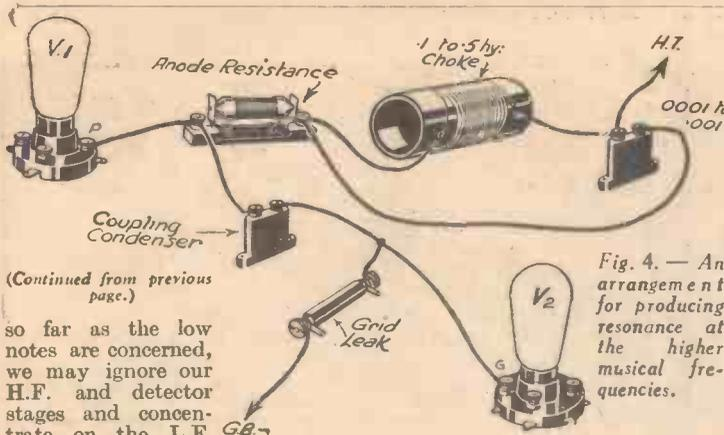
Fig. 4.—An arrangement for producing resonance at the higher musical frequencies.
