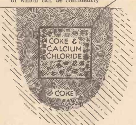
Fig. 2.—A chemical earth of high efficiency.
