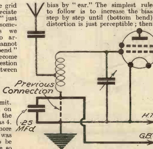
Fig. 9.—Showing the method of applying grid bias to a high-frequency valve.
