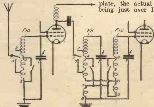
Fig. 2.—Circuit essentials of the new Ferrocart Coils.
