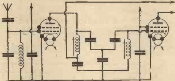
Fig. 5.—Permeability tuned circuit with band pass intervalve coupling.
