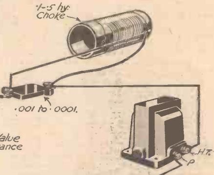
Fig. 5.—A similar arrangement to Fig. 4, but designed for Transformer coupling.
