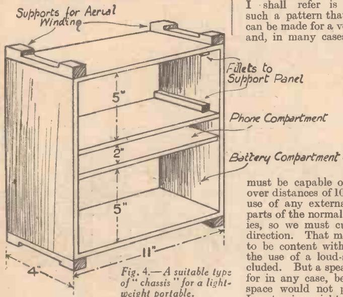
Fig. 4.—A suitable type of "chassis" for a lightweight portable.
