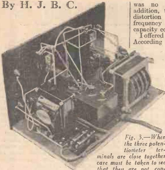
Fig. 3.—When the three potentiometer terminals are close together care must be taken to see that they are not connected up incorrectly.
