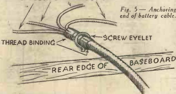
Fig. 5—Anchoring end of battery cable.
