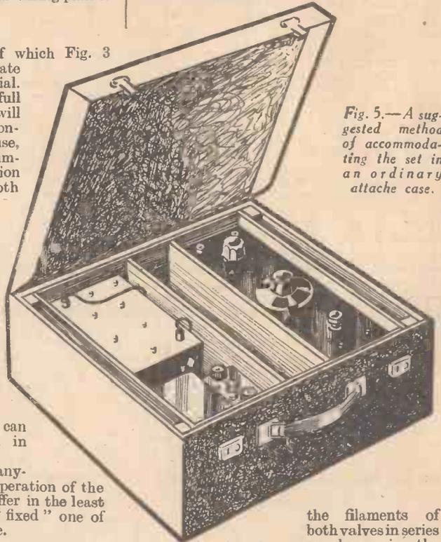
Fig. 5.—A suggested method of accommodating the set in an ordinary attaché case.
