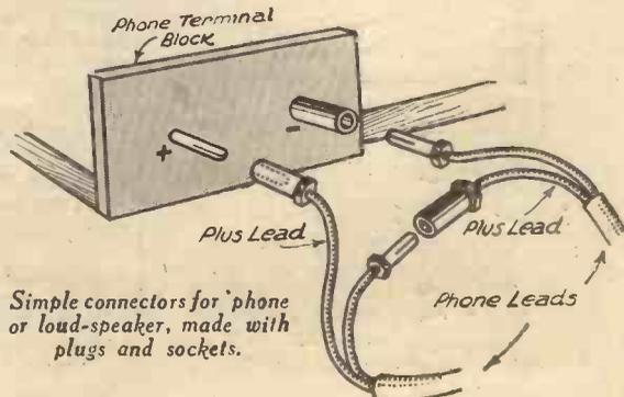
Simple connectors for 'phone or loud-speaker, made with plugs and sockets.
