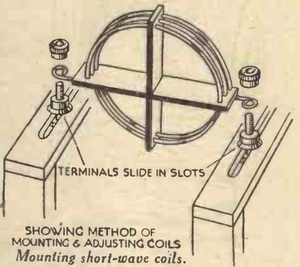
material. It possesses advantages, especially for the experimenter, in that each individual coil is easily interchangeable, and all are adjustable. The diagram is self-explanatory, and the materials required are: one piece of hardwood, 4in. by 4in.; four wooden uprights, 2 1/2in. by 1/2in. by 1/2in.; two pieces of ebonite, 4in. by 1/2in.; six terminals, and a quantity of 16 S.W.G. bare wire. The terminals are mounted three in each slot, one pair for each coil.—F. C. TREND (Upper Norwood).
