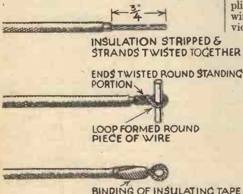
Fig. 4—Finishing ends of flex.
