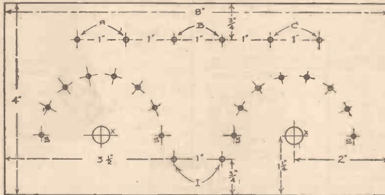
Fig. 3.—Drilling dimensions.
