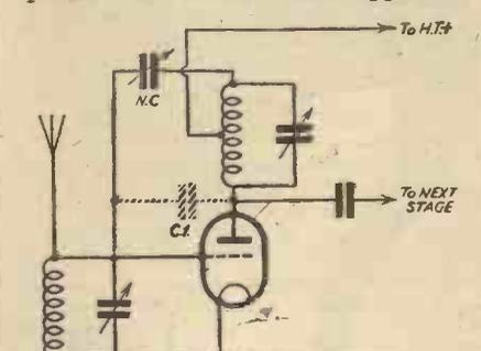
Fig. 7.—Principle of neutralized H.F. amplifier.
