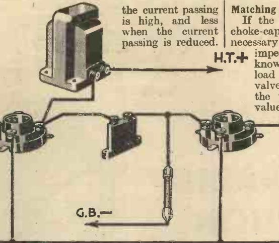
Fig. 3.—Showing the connections for choke-capacity L.F. coupling.
