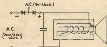
Fig. 1.—Half-wave rectification without a mains transformer.
