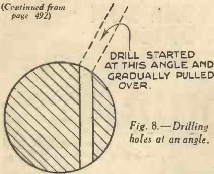
Fig. 8.—Drilling holes at an angle.
