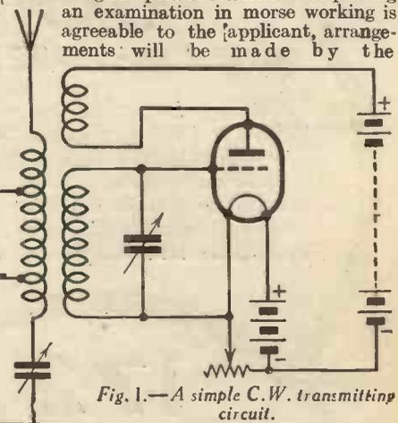
Fig. 1.—A simple C.W. transmitting circuit.
