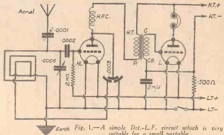
Fig. 1.—A simple Det.-L.F. circuit which is very suitable for a small portable.
