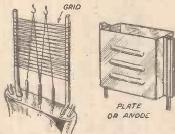
Fig. 2.—Valve parts showing the grid.
