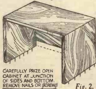
CAREFULLY PRIZE OPEN CABINET AT JUNCTION OF SIDES AND BOTTOM. REMOVE NAILS OR SCREWS Fig. 2.
