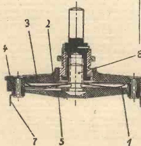
Fig. 3.—Practical execution of the new condenser:
