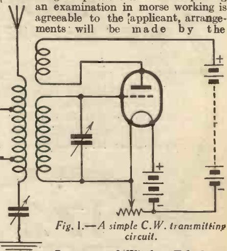
Fig. 1.—A simple C.W. transmitting circuit.
