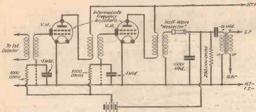
Fig. 5.—Using the "Westector" in a battery-operated receiver, for volume control.
