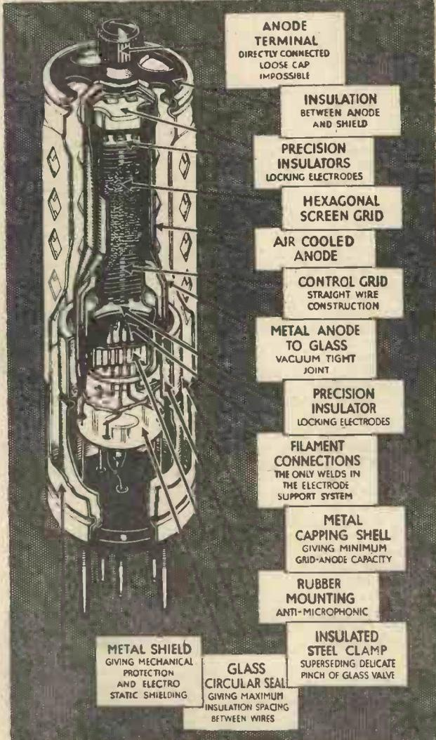
A study of the diagram reveals at once the advantages of the OSRAM "CATKIN" VALVE assembly over the previous method. The increasing accuracy in the use of valves demands an increasing accuracy in performance, and therefore increasing precision in construction. The "Catkin" construction permits a greater uniformity in production than was possible with the equivalent glass types, and so allows for a greatly improved performance in the set.
