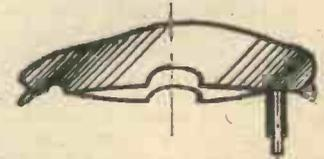
Fig. 5.—The electrodes of the new condenser.
