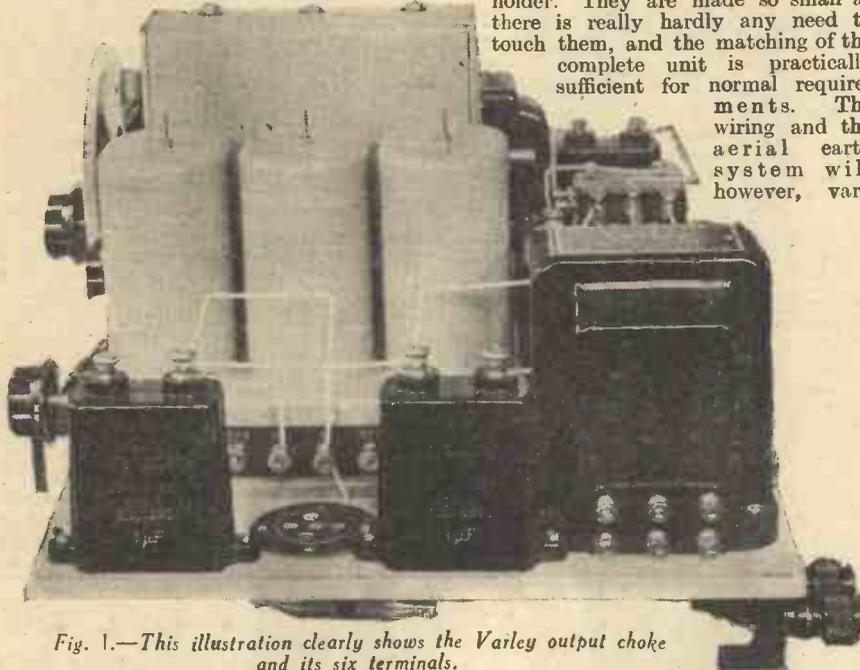
Fig. 1.—This illustration clearly shows the Varley output choke and its six terminals.
