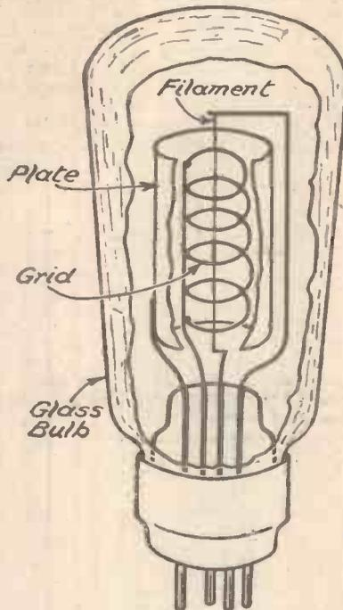
Fig. 1.—A "break-away" sketch showing the main constructional details of a three-electrode valve.
