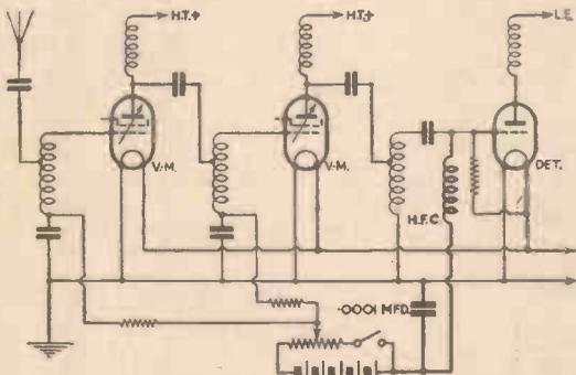
Fig. 1.—Showing how automatic grid bias was added to an ordinary battery set having two V.-M. valves. The new components and connections are shown in heavy lines.
