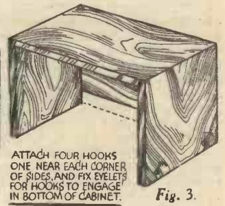
ATTACH FOUR HOOKS ONE NEAR EACH CORNER OF SIDES AND FIX EYELETS FOR HOOKS TO ENGAGE IN BOTTOM OF CABINET. Fig. 3.
