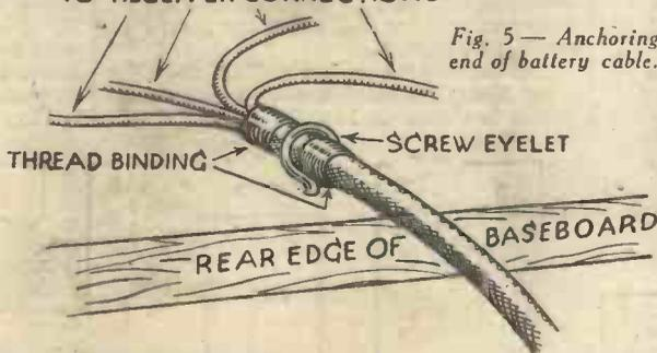
Fig. 5—Anchoring end of battery cable.
