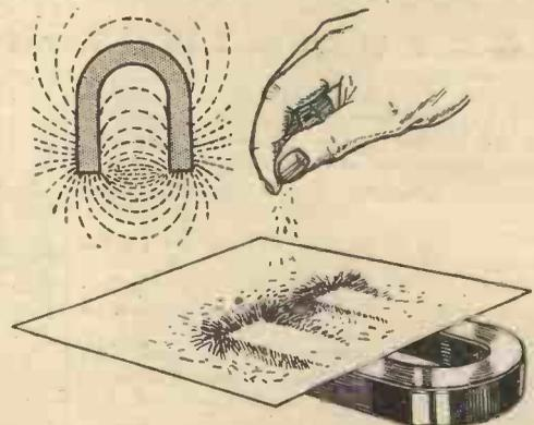
Fig. 3.—Experiment to illustrate the lines of force around a permanent magnet.
