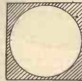
Fig. 4.—The dark areas which appear when using a round hole in the scanning disc.
