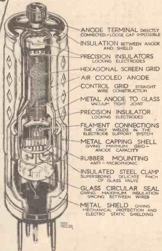
A complete breakaway from the usual method of making wireless valves with a glass bulb has been accomplished by the introduction of the OSRAM 'CATKIN' VALVE. Not only has metal been substituted for glass, but the electrodes have been greatly strengthened by a packed and rigid assembly. Special features of the OSRAM 'CATKIN' valve include
