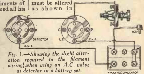
Fig. 1.—Showing the slight alteration required to the filament wiring, when using an A.C. valve as detector in a battery set.
