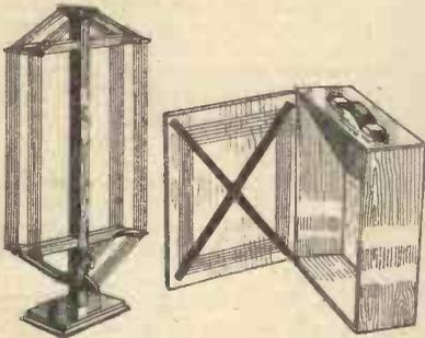
Fig. 7.—Two forms of frame aerial. That shown on the right is wound on the inside of the door of a portable receiver.
