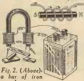
Fig. 2. (Above), a bar of iron can be magnetized by passing an electric current round it. (Below), a simple horseshoe electro-magnet.
