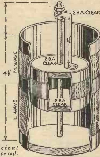
An efficient dual-wave coil.
