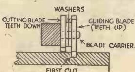
A simple method of slotting coil-formers.
