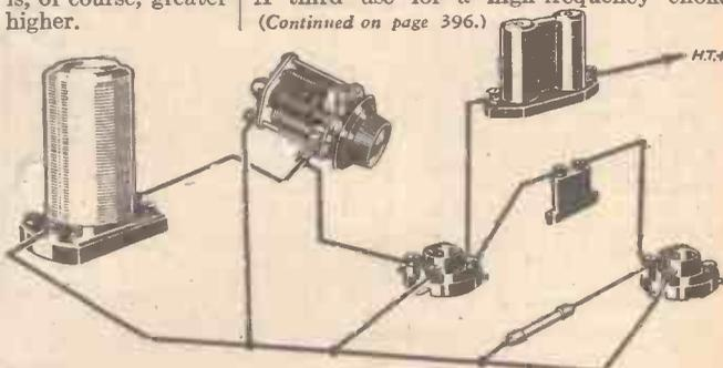
Fig. 2.—Aperiodic coupling between H.F. and detector stages.
