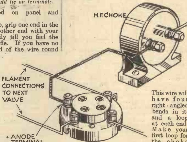
Fig. 3—Wiring a choke to the anode terminal of a valveholder.
