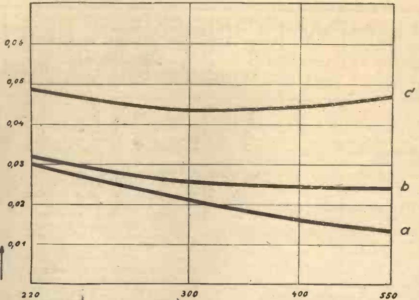
Fig. 8.—Damping curve of: (a) an air condenser. (b) a Vogt flat condenser. (c) a hard paper condenser.
