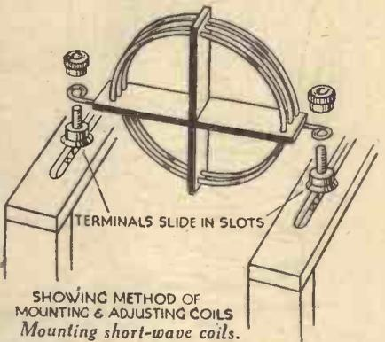
material. It possesses advantages, especially for the experimenter, in that each individual coil is easily interchangeable, and all are adjustable. The diagram is self-explanatory, and the materials required are: one piece of hardwood, 4in. by 4in.; four wooden uprights, 2 1/2in. by 1/2in. by 1/4in.; two pieces of ebonite, 4in. by 1/2in.; six terminals, and a quantity of 16 S.W.G. bare wire. The terminals are mounted three in each slot, one pair for each coil.—F. C. TREND (Upper Norwood).
