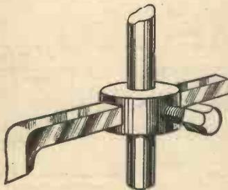
Fig. 12.—Expanding or trepanning cutter for large holes.
