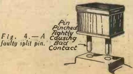
Fig. 4.—A faulty split pin.
