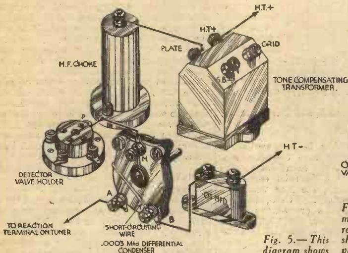
Fig. 5.—This diagram shows the practical wiring details for the arrangement shown in Fig. 4.
