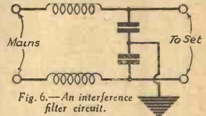
Fig. 6.—An interference filter circuit.
