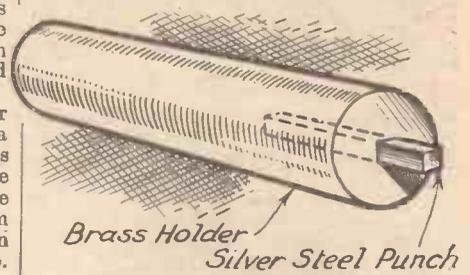
Fig. 4.—Punch for making the holes.
