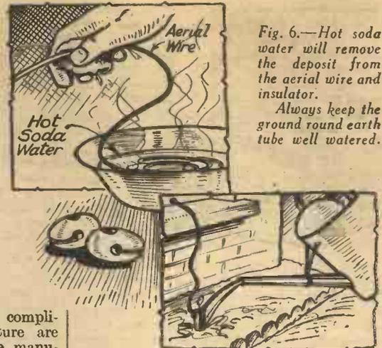
Fig. 6.—Hot soda water will remove the deposit from the aerial wire and insulator.
