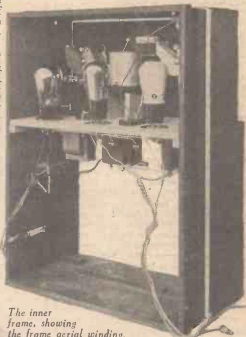
The inner frame, showing the frame aerial winding.
