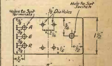
Fig. 5.—Detail of terminal strip.
