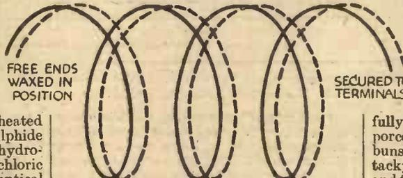
Fig. 2.—Sketch showing system of parallel winding employed.
