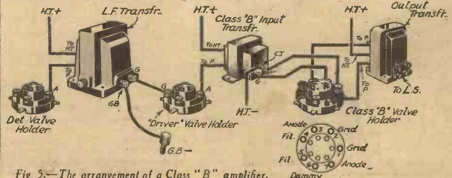
Fig. 5.—The arrangement of a Class "B" amplifier.
