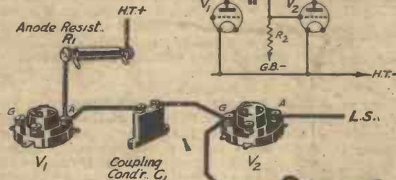
Fig. 1.—The connections for a resistance-capacity coupled stage.
