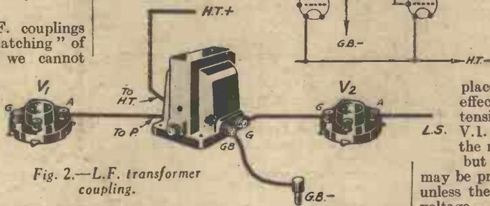
Fig. 2.—L.F. transformer coupling.
