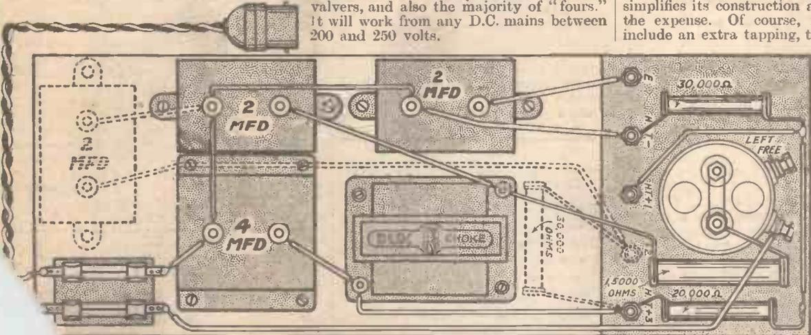
Fig. 2.—Wiring diagram. Dotted outlines indicate extra components needed for an additional tapping.
