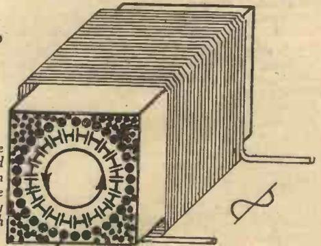
Fig. 5.—A core made of iron particles mixed with insulating material. It is impossible absolutely to insulate the particles and prevent eddy current losses in this way, as there are forming dielectric displacement currents due to capacitive coupling between the particles.
