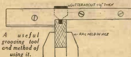
A useful grooving tool and method of using it.
