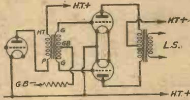
Fig. 4.—The push-pull circuit; identical connections are used for quiescent push-pull.
