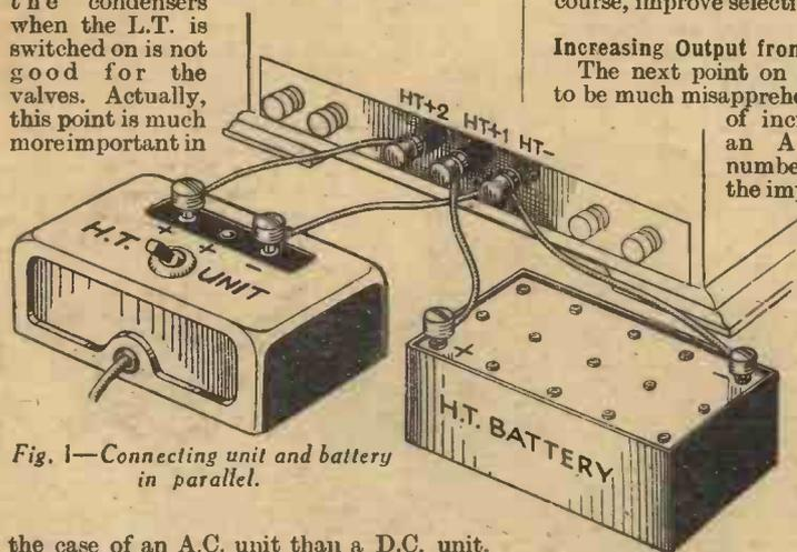
Fig. 1.—Connecting unit and battery in parallel.
