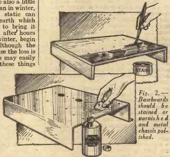
Fig. 2.— Baseboards should be stained or varnished and metal chassis polished.
