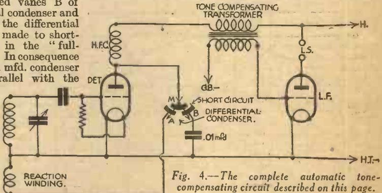
Fig. 4.—The complete automatic tone-compensating circuit described on this page.
