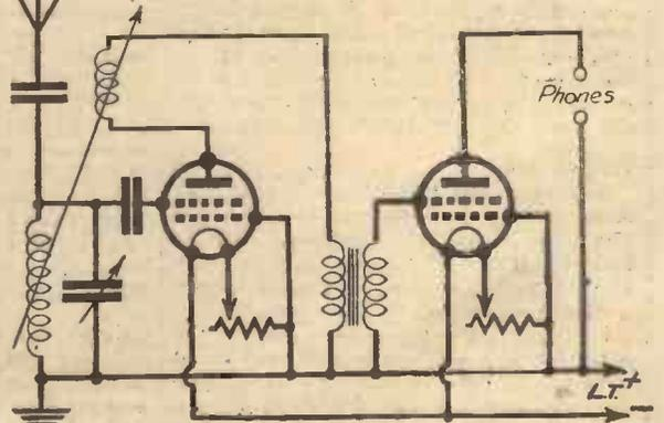
Fig. 8.—Circuit of a two-valve set—L.F. high-tension-less receiver.
