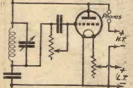
Fig. 9.—The Ultra-Audion, a tricky but interesting single valve "super" circuit.
