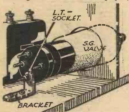
Mounting a screened-grid valve holder.
