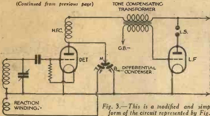
Fig. 3.—This is a modified and simplified form of the circuit represented by Fig. 2.
