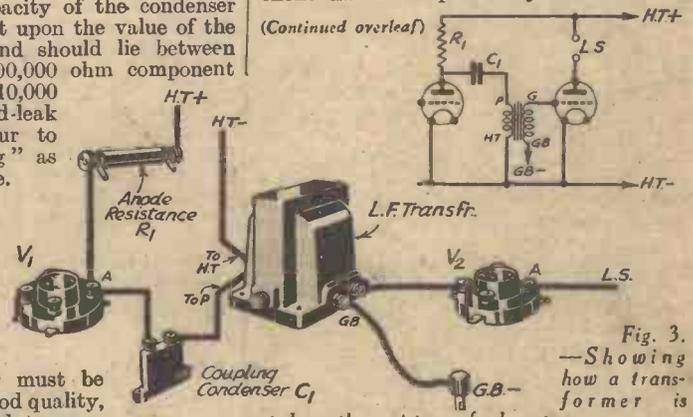
Fig. 3.—Showing how a transformer is connected on the resistance-feed system.
