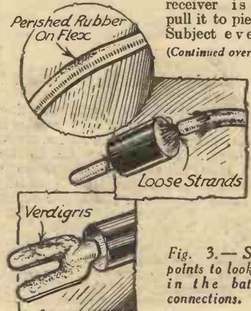
Fig. 3.— Some points to look for in the battery connections.
