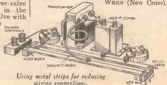
Using metal strips for reducing wiring connections.
