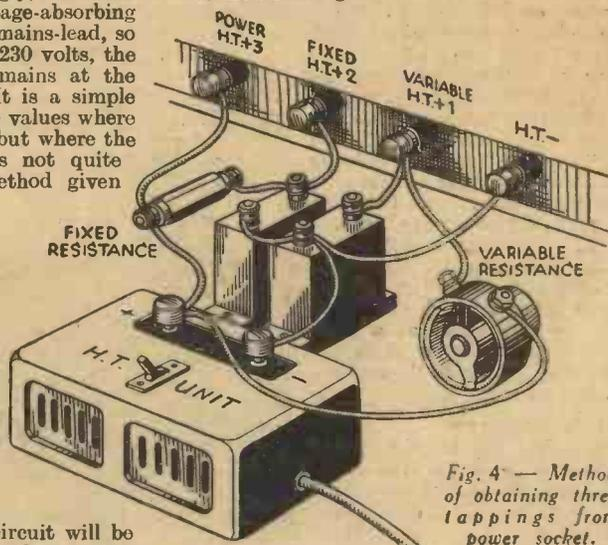
Fig. 4 — Method of obtaining three tappings from power socket.
