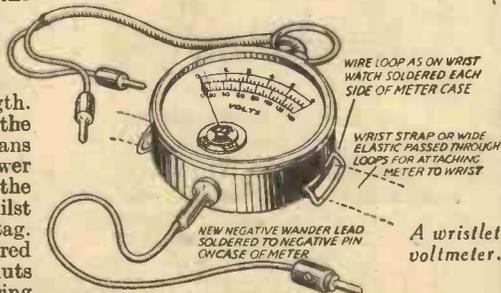
the common negative to the pin at the base of the meter, an extra lead can be soldered to this pin, as shown in the sketch, to facilitate use when the meter is attached to the wrist.
