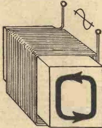
Fig. 3.—In a solid iron core, considerable eddy current losses are induced by the alternating magnetic field.
