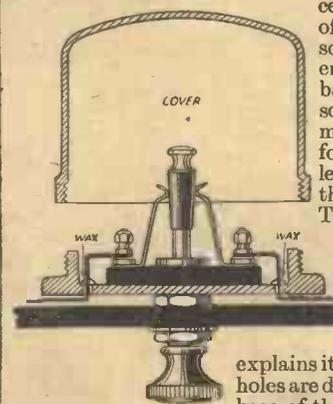
The method of adaptation is shown in the sketch which almost explains itself. Three holes are drilled in the base of the container—a central one for the fixing-bush, and two others for the connecting wires to enter. After mounting the switch and connecting up the wires, the holes through which they pass are sealed up airtight with a little melted wax. The cover is then screwed on, making the whole switch assembly completely dustproof and damp-proof.—N. HURST (Wimbledon).
