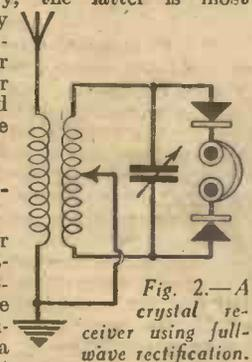
Fig. 2.—A crystal receiver using full-wave rectification.
