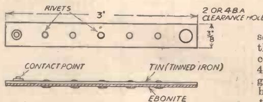
Fig. 4.—Details of expanding strip
