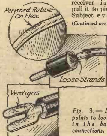
Fig. 3.— Some points to look for in the battery connections.
