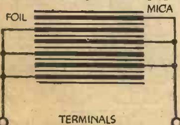
Fig. 3.—So called condenser type cell (coating omitted for clearness).
