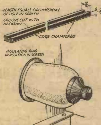
hole in the screen, the edge of which fits neatly in the central slot. The diagram shows this ring in position.—F. BISSEKER (Blackburn).
