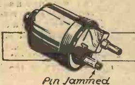
Fig. 3.—A jammed contact pin causes bad contact.
