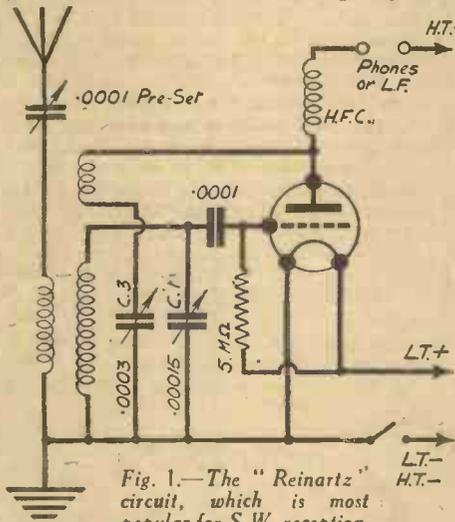
Fig. 1.—The "Reinartz" circuit, which is most popular for S.W. reception.
