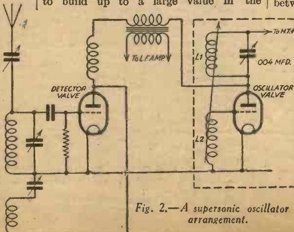
Fig. 2.—A supersonic oscillator arrangement.
