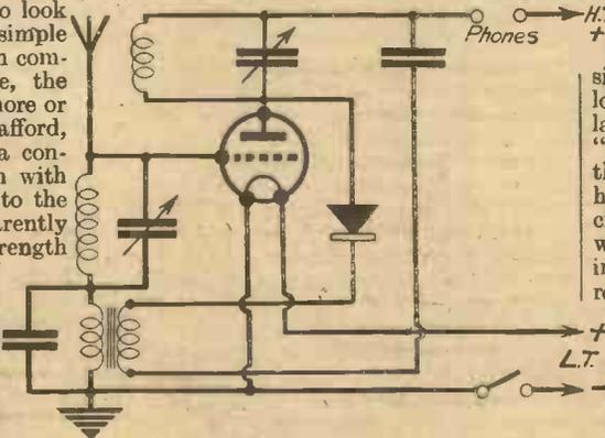
Fig. 4.—An early form of valve-crystal reflex circuit.
