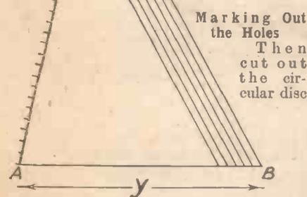
Fig. 3.—Simple method of accurately spacing the holes.
