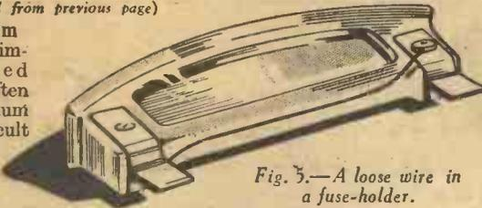
Fig. 5.—A loose wire in a fuse-holder.
