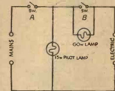
Switchboard arrangement for protecting an electric soldering iron.
