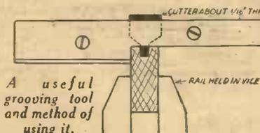
A useful grooving tool and method of using it.
