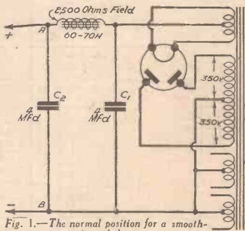
Fig. 1.—The normal position for a smoothing choke.
