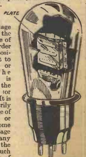
Fig. 5.—Valve cut away to show the plate.
