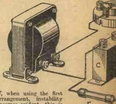
If, when using the first arrangement, instability becomes evident, this is really due to insufficient decoupling in the receiver, but a 2 mfd. condenser connected directly across negative and positive of the battery usually has the desired result.
