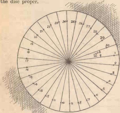
Fig. 1.—Marking out the holes in the scanning disc.
