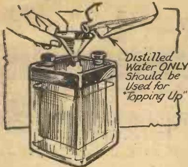
Fig. 4.—Never add acid when "topping" up accumulators.
