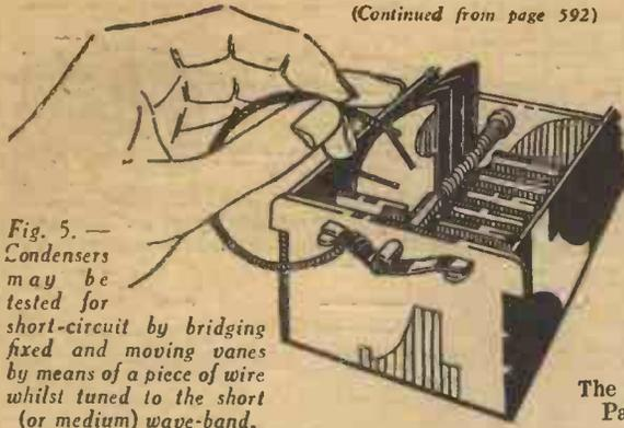
Fig. 5. — Condensers may be tested for short-circuit by bridging fixed and moving vanes by means of a piece of wire whilst tuned to the short (or medium) wave-band.
