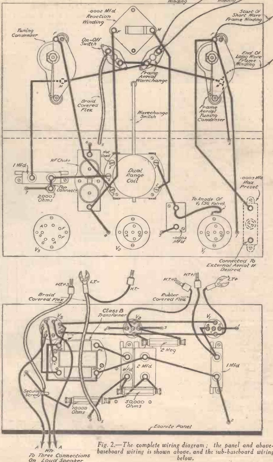
Fig. 2.—The complete wiring diagram; the panel and above-baseboard wiring is shown above, and the sub-baseboard wiring below.
