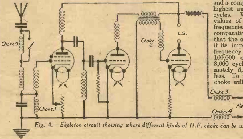
Fig. 4.—Skeleton circuit showing where different kinds of H.F. choke can be used.
