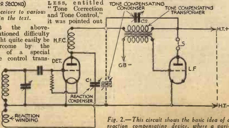
Fig. 2.—This circuit shows the basic idea of a reaction compensating device, where a variable condenser is used to reduce high-note emphasis produced by using reaction.
