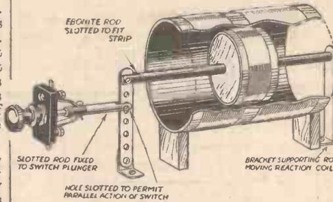
Fitting an adjustable reaction coil.
