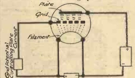
Fig. 6.—Illustrating the function of the three-electrode valve.
