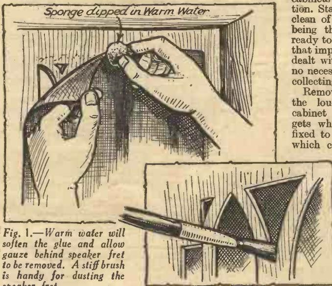
Fig. 1.— Warm water will soften the glue and allow gauze behind speaker fret to be removed. A stiff brush is handy for dusting the speaker fret.
