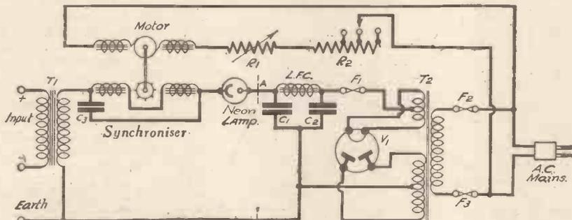
Fig. 1.—The theoretical circuit employed in the "Portovisor."
