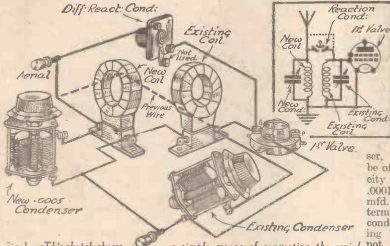
Fig. 1.—This sketch shows a simple means of converting the aerial tuning condenser of a receiver to a simple band-pass arrangement.
