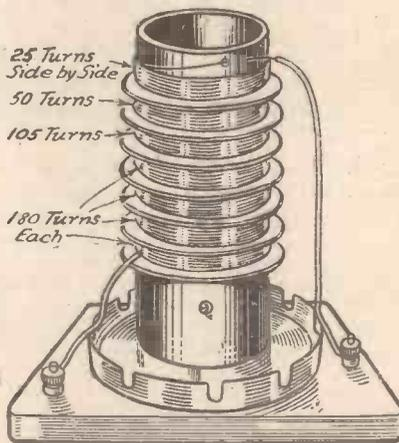
Fig. 6.—Details of an excellent all-wave or universal H.F. choke.
