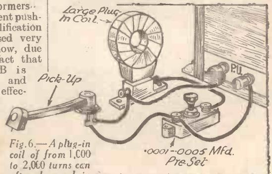
Fig. 6.—A plug-in coil of from 1,000 to 2,000 turns can often be used in series with a pre-set condenser as a pick-up scratch filter.
