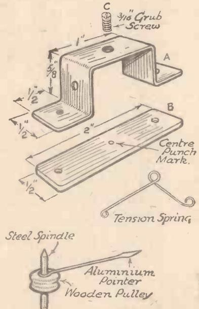
Fig. 2.—The above sketches give all constructional details for the more important parts of the meter described.
