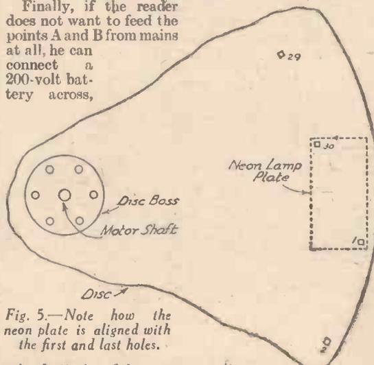
Fig. 5.—Note how the neon plate is aligned with the first and last holes.
