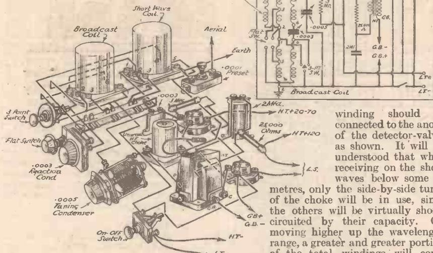
Fig. 5.—A useful all-wave two-valve circuit using two of the coils described.
