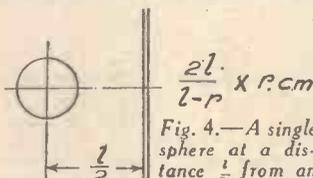
Fig. 4.— A single sphere at a distance  $\frac{l}{2}$  from an earthed boundary wall.
