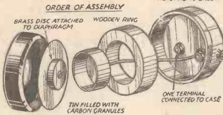
A simple microphone made from a telephone earpiece.
