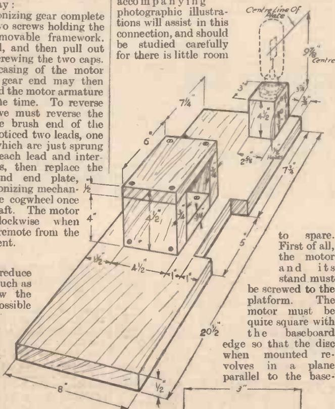
Fig. 9.—The wooden base and motor support.
