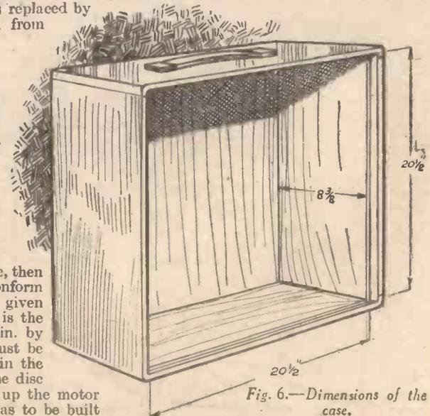
Fig. 6.—Dimensions of the case.
