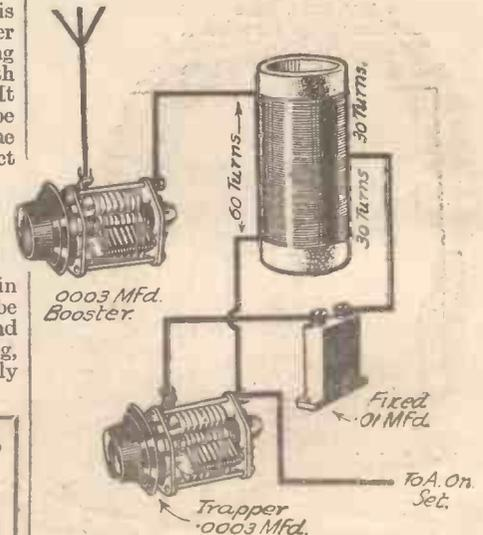
An efficient type of wavetrap.
