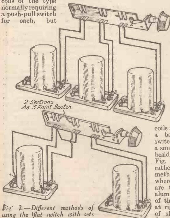
Fig. 2.—Different methods of using the flat switch with sets of the coils described in this series.
