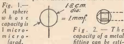
Fig. 2.— The capacity of a metal fitting can be estimated from the size of a sphere which will contain it.
