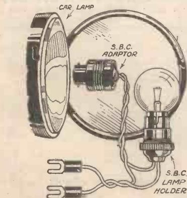
Fig. 4.—First aid apparatus for recharging your wireless battery from the car.
