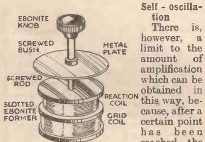
Fig. 3.—A form of "damping-plate" control which was successfully employed in some of the earlier receivers.
