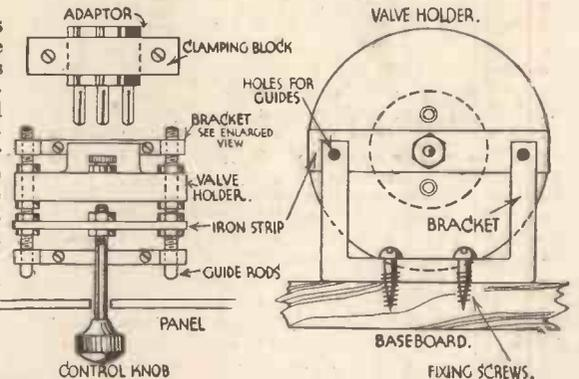
Fig. 4.—A valve holder may be converted as shown here to provide a very efficient switch.
