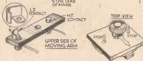
A rotary switch for H.T. eliminator.
