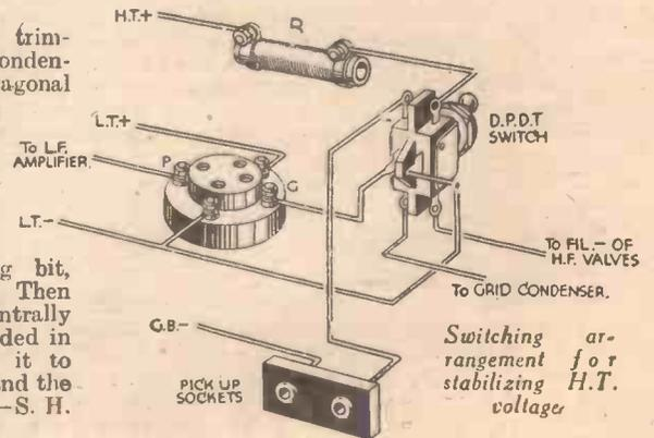
Switching arrangement for stabilizing H.T. voltage
