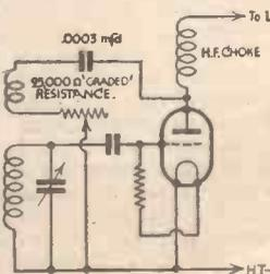
Fig. 5.—Resistance-controlled reaction. The variable reaction condenser is replaced by a fixed condenser and "graded" variable resistance.
