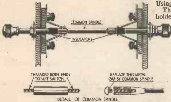
Fig. 1.—Two switches "back-to-back" to act as change-over switch.
