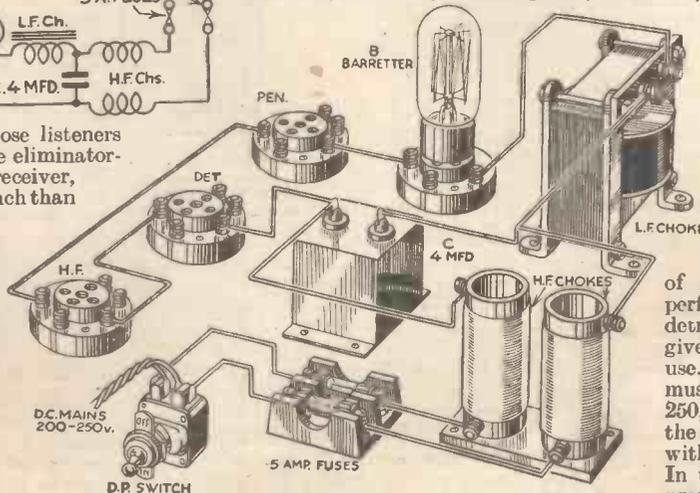
Fig. 2.—Heater circuit diagram showing the inclusion of suitable smoothing and interference-suppressor chokes.
