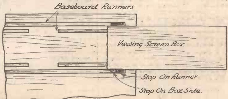
Fig. 5.—Adding stops to act as registers for the correct focusing positions.
