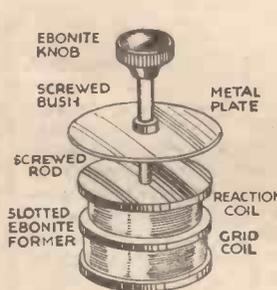
Fig. 3.—A form of "damping-plate" control which was successfully employed in some of the earlier receivers.
