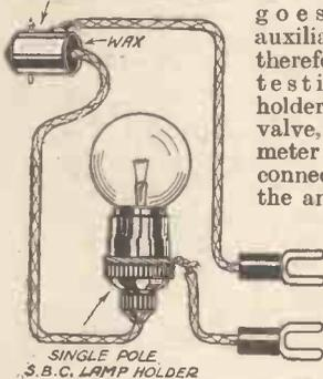
Fig. 5.—Modification of Fig. 4 when the "one-wire" system is employed.
