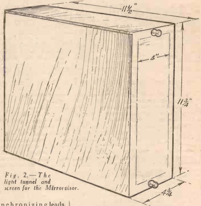
Fig. 2.—The light tunnel and screen for the Mirrorvisor.
