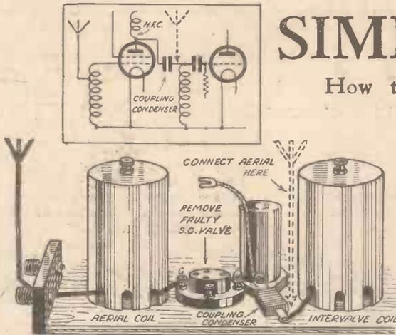
Fig. 6.—How to cut out the H.F. stage of a set in the event of an S.G. valve failure.
