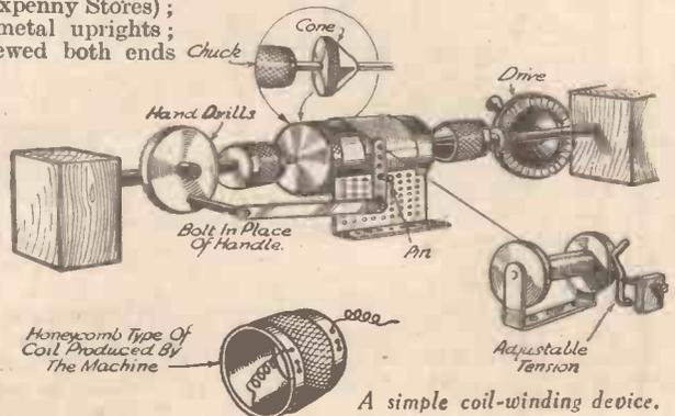
A simple coil-winding device.
