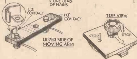
A rotary switch for H.T. eliminator.
