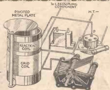
Fig. 2.—A method of reaction control in which two fixed coils are used in conjunction with a "damping-plate."
