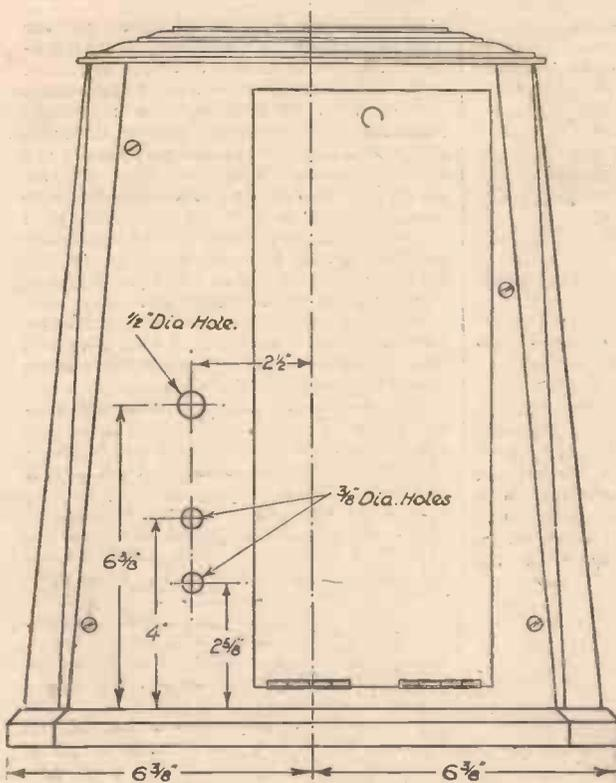
Fig. 3.—Drilling details for the cabinet front.
