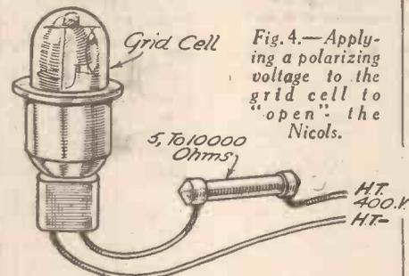
Fig. 4.—Applying a polarizing voltage to the grid cell to "open" the Nicols.
