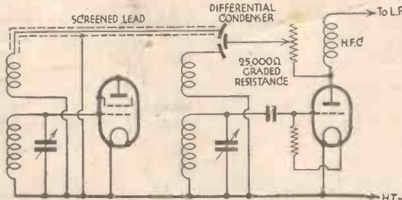
Fig. 8.—A skeleton circuit showing how double reaction can be obtained by feeding back from the detector anode to the grid of both this and the preceding valve.
