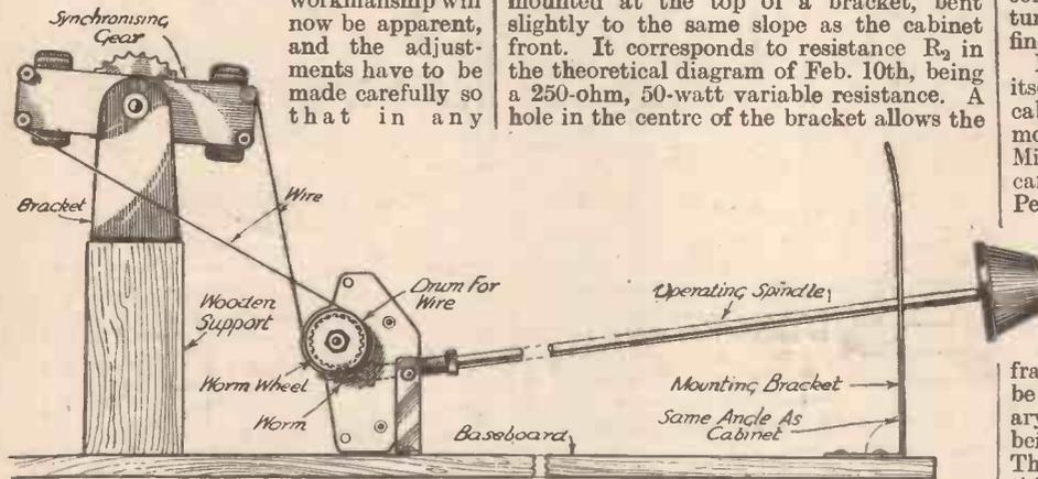
Fig. 1.—The arrangement of the "framing" control.
