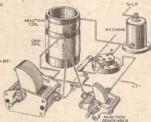
Fig. 4.—The above theoretical and pictorial circuits show the arrangement of the Reinartz system of reaction which is now universally employed.
