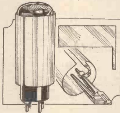
Fig. 7.—How to make a simple and effective valve screen for an unmetallized valve. The lug is connected to the negative filament pin or the cathode pin.
