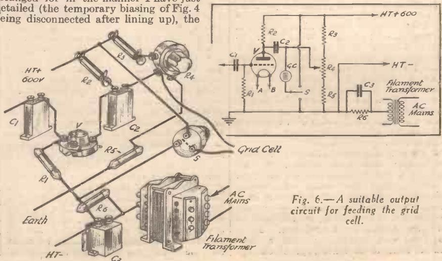
Fig. 6.—A suitable output circuit for feeding the grid cell.
