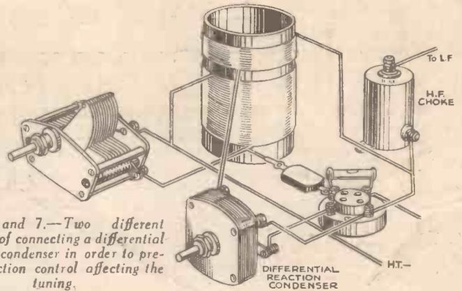
Figs. 6 and 7.—Two different methods of connecting a differential reaction condenser in order to prevent reaction control affecting the tuning.
