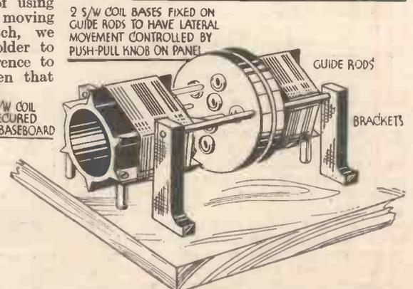
Fig. 5.—Short-wave coils which are assembled to plug-in and thus avoid switches.
