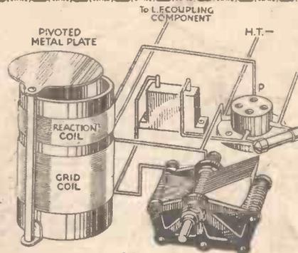
Fig. 2.—A method of reaction control in which two fixed coils are used in conjunction with a "damping-plate."
