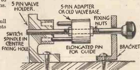
Fig. 3.—Using a valve base or similar adaptor for switching purposes.
