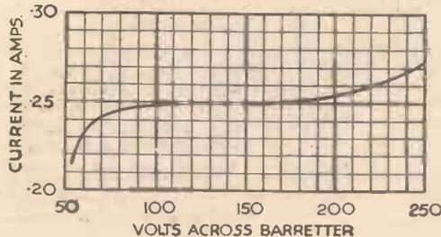
Fig. 4.—Typical barretter curve.
