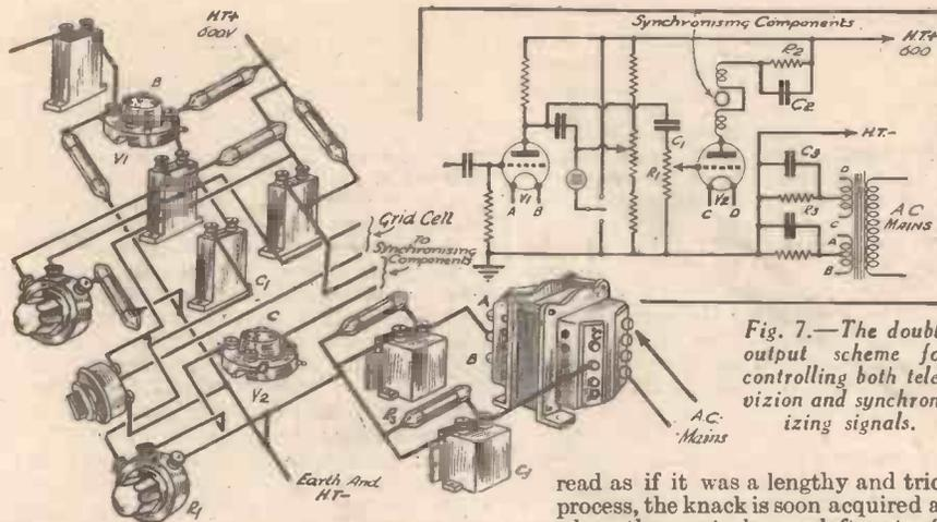
Fig. 7.—The double output scheme for controlling both television and synchronizing signals.
