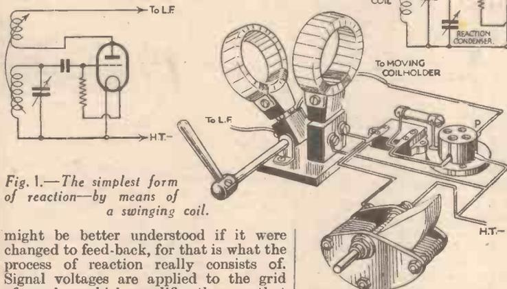
Fig. 1.—The simplest form of reaction—by means of a swinging coil.
