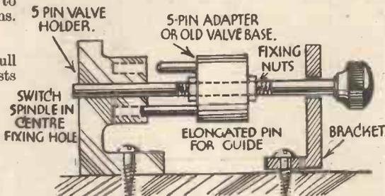
Fig. 3.—Using a valve base or similar adaptor for switching purposes.
