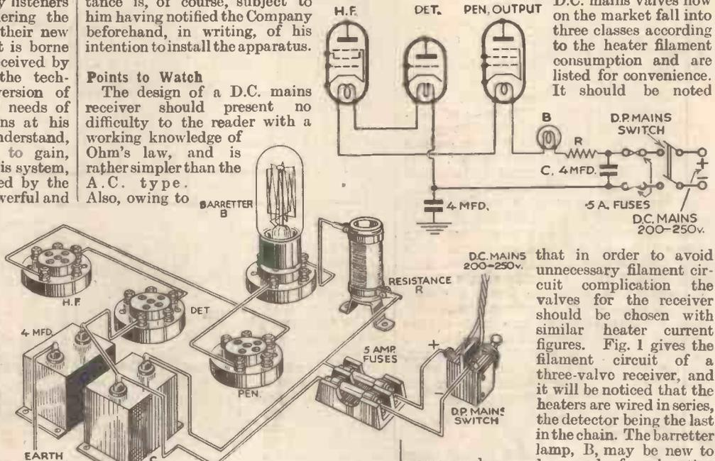
Fig. 1.—Heater circuit diagram shown pictorially and theoretically.
