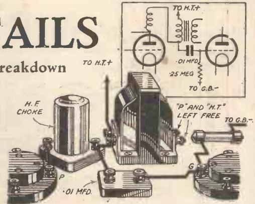
Fig. 8.—Connecting a broken transformer to work as a choke.
