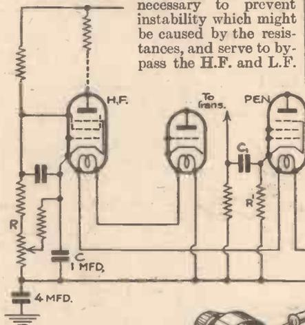
Fig. 3.—Heater and grid circuit arrangement.
