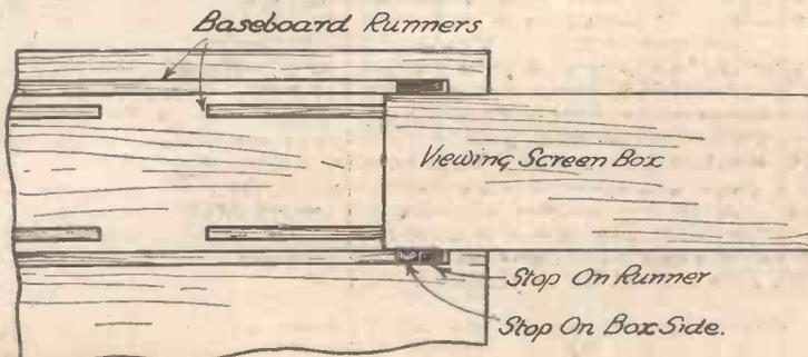
Fig. 5.—Adding stops to act as registers for the correct focusing positions.
