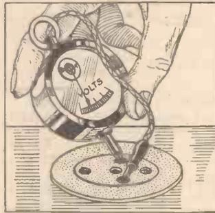
Fig. 2.—Testing filament voltage at the valve holder.
