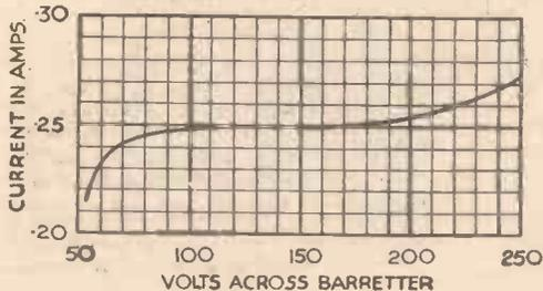
Fig. 4.—Typical barretter curve.
