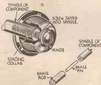
A neat method of fitting extension spindles.
