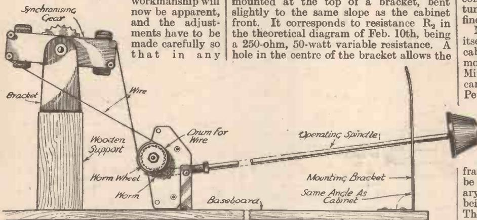
Fig. 1.—The arrangement of the "framing" control.
