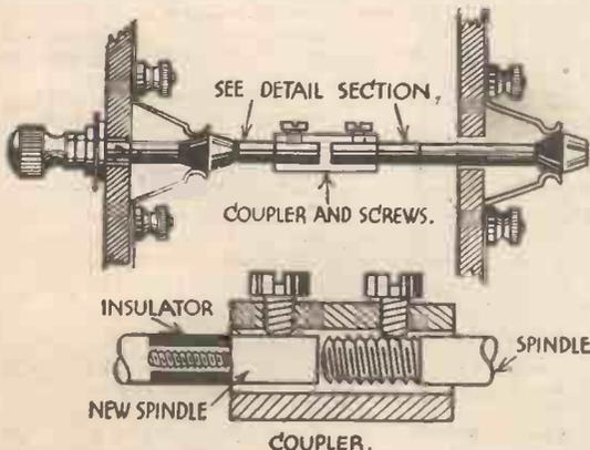
Fig. 2.—Coupling two or more push-pull switches to operate simultaneously.
