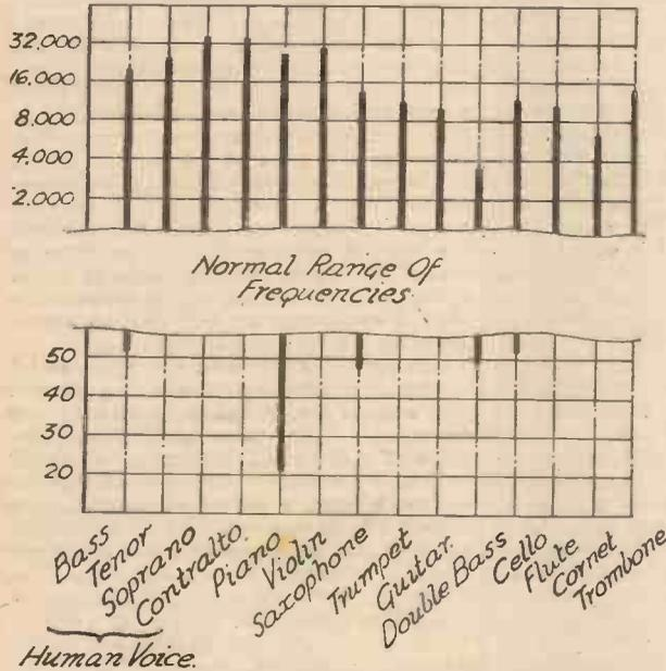
Fig. 1.—The range below 50 cycles and above 2,000 cycles which is covered by the human voice and the majority of popular instruments.
