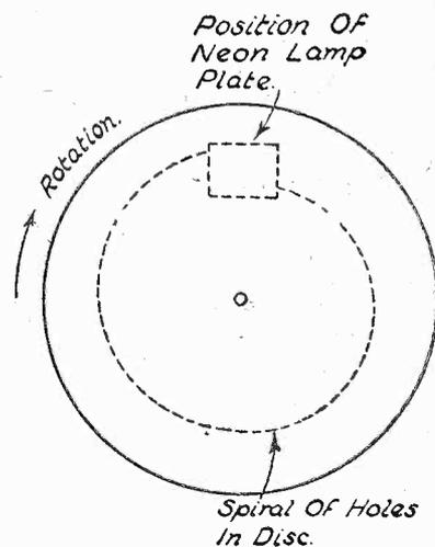
Fig. 4.—Mount the neon lamp centrally at the top back of the disc for reception.
