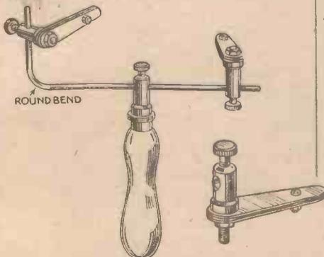
Easily-made soldering tweezers.
