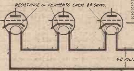
Fig. 4.—Ohm's Law enables us to find the current passing through these valves.
