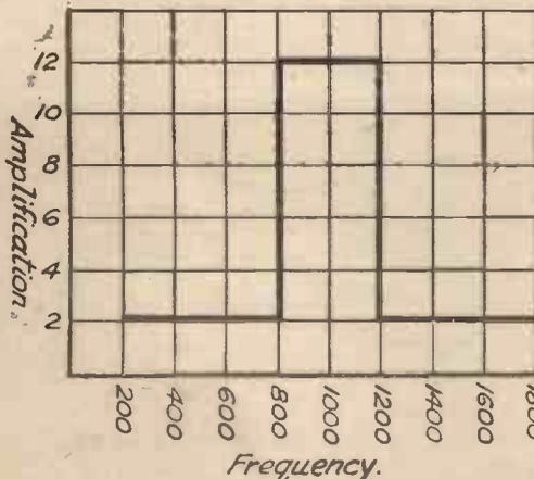
Fig. 2.—This diagram illustrates the ideal which should be aimed at in designing the frequency response of a broadcast receiver.
