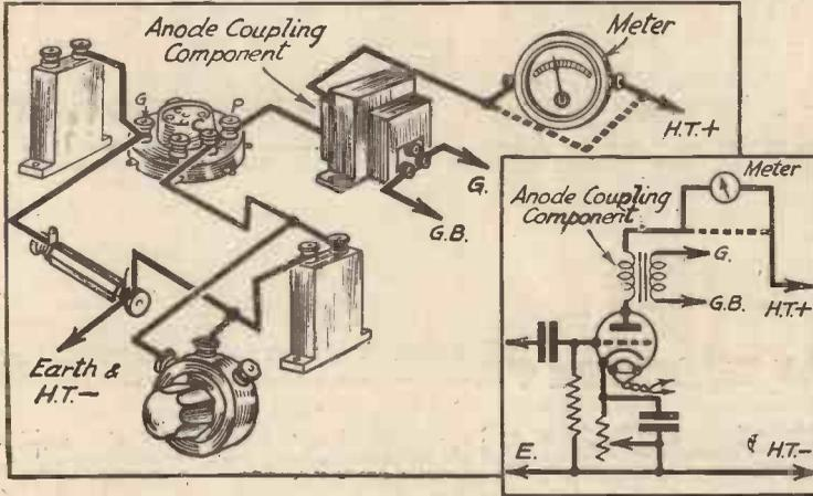
Fig. 3.—The best way to determine the correct G.B. voltage for an L.F. valve is to insert a milliammeter in the anode circuit and vary the bias until the correct anode-current reading is obtained.
