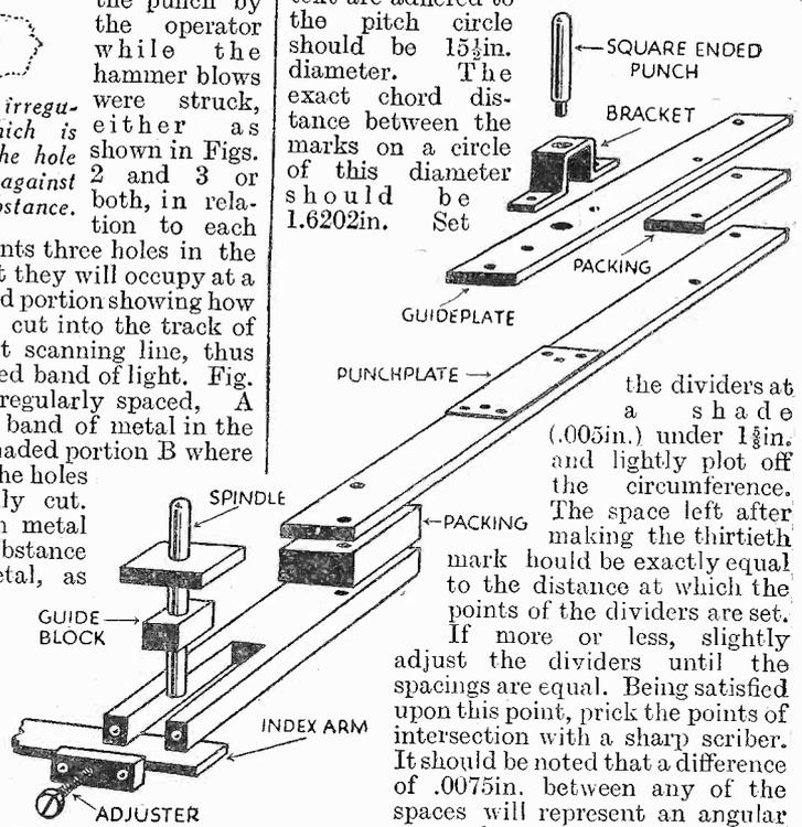
Fig. 7.—Assembly details of the complete apparatus.
