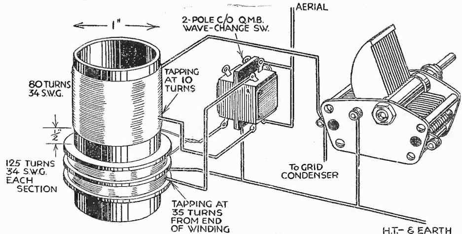
Fig. 3.—Details of an excellent aerial coil with aerial transfer tapping. Constructional details can be obtained from the article "Making Your Own Screened Coils," on page 633 of "Practical Wireless" dated December 9th, 1933.
