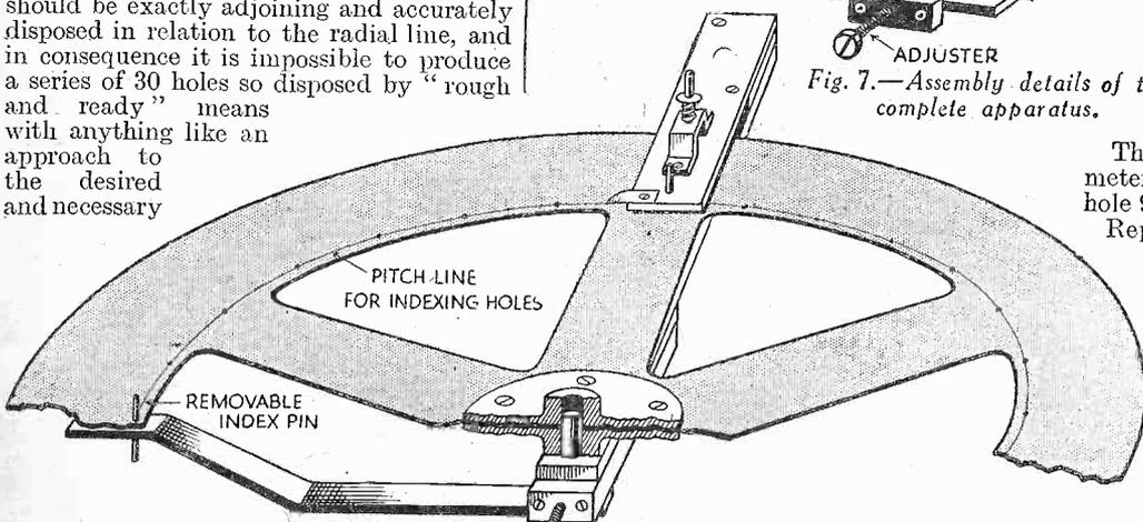
Fig. 5.—The device which is described in this article and which enables the holes to be accurately positioned and cleanly cut.
