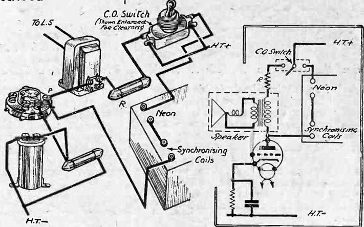
Fig. 1.—The method of switching from "sound" to "vision" when the apparatus is wired in series with the anode of the output valve.
