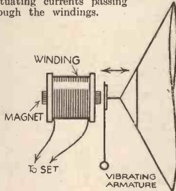
Fig. 2.—This sketch shows the working parts of a moving-iron speaker.
