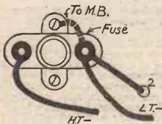
The broken line indicates the earthing wire which has to be fitted.
