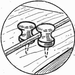
Fig. 2.—Glass-headed photographic pins are useful for anchoring wiring.
