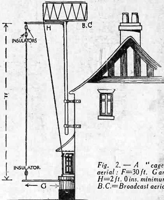
Fig. 2.—A "cage" aerial: F=30ft. G and H=2ft. 0ins. minimum. B.C.=Broadcast aerial.
