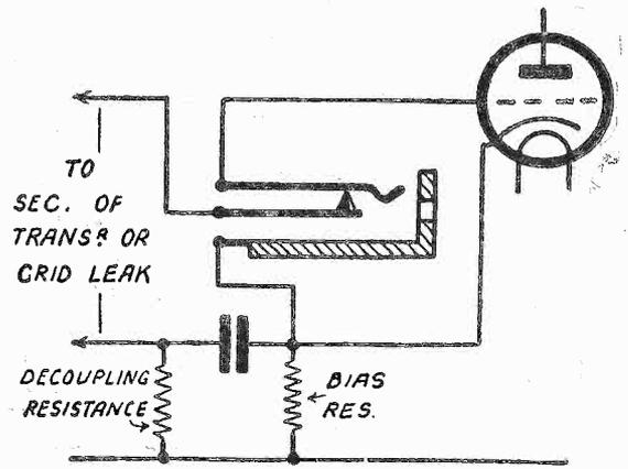
Fig. 2.—A modification of Fig. 1 for use with indirectly-heated valve.
