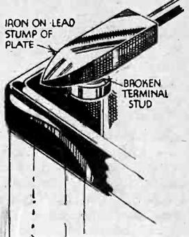
Method of removing broken terminals from accumulators.
