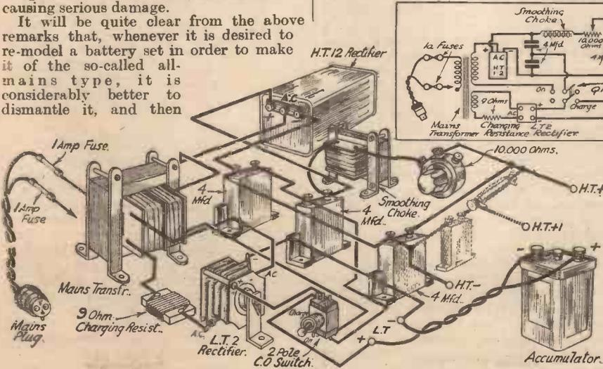
Fig. 2.—The combined H.T. unit and trickle charger shown above is for A.C. operation.
