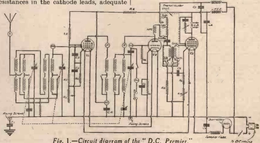
Fig. 1.—Circuit diagram of the "D.C. Premier."
