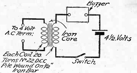
Fig. 5.—Method of using a buzzer to provide oscillations.
