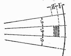
Method of marking out and punching a television scanning disc.
