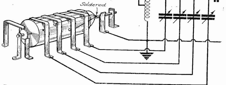
Fig. 8.—A remote tuning scheme which makes use of a relay similar to that shown in Fig. 6. This works in conjunction with a number of pre-set condensers.
