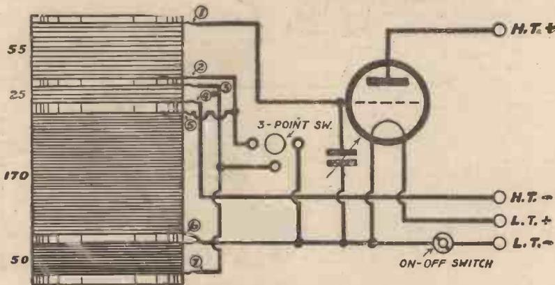
Theoretical diagram of the Heterodyne Wavemeter.
