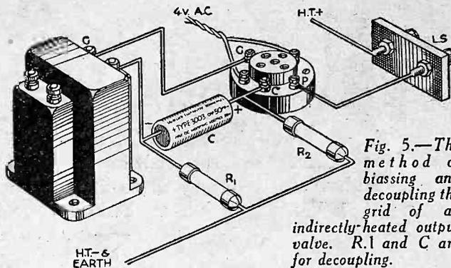
Fig. 5.—The method of biasing and decoupling the grid of an indirectly-heated output valve. R.1 and C are for decoupling.
