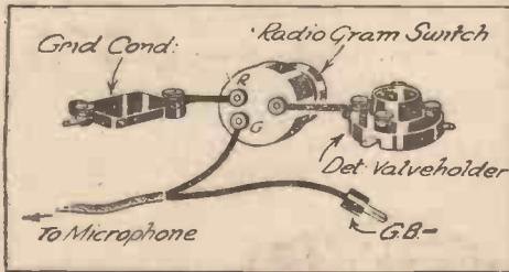
Fig. 1.—This diagram shows the simple connections of a radiogram switch to the detector circuit of a battery receiver.
