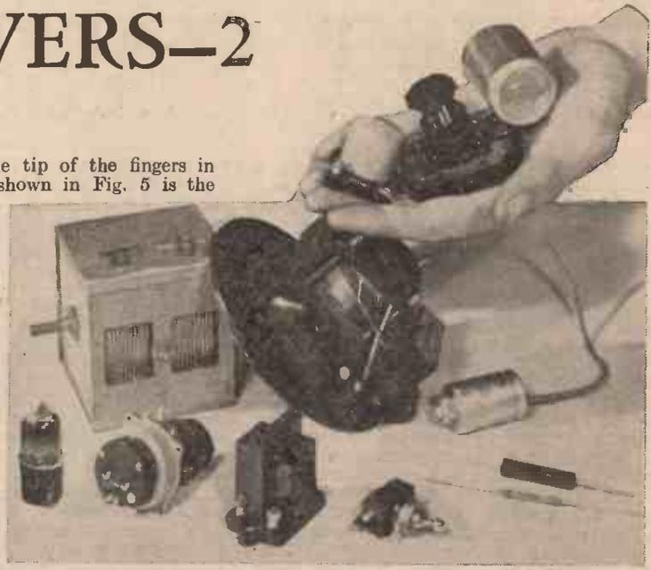
Fig. 1.—An interesting photograph which shows a number of new midget components: their size can be judged by comparison with the hand.
