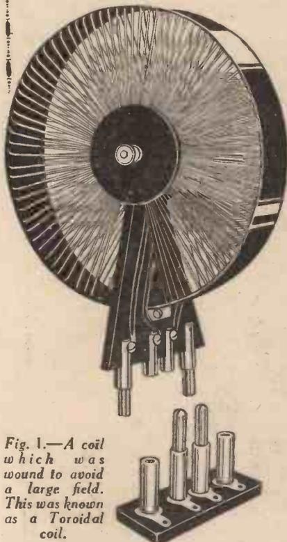
Fig. 1.—A coil which was wound to avoid a large field. This was known as a Toroidal coil.
