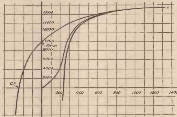
Fig. 1.—The hysteresis loop of a high-grade cobalt magnet steel.
