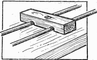
Fig. 1.—Small wooden cleats keep the base-board wiring neat.
