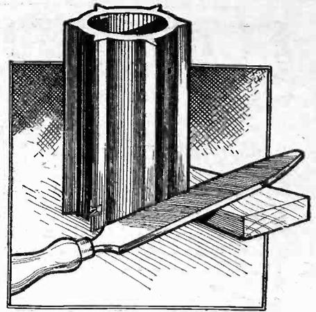
A method of slotting ribbed coil formers.
