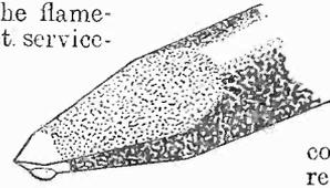
Fig. 4.—The tip should be filed as shown in this illustration.
