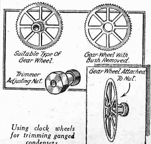
Using clock wheels for trimming ganged condensers.
