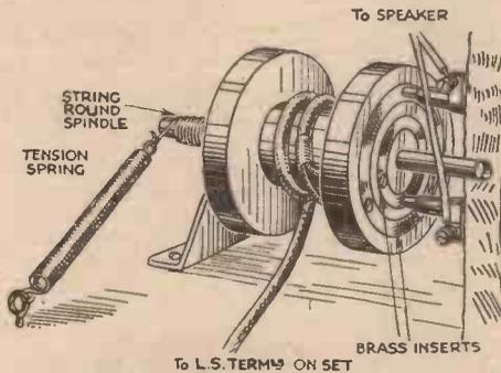
An automatic winding device for L.S. leads.
