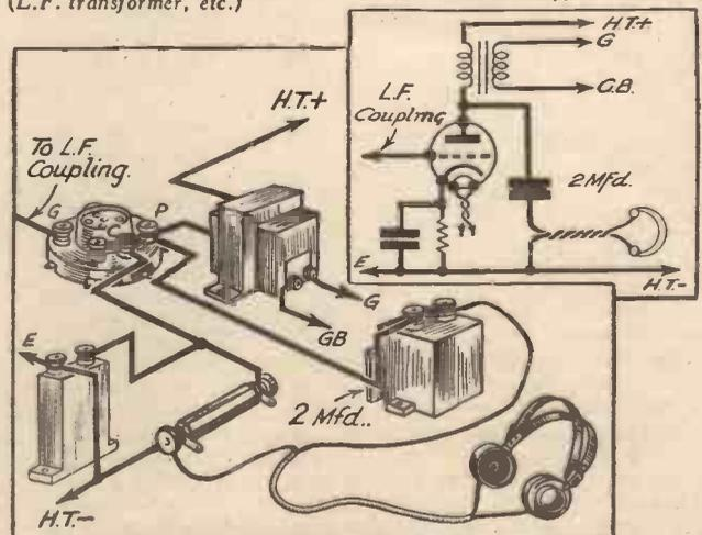
Fig. 2.—A better way of connecting the 'phones or speaker when cutting out an L.F. stage is shown above. This is particularly useful in the case of a mains set, since it isolates the 'phones from the H.T. supply.
