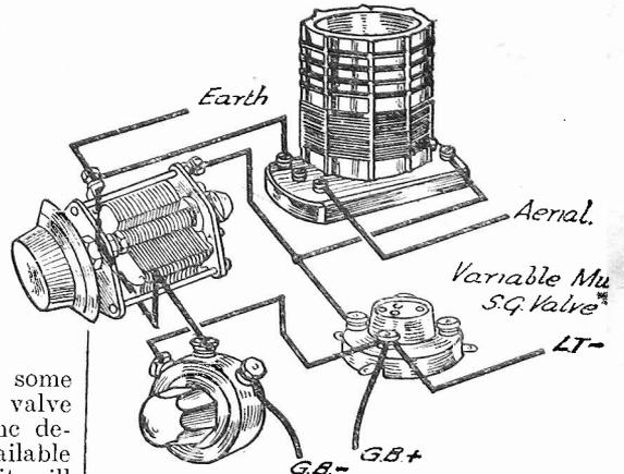
Fig. 4.—Gain control by variable-mu S.G. valve in battery set.
