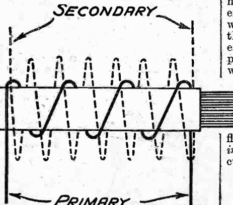
Fig. 6.—A simple transformer made of two coils of wire.
