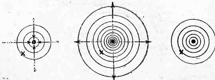
Figs. 2, 3 and 4.—Diagrams showing the lines of force round a wire carrying an electric current.
