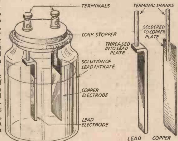
This sketch shows the construction of the photo-electric cell described.
