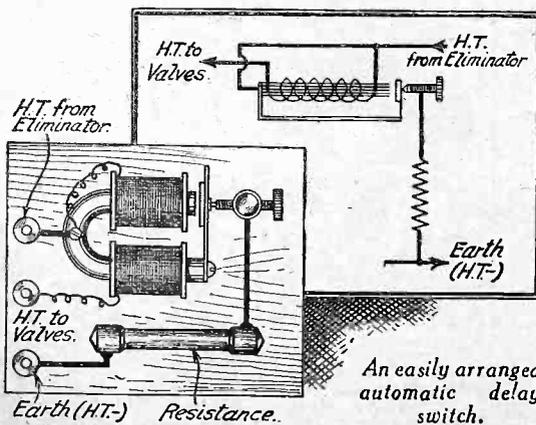
An easily arranged automatic delay switch.
