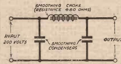
Fig. 7.—The voltage obtainable from this mains unit after the current has passed through the smoothing choke can be determined by Ohm's Law.
