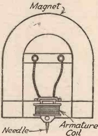
Fig. 1.—The principal parts of a pick-up are shown in this diagram.
