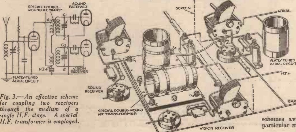
Fig. 3.—An effective scheme for coupling two receivers through the medium of a single H.F. stage. A special H.F. transformer is employed.
