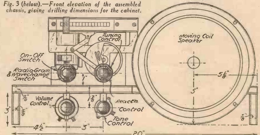
the template once again for this purpose. Fix the escutcheon plate. For convenience in wiring the speaker was held to the baseboard by two small brackets, but I mentioned that the four connecting leads should be left longer than actually required. This was to allow the speaker flange to be screwed to the cabinet front, which acts as the baffle.
