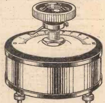
Fig. 5.—A variable condenser of the compression type.
