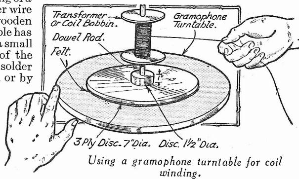
Using a gramophone turntable for coil winding.
