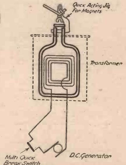
Fig. 9.—Another commercial form of magnetizer, the advantages of which are described.
