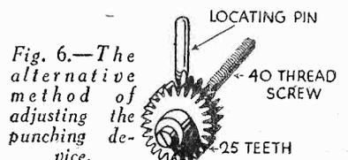
Fig. 6.—The alternative method of adjusting the punching device.
