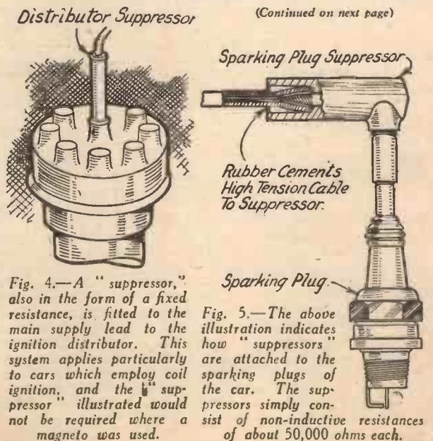
Fig. 4.—A "suppressor," also in the form of a fixed resistance, is fitted to the main supply lead to the ignition distributor. This system applies particularly to cars which employ coil ignition, and the "suppressor" illustrated would not be required where a magneto was used.
