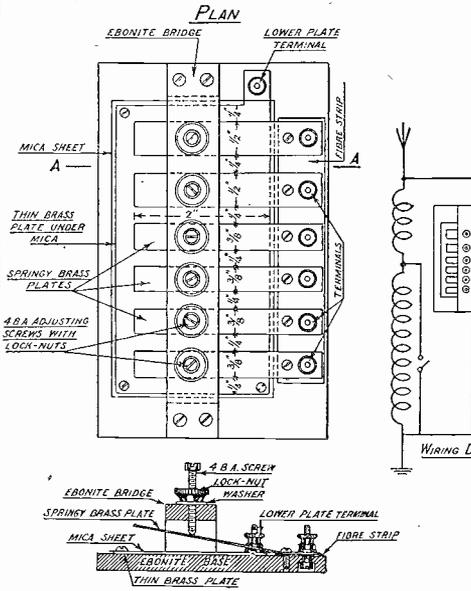
A simple method of making a bank of pre-set condensers.
