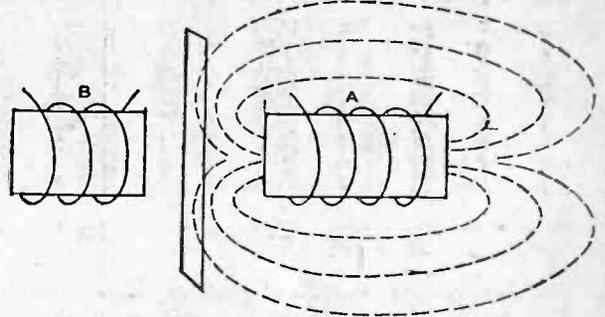
Fig. 3.—Employing an iron screen to "protect" B.
