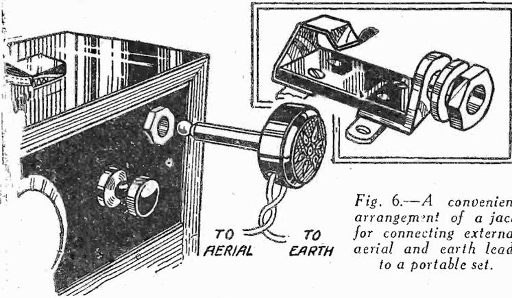
Fig. 6.—A convenient arrangement of a jack for connecting external aerial and earth leads to a portable set.
