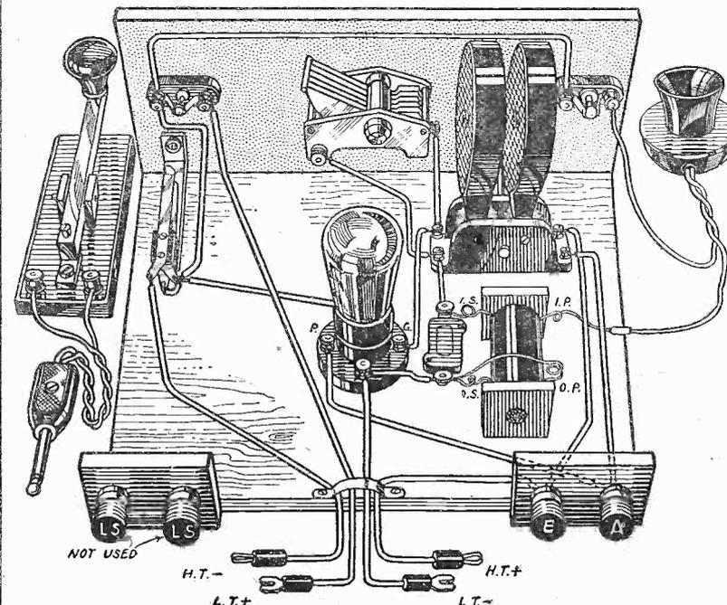
Fig. 4. Circuit diagram and layout for a simple one-valve transmitter.
