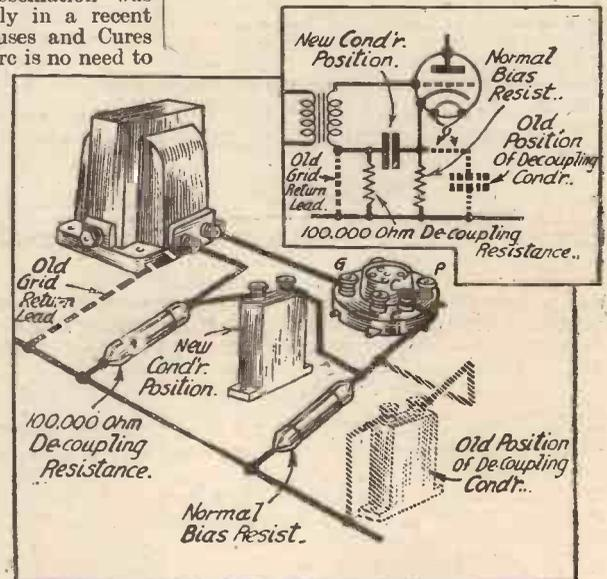
Fig. 4.—Mains hum and L.F. instability in a mains set can often be cured by fitting a grid de-coupling resistance as shown above.
