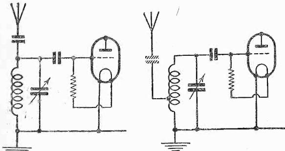
Fig. 1.—The usual form of aerial-grid circuit employed in simple receivers.
