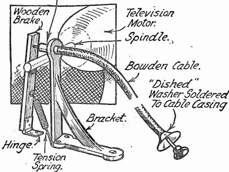
Simple speed regulator for a television motor.
