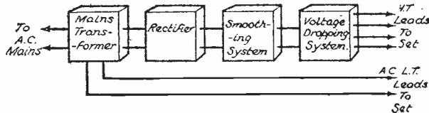
Fig. 1.—This diagram shows the principal parts of a mains unit arranged in their correct sequence. The last section—for voltage dropping—generally forms a part of the receiver.
