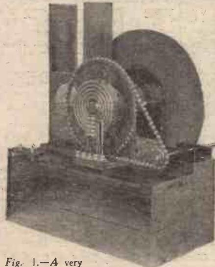
Fig. 1.—A very early type experimental receiver showing how the current was fed into the motor and also the chain framing device.
