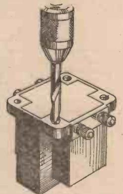
Countersinking fixing holes in components.
