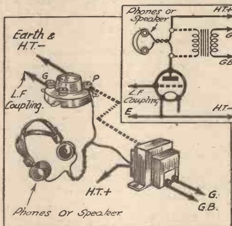
Fig. 1.—An L.F. stage can easily be cut out by connecting a pair of 'phones or a loud-speaker in the anode circuit of the preceding valve in place of the normal coupling component (L.F. transformer, etc.)
