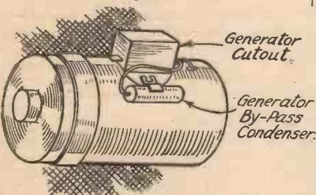
Fig. 3.—Showing the connections of a by-pass condenser used in conjunction with a generator. The condenser case is "earthed" to the frame of the generator.
