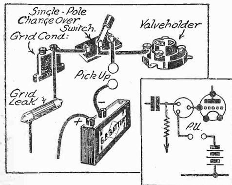
*This diagram shows how the change-over switch may be fitted.*
