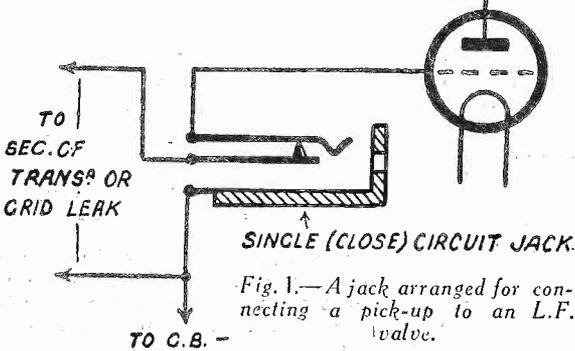
Fig. 1.—A jack arranged for connecting a pick-up to an L.F. valve.
