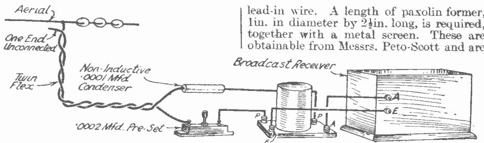
Fig. 5.—Connections for anti-interference device.
