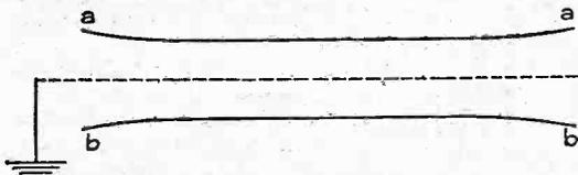
Fig. 1.—Showing simple electrostatic screening.
