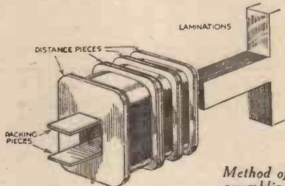
Method of assembling transformer windings on individual spools.
