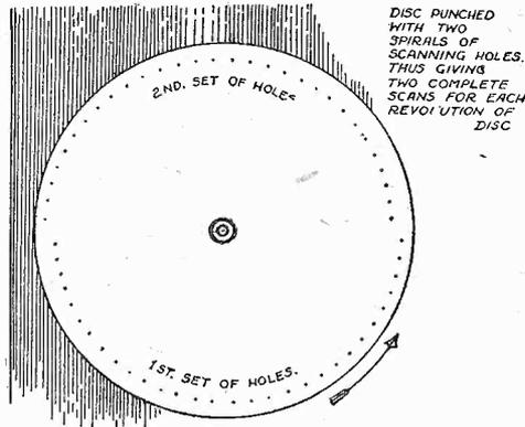
EACH HOLE SPACED 1/64 GIVING PICTURE WIDTH OF 15/32
