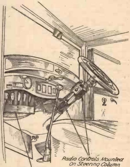
Fig. 1.—This pictorial illustration shows the arrangement of a receiver and its controls in a typical car. Note the mounting of the principal controls on the steering column.
