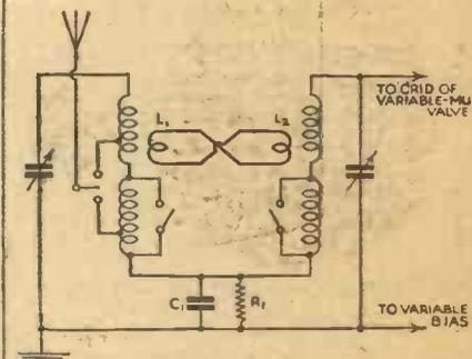
Fig. 4.—A band-pass circuit of the "mixed-coupling" type.
