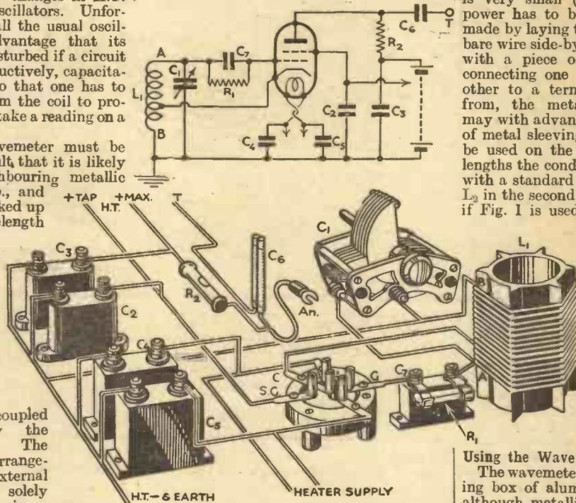
Fig. 1.—Theoretical and pictorial diagrams of an electron-coupled oscillator.
