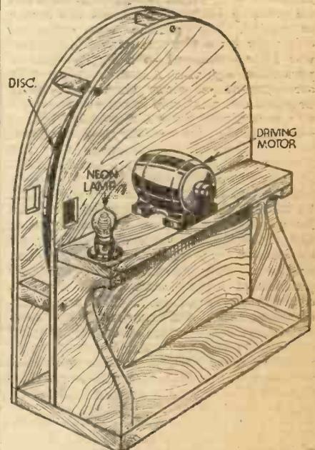
Fig. 2.—A novel form of television receiver design which has the advantage of being quite cheap to build.
