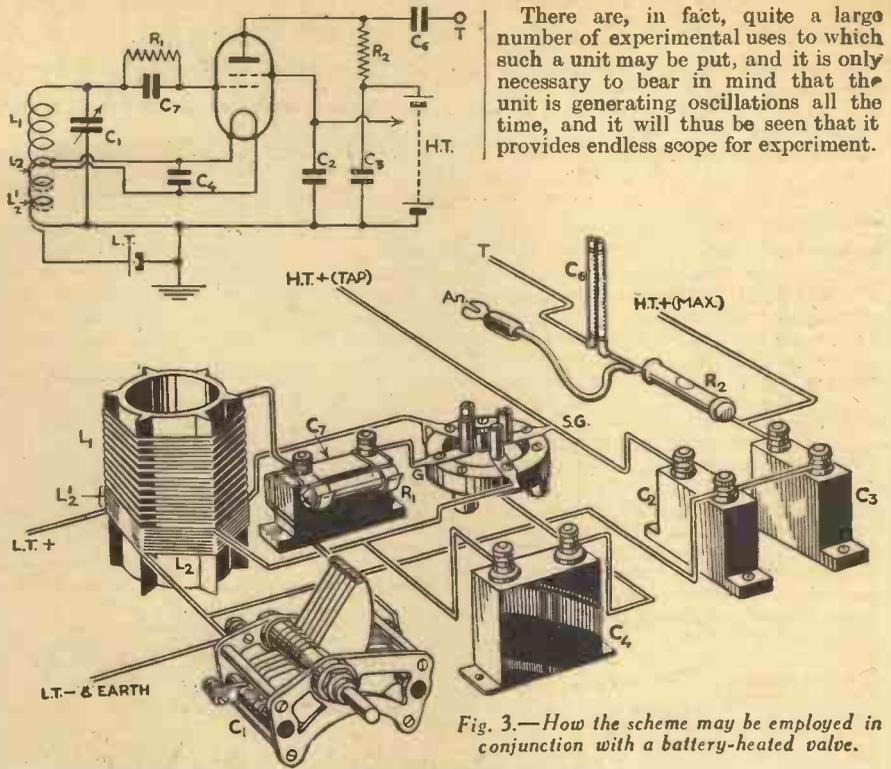
Fig. 3.—How the scheme may be employed in conjunction with a battery-heated valve.
