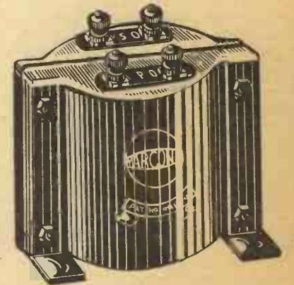
Fig. 10.—One of the first L.F. transformers of the shrouded type.
