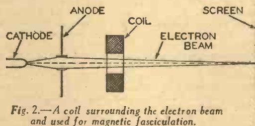
Fig. 2.—A coil surrounding the electron beam and used for magnetic fasciculation.
