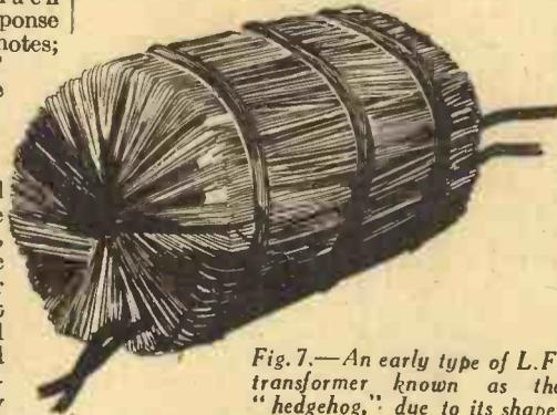
Fig. 7.—An early type of L.F. transformer known as the "hedgehog," due to its shape.
