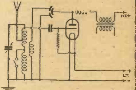
Fig. 2.—A typical tuning circuit combined with a differential-controlled reaction arrangement.
