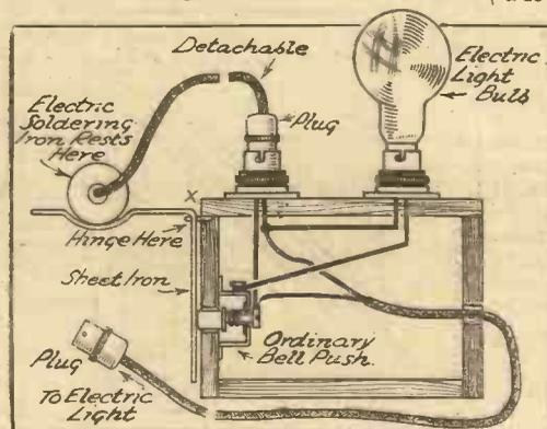
An automatic switching stand for a soldering iron.
