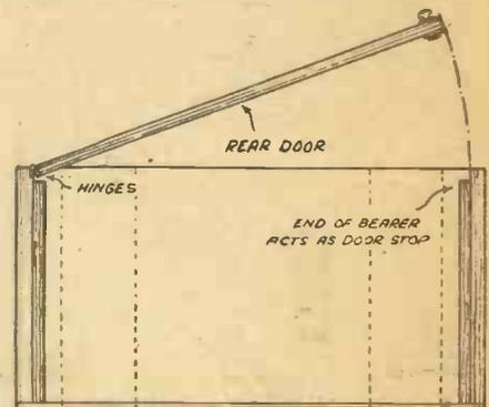
This drawing shows how the lid is fitted.
