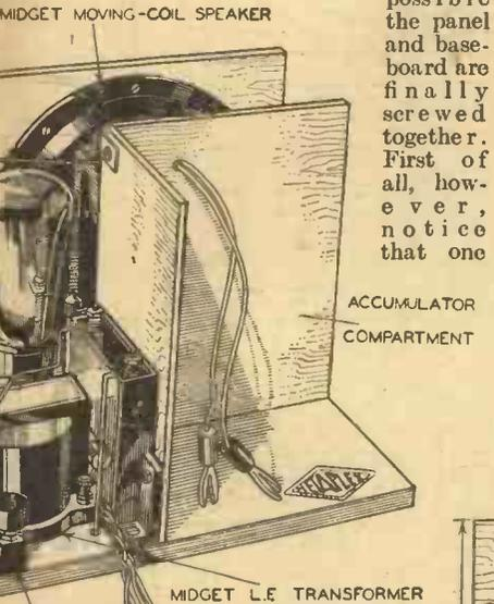
panel bracket is cut short to clear the accumulator compartment. This one, therefore, must be removed from the panel and have part of one arm sawn off.
