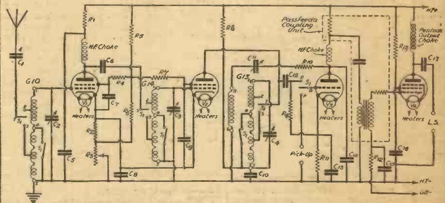
Fig. 5.—Circuit diagram of the Fury Four Super.
