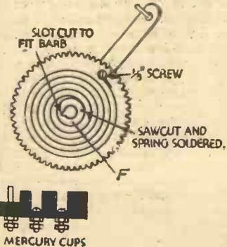
Method of re-mounting the spring.
