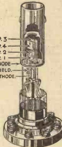
Fig. 3.—The normal electrode system of a cathode-ray tube in which the Wehnelt cylinder is indicated as the shield.
