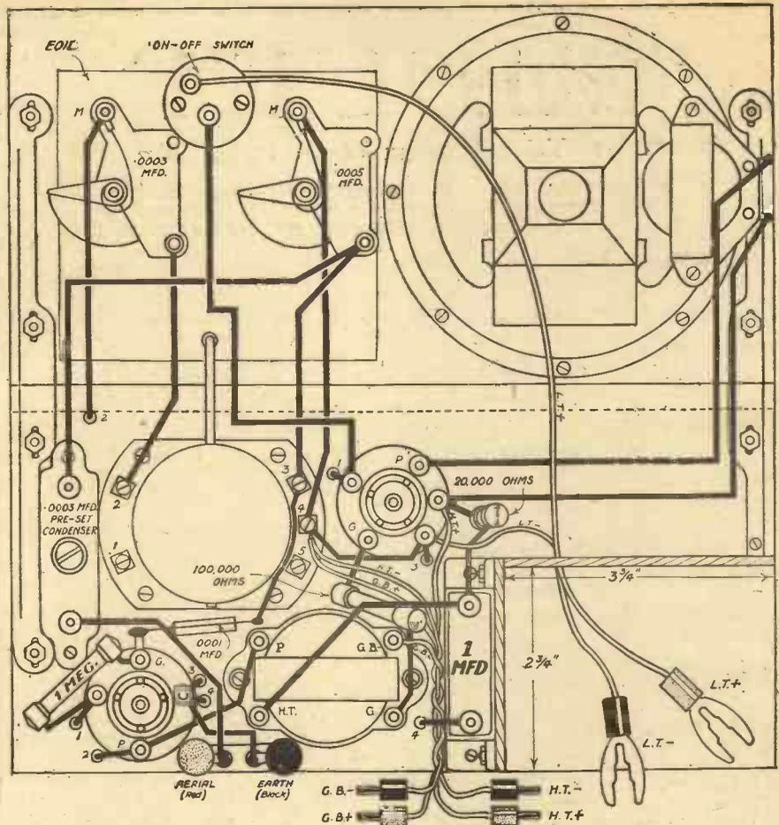
Wiring diagram of the "Master Midget."
