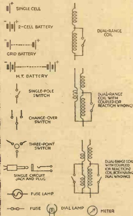
Fig. 1.—These symbols will assist you in reading circuit diagrams.
