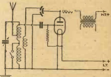
Fig. 2.—A typical tuning circuit combined with a differential-controlled reaction arrangement.
