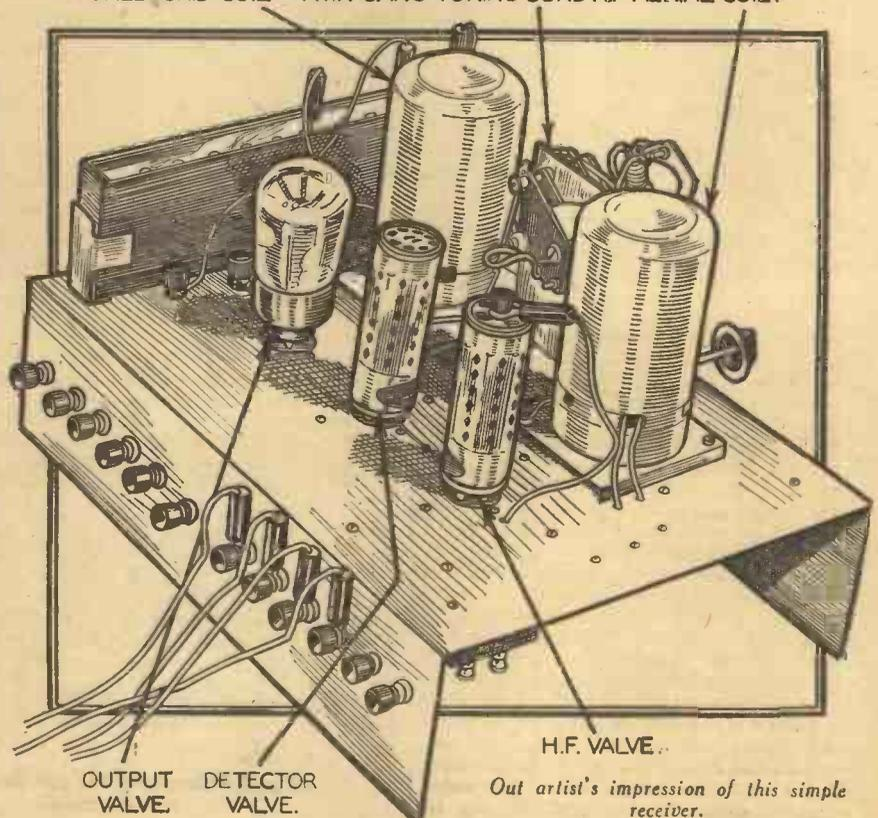
OUTPUT VALVE. DETECTOR VALVE.
