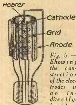
Fig. 5.—Showing the construction of the electrodes in an indirectly-heated valve.
