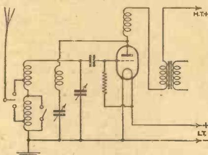
Fig. 3.—Circuit of a tuning coil having an aerial transfer tapping.
