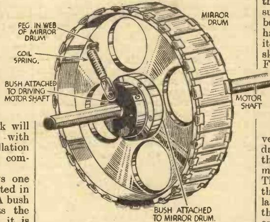
Fig. 1.—Showing one form of flexible coupling which may be used between the driving motor shaft and the mirror drum.
