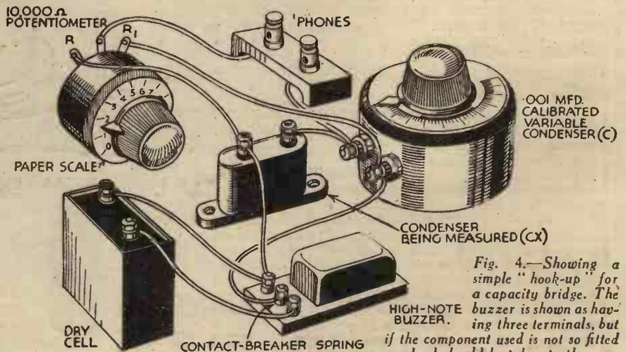
Fig. 4.—Showing a simple "hook-up" for a capacity bridge. The buzzer is shown as having three terminals, but if the component used is not so fitted one lead should be taken to the contact-breaker spring which is internally joined to one end of the windings.
