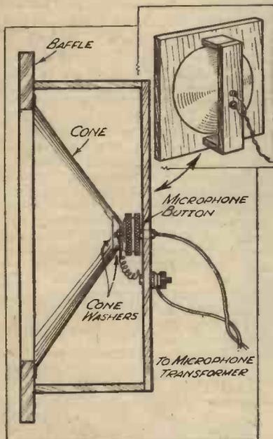
An easily-made super-sensitive microphone.
