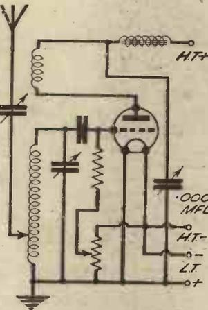
Fig. 1.—A "throttle-control" circuit.
