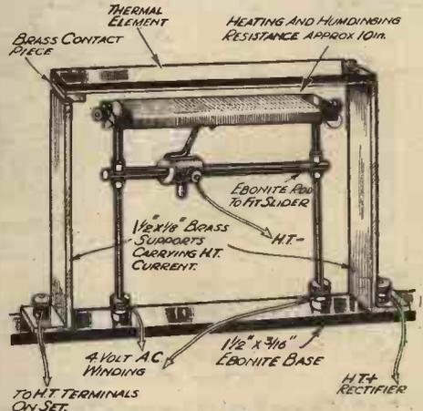
A combined thermal-delay switch and humdinger.
