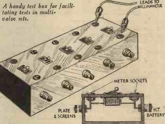
A handy test box for facilitating tests in multi-valve sets.
