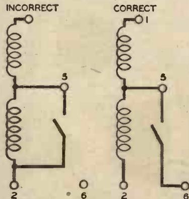
Wave changing connections for G.I.C.7 oscillator coil of £5 Superhet.
