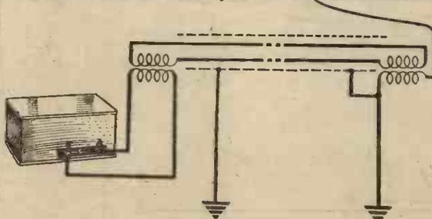
Fig. 2.—An aerial and H.F. transmission line.
