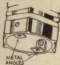
Fig. 3. Showing how the coil former is mounted on an ebonite base.
