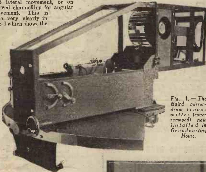
Fig. 1.—The Baird mirror-drum transmitter (cover removed) now installed in Broadcasting House.
