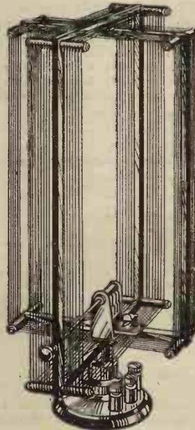
Fig. 7.—A frame aerial having separate windings for medium and long waves. The changer is effected by means of a multi-pole switch.
