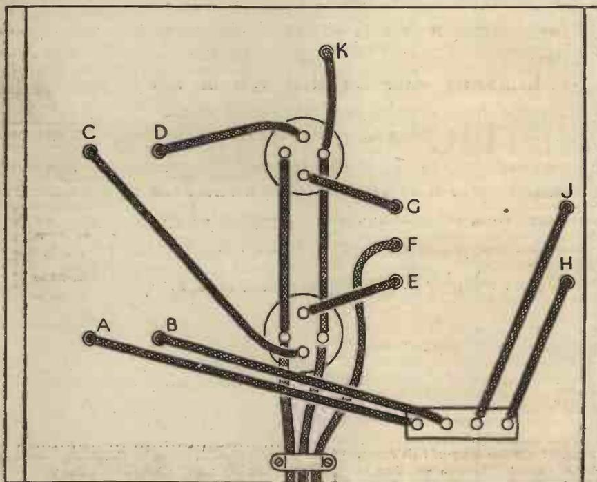
The simple nature of the wiring is clearly shown in the above wiring plans L.T.+ H.T.+ for the push-pull amplifier and below — chassis given here.
