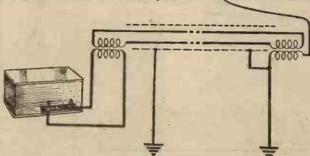
Fig. 2.—An aerial and H.F. transmission line.
