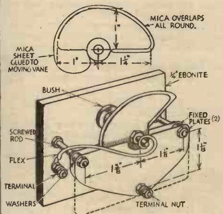
Fig. 5. Constructional details of the reaction condenser described.
