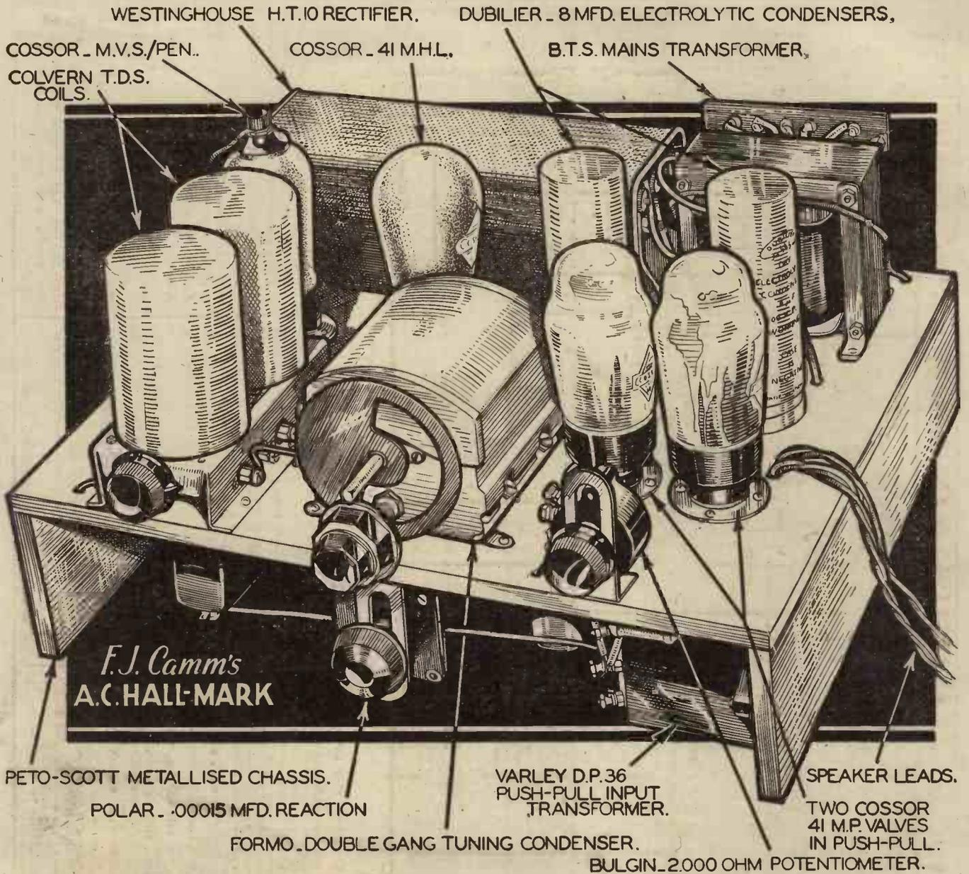
holes for the valve-holders it must be remembered that the MVS/Pen valve-holder requires a 1½ in. hole, whereas the other three require 1 in. holes. Secure the valve-holders centrally in the holes to avoid the possibility of short circuits from the pins to the metallised baseboard. This latter, by the way is supplied already assembled, and Messrs. Peto-Scott Co., Ltd., supply them ready drilled to order.
