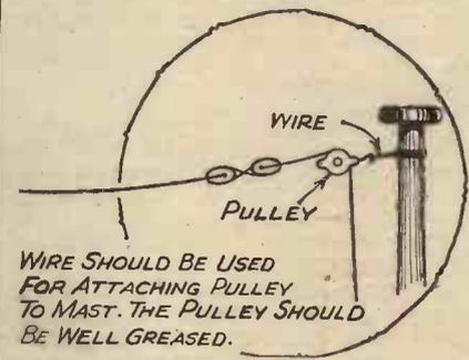
Fig. 9.—Details of the aerial insulators and the method of fixing the aerial to the pole.
