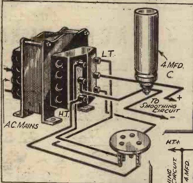
Fig. 1.—The theoretical and practical circuits given here show the connection for a full-wave valve rectifier.
