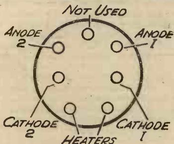
Fig. 3.—Showing the connections to a seven-pin rectifier. The illustration shows the valve base—not the holder.
