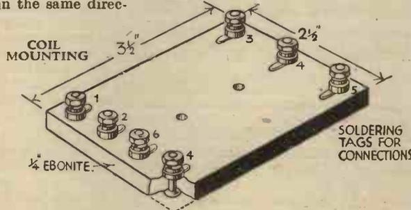
bracket. An ebonite base is used, and two round-headed 4 B.A. screws are tapped into this, placing a soldering tag under the head of each. The next requirement is a short length of springy brass, and this is fitted in the position shown by means of another pair of 4 B.A. screws again tapped into the ebonite, and a soldering tag is again placed under the head of one of these.
