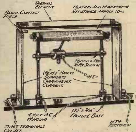
A combined thermal-delay switch and humdinger.
