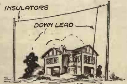
Fig. 8.—An inverted L-Type aerial.
