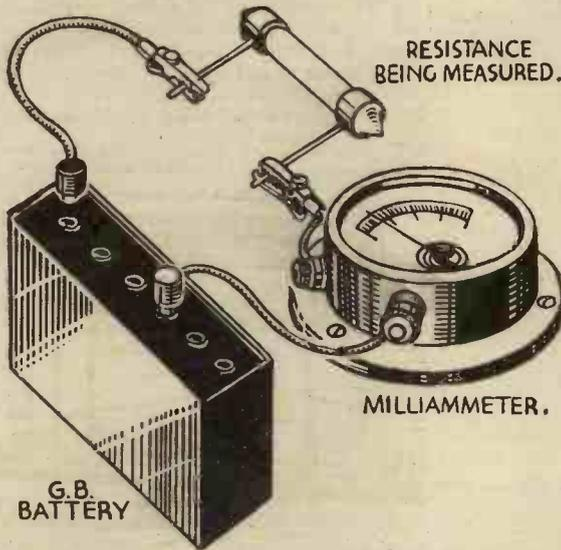
Fig. 1. Resistance values can easily be measured by employing the connections shown here. It will be seen that the resistance to be measured is wired in series with a milliammeter and battery.
