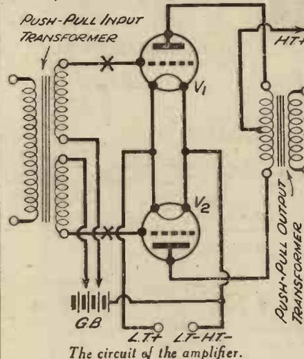
push-pull amplifier in question is so low (largely due to the use of efficient modern valves), and the price of H.T. batteries has been so much reduced, that we feel fully justified in reviving interest in push-pull.
