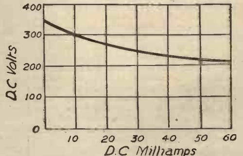
Fig. 2.—This graph shows how the output of a typical rectifier varies with the current load.
