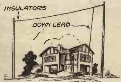
Fig. 8.—An inverted L-Type aerial.
