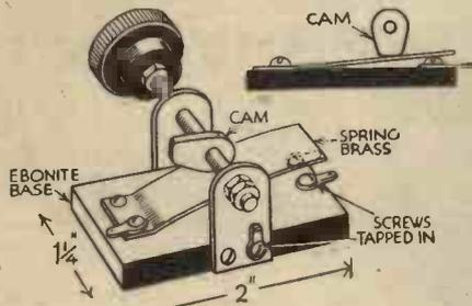
Fig. 4. Details of the easily-made three-point switch.
