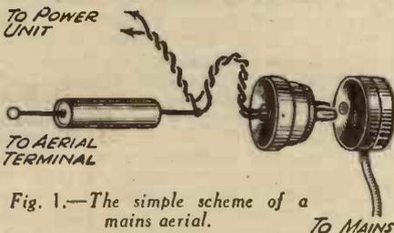
Fig. 1.—The simple scheme of a mains aerial.
