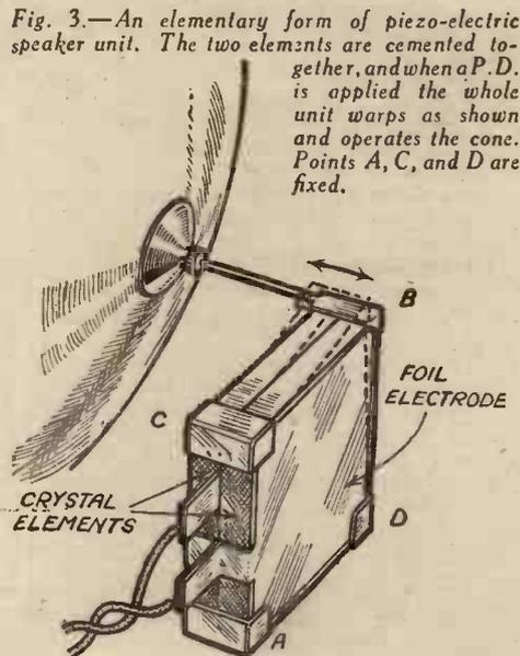
Fig. 3.—An elementary form of piezo-electric speaker unit. The two elements are cemented together, and when a P.D. is applied the whole unit warps as shown and operates the cone. Points A, C, and D are fixed.
