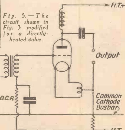
Fig. 5.—The circuit shown in Fig. 3 modified for a directly-heated valve.
