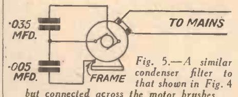
Fig. 5.—A similar condenser filter to that shown in Fig. 4 but connected across the motor brushes.
