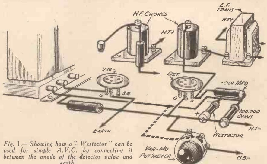
Fig. 1.—Showing how a "Westector" can be used for simple A.V.C. by connecting it between the anode of the detector valve and earth.
