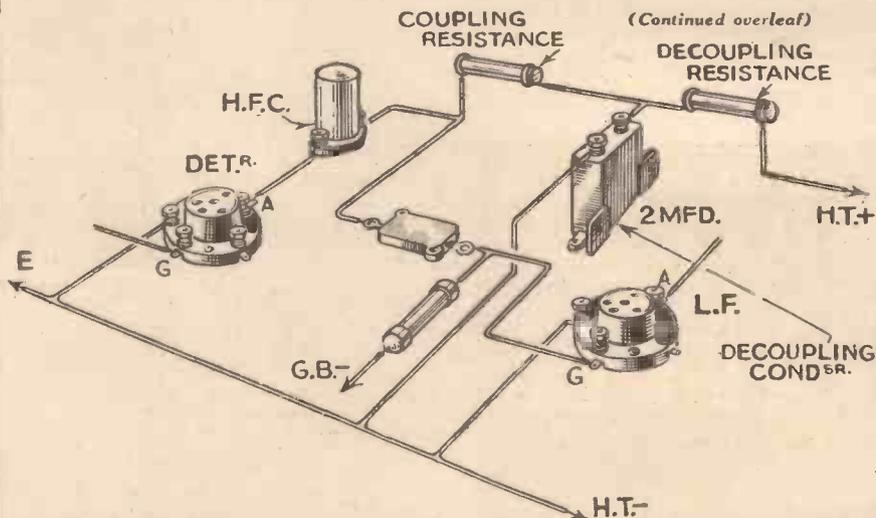
Fig. 1.—Showing the R.C.C. coupling between detector and L.F. valves. The various parts are referred to in the text.
