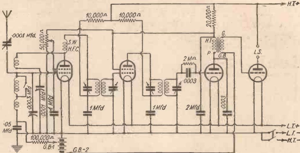
Fig. 3.—Circuit diagram of a short-wave superhet.
