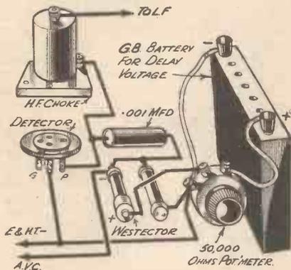
Fig. 2.—This skeleton pictorial circuit shows how the arrangement illustrated in Fig. 1 can be modified to provide delayed A.V.C.
