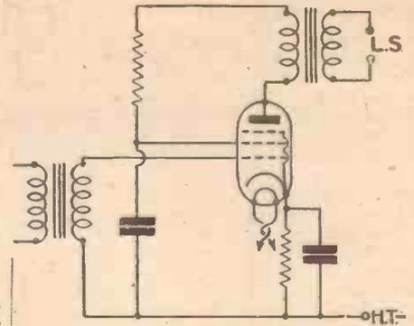
Fig. 2.—Using a mains-operated pentode valve for Class "A" output.
