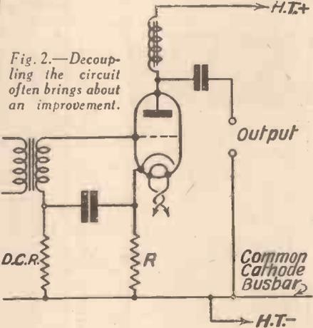
Fig. 2.—Decoupling the circuit often brings about an improvement.
