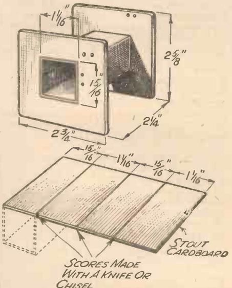
Fig. 3.—Details of the transformer winding spool are given in these sketches.
