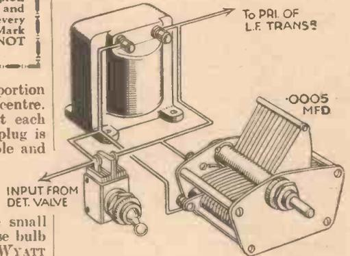
Using a choke and a variable condenser as a tone control unit.
