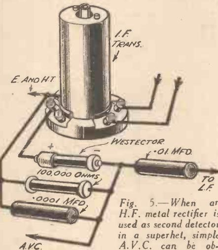
Fig. 5.—When an H.F. metal rectifier is used as second detector in a superhet, simple A.V.C. can be obtained by taking a lead from the negative end to the grid circuits of the V.M. valves.
