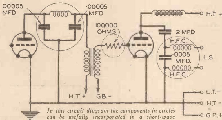
In this circuit diagram the components in circles can be usefully incorporated in a short-wave receiver for improving quality of reproduction.
