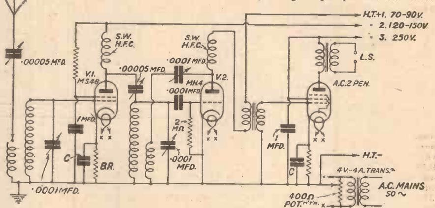
Fig. 2.—Theoretical diagram of a three-valve A.C. short-waver.
