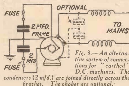
Fig. 3.—An alternative system of connections for "earthed" D.C. machines. The condensers (2 mfd.) are joined directly across the brushes. The chokes are optional.
