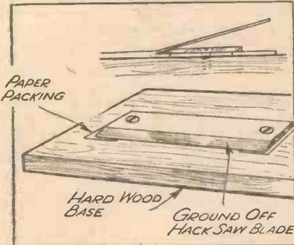
A simple method of splitting mica sheets.
