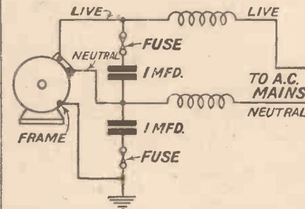
Fig. 2.—Stationary fractional-H.P. universal or A.C. motors operating on A.C. are best silenced as shown, the condensers being 1 mfd. each. Chokes need only be added in difficult cases. The wiring of the condensers depicted is recommended where the brushes are inaccessible. Note that the mains plug must not be reversible.
