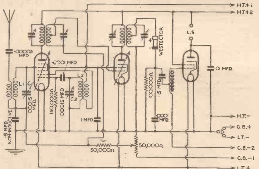
Fig. 1.—A modified circuit diagram of the £5 Superhet Three referred to in the text.
