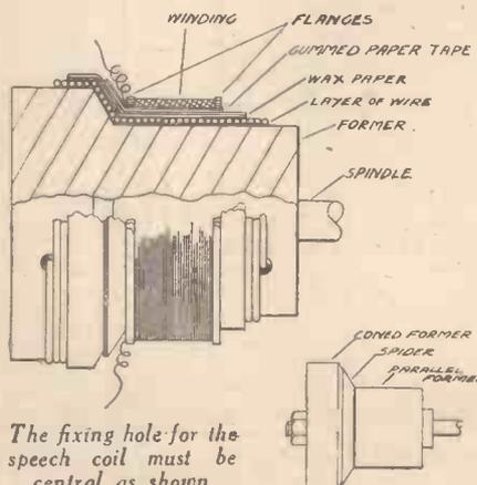
coil can be left for a few hours to dry, after which the binder is removed. Then prepare some very narrow strips of paper, and gum these on the former to form a ridge of the required height.
