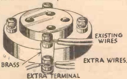
An easily-made wire-connecting link.
