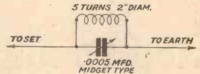
Fig. 3.—A filter for preventing induced hum.
