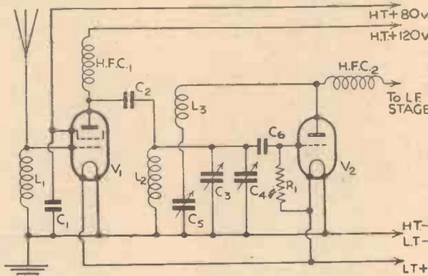
Fig. 1.—Circuit diagram of an untuned H.F. amplifier.
