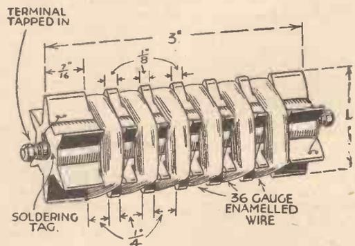
Fig. 3.—Winding data for the choke are given in this drawing.
