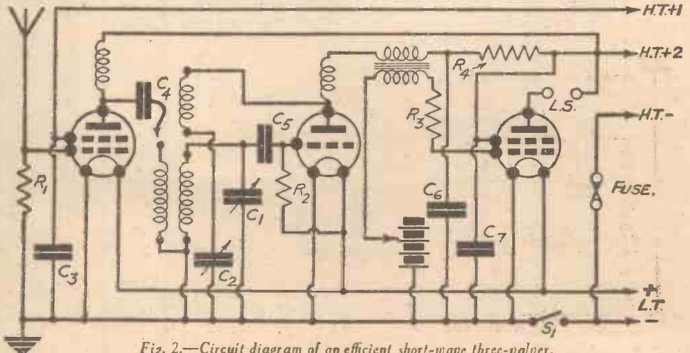
Fig. 2.—Circuit diagram of an efficient short-wave three-valver.
