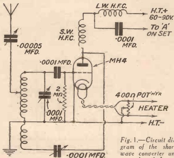
Fig. 1.—Circuit diagram of the short-wave converter unit described.
