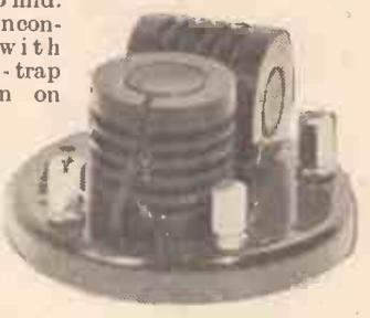
Showing the new Wearite wave-trap coil.
