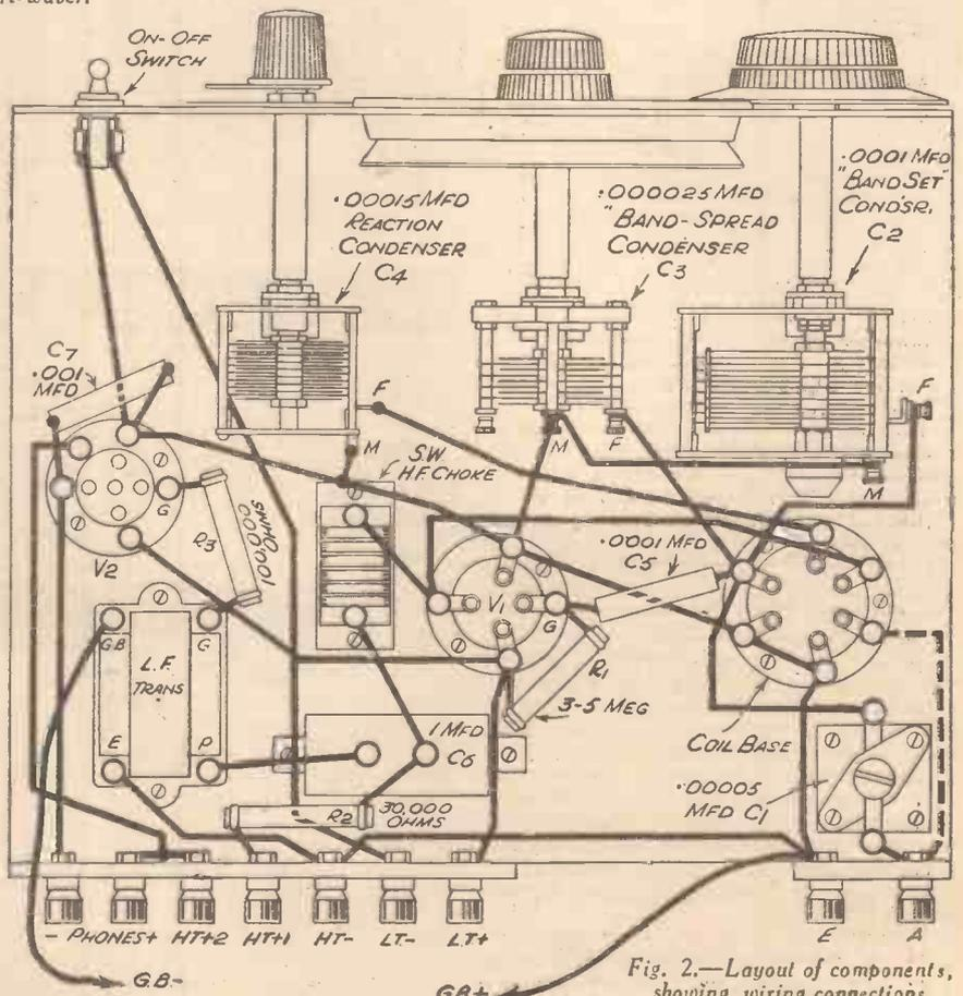
Fig. 2.—Layout of components, showing wiring connections.
