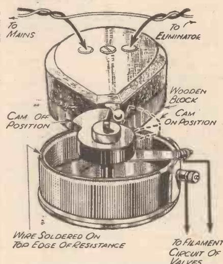
A useful combined filament and eliminator switch.
