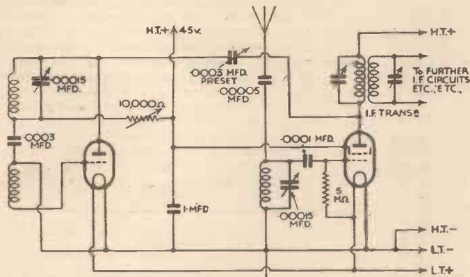
Fig. 2.—A circuit including an S.G. first detector and a separate oscillator.
