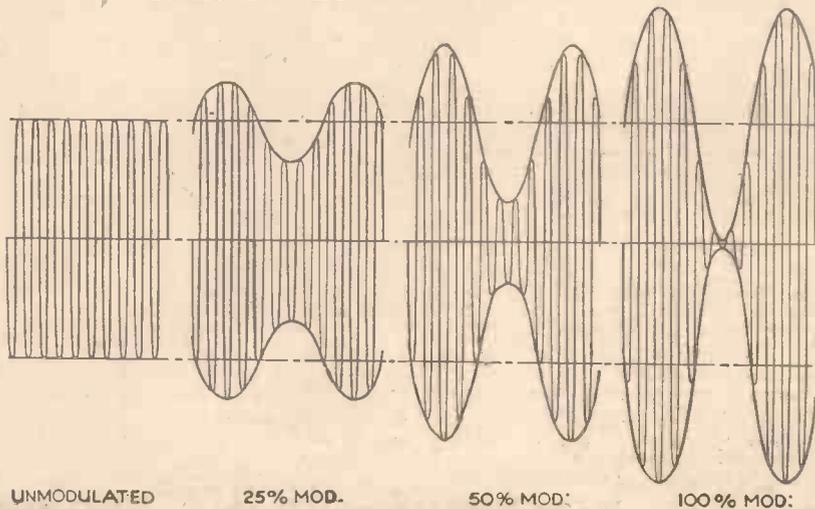
Fig. 2.—Different degrees of modulation.
