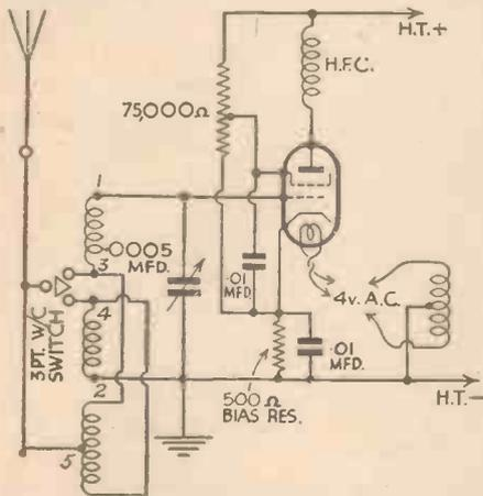
Fig. 5.—The altered connections in the cathode circuit of the H.F. valve are shown here.
