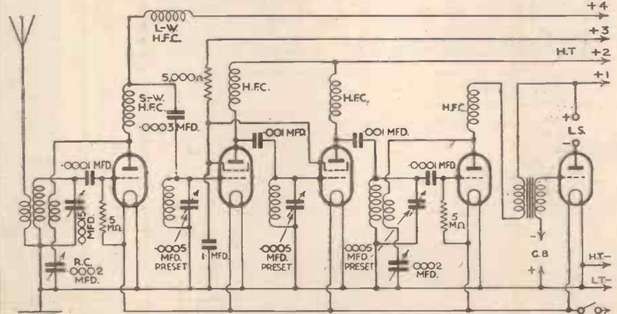
Fig. 4.—A circuit showing a triode used as first detector and oscillator.
