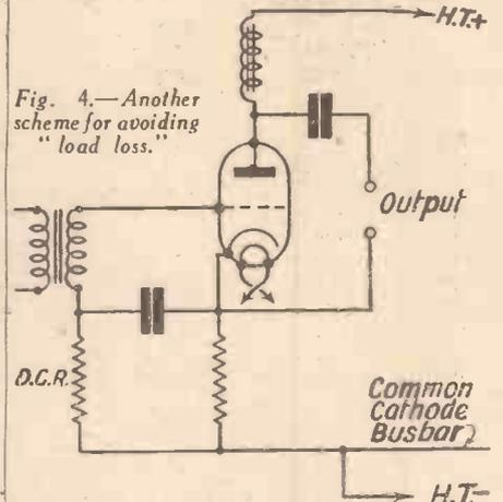
Fig. 4.—Another scheme for avoiding "load loss."
