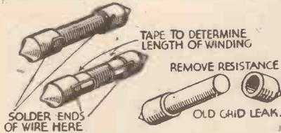
A simple method of making short-wave chokes.
