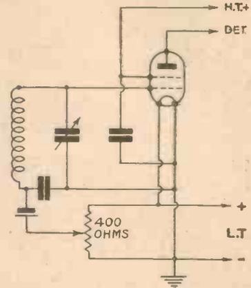
Using a variable resistance for obtaining accurate grid bias.
