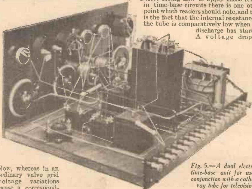
Fig. 5.—A dual electrical time-base unit for use in conjunction with a cathode-ray tube for television.
