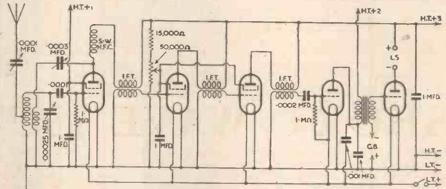
Fig. 3.—A circuit showing an S.G. valve used as first detector and oscillator.
