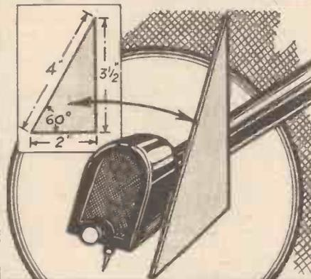
Pick-ups Should Be Set At An Angle Of 60°. A Cardboard Set Square Made To The Dimensions Shown Above Will Be Found Useful For Checking Up This Angle.
