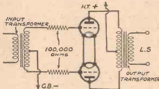
Fig. 1.—A standard push-pull circuit.
