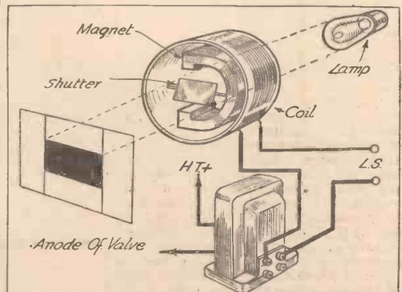
Fig. 5.—A visual tuning indicator in which a shutter is used to vary a band of light for giving the desired indication.
