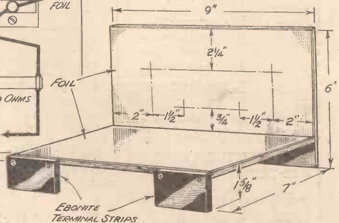
Fig. 2.—Rear view of the panel and baseboard, showing the terminal strips.
