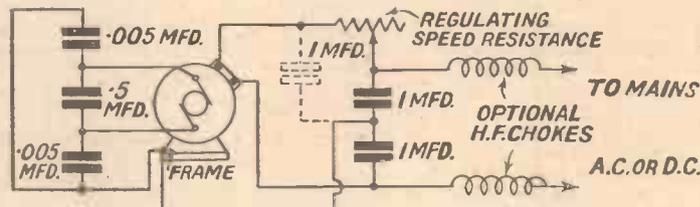
Fig. 7.—Where a sewing-machine motor or fan is fitted with a speed regulator, the additional suppressing devices shown are usually necessary. The metal frames of both motor and regulator should be connected together (not shown), if not already contacted.
