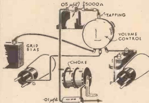
Fig. 2.—The circuit shown pictorially.
