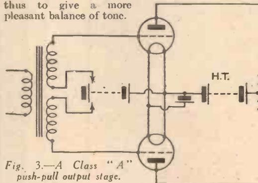
Fig. 3.—A Class "A" push-pull output stage.
