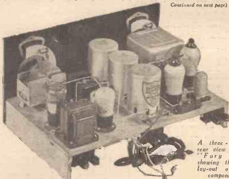
A three-quarter rear view of the "Fury Four," showing the neat lay-out of the components.
