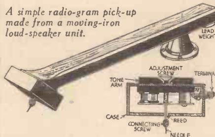
mounted at an angle of 60 degrees, and the two leads connected to the set as usual.—M. PULVER (Luton).
