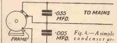
Fig. 4.—A simple condenser arrangement for gramophone motors (D.C. and universal), hair dryers, toy motors, small fans, and similar devices. The system is applicable to commutator motors on both A.C. and D.C. supplies. Earthing the motor frame can be tried, but is not always essential.
