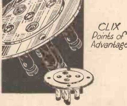
Clix obtain maximum insulation by mounting only the heads of valve sockets in thin paxolin, providing true low-loss construction, with resultant gain in efficiency. Although thin, the insulation is very strong, and will not chip or fracture with careless treatment.
