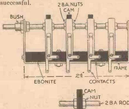
An efficient rotary switch for pick-up, wave-changing, and other purposes.
