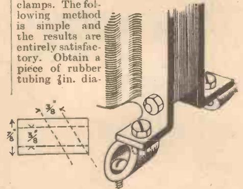
Mounting a mains transformer on pieces of stout rubber tubing to eliminate noise.
