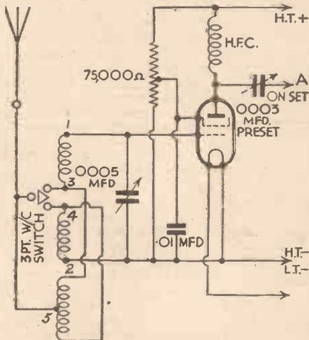
Fig. 1.—The circuit of the H.F. amplifier unit for which constructional details are given.
