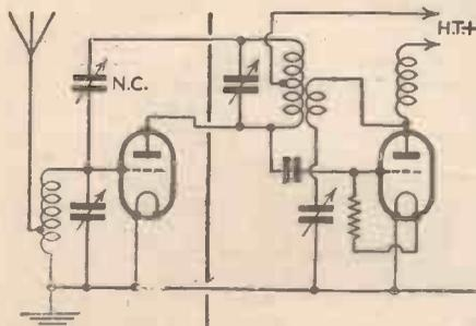
Fig. 3.—A neutralised triode circuit, with centre-tapped tuned anode.
