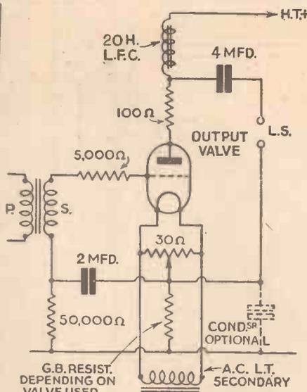
Fig. 4.—A method of removing hum in the output L.F. stage employing a directly-heated power valve. The 30-ohm potentiometer is suitable for 4- and 6-volt valves. Note the A.C.-L.T. centre tap is not required. Fit the potentiometer close to the valve-holder for best results.
