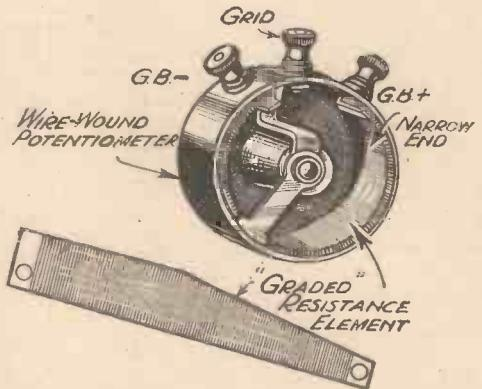
Fig. 3.—Showing the usual form of construction of a "graded" potentiometer.
