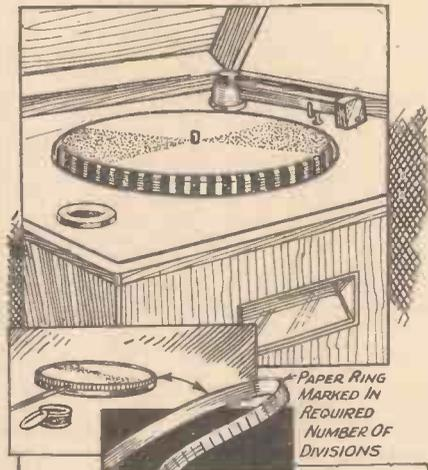
THE EDGE OF A GRAMOPHONE TURNTABLE IF DIVIDED IN ALTERNATE BLACK & WHITE SECTIONS, AS SHOWN ABOVE, FORMS A PERMANENT STROBOSCOPE.
