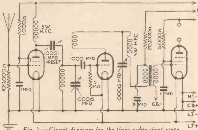
Fig. 1.—Circuit diagram for the three-valve short-wave portable described.
