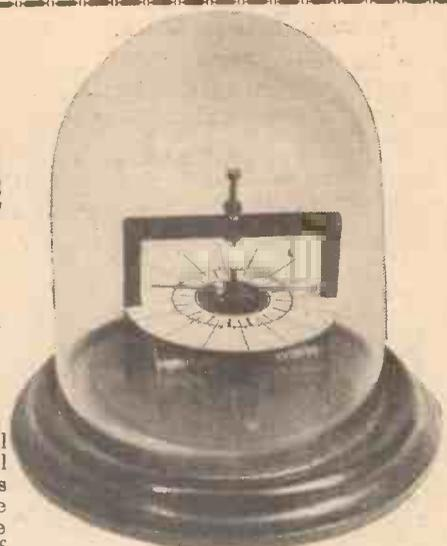
The finished galvanometer.
