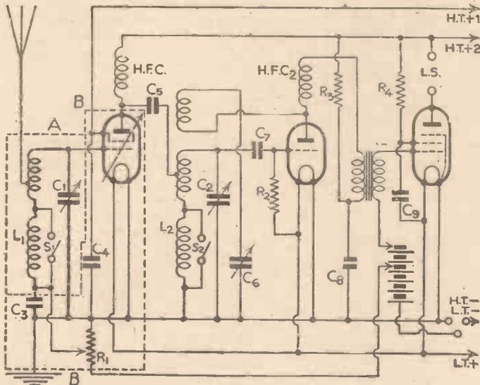
Fig. 1.—The complete three-valve circuit considered in this series of articles, the components described this week being enclosed in the box marked B.
