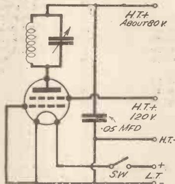
Fig. 1.—The "Autodyne" circuit.
