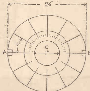
Fig. 9.—How to mark out the scale.
