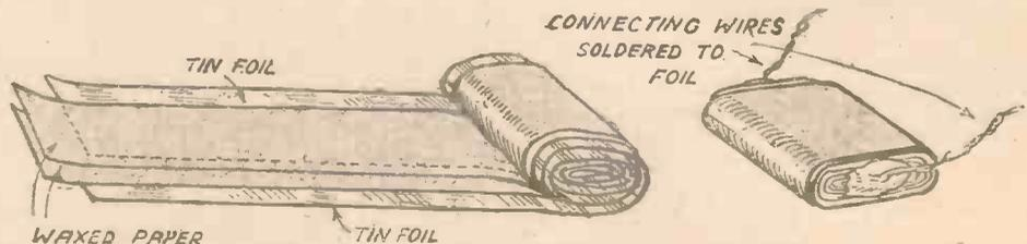
Fig. 2.—The above illustrations show the different forms of construction used for ordinary and non-inductive fixed condensers. The differences and reasons for the choice of non-inductive for certain positions in the circuit are fully explained in the text.
