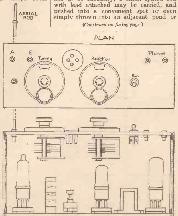
Fig. 2.—The panel and chassis layouts.
