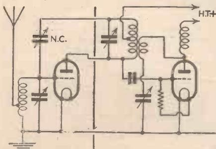
Fig. 3.—A neutralised triode circuit, with centre-tapped tuned anode.
