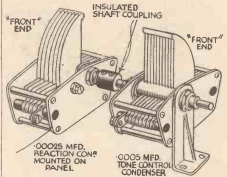
Fig. 7.—Ganging two condensers for use in the circuit given in the first column.
