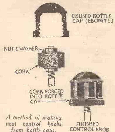
A method of making neat control knobs from bottle caps.
