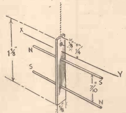
Fig. 10.—Simple suspension frame for the needles and pointer.
