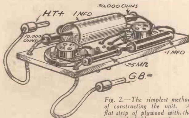
Fig. 2.—The simplest method of constructing the unit. A flat strip of plywood with the two valveholders, resistances, and condensers firmly mounted on the top and the plug screwed to the underside.
