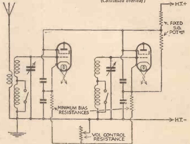
Fig. 3.—A system of variable-mu volume control frequently used in 2 H.F. or superhet. mains receivers. It often proves inferior to the circuit arrangement shown in Fig. 4. Component values are not shown, since they depend entirely upon the particular valves employed.
