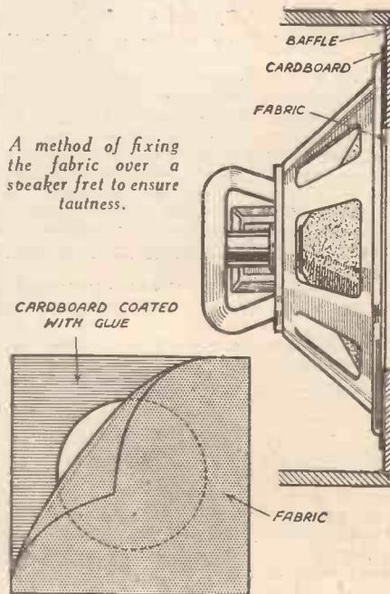
A method of fixing the fabric over a speaker fret to ensure tautness.
