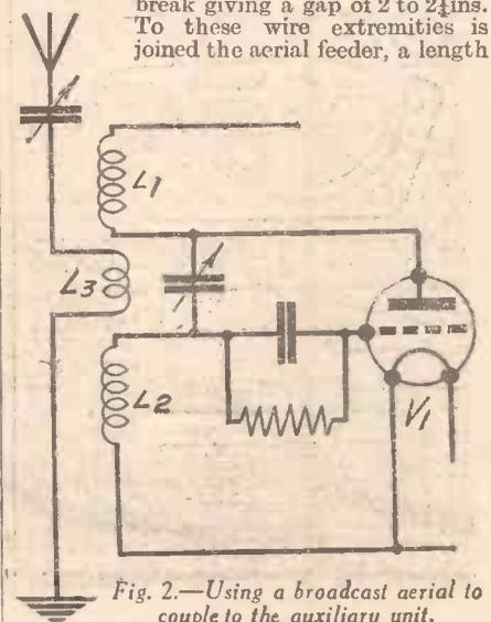
Fig. 2.—Using a broadcast aerial to couple to the auxiliary unit.
