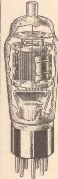
Showing the electrode construction of the Mullard octode frequency changer, which is a battery-operated valve.
