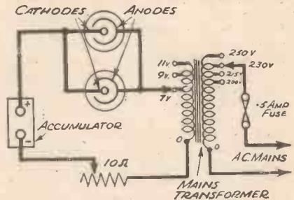
Fig. 3.—The circuit for the A.C. charger described, and which uses two chemical rectifiers wired in parallel.
