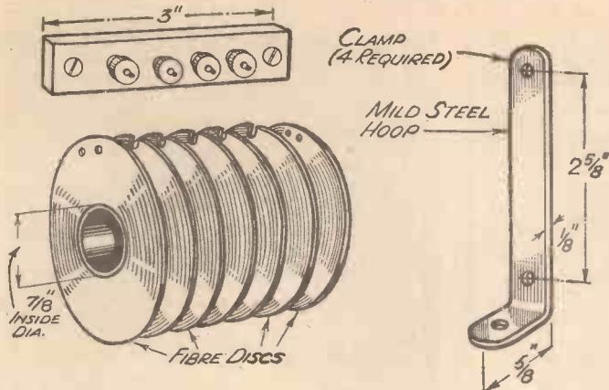
Fig. 3.—Details of the winding spool.
