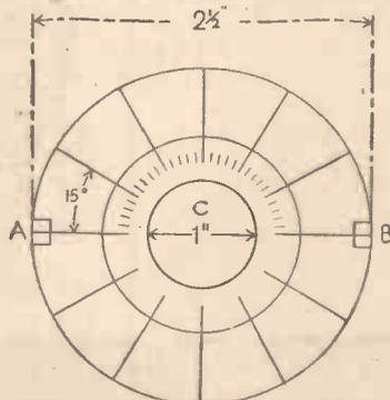
Fig. 9.—How to mark out the scale.
