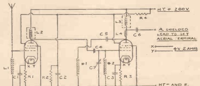
The new Mervyn 3-range short-wave coil unit, and a theoretical circuit of a short-wave converter incorporating the unit.
