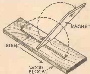
Fig. 6.—The single-stroke method of magnetising a steel needle.
