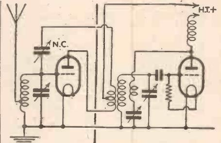
Fig. 4.—A modification of Fig. 3—using a tapped H.F. transformer.
