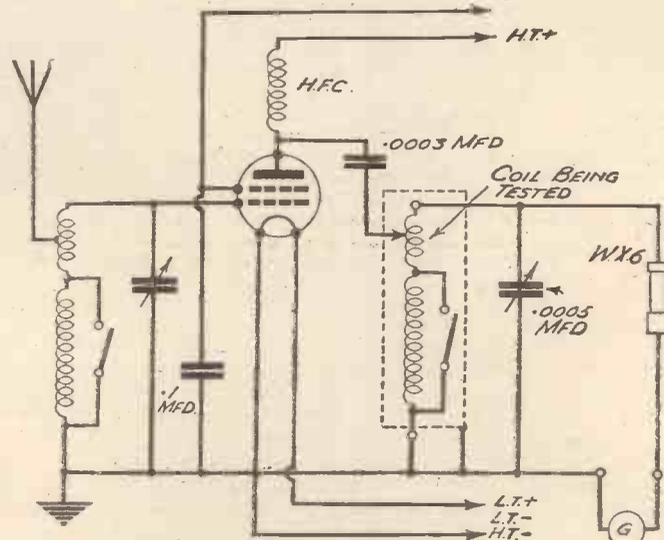
Fig. 2.—When the receiving aerial is more than ten miles or so from the transmitter it may be necessary to precede the test circuit by an H.F. stage as shown.
