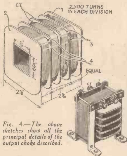
Fig. 4.—The above sketches show all the principal details of the output choke described.
