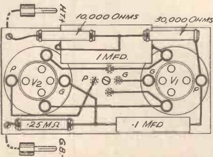
Fig. 4.—Wiring plan using the flat construction. This may, of course, be modified to suit the particular construction which is adopted.
