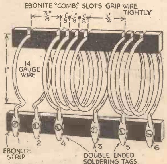
Fig. 2.—Showing a convenient and simple method of making an under 5-metre tuner.
