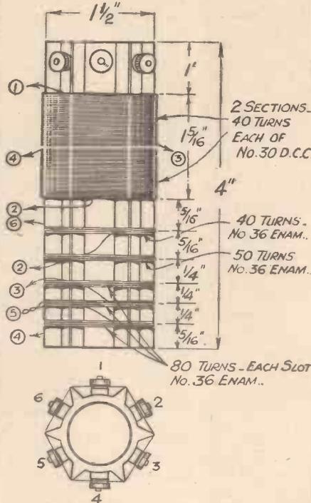
Fig. 1.—Details of the tuning coil.
