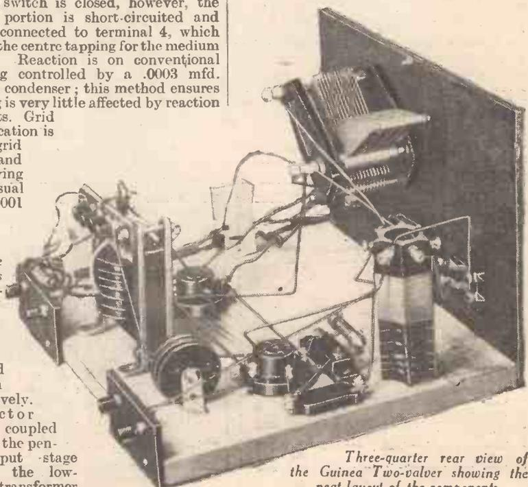
Three-quarter rear view of the Guinea Two-valver showing the neat layout of the components.
