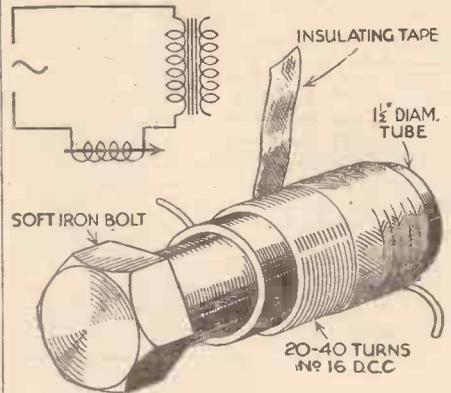
An easily-made voltage regulator for A.C. mains.
