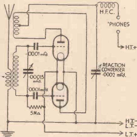
Fig. 1.—The push-pull detector circuit described.
