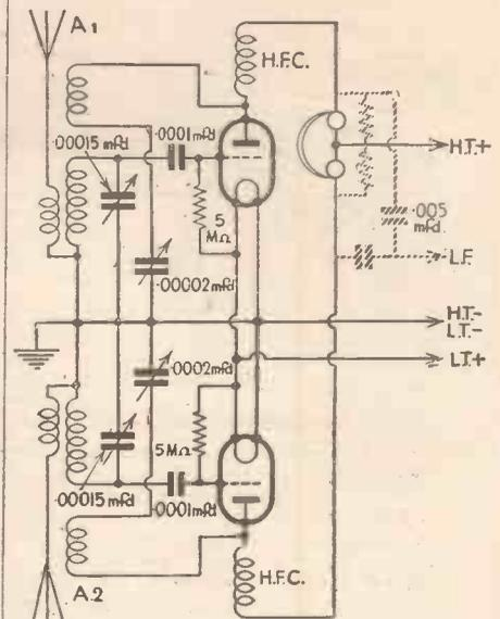
Fig. 4.—A double detector circuit which is suggested for experimental purposes. Both detectors are individually tuned and have their own aerials.
