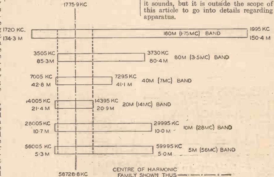
Showing frequency relation of amateur bands, and frequency-wavelength limits. Frequencies in harmonic relation are shown between outer dotted lines, the centre dotted line indicating the centre of harmonic family.
