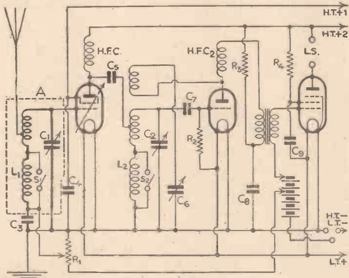
Fig. 1.—The circuit taken as an example. Instead of assigning values to the components, these are indicated by letter references.
