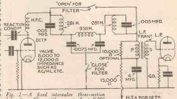
Fig. 2.—A fixed interval three-section heterodyne filter with a cut-off at 9,000 cycles. The two switches can be linked together to operate as denoted, so that for transmissions free of sideband interference the full frequency response of the set may be utilised.
