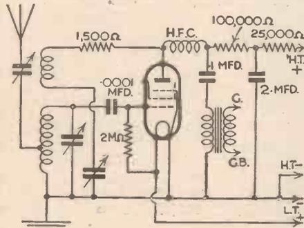
Fig. 2.—An H.F. pentode as detector.
