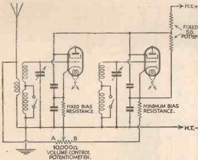
Fig. 4.—Another system of volume control which has many important advantages.
