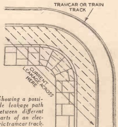
Showing a possible leakage path between different parts of an electric tramcar track.
