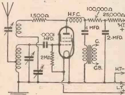
Fig. 2.—An H.F. pentode as detector.
