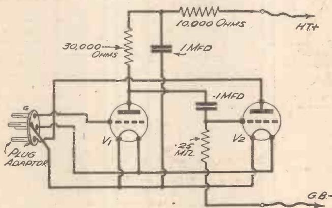
Fig. 1.—Theoretical circuit of the Plus-1 unit.
