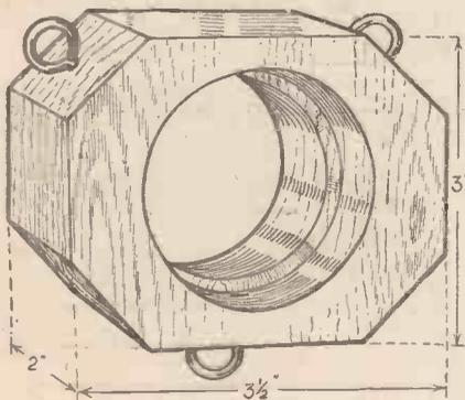
Fig. 1.—How the wooden block is shaped to form the microphone case.
