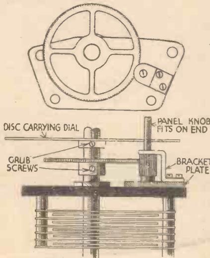
A slow-motion drive made with old gramophone motor gear wheels.
