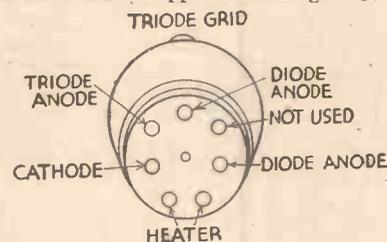
Fig. 2.—The valve base connections for the double-diode triode.
