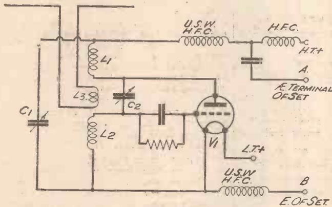
Fig. 1.—The circuit for a suitable ultra-short-wave converter.
