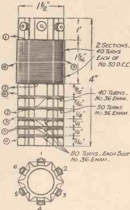
Fig. 1.—Details of the tuning coil.
