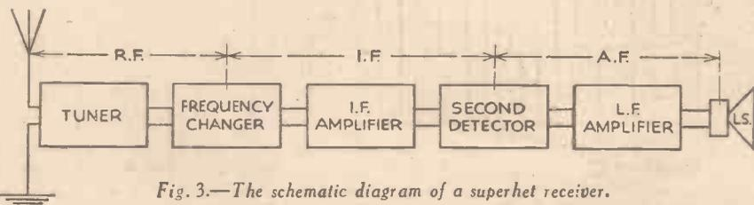
Fig. 3.—The schematic diagram of a superhet receiver.
