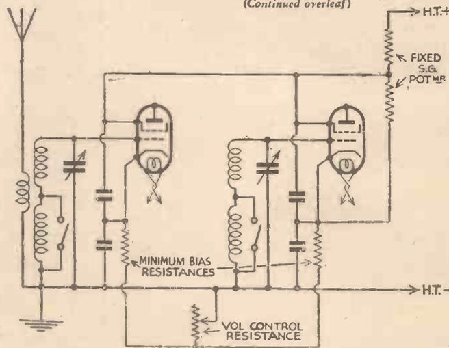
Fig. 3.—A system of variable-mu volume control frequently used in 2 H.F. or superhet. mains receivers. It often proves inferior to the circuit arrangement shown in Fig. 4. Component values are not shown, since they depend entirely upon the particular valves employed.
