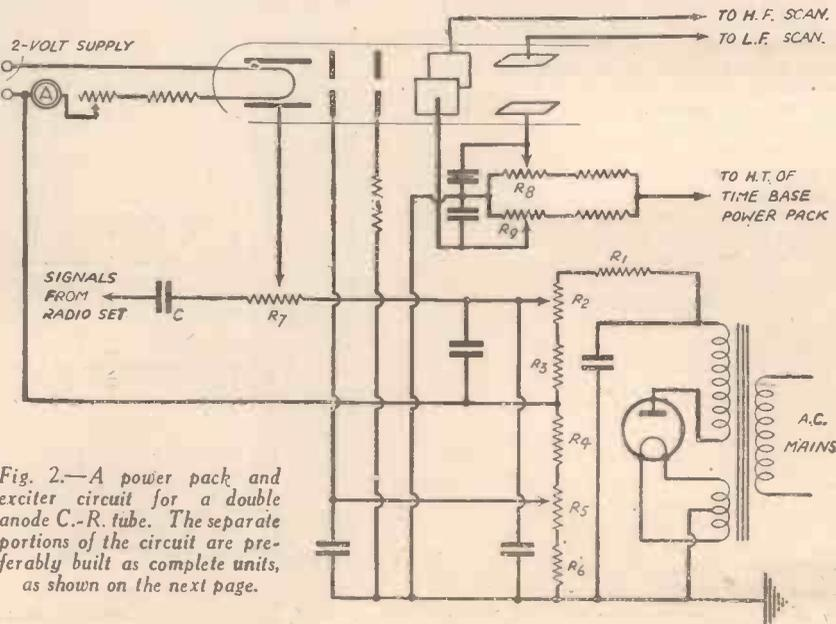
Fig. 2.—A power pack and exciter circuit for a double anode C.-R. tube. The separate portions of the circuit are preferably built as complete units, as shown on the next page.
