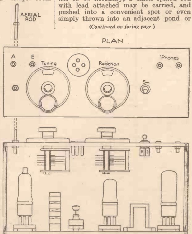
Fig. 2.—The panel and chassis layouts.
