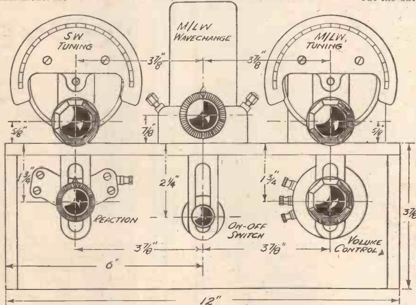
Drill the panel to the dimensions given here.
