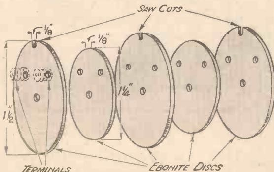
Fig. 2.—Constructional details of the high-frequency choke.
