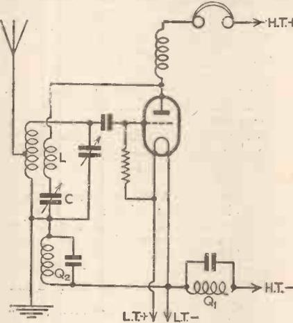
Fig. 5.—The basic circuit of a super-regenerative receiver.
