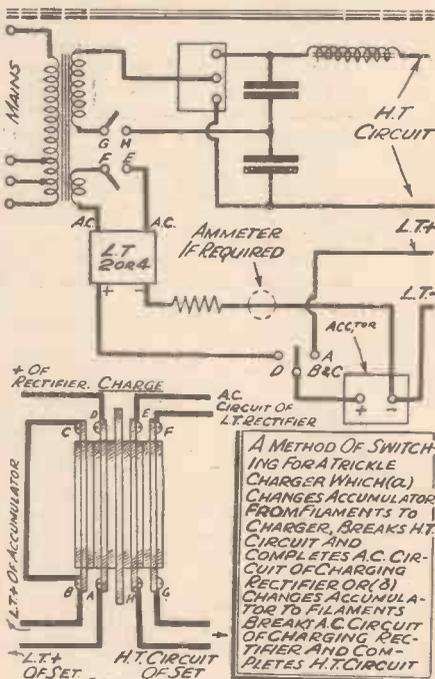
A METHOD OF SWITCHING FOR A TRICKLE CHARGER WHICH (1) CHANGES ACCUMULATOR FROM FILAMENTS TO CHARGER, BREAKS H.T. CIRCUIT AND COMPLETES A.C. CIRCUIT OF CHARGING RECTIFIER OR (2) CHANGES ACCUMULATOR TO FILAMENTS BREAKS A.C. CIRCUIT OF CHARGING RECTIFIER AND COMPLETES H.T. CIRCUIT
