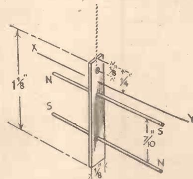
Fig. 10.—Simple suspension frame for the needles and pointer.
