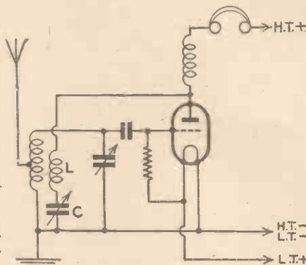
Fig. 1.—A simple one-valve detector circuit with reaction to illustrate the principles.
