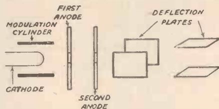
Fig. 1.—Adding a second accelerator anode to cathode-ray tubes for television reception.
