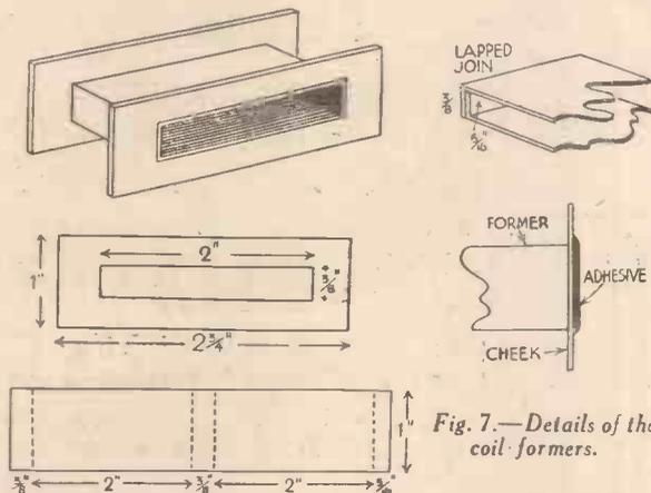
Fig. 7.—Details of the coil formers.
