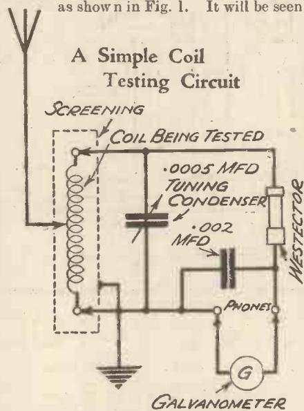
Fig. 1.—The simple test circuit described, in which an H.F. metal rectifier and galvanometer are connected to the coils to be compared.
