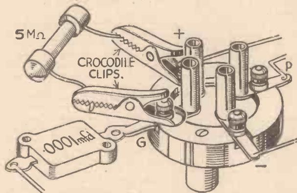
Fig. 1.—A simple scheme for adjusting the detector circuit.
