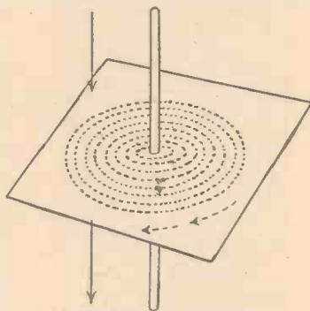
Fig. 2.—Illustrating the lines of force round a current-carrying conductor.
