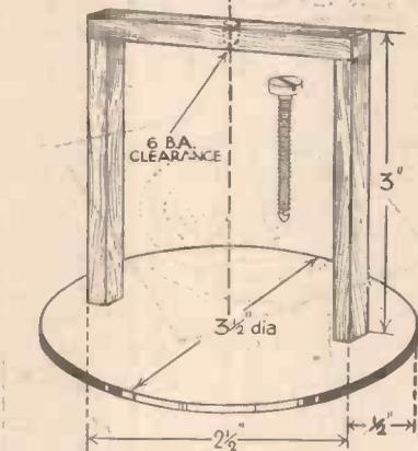
Fig. 8.—The galvanometer bridge and base.
