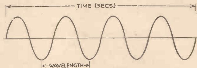
Fig. 2.—A diagram which shows the relationship between wavelength and frequency. Frequency is the number of waves per second.
