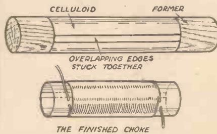
A neat method of making formers for chokes or other small coils.
