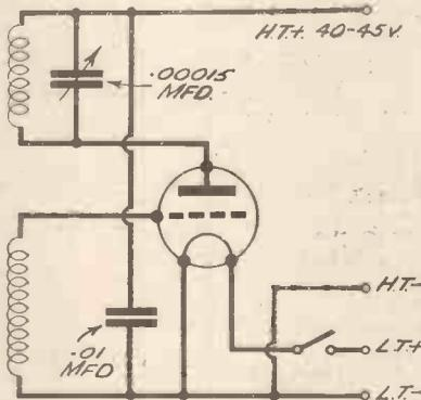
Fig. 2.—An alternative tuned-anode circuit.
