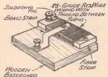
Fig. 4.—This illustration shows the constructional details of the 10 ohm variable resistance described.
