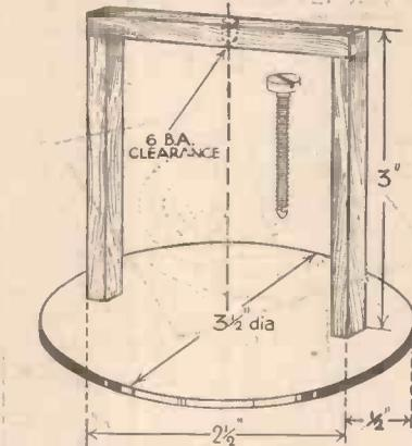
Fig. 8.—The galvanometer bridge and base.
