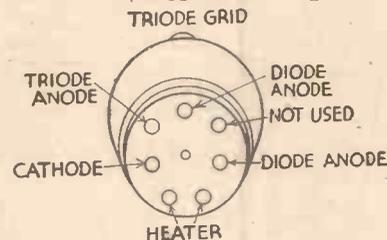
Fig. 2.—The valve base connections for the double-diode triode.
