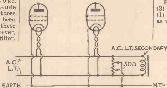
Fig. 5.—Connections of heater potentiometer for indirectly-heated A.C. valves. There is not usually a critical nodal point, but the potentiometer will often prove preferable to taking the usual centre tap on the A.C.-L.T. winding to the earth lead.
