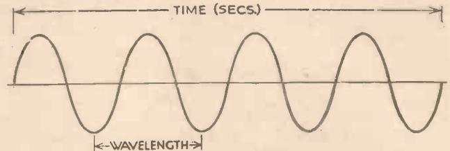
Fig. 2.—A diagram which shows the relationship between wavelength and frequency. Frequency is the number of waves per second.
