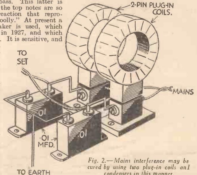
Fig. 2.—Mains interference may be cured by using two plug-in coils and condensers in this manner.
