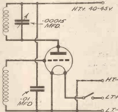
Fig. 2.—An alternative tuned-anode circuit.
