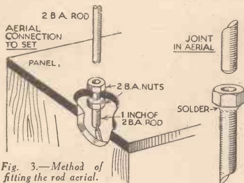
Fig. 3.—Method of fitting the rod aerial.
