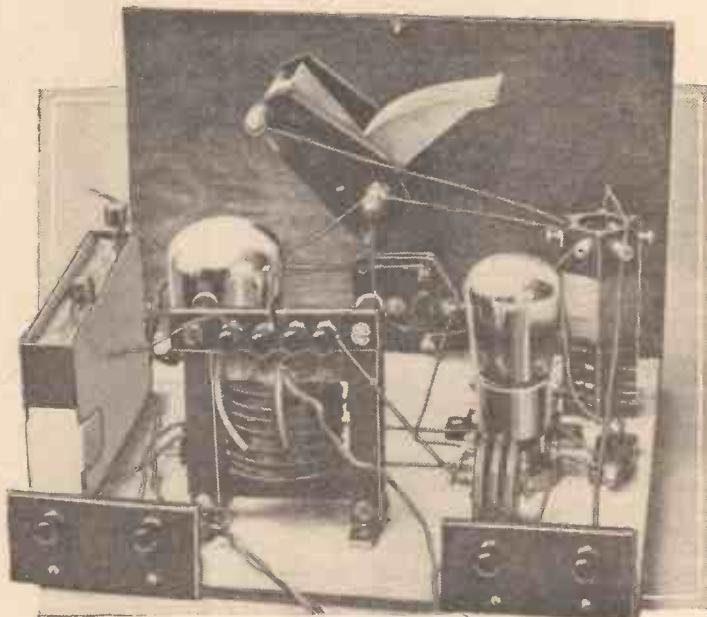
Fig. 7.—Rear view of the receiver showing the lay-out of the components.
