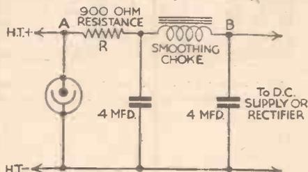
Fig. 5.—Showing how a neon stabiliser should be connected. Note the extra resistance used to bring the total value between the rectifier and H.T.+ lead up to 1,800 ohms.
