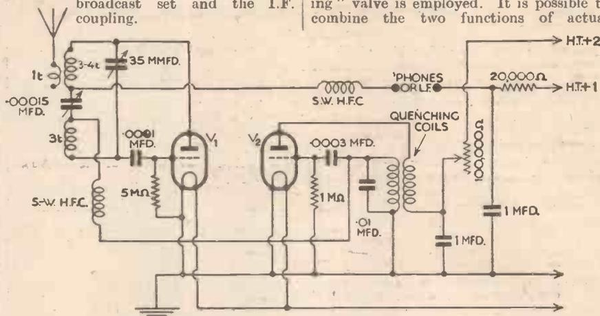
Fig. 3.—The circuit for a two-valve regenerative receiver which has particular advantages for ultra-short-wave reception.
