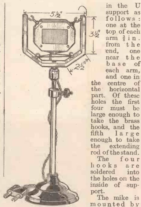
Fig. 2.—The finished microphone and stand.
