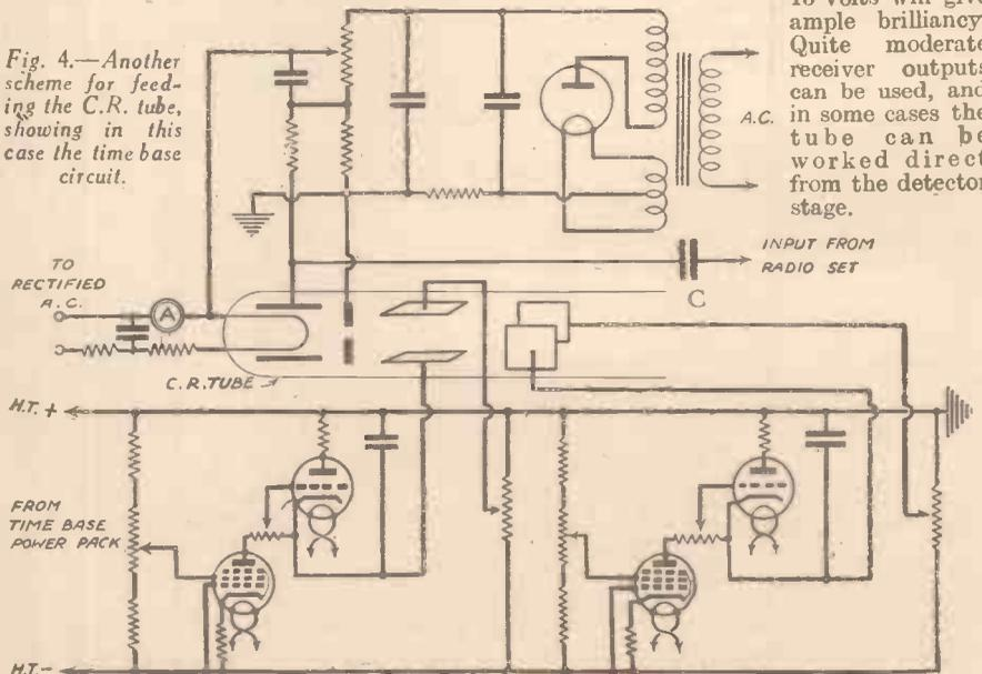
secondary of a transformer through the primary of which this current is caused to pass. By applying this kick voltage with suitable polarity to the modulation cylinder of the cathode-ray tube, a momentary static field is produced which will completely cut off the electron beam and so render the return stroke invisible.
