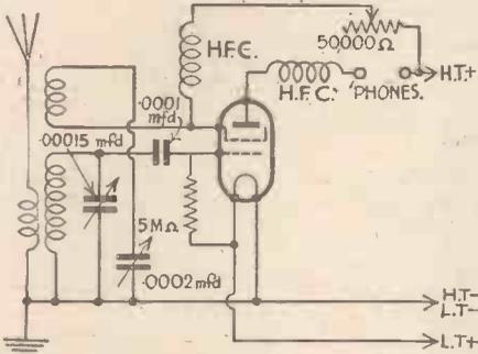
Fig. 3.—A modified arrangement of the circuit shown in Fig. 2, but using an S.G. valve for detection and reaction control.
