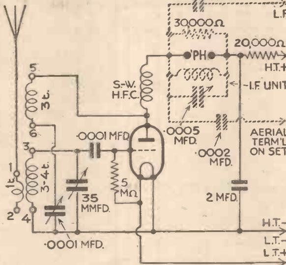
Fig. 1.—The circuit of an ultra-short-wave unit which may be used either as a simple one-valve receiver by connecting the 'phones to the terminals indicated, as a converter by using the connections shown below the 'phone terminals, or in conjunction with an L.F. amplifier by using the connections shown above those terminals.
