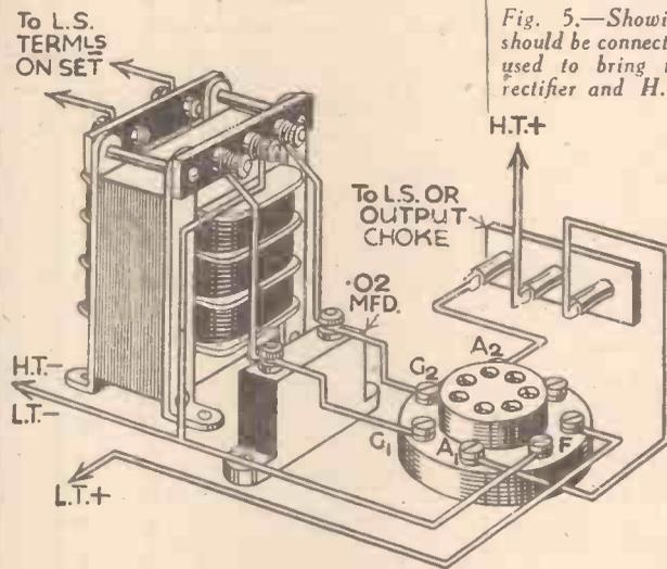
Fig. 3.—A practical wiring plan of the amplifier. The arrangement is the same as that shown in the theoretical in Fig. 1.
