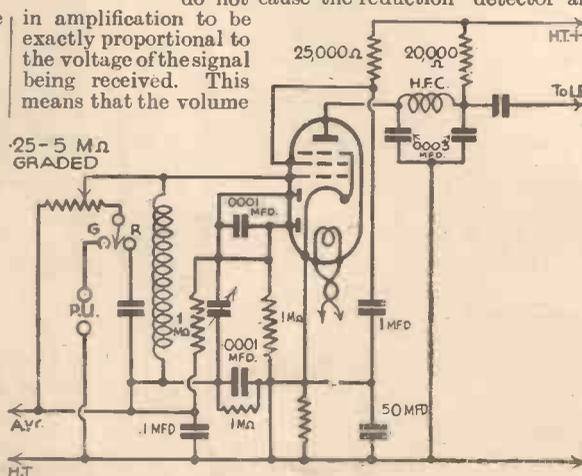
Fig. 3.—A typical circuit for corrected A.V.C., using the Cossor double-diode pentode, type D.D./Pen.
