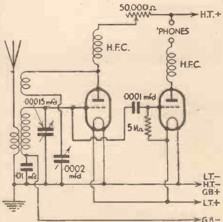
Fig. 2.—A detector circuit in which an additional valve (the first) is used for reaction control.
