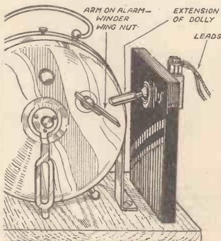
A simple but reliable time switch for use with either a battery or mains receiver.
