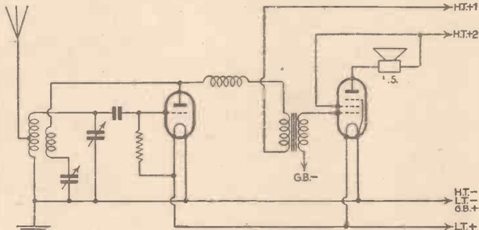
Fig. 2.—Adding a stage of L.F. amplification to the circuit shown in Fig. 1 to increase signal output.
