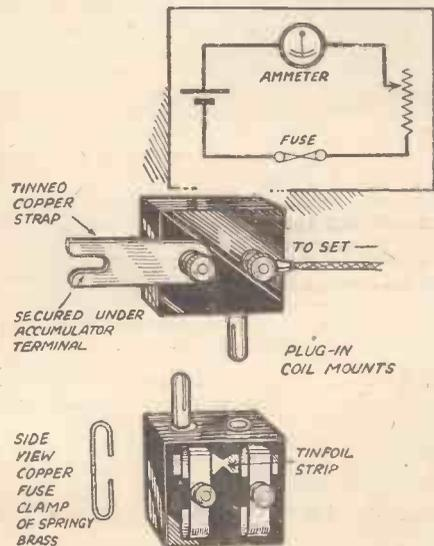
A plug-in fuse using a strip of tinfoil.
