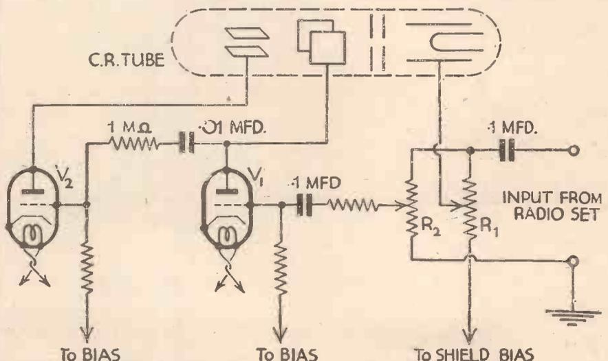
Fig. 1.—One arrangement for linking the signals from the radio receiver to the C.-R. tube.
