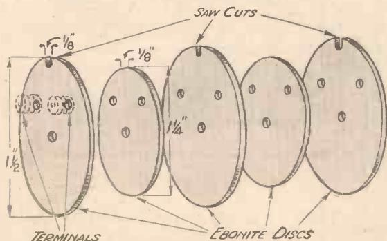
Fig. 2.—Constructional details of the high-frequency choke.
