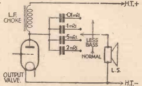
Fig. 3.—Varying the tone by means of a condenser circuit.
