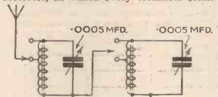
Fig. 1.—A double wave-trap or acceptor unit using iron-cored coils for reducing the overloading effects of the local stations on the first valve, and thereby avoiding cross-modulation or, in superhets, second-channel whistles. One coil unit (tuned to the long waves) will often prevent similar effects due to 5XX.
