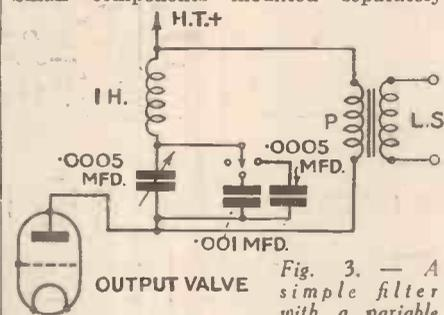
Fig. 3.—A simple filter with a variable response over quite a wide frequency range. The tuning condenser can be of the bakelite dielectric type, the other condensers being of fixed capacities. For commercial receivers the components can be mounted in a small box and then connected across the primary of the transformer fitted to the loudspeaker, as shown. It is also possible to join the filter across the primary of an L.F. transformer.
