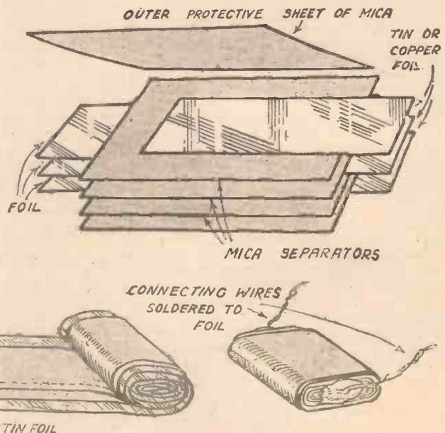
Fig. 2.—The above illustrations show the different forms of construction used for ordinary and non-inductive fixed condensers. The differences and reasons for the choice of non-inductive for certain positions in the circuit are fully explained in the text.
