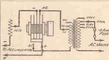
Fig. 5.—The circuit required when using the Westinghouse L.T.2 rectifier.
