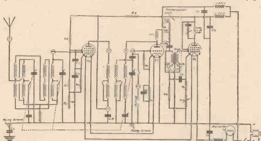
Fig. 1.—The circuit of a typical receiver where the band-pass filter precedes the first valve.
