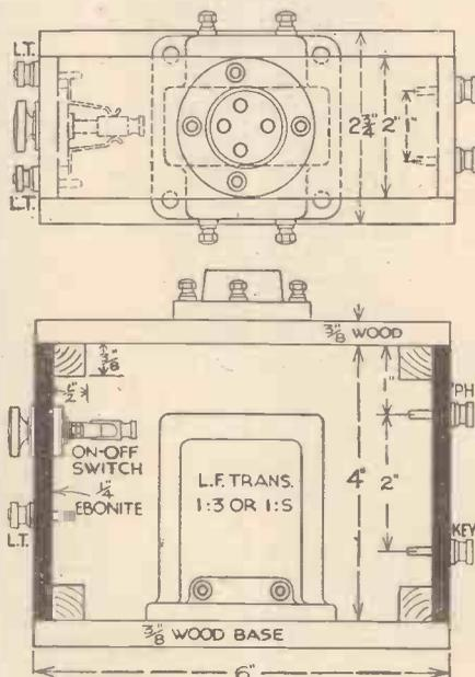
Figs. 1 and 2.—Plan and elevation of a morse code practice unit for giving noiseless signals.
