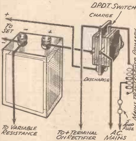
Fig. 6.—The switching system required when using an A.C. trickle charger.
