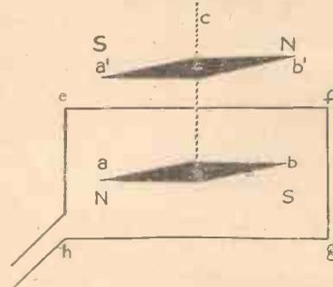
Fig. 5.—Two magnetic needles suspended with opposite poles adjacent, and known as the astatic system.
