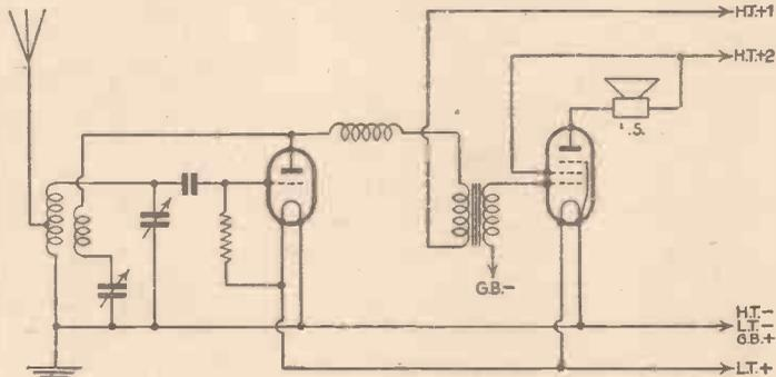
Fig. 2.—Adding a stage of L.F. amplification to the circuit shown in Fig. 1 to increase signal output.
