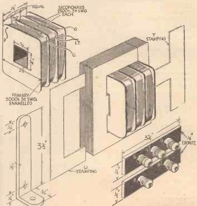
Fig. 2.—All the main details for constructing the driver transformer are given in the above sketches.
