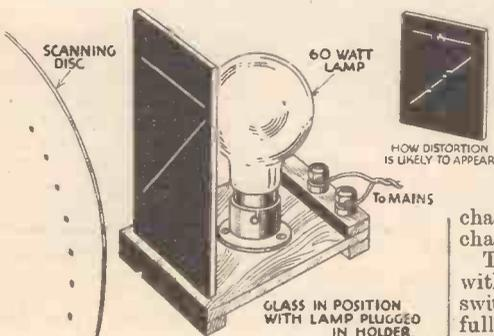
A useful dodge for testing the accuracy of the holes in a scanning disc:
