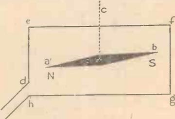
Fig. 4.—A magnetic needle suspended in a single coil of wire.
