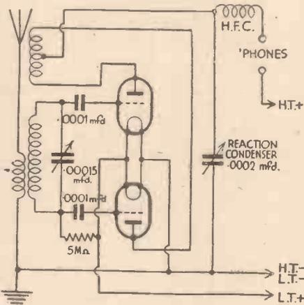
Fig. 1.—The push-pull detector circuit described.
