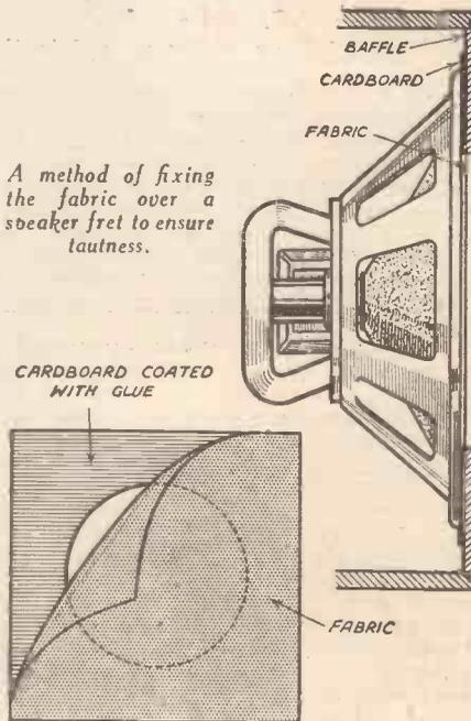
A method of fixing the fabric over a speaker fret to ensure tautness.
