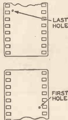
Fig. 4.—The two film ends showing the first and last scanning holes and the trimmed edges.
