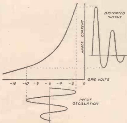
Fig. 1.—This diagram shows the effect of a weak signal, or a wrong type of valve used as an anode-bend rectifier.
