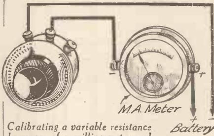
Calibrating a variable resistance by means of a milliammeter and battery.
