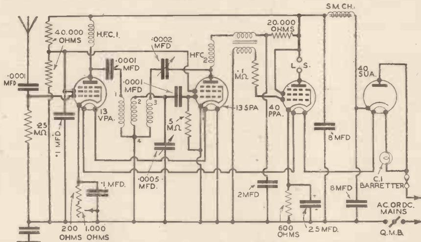
A universal mains 4-valve receiver. All valves are marked, and the valves specified are of Cossor make, whilst the barretter is a Philips type C.1. The layout should approximate to that of the component shown in the theoretical diagram.
