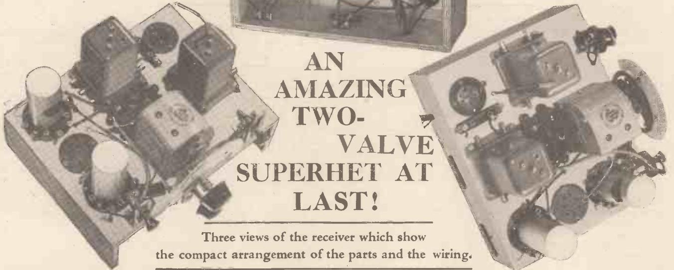
it should not be difficult to obtain a good performance within a very short space of time. Remember that any adjustment in one part of the scale should immediately be checked by turning to the opposite end of the scale in order to make certain that a balance is being maintained. If a loud signal is obtained, reduce volume by means of the volume control and work always throughout the trimming operations with the faintest signal which can be obtained.
