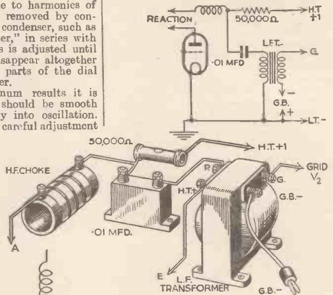
Fig. 2.—Parallel-feeding the L.F. transformer will often cure threshold howl.
