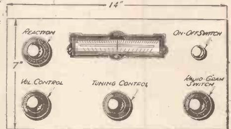
Fig. 3.—The panel dimensions and layout. Note the neat and orderly appearance of the controls.
