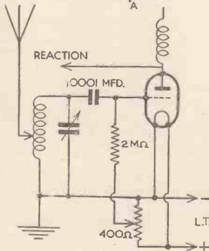
Fig. 3.—Making reaction control smooth by adjusting the bias for the detector valve.
