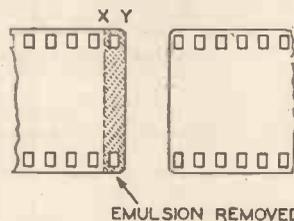
Fig. 5.—Preparing the film for jointing.
