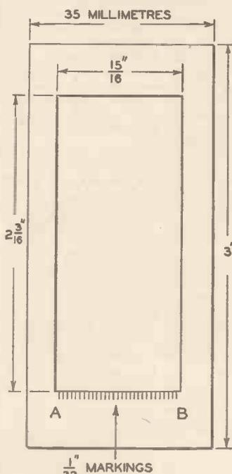
Fig. 2.—Details of the metal template.
