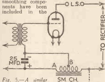
Fig. 5.—A similar arrangement to that shown in Fig. 4, but where the bias voltage is developed across only a portion of a tapped smoothing choke, between points A and B.
