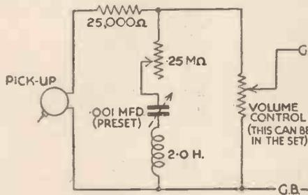
Fig. 1.—One method of controlling the output from the pick-up.
