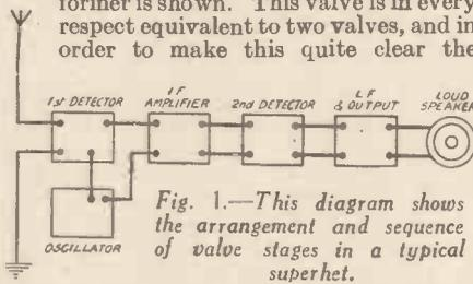
Fig. 1.—This diagram shows the arrangement and sequence of valve stages in a typical superhet.
