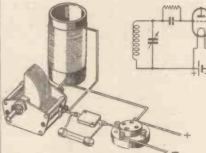
Fig. 1.—One method of giving the grid a positive bias.
