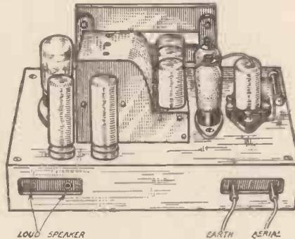
Fig. 1.—Although apparently arranged for appearance, there is a sound technical reason for the usual arrangement of the aerial, earth, and loud-speaker leads at opposite ends of a receiver.
