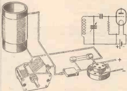
Fig. 2.—An alternative method of making the grid positive.
