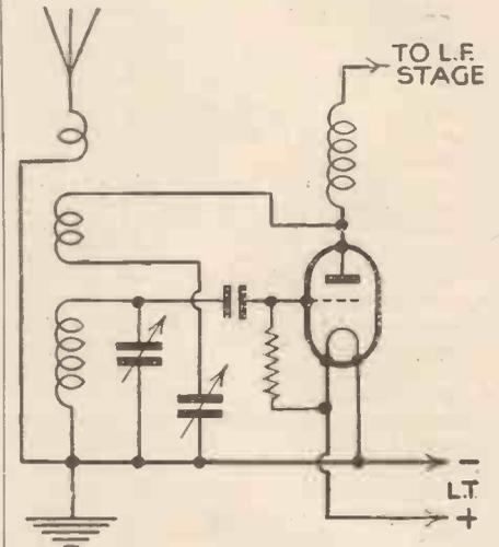
Fig. 2.—Improved reaction effects may be obtained by placing the reaction winding between the aerial and grid coils.
