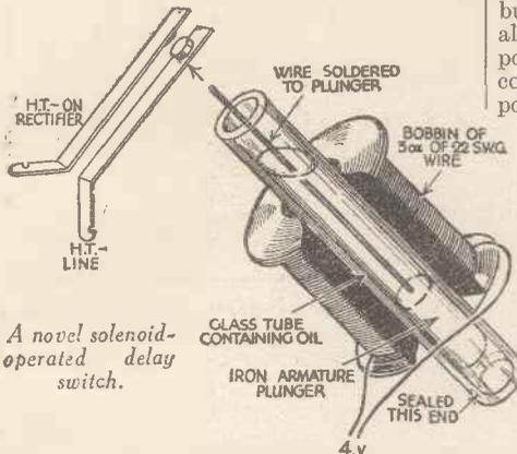
A novel solenoid-operated delay switch.
