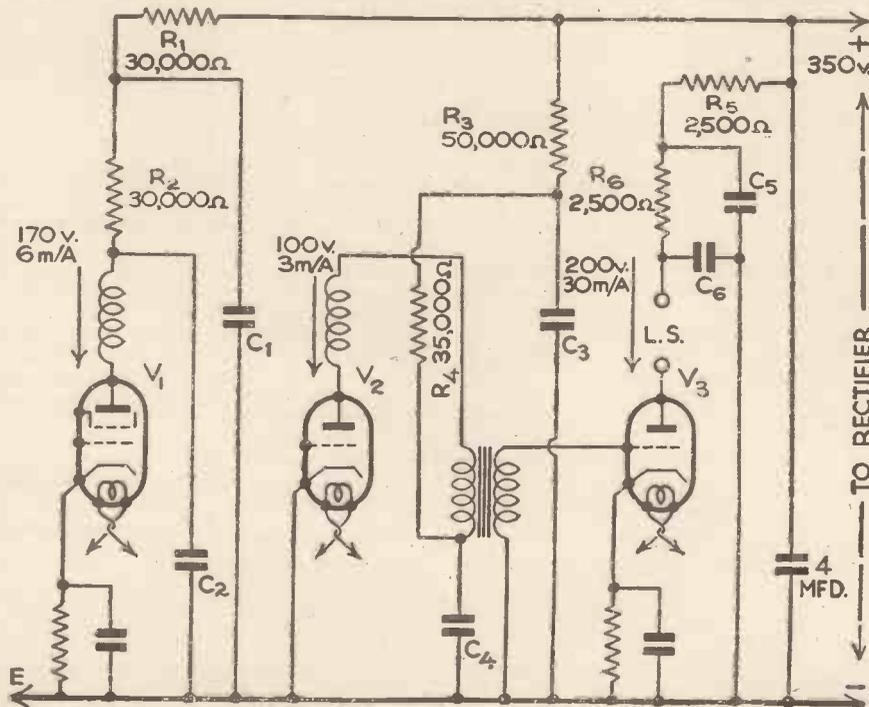
Fig. 3.—This skeleton circuit shows the method of smoothing the H.T. supply without the use of an L.F. choke. Resistances and condensers only are employed, and these serve also for decoupling. Condensers C1 to C6 may each have a capacity of 2 mfd.
