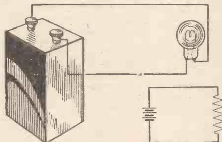
Fig. 1.—A direct current supply across a resistance.
