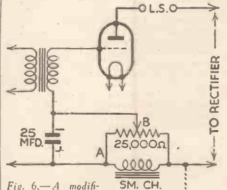
Fig. 6.—A modification of the circuit shown in Fig. 5. In this case the bias voltage is obtained from a potentiometer in parallel with the smoothing choke.
