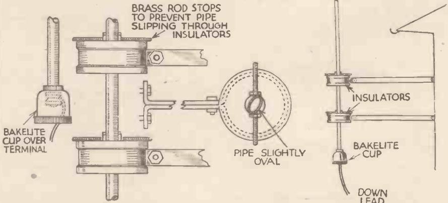
A vertical short-wave aerial system, using standard insulators and a length of copper tubing.
