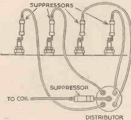
The method of fitting noise suppressors.
