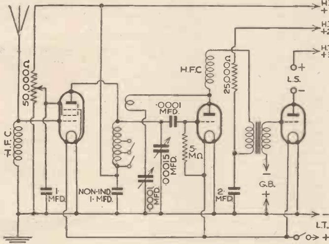
via a variable potentiometer. I have found that this assists to a great extent in obtaining the maximum sensitivity of the valve. In one of my sets the optimum position is quite critical, and enormously improved results are obtained by setting the potentiometer correctly. As readers
