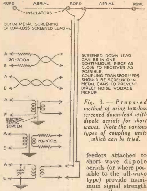
Fig. 3.—Proposed method of using low-loss screened downlead with dipole aeriels for short waves. Note the various types of coupling units which can be tried.
