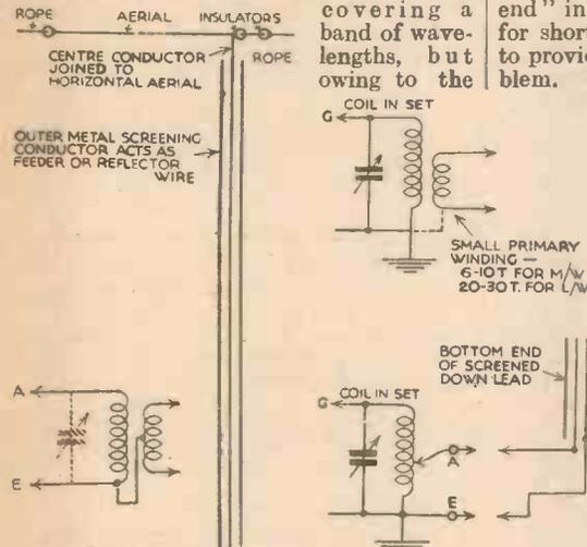
Fig. 1.—An inverted L aerial arranged for short waves as mentioned in the text. Further S.W. couplings, as shown in Fig. 3, can be tried.
