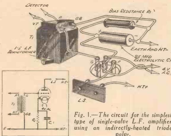
Fig. 1.—The circuit for the simplest type of single-valve L.F. amplifier using an indirectly-heated triode valve.
