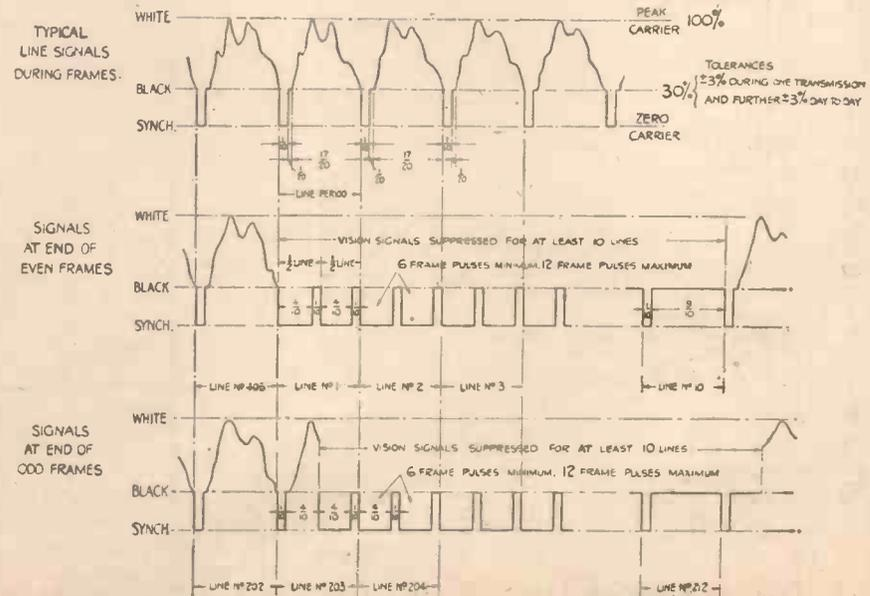
Fig. 2.—The transmitted wave-form of the Marconi-E.M.I. high-definition system.
