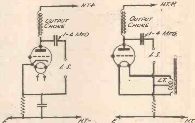
Fig. 5.—Skeleton circuits, showing choke-capacity coupling for the loud-speaker when using indirectly- and directly-heated valves.
