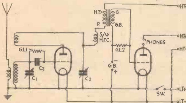
Fig. 1.—A simple two-valve regenerative short-wave receiver. C1=.0001 mfd., C2=.0003 mfd., C3=.0001 mfd., GL1=2 to 5 megohms, GL2=1 megohm.
