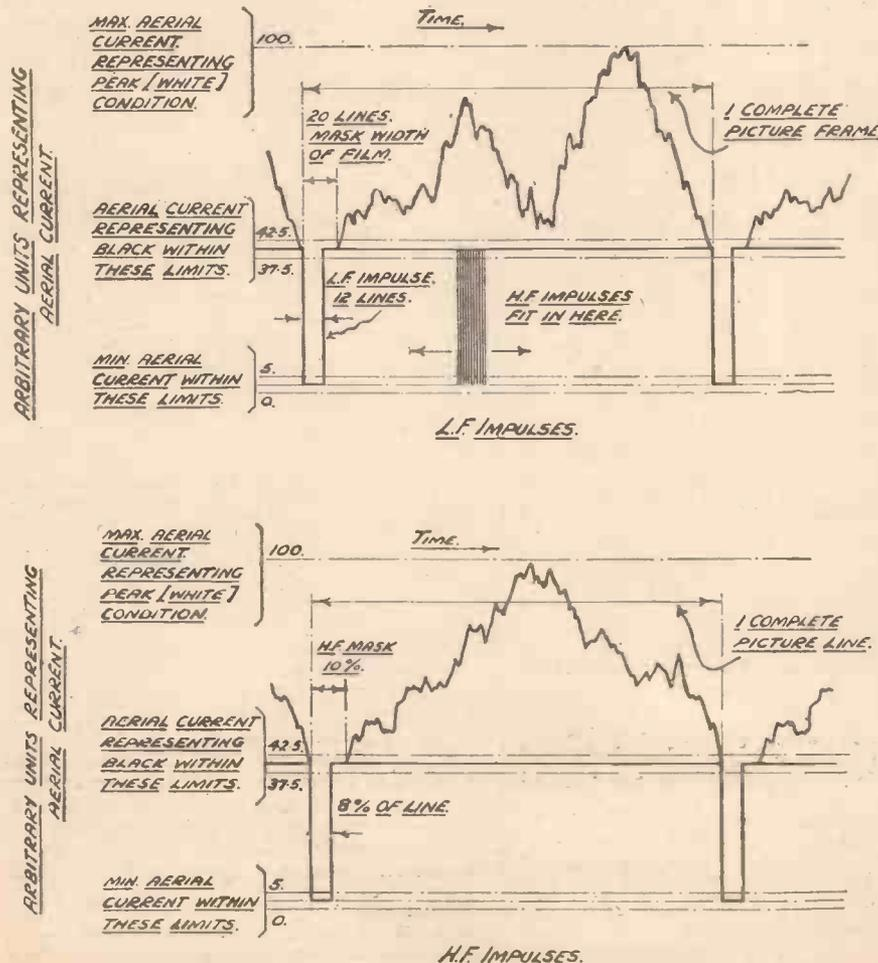
Fig. 1.—Picture modulation and synchronising impulses of the Baird system. These drawings are made from tracings taken from the vision transmitter monitoring oscillograph.
