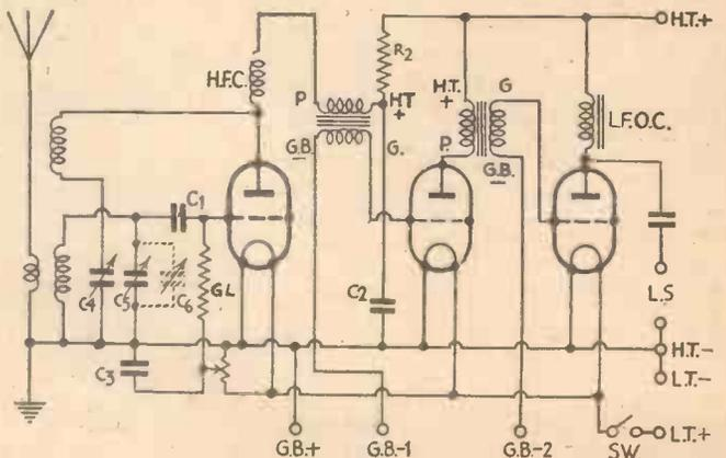
Fig. 3.—Circuit for a straight three-valve short-wave receiver with two stages of L.F. transformer coupling. C1=.0001 mfd., C2=2 mfd., C3=1 mfd., C4=.00016 mfd., C5=.00016 mfd., C6=Band Spread (capacity will depend upon coils used), R2=20,000 ohms, GL=2-3-5 megohms, R3=400 ohms potentiometer, SW=on-off switch.
