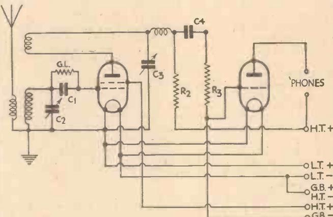
Fig. 2.—A circuit incorporating S.G. Detector, and R.C.C. L.F. stage. C1=.0001 mfd., C2=.0001 mfd. to .00016 mfd., C3=.0001 mfd. to .00016 mfd., C4=.01 mfd., GL=3 megohms, R2=100,000 ohms, and R3=1/2 megohm.
