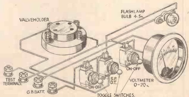
A simple apparatus for testing valve filaments.
