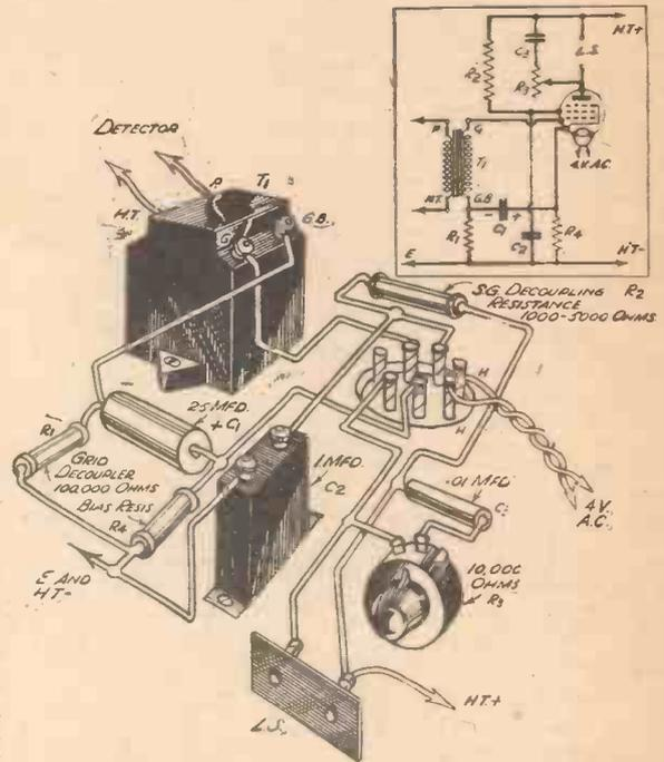
Fig. 3.—Showing the method of decoupling the grid and screening-grid circuits of an indirectly-heated pentode.
