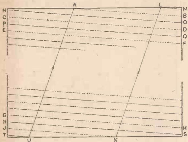
Fig. 3.—Diagram explaining the E.M.I. system of interlaced scanning.
