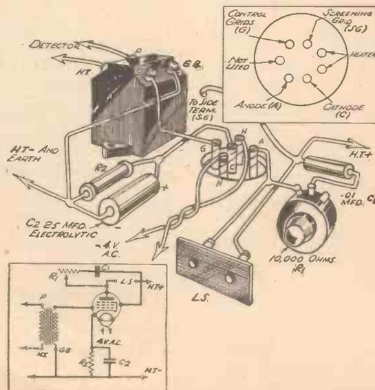
Fig. 2.—The connections for an indirectly-heated pentode. The pictorial view shows the valve connections when using a pentode with side-base screening-grid terminal, but inset are connections when using a seven-pin valve.
