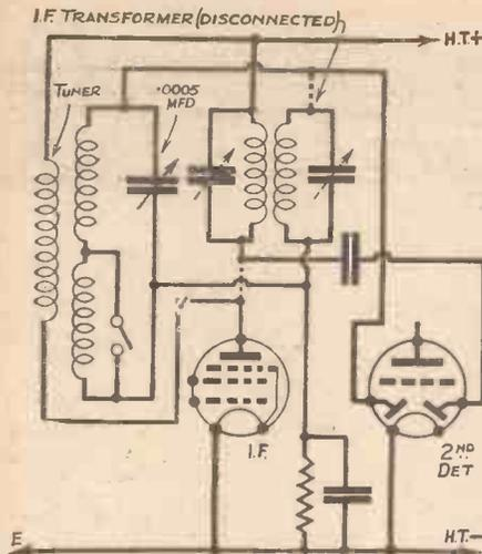
Fig. 4.—When a double-diode-triode type of valve is used as second detector the I.F. transformer which feeds it should be replaced by a double-wound tuner and .0005 mfd. variable condenser as shown here.
