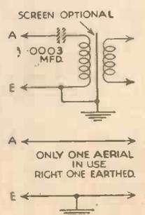
Fig. 4.—The same aerial system as that shown in Fig. 3, arranged for medium and long-wave reception. Note remarks with reference to coupling units.
