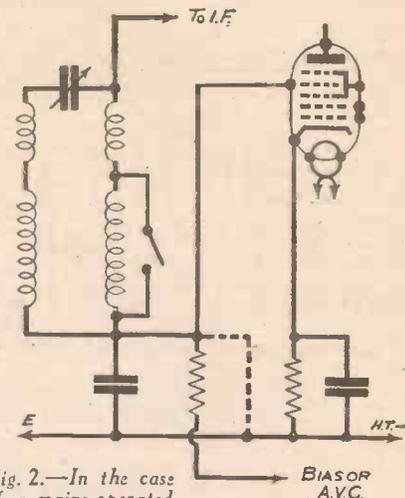
Fig. 2.—In the case of a mains-operated set the detector grid of the frequency-changer should be connected so as to receive the normal bias, as shown, when using the modified connections shown in Fig. 1.
