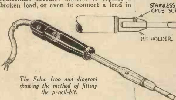
The Solon Iron and diagram showing the method of fitting the pencil-bit.
