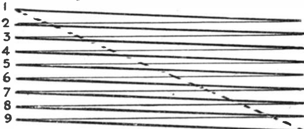
Fig. 1.—The above diagram shows how the picture area of the Baird System is built up in a regular manner. Each line is formed immediately below the preceding one, and it is claimed that the alternative system shown in Fig. 2 avoids flicker. The dotted line shows the course of the spot in its return to the commencement of the picture area.
