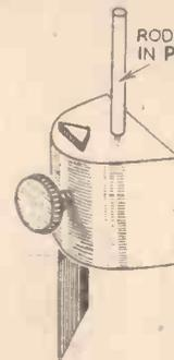
Fig. 9.—If the triangular type of fibre needle is obtained an adaptor of this type must be used. Fibre needles may now be obtained, however, with a round shank.
