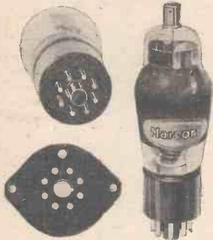
The above illustrations show the new Marconi octal base and holder, and the high-efficiency valve W.63.
