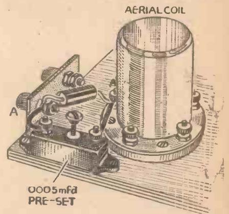
Fig. 3.—An alternative method to that shown in Fig. 2. A pre-set condenser is connected in parallel with the normal aerial-series condenser.
