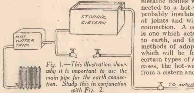
Fig. 1.—This illustration shows why it is important to use the main pipe for the earth connection. Study this in conjunction with Fig. 2.
