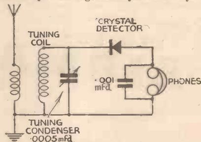
Fig. 2.—A simple crystal-receiver circuit which shows how a tuning circuit and a detector circuit can be combined.
