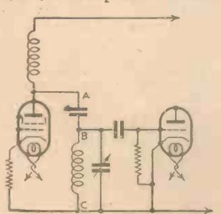
In this arrangement the ripple voltage across the grid circuit BC is practically negligible.
