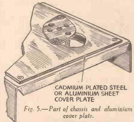
Fig. 5.—Part of chassis and aluminium cover plate.
