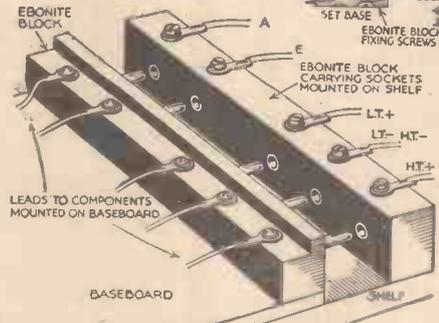
A simplified method of making connections for experimental purposes.
