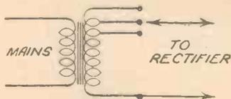
Fig. 5.—A tapped transformer will enable various accumulators to be charged.
