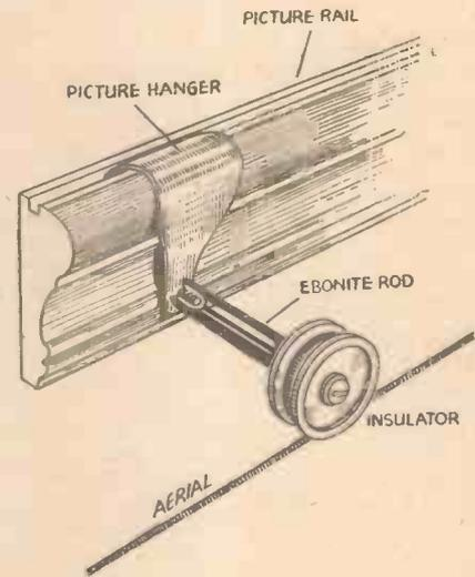
Fig. 3.—An aerial may be suspended from a picture rail by means of this device.
