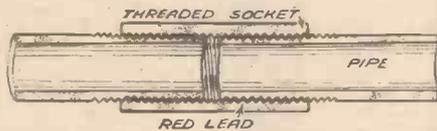
Fig. 2.—Some pipes are painted when joined, and thus a high resistance may be set up, resulting in inefficiency.
