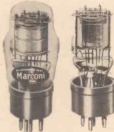
General view and the electrode assembly of the KT type valves.
