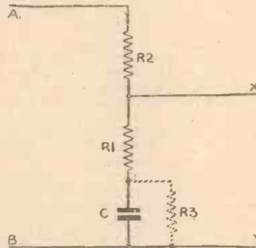
Fig. 6.—How the bass booster is connected and its method of working.
