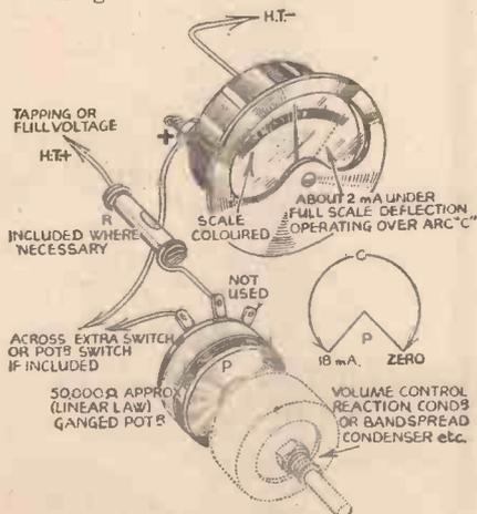
A method of obtaining visual indication of the functions of a circuit.
