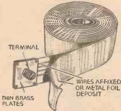
Fig. 1.—The invisible type of adhesive aerial, of which the "Pix" is a good example.
