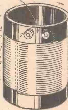
Terminals should not be placed too near each other, as leakage and signal loss may thereby arise as indicated here.
