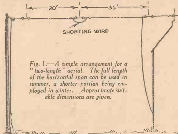
Fig. 1.—A simple arrangement for a "two-length" aerial. The full length of the horizontal span can be used in summer, a shorter portion being employed in winter. Approximate suitable dimensions are given.
