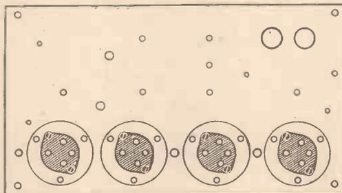
Fig. 4.—Four combined rings and sockets mounted on a chassis.
