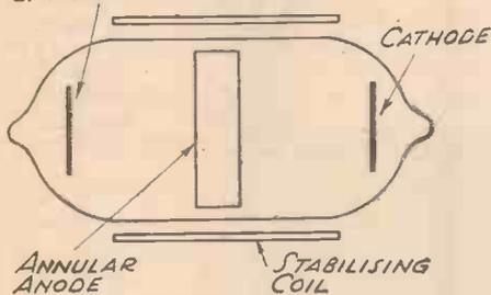
Fig. 1.—The form of multiplier due to Farnsworth which operates in a reciprocal fashion.
