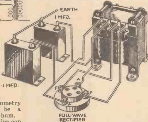
Modulation hum may sometimes be cured by means of fixed condensers connected as shown here.
