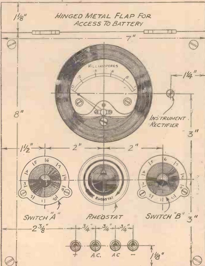
Fig. 1.—These measurements give the layout position for the panel of the instrument.
