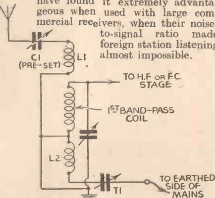
Fig. 2.—The static-suppressor applied to a band-pass circuit of a receiver. Component values as in Fig. 1.
