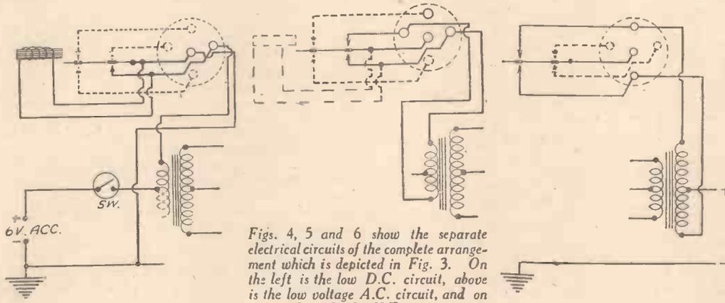
Figs. 4, 5 and 6 show the separate electrical circuits of the complete arrangement which is depicted in Fig. 3. On the left is the low D.C. circuit, above is the low voltage A.C. circuit, and on the right the H.T. circuit.
