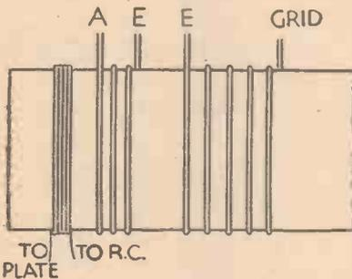
For the simple detector stage the necessary aerial, grid and reaction windings should be arranged as shown here.
