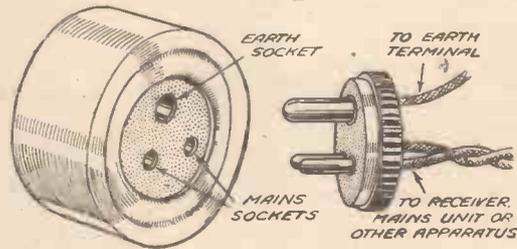
Fig. 3.—An ideal indoor earth connection may be made to the earthing pin on a 3-wire mains system as shown here.
