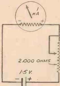
Fig. 4.—This diagram shows how the other ranges are obtained by means of a resistance connected in series.
