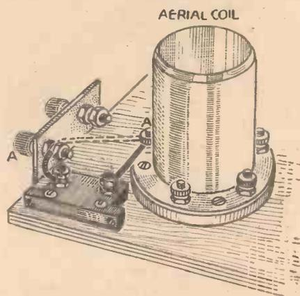
Fig. 2.—Try the effect of cutting out the aerial-series condenser by means of the wire shown as a broken line.
