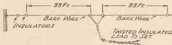
Fig. 4.—Arrangement of the doublet aerial, which gave most satisfactory results.
