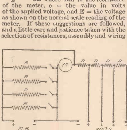
Fig. 7.—Complete circuit of the all-purpose meter as described.
