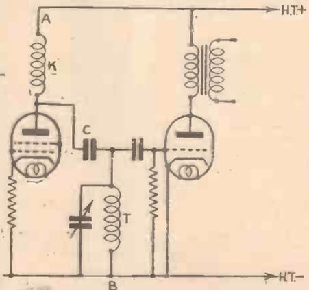
Fig. 3.—The tuned-grid circuit which overcomes the difficulties mentioned above.
