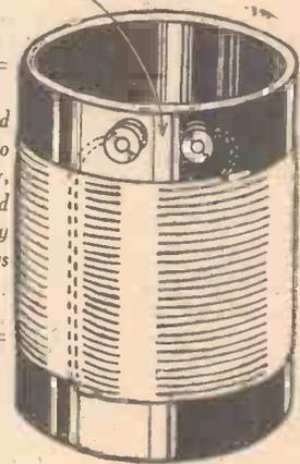
Terminals should not be placed too near each other, as leakage and signal loss may thereby arise as indicated here.
