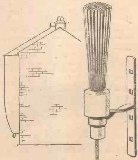
Fig. 4.—The "No-Mast" aerial which is highly successful when garden facilities are not available.
