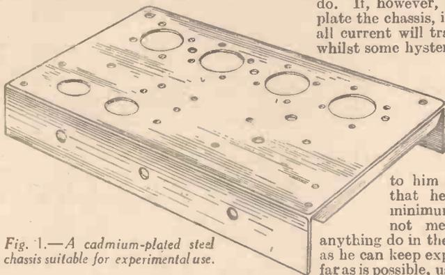
Fig. 1.—A cadmium-plated steel chassis suitable for experimental use.
