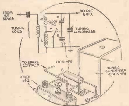
Trimming condensers may be switched by adopting the arrangement shown here.
