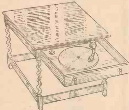
Fig. 2.—When the table is fitted with a drawer, it is often a simple matter to install the turntable. The drawer must be long, so that it is supported and kept in a horizontal position when partly open to make the pick-up accessible.
