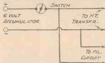
Fig. 2.—Theoretical connections for feeding the heater circuit of 6 volt mains-type valves.
