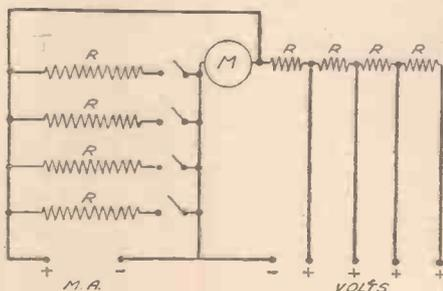
Fig. 7.—Complete circuit of the all-purpose meter as described.
