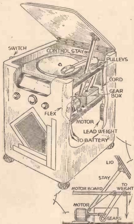
Raising a radiogram lid by means of a small electric motor.
