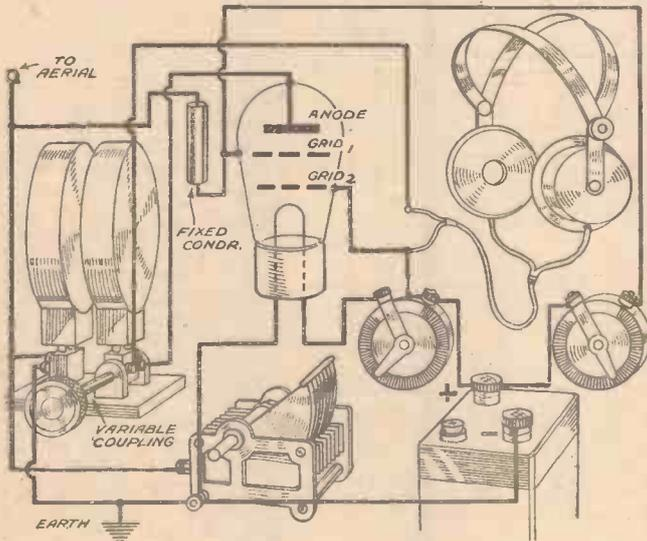
Fig. 1.—This is one of the earliest circuits designed to dispense with the H.T. Battery. A special 2-grid valve was employed with the connections shown here
