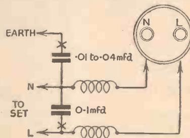
Fig. 2.—How to connect the filter to a 2-wire mains system. It is necessary to ascertain correct polarity by testing with a lamp between each pole and earth. The one which lights the lamp is "L" (live).
