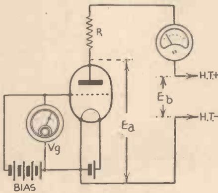
Fig. 3.—Circuit arrangement for taking dynamic curves or other valve data.
