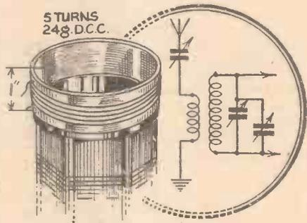
Fig. 2.—A loose coupled aerial coil to stand on top of the standard four-pin plug-in coil.
