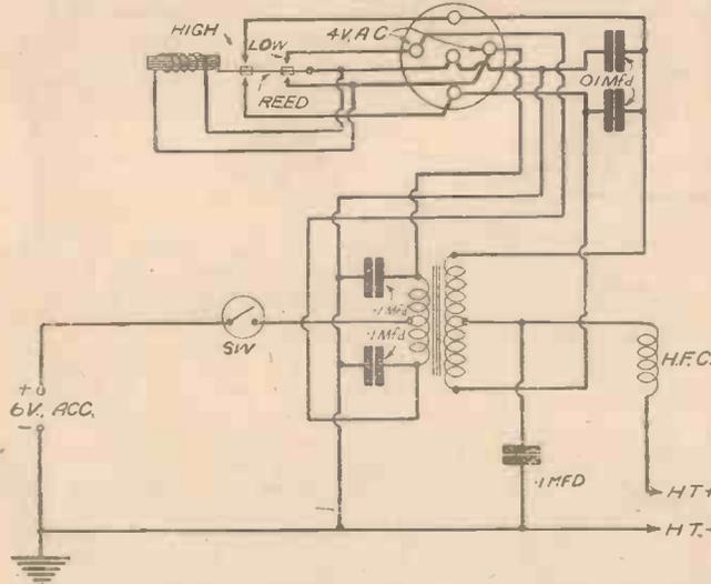
Fig. 1.—Complete circuit diagram of the H.T. unit showing the vibrator and rectifier on the left, and smoothing and voltage dropping circuit on the right.
