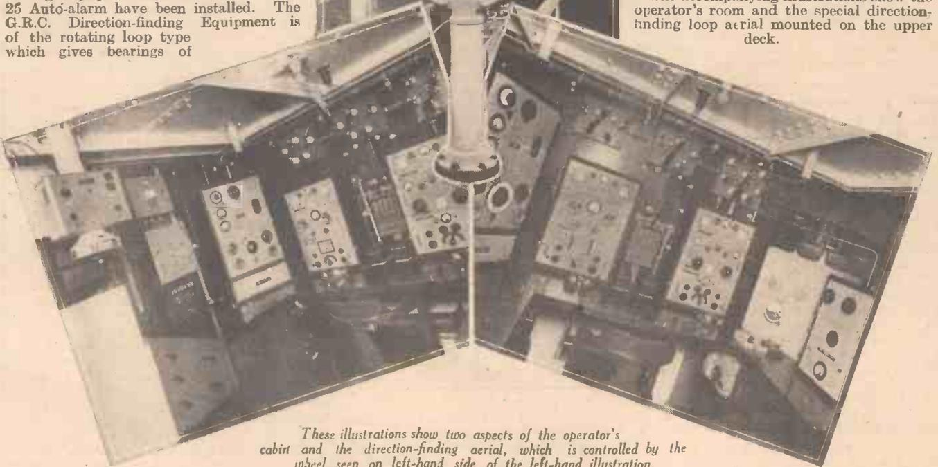
These illustrations show two aspects of the operator's cabin and the direction-finding aerial, which is controlled by the wheel seen on left-hand side of the left-hand illustration.
