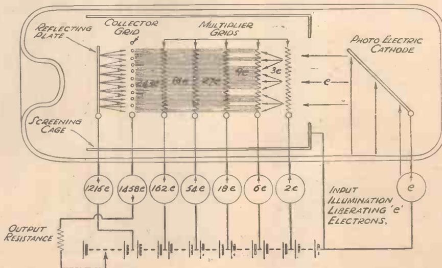
Fig. 5.—A simple schematic diagram to show the Weiss principle of secondary multiplication.
