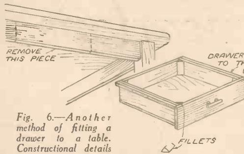
Fig. 6.—Another method of fitting a drawer to a table. Constructional details of the drawer are also suggested.
