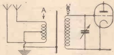
Fig. 2.—How the electro-static screen is interposed to prevent the capacity coupling.
