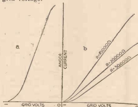
Fig. 1.—The standard grid-volts/anode-current curve, and the effect of varying loads shown graphically.
