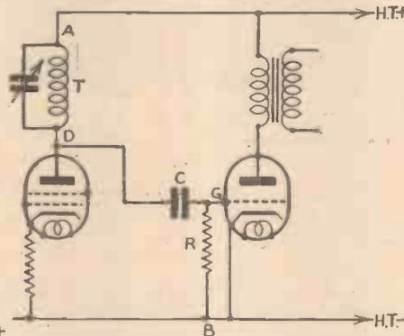
Fig. 1.—A standard tuned-anode circuit.
