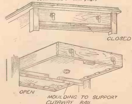
Fig. 5.—This form of construction can be used when the drawer is fairly shallow.
