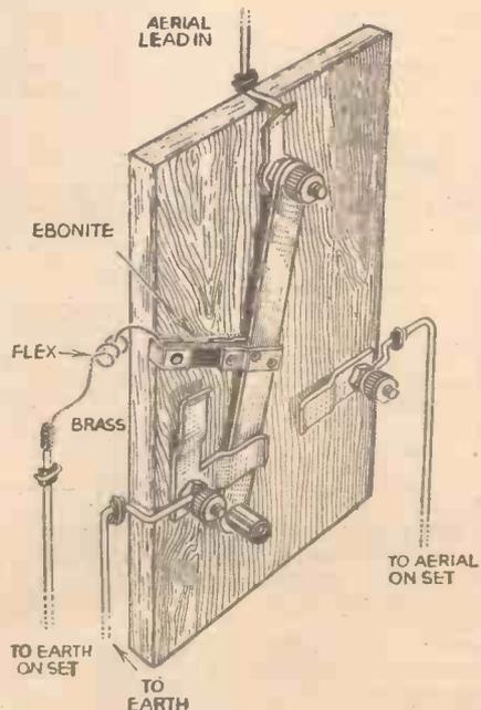
An aerial-earth switch which completely isolates the earth lead when the set is not in use.
