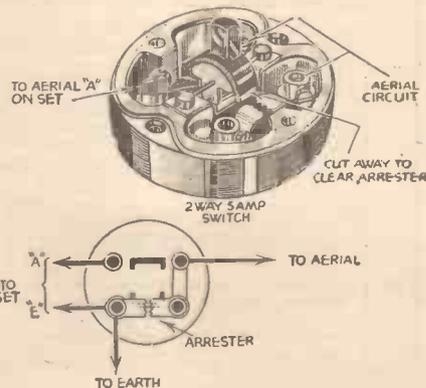
A two-way electric-light switch adapted for use as an aerial-earth switch.
