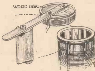
Fig. 3.—A "swinging" aerial coupling coil, which was used with success. Leads from the moving coil should be kept as short as possible.
