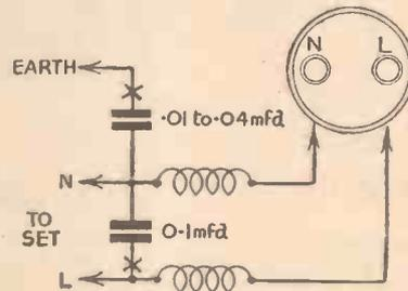
Fig. 2.—How to connect the filter to a 2-wire mains system. It is necessary to ascertain correct polarity by testing with a lamp between each pole and earth. The one which lights the lamp is "L" (live).
