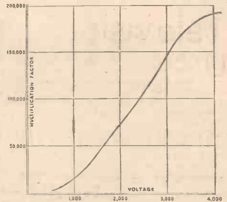
Fig. 6.—Multiplication plotted against total voltage for the smaller type Baird cell.
