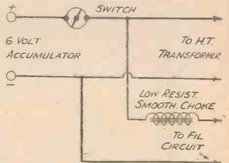
Fig. 3.—This arrangement must be used for supplying the filaments of battery (2 volt) valves.
