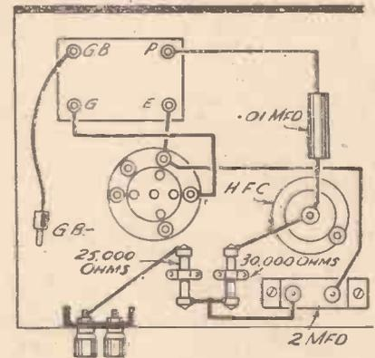
Fig. 5.—Here the connections shown in Fig. 3 have been modified to include a 25,000-ohm decoupling resistance and 2-mfd. condenser. The position of the 30,000-ohm resistance has also been changed.
