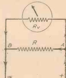
Fig. 2.—This diagram shows the principle upon which the shunts work when joined across the meter.
