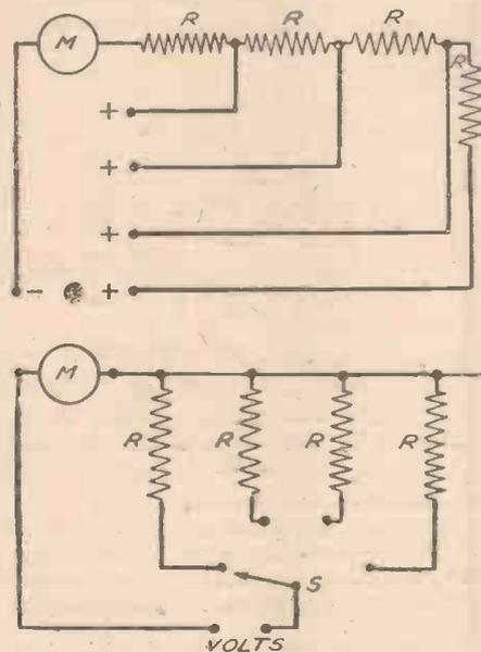
Fig. 6.—How to arrange the separate resistances to provide alternative readings.
