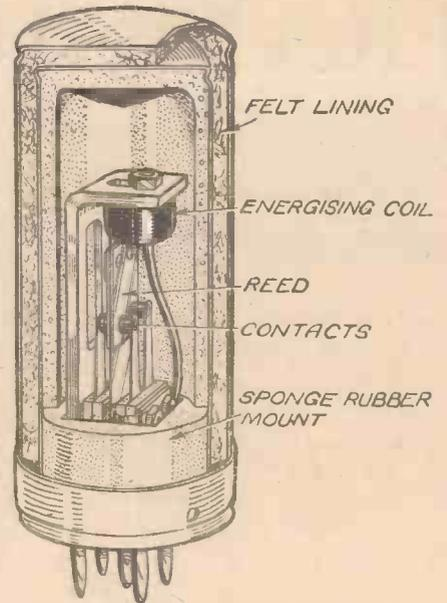
Fig. 5.—Our artist has here shown the internal arrangement of the vibratory-rectifier, but the constructor should not remove the screening cover in view of the risk of damage.
