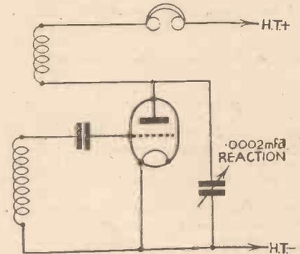
Fig. 5.—Connections for throttle-control reaction.
