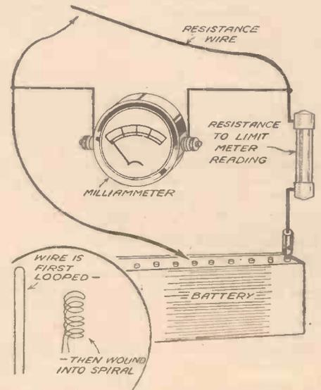
Fig. 5.—Method of making accurate shunts from resistance wire.
