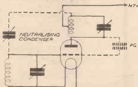
Fig. 2.—The inter-electrode capacity and method of balancing it out.
