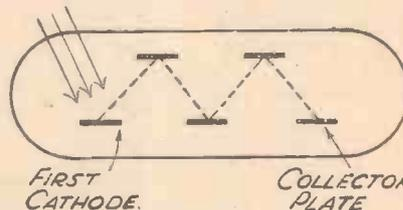
Fig. 3.—Showing the zig-zag path, followed by the electrons in moving from each secondary emitting surface.
