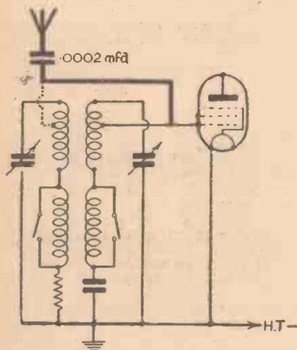
Fig. 4.—Cutting out one circuit of a band-pass filter. The original aerial lead is shown as a broken line, and the new one as a heavy line.
