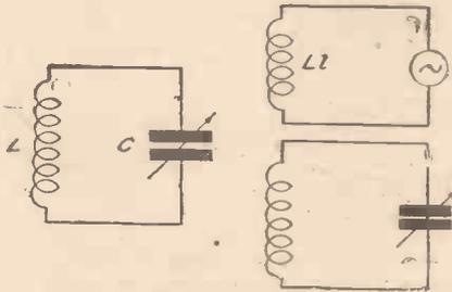
Figs. 1 and 2.—Circuit diagrams of an absorption type frequency meter.
