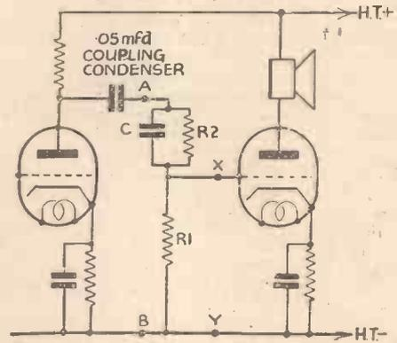
Fig. 3.—Standard R.C. circuit with high-note booster.
