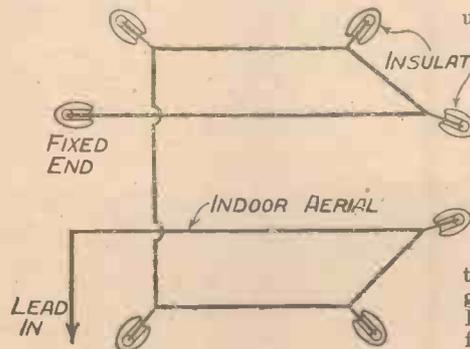
Fig. 2.—When erecting an aerial in a loft, adopt this arrangement in order to accommodate a lot of wire in a small area.
