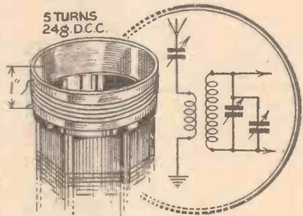
Fig. 2.—A loose coupled aerial coil to stand on top of the standard four-pin plug-in coil.
