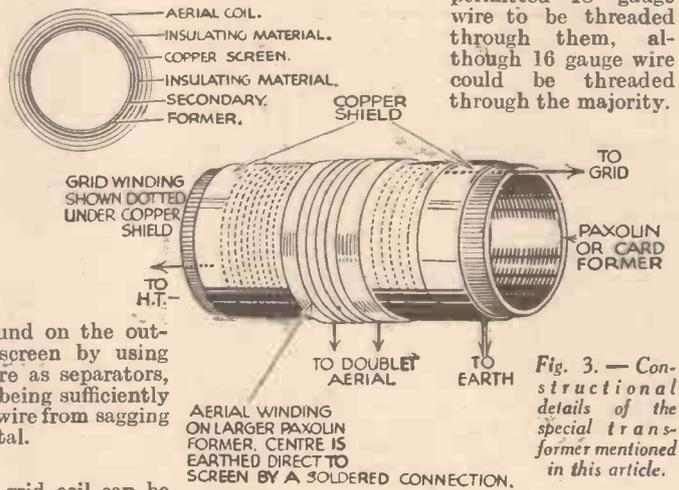
Fig. 3.—Constructional details of the special transformer mentioned in this article.
