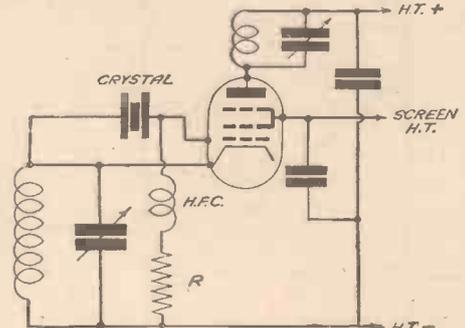
Fig. 4.—Circuit diagram of the Tritet oscillator.
