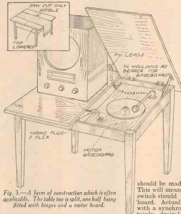
Fig. 3.—A form of construction which is often applicable. The table top is split, one half being fitted with hinges and a motor board.
