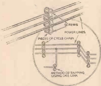
A method of using odd pieces of cycle chain for supporting outdoor wiring.
