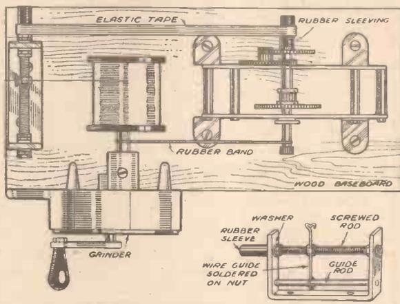
An automatic wire guide for use in coil winding.
