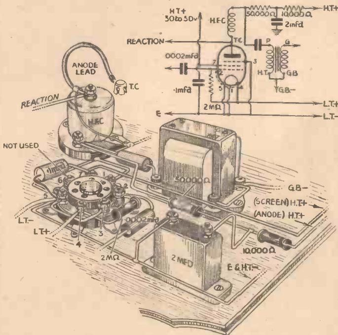
Fig. 6.—How an H.F. pentode can be used as detector to improve sensitivity and reaction control.
