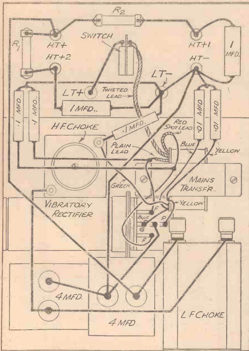
Fig. 4.—Wiring Diagram of the complete H.T. Unit.
