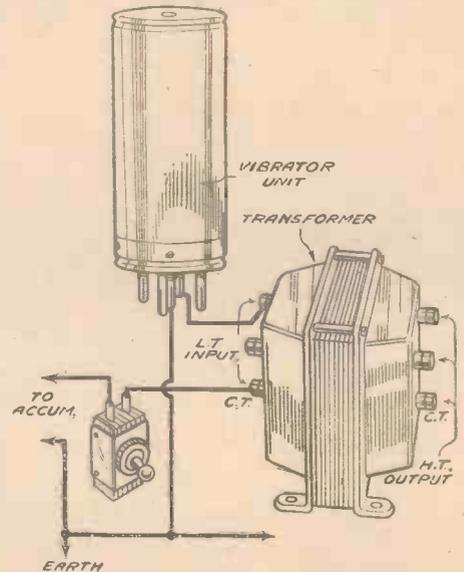
Fig. 6.—Pictorial diagram showing the input arrangements for rectifier and transformer.
