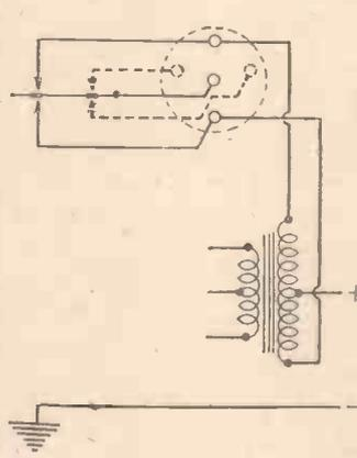
Figs. 4, 5 and 6 show the separate electrical circuits of the complete arrangement which is depicted in Fig. 3. On the left is the low D.C. circuit, above is the low voltage A.C. circuit, and on the right the H.T. circuit.
