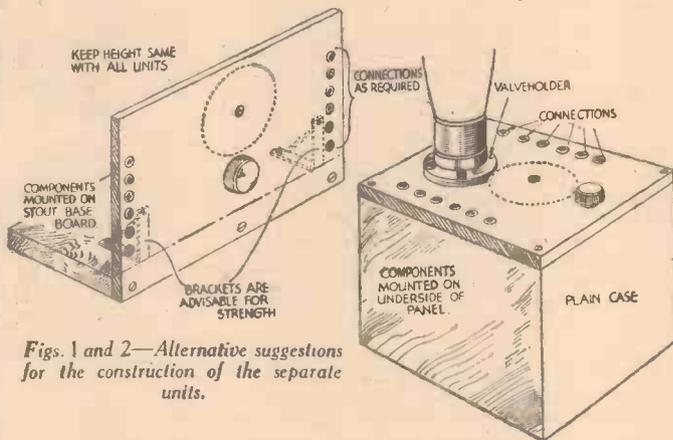
Figs. 1 and 2—Alternative suggestions for the construction of the separate units.
