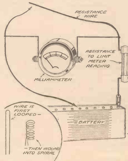
Fig. 5.—Method of making accurate shunts from resistance wire.
