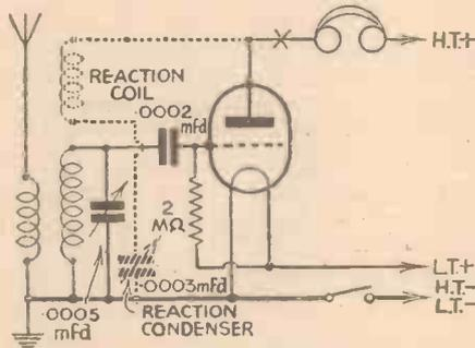
Fig. 3.—Circuit for a single valve set having a tuning system similar to that shown in Fig. 2. The reaction circuit is shown in broken lines. When using reaction it is generally desirable to insert an H.F. choke at the point marked X.
