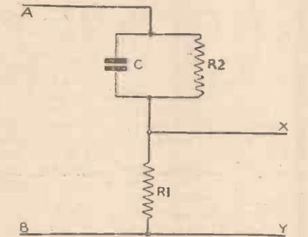
Fig. 2.—In this arrangement high notes will be boosted.
