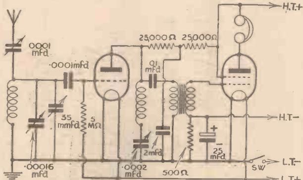
Fig. 1.—The two-valve S.W. circuit sent by a reader, G6KR.
