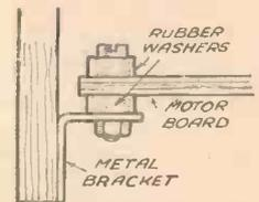
Fig. 4.—It is a good plan to fit rubber washers above and below the motor board to permit a small amount of "float."
