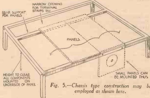
Fig. 5.—Chassis type construction may be employed as shown here.
