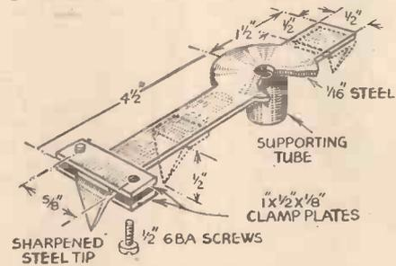
A handy tool for cutting thin sheet-metal, plywood or ebonite.
