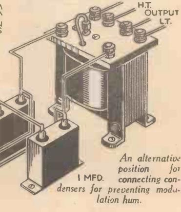
An alternative position for connecting condensers for preventing modulation hum.
