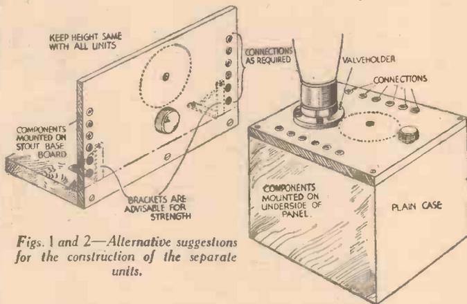
Figs. 1 and 2—Alternative suggestions for the construction of the separate units.
