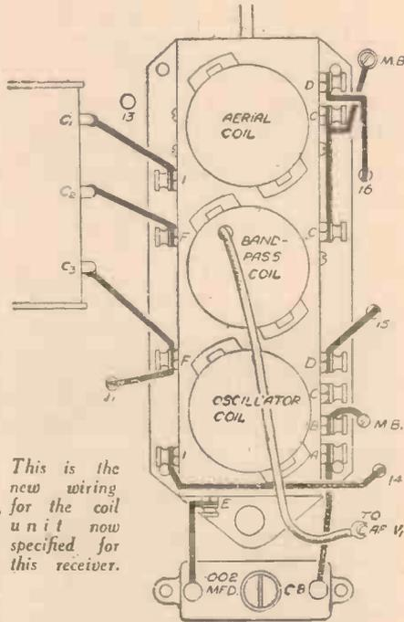
This is the new wiring for the coil unit now specified for this receiver.
