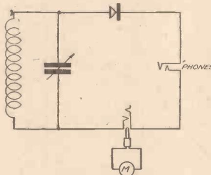
Fig. 3.—Circuit diagram of a simple over-modulation indicator.
