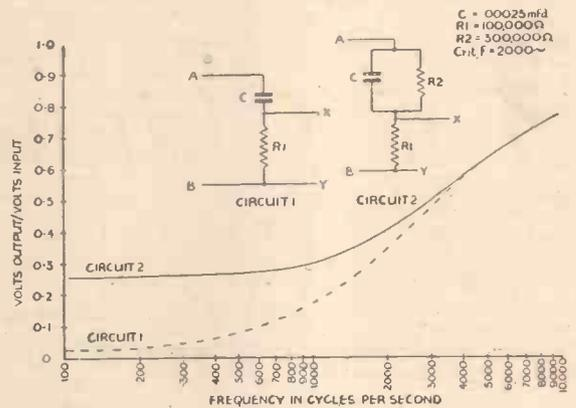
Fig. 4.—Graph illustrating the effects of high- and low-note boosters.
