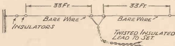
Fig. 4.—Arrangement of the doublet aerial, which gave most satisfactory results.
