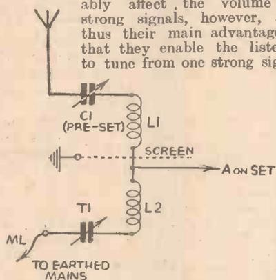
Fig. 1.—A simple circuit for cutting out interference. L1 and L2 are 40 to 60 microhenries each. C1—.0001 to .0003 mfd. T1—.00005-.00025 mfd.
