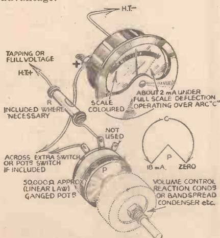
A method of obtaining visual indication of the functions of a circuit.
