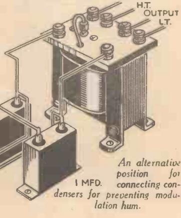
An alternative position for connecting condensers for preventing modulation hum.
