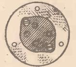
Fig. 3.—A wafer socket mounted on a paxolin ring.
