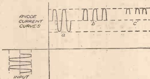
Fig. 1.—The different effects on a signal due to working on various parts of the grid-volts/anode-current curve.
