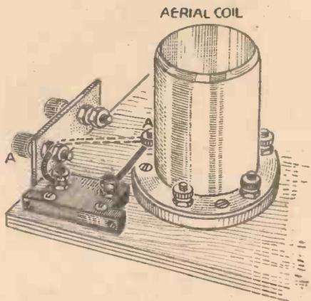
Fig. 2.—Try the effect of cutting out the aerial-series condenser by means of the wire shown as a broken line.
