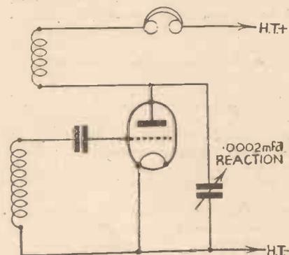
Fig. 5.—Connections for throttle-control reaction.
