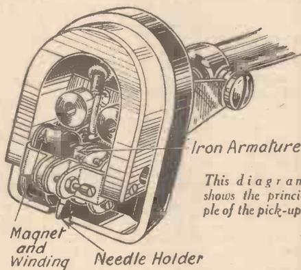
example of which is shown here, the magnet has usually two poles, and the needle is inserted into a holder which is extended and rests between the two poles. As the needle is moved by the sound grooves on the record, the armature moves, and this varies the magnetic field causing a varying current to flow in the windings. This current variation is applied to a valve, just as in the case of wireless signals, and so produces the signal.
