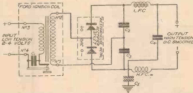
Fig. 2.—This is the early form of H.T. generator using a dismantled Ford car spark coil.
