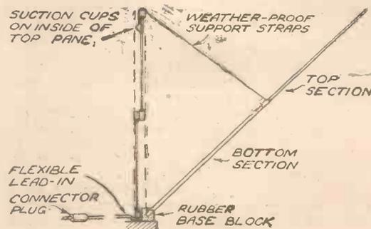
a useful device is the Philco aerial which is made to suspend out of the window, and the accompanying illustration shows how this is fixed to the window frame.
