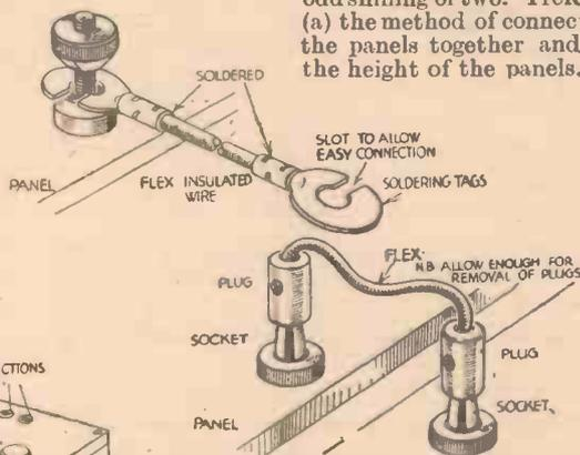
Fig. 3.—Inter-connection between units may be carried out by such schemes as those illustrated above.
