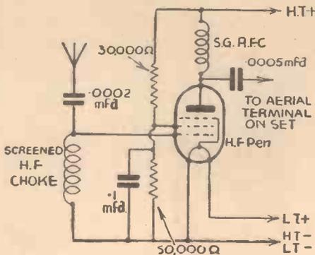
Fig. 5.—Circuit for a simple untuned H.F. amplifier for use between the aerial and aerial circuit of a Det.-L.F. receiver.
