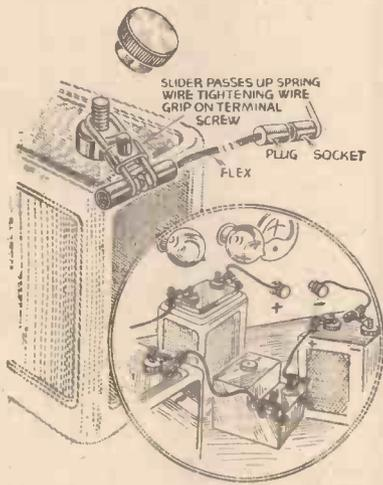
A simple and effective way of making good connection to terminals.
