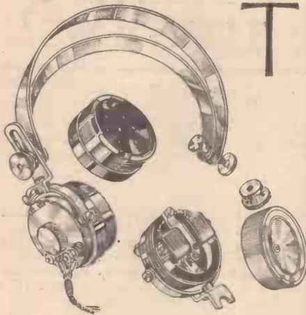
Fig. 1.—A complete earpiece and details of the reed type headphones made by S. G. Brown and Co.
