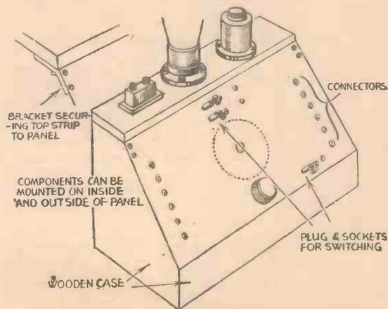
Fig. 4.—This form of construction possesses several advantages but is slightly more difficult to build.
