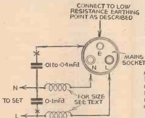
Fig. 1.—Connecting an H.F. filter to a 3-pin mains point.
