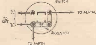
A two-way electric-light switch adapted for use as an aerial-earth switch.
