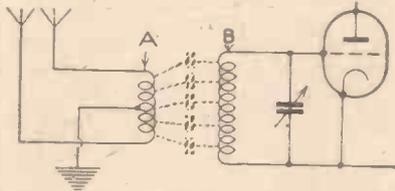
Fig. 1.—Diagram illustrating self-capacity between the grid and aerial coils.
