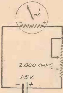
Fig. 4.—This diagram shows how the other ranges are obtained by means of a resistance connected in series.
