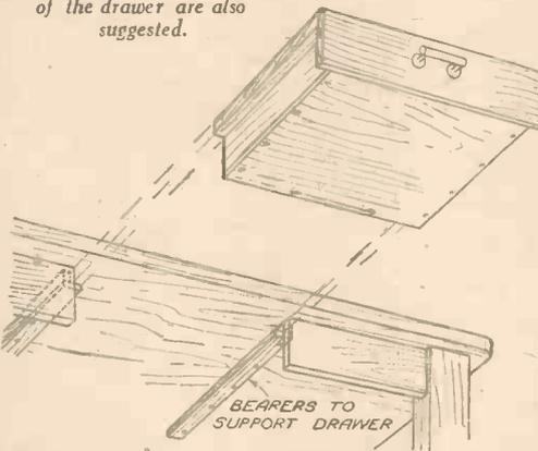
parts of the front member. If the work is neatly carried out, the table will appear to be unaltered when the drawer is closed. Here again, however, it will generally be considered wise to have the assistance of a joiner if the table is not to be disfigured.
