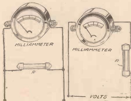
Figs. 3 and 4 show the method of connecting shunts and series resistances for multiplying the range.
