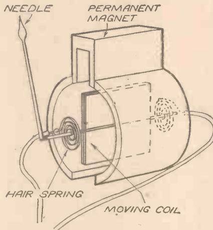
Fig. 2.—The method of construction employed in the milliammeter.
