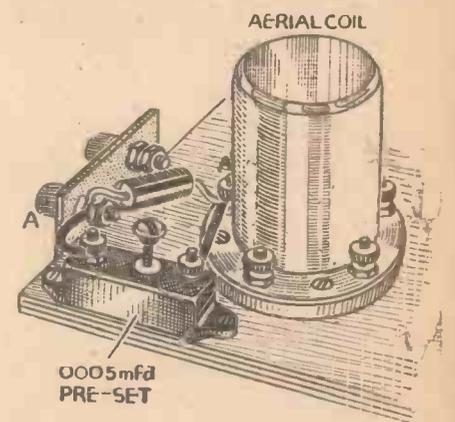
Fig. 3.—An alternative method to that shown in Fig. 2. A pre-set condenser is connected in parallel with the normal aerial-series condenser.
