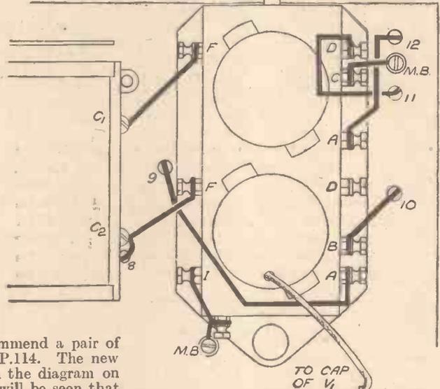
Connections required for the new coil unit Varley B.P. 114.
