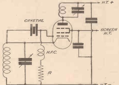
Fig. 4.—Circuit diagram of the Tritet oscillator.
