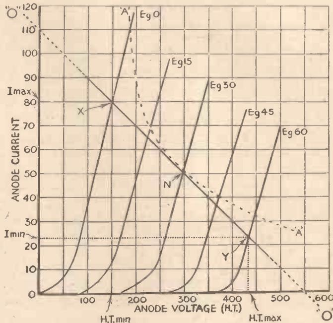
Fig. 2.—Dynamic curve, showing load line, dissipation, and other important working data.
