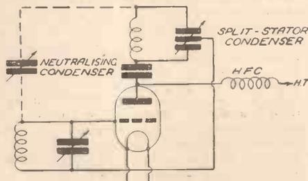
Fig. 3.—An alternative method of obtaining a centre-tapped anode load, utilising a split-stator condenser.
