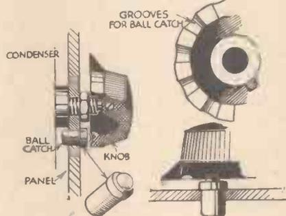
A band-setting device for use with ordinary control knobs.
