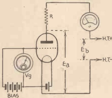
Fig. 3.—Circuit arrangement for taking dynamic curves or other valve data.
