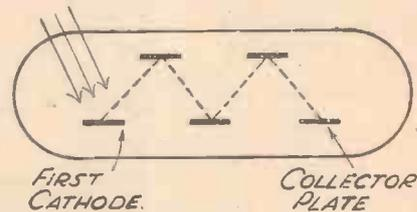
Fig. 3.—Showing the zig-zag path, followed by the electrons in moving from each secondary emitting surface.
