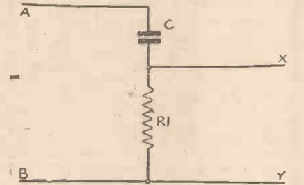
Fig. 1.—Circuit to illustrate reactance of a condenser and resistance.
