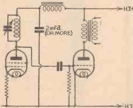
Fig. 2.—How the smoothing may be increased by including an L.F. choke.
