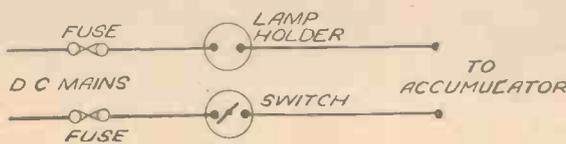
Fig. 2.—On D.C. Mains, quite a simple arrangement is called for, the circuit to be used being as shown here.
