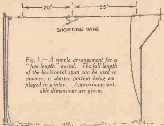
Fig. 1.—A simple arrangement for a "two-length" aerial. The full length of the horizontal span can be used in summer, a shorter portion being employed in winter. Approximate suitable dimensions are given.
