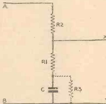
Fig. 6.—How the bass booster is connected and its method of working.
