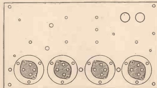
Fig. 4.—Four combined rings and sockets mounted on a chassis.
