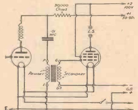
Fig. 2.—A modified form of the circuit shown in Fig. 1, where a transformer is used to feed the pentode.
