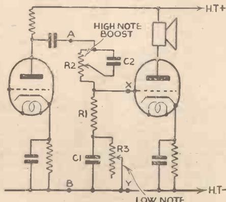
Fig. 5.—Complete circuit diagram of L.F. stage with both high- and low-note compensators.
