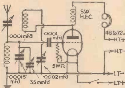
Fig. 1.—The original circuit of the single-valve set which was used for the experiments.
