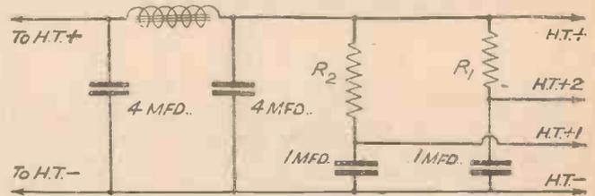
(L.F.) choke and two large capacity condensers are provided, with the separate voltage-dropping or decoupling components for the lower H.T. tapings (Fig.1). The two smoothing condensers which we used were 4 mfd. Mansbridge type, and again the individual may modify these if he so desires and use electrolytic components, provided that suitable provision for mounting them can
