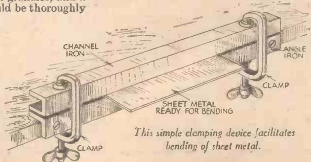
This simple clamping device facilitates bending of sheet metal.
