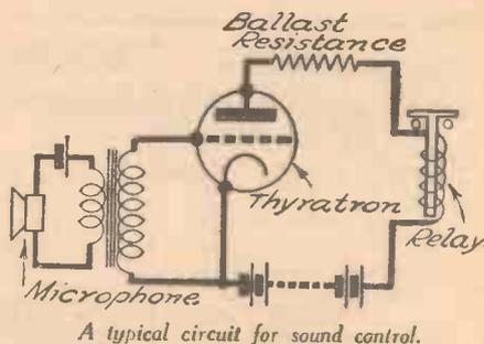
A typical circuit for sound control.
