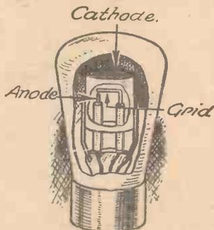
Diagram of a cold-cathode relay.
