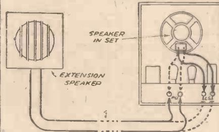
Diagram showing how the two-way phone scheme operates.
