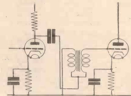
Fig. 25.—Auto-transformer coupling.
