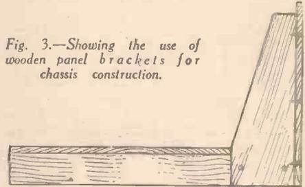
Fig. 3.—Showing the use of wooden panel brackets for chassis construction.
