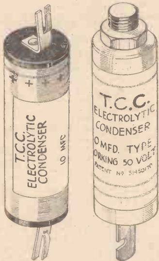
Two types of modern T.C.C. electrolytic condenser which facilitate constructional work. The model on the left may be suspended in the wiring, for which soldering tags are provided, and the right-hand model may be locked to a metal chassis for the negative connection, a lead being soldered to the tag for the positive connection.
