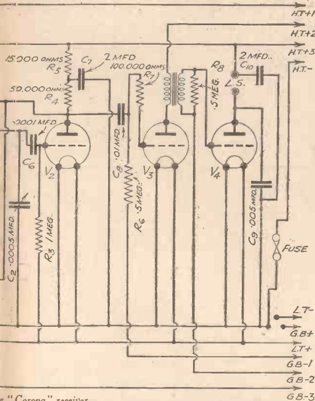
plug is inserted into the positive socket on the G.B. battery, and the G.B.—3 plug is inserted into the 9-volt socket at the other end of the battery. G.B.—1 should be plugged into the 3-volt socket and the G.B.—2 plug into the 6-volt socket for the time being, although at a later date you might find that these can be modified to produce better working results. The consumption of H.T. depends upon
