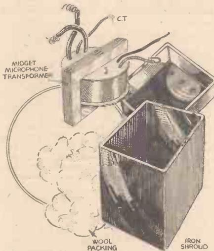
The Shaftesbury Microphone Transformer obtainable in a heavy-shrouded or an unshrouded pattern. It may be obtained to suit any particular characteristics, but standard models with 200- to 400-ohm primaries are most suitable for general use. It is designed for use with the velocity type microphone, and it will be noted that wool packing is employed to avoid vibration and other troubles.
