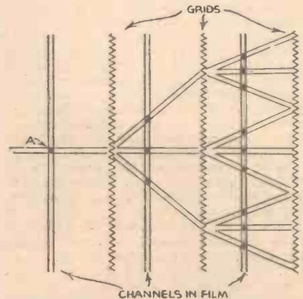
and photo-electric emission. Secondary electrons can be made to leave a prepared metallic surface provided the impact of primary electrons is undertaken with sufficient velocity. In the Baird cell, therefore, there is a series of secondary amplifying stages consisting of fine mesh metallic grids treated in such a manner that a high secondary factor exists. These are arranged
