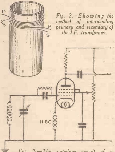
Fig. 2.—Showing the method of interwinding primary and secondary of the I.F. transformer.
