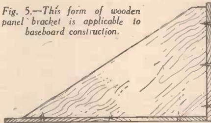
Fig. 5.—This form of wooden panel bracket is applicable to baseboard construction.
