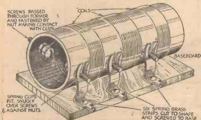
A handy coil mount with spring contact supports.
