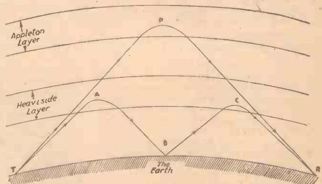
Diagram illustrating the effects of the Appleton and Heaviside layers on a wireless signal.
