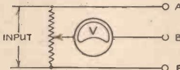
Fig. 21.—Reducing input by potentiometer control.
