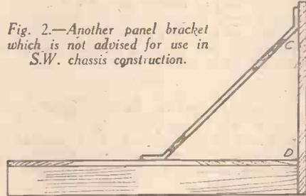
Fig. 2.—Another panel bracket which is not advised for use in S.W. chassis construction.
