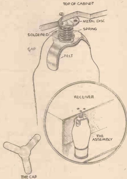
Method of making anti-vibration valveholders.
