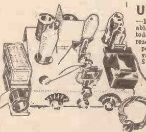
UNIQUE All-World reception —12-94 metres. Variable Mu H.F. pentode, leaky grid reacting detector, pentode output and valve rectification. Slow motion bandspread tuning. 3 calibrated scales 0-180, 0-180, 0-10. For A.C. Mains 230-250 volts, 43-100 cycles.
