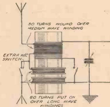
Fig. 7.—How a normal two-range coil, without separate aerial winding, can be modified for use with a doublet.
