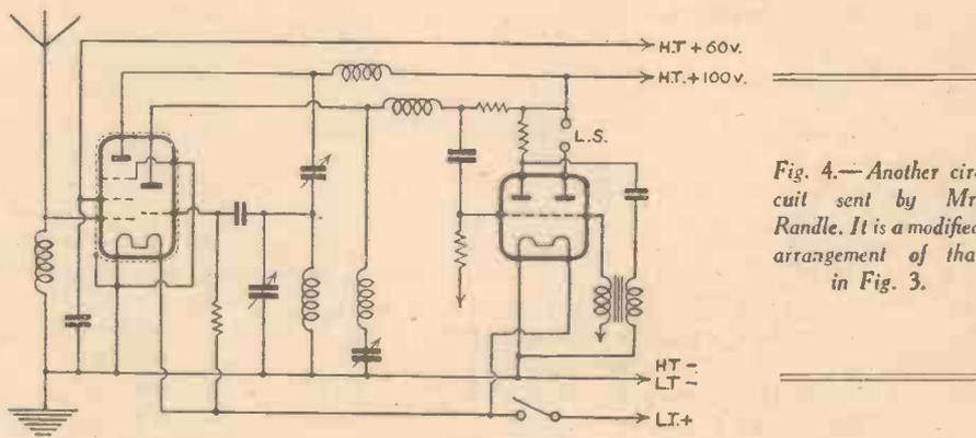
Fig. 4.—Another circuit sent by Mr. Randle. It is a modified arrangement of that in Fig. 3.
