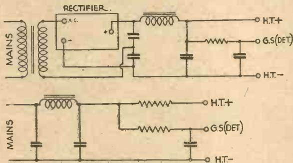
Fig. 1.—Standard circuits for an A.C. and a D.C. mains unit.
