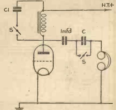
Fig. 4.—Circuit for obtaining a peaked response when using phones.
