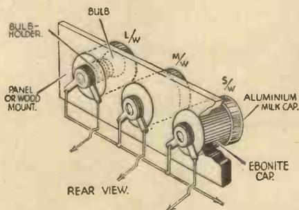
this purpose, fitting over the ebonite caps snugly. The fitment is wired to the wave-change switch contacts as shown in the theoretical circuit drawing. The holes to be drilled for the bulb holders should be
