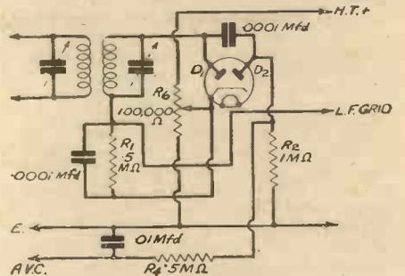
Fig. 4.—A usual form of double-diode circuit for detection and delayed A.V.C.
