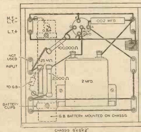
Fig. 4.—Practical wiring plan for the circuit in Fig. 1.
