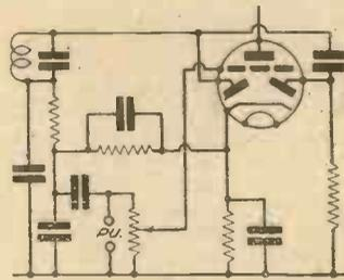
Fig. 70.—The simplest method of connecting a pick-up in a double-diode triode stage.
