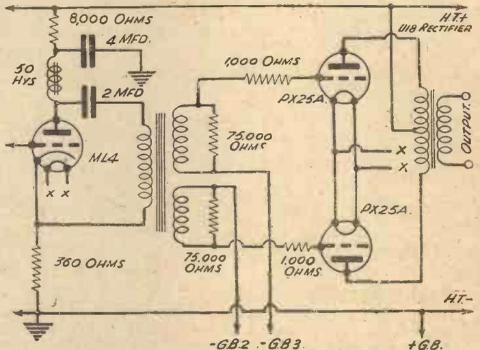
Fig. 5.—A low-impedance-loading, or class A-B circuit, using a pair of Osram PX25A valves.
