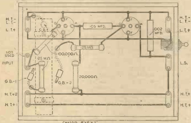
Fig. 5.—Practical layout and wiring plan for the two-valve amplifier shown in theoretical form in Fig. 3.
