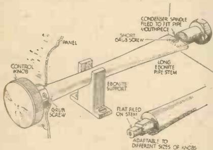
An improvised extension rod made from an old pipe mouthpiece.
