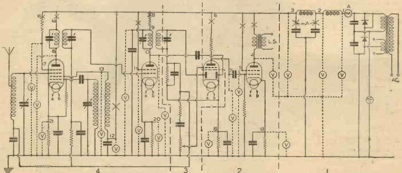
Fig. 17.—Circuit of a simple A.C. Mains superhet indicating the points at which voltage and current tests should be made.
