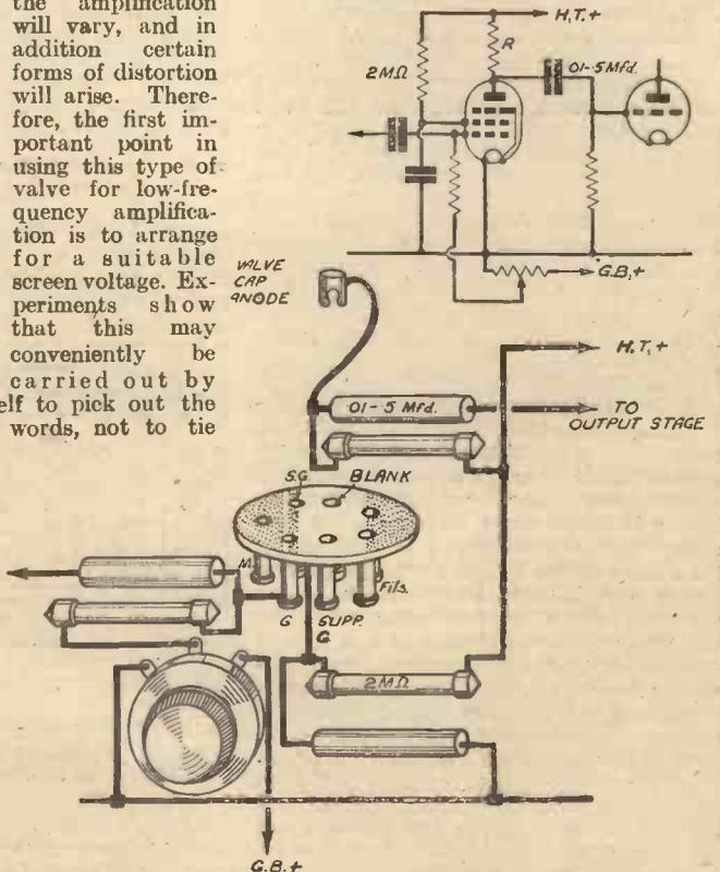
Fig. 2.—The same circuit as used when a battery valve is employed.
