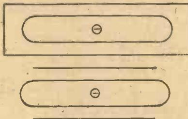
Fig. 1.—Sectional view of two triodes. Although mechanically different they are electrically similar.
