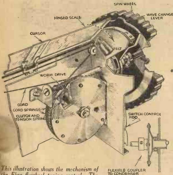
This illustration shows the mechanism of the Ekco flywheel tuning control. The drive has machine-cut gears (40 to 1), and the rim, which is 14 in. in circumference, permits very accurate settings to be obtained.
