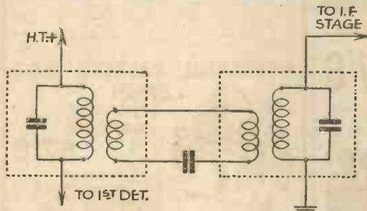
Fig. 1.—Circuit showing the principle of an I.F. filter coupling the first detector to the I.F. stage of a superhet.
