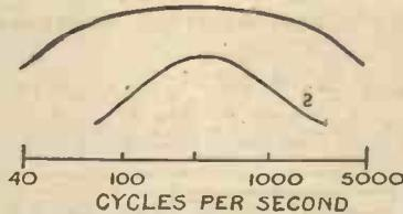
Fig. 3.—Showing what happens to speaker response when frequency range is restricted.
