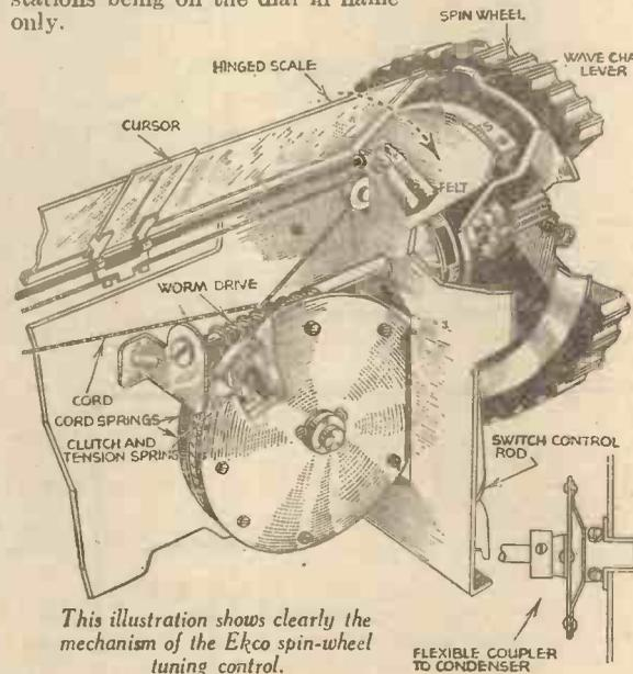
This illustration shows clearly the mechanism of the Ekco spin-wheel tuning control.
