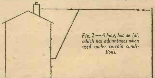
Fig. 2.—A long, low aerial, which has advantages when used under certain conditions.
