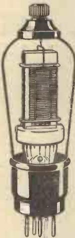
Fig. 2.—The electrode assembly of an early high-impedance valve of the type referred to in the text.
