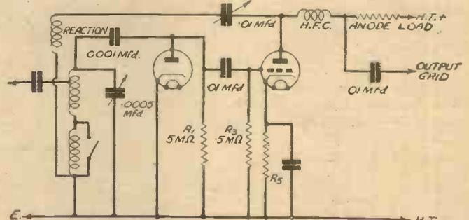
Fig. 7.—A method of obtaining reaction when using a diode detector in the normal manner. Feed-back is from the first L.F. stage.
