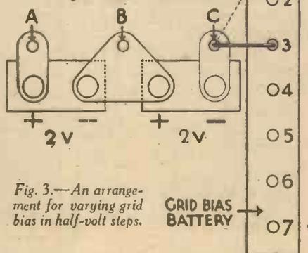
Fig. 3.—An arrangement for varying grid bias in half-volt steps.
