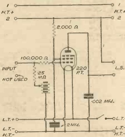
Fig. 1.—Circuit for a resistance-coupled pentode amplifier.
