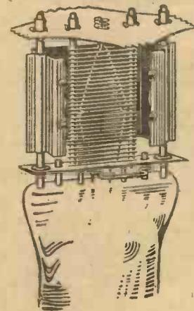
Fig. 2.—A typical triode; note the close spacing of the electrodes. The filament is held at each side by insulated hooks to keep it taut.
