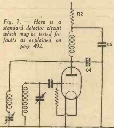
Fig. 7. — Here is a standard detector circuit which may be tested for faults as explained on page 492.
