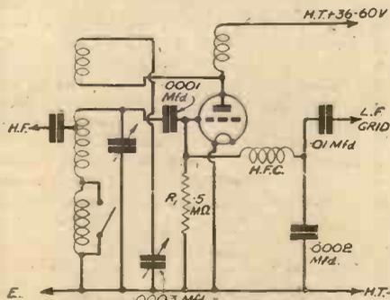
Fig. 3.—An ordinary triode valve used as a diode detector and reactor. The grid acts as a diode anode and also as a normal grid in conjunction with the "legitimate" anode, which is now used in a reaction circuit.
