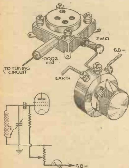
Fig. 3.—The simplest way to convert a "straight" S.G. or H.F. pentode valve into a variable-control stage is shown above. To avoid the grid bias battery discharging through the volume control an on-off switch may be joined in the G.B.—lead, as shown in broken lines, or the modification shown in Fig. 4 may be adopted.
