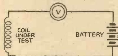
Figs. 4 and 5.—Circuit diagrams for testing a condenser, and a coil, respectively.
