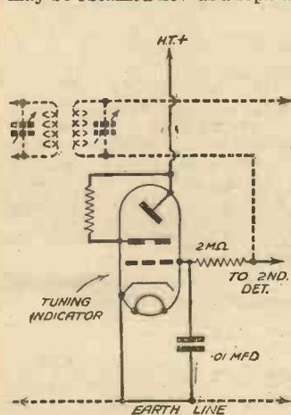
Connections for the Osram visual tuning indicator.
