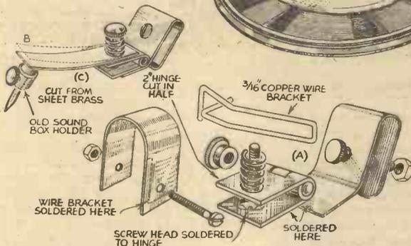
General view and details of construction of a home-made tracking device.
