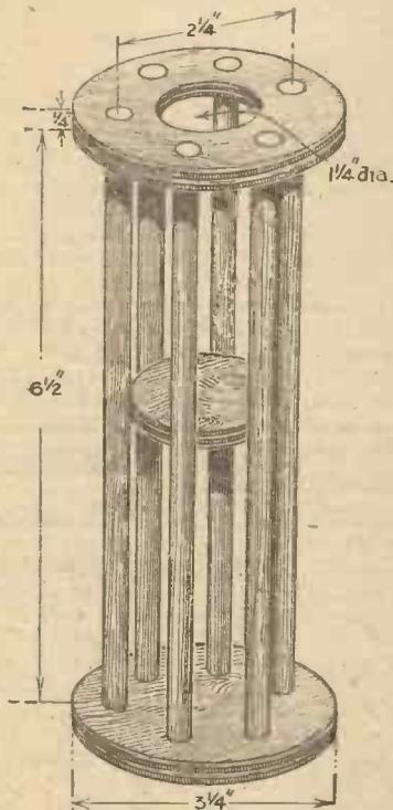
Fig. 1.—Method of making up a low-loss (squirrel-cage) coil-former.
