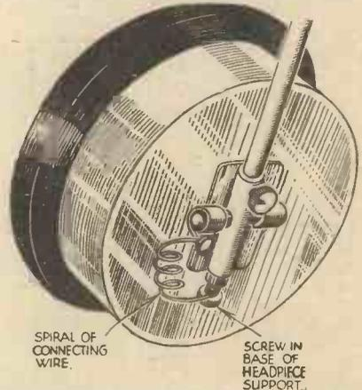
A method of preventing cracking in headphones.
