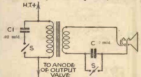
Fig. 2.—Circuit for restricting frequency range to improve signal to interference ratio.
