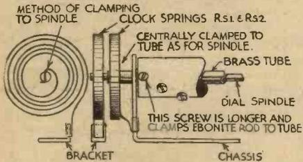
Fig. 2.—This diagram shows how the return spring is mounted on the spindle
