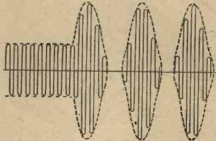
Fig. 5.—Showing the effects of over modulation. Note the wave form distortion and breaks in the carrier.
