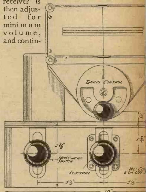
Dimensioned sketch for drilling a panel or chassis.
