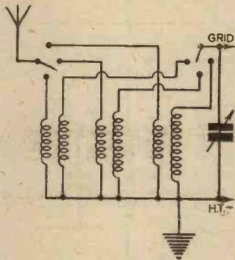
Fig. 8.—An improved form of the all-wave tuning system, shown in Fig. 7. In this case each tuned winding has its own primary or aerial winding.
