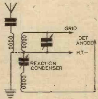
Fig. 10.—The same circuit as that in Fig. 9, but using entirely separate windings for aerial, grid, and reaction.
