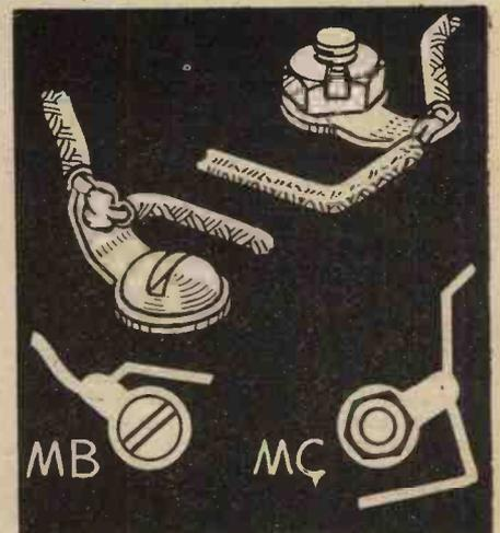
Fig. 3.—Common earth return points are joined to screws or bolts in the chassis, and are indicated as shown in this illustration.
