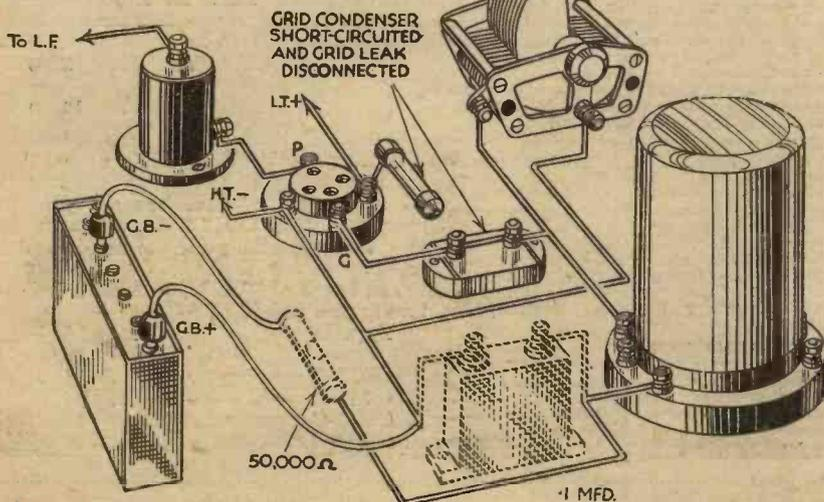
How to convert a standard detector circuit for anode-bend rectification.
