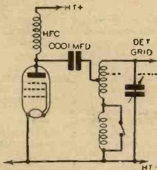
Fig. 2.—A tapped coil used in a circuit similar in form to that in Fig. 1.
