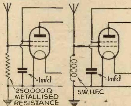
Figs. 1 and 2. Circuit diagrams showing resistance coupling and choke coupling methods.
