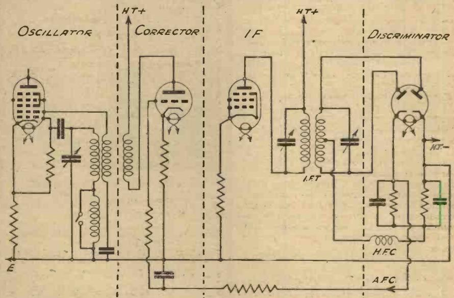
This skeleton diagram illustrates the principles described, and shows how the discriminator and corrector valves are connected.
