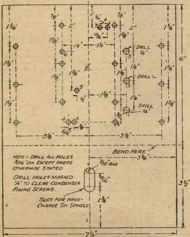
Fig. 4.—Drilling dimensions for the chassis.
