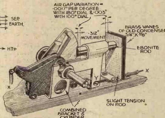
A novel device for modifying the tracking of a condenser.
