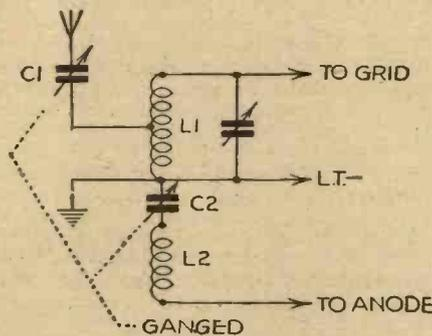
Fig. 2.—A circuit for providing constant selectivity.
