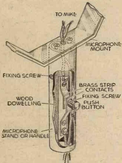
A safety-switch for a home-made microphone stand.
