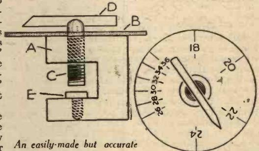
An easily-made but accurate wire gauge.
