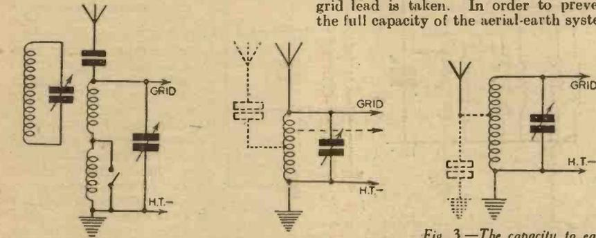
Fig. 1.—The simplest type of tuning circuit. On the right is the diagram relating to a two-range coil.
