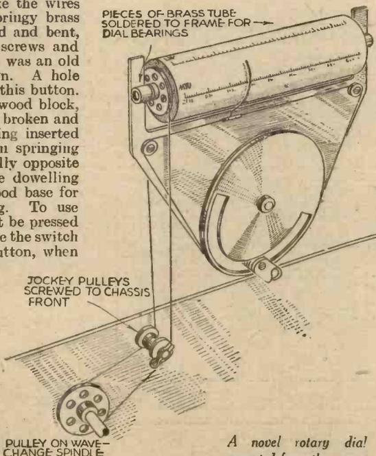
A novel rotary dial operated from the wave-change spindle.
