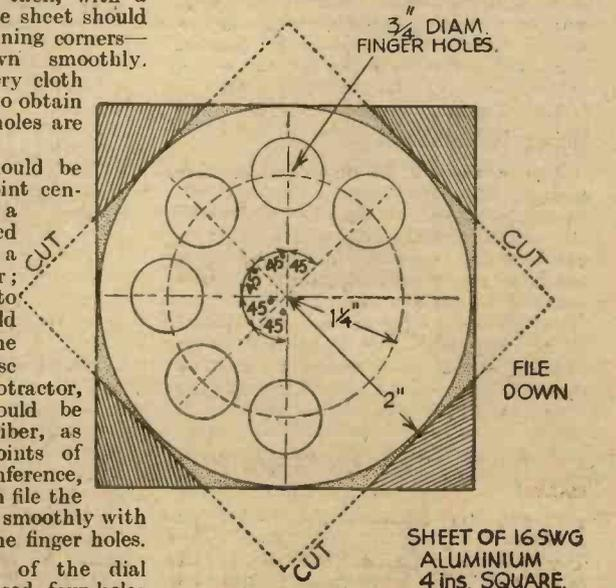
Fig. 4.—How to mark out and cut the dial.
