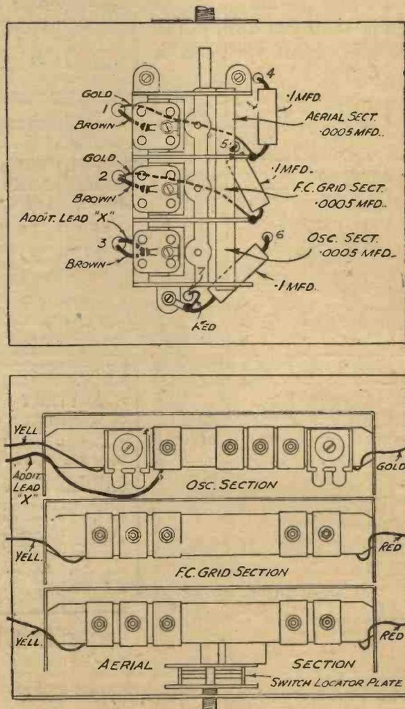
Fig. 5.—Details of the wiring above and below chassis.
