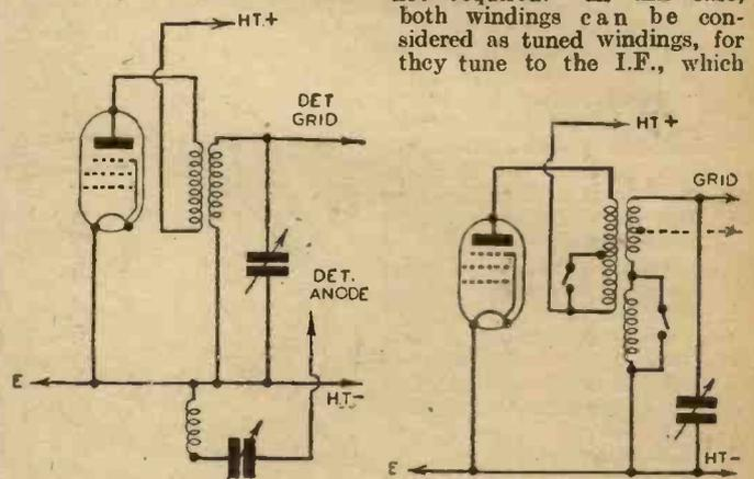
Fig. 4.—A double-wound coil used for tuned-transformer coupling. Reaction connections are also shown.
