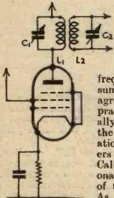
Fig. 17.—Standard I.F. transformer connections.
