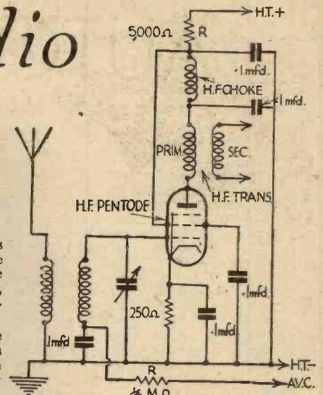
A typical circuit for an H.F. amplifier.
