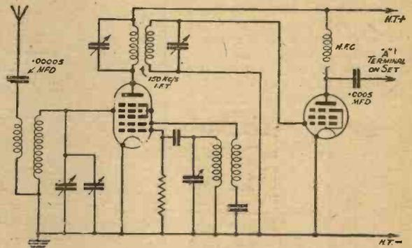
Fig. 5.—Skeleton diagram of a converter for use with a broadcast superhet. It incorporates both frequency-changer and I.F. valves.
