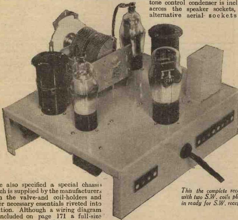
This the complete receiver, with two S.W. coils plugged in ready for S.W. reception.
