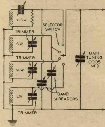
Fig. 7.—A comprehensive all-wave tuning circuit, showing how to incorporate all refinements as mentioned in this article.
