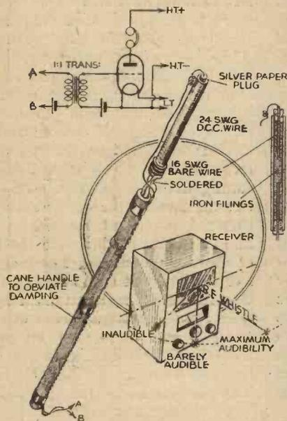
A novel tester rod for detecting resonance.
