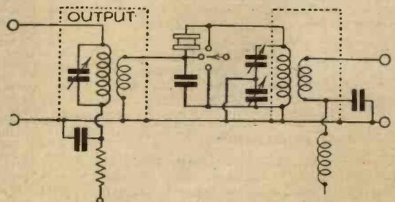
Fig. 2.—A crystal gate and variable selectivity filter.
