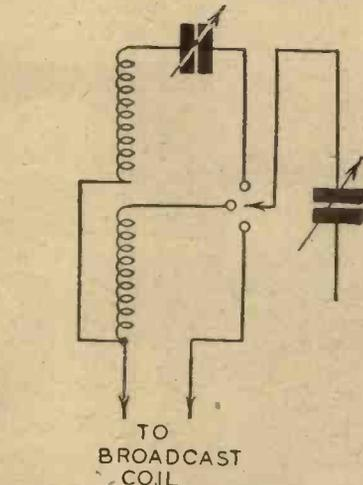
Fig. 5.—Efficiency on the ultra-short wavelengths may be increased by including a small capacity in series with the ultra-short-wave coil.
