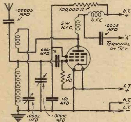
Fig. 1.—Circuit of a typical autodyne (single valve) S.W. superhet converter.
