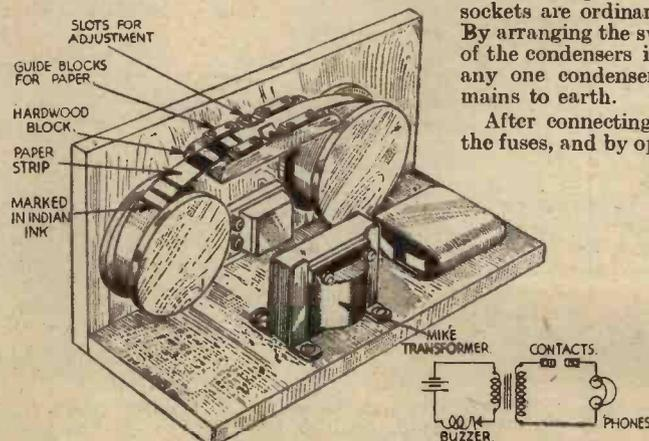
Pictorial view and circuit diagram of a simple automatic Morse transmitter.
