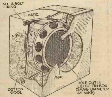
An effective method of mounting a microphone to avoid "boom" effects.
