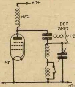
Fig. 1.—Simplest arrangement of tuned-grid coupling.
