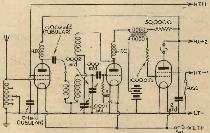
Fig. 3. A conventional untuned H.F. short-wave receiver circuit.
