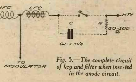
Fig. 5.—The complete circuit of key and filter when inserted in the anode circuit.
