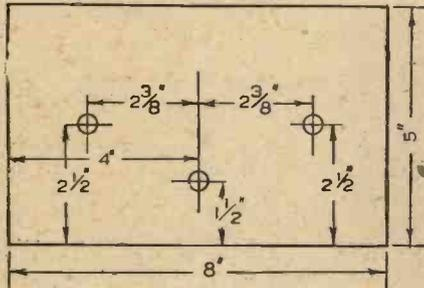
Fig. 3.—Panel-drilling dimensions.
