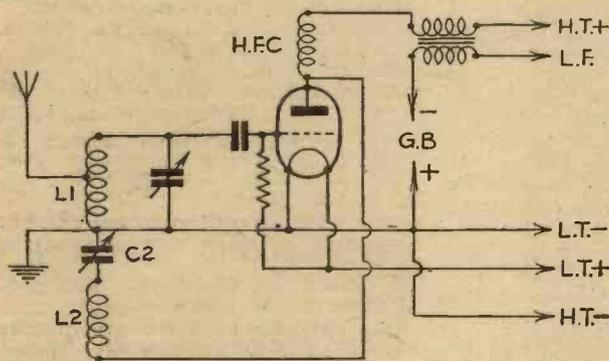
Fig. 1.—A typical cumulative grid detector circuit.
