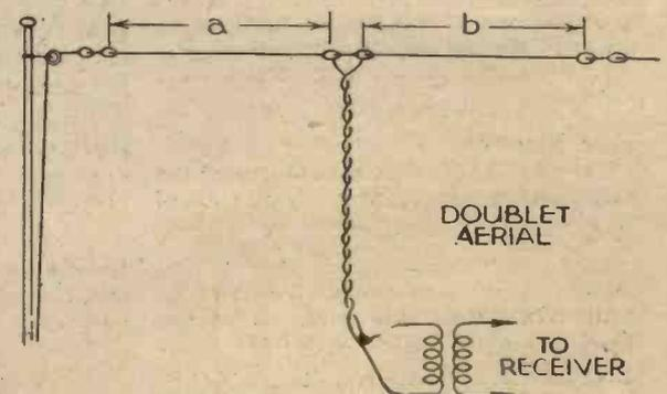
Fig. 3.—An efficient doublet aerial. Lengths a and b are equal to 1/4 wavelength depending on the waveband concerned.
