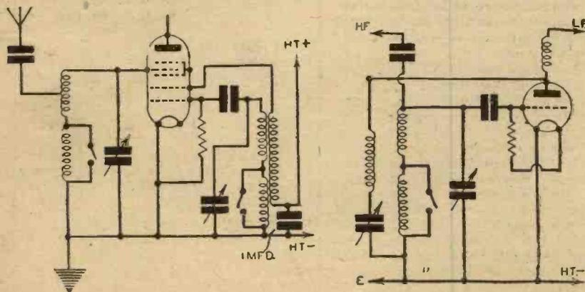
Fig. 6.—Conventional oscillator-coil connections for a pentagrid compared with those for a similar pattern of coil used in a triode detector circuit.
