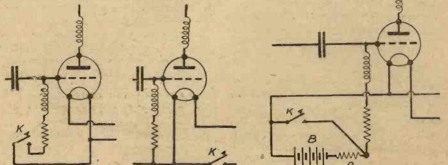
Fig. 4.—Showing various keying arrangements for battery-operated valves, the key being at safe potential.
