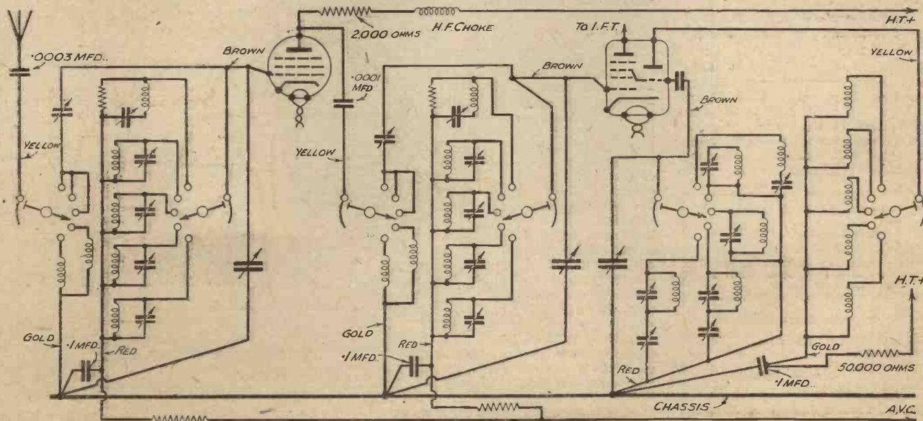
Fig. 2.—Theoretical diagram of the tuner. Note that various earth connections are made to single points to keep the circuits separate.
