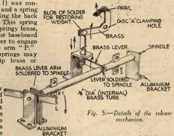
Fig. 5.—Details of the release mechanism.
