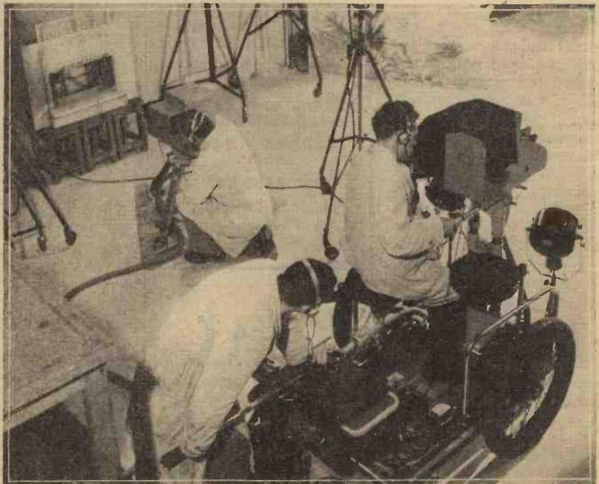
This illustration shows how the television cameras are used to relay both the actual artists and small models which are 'mixed' to provide most realistic effects. The small model provides the proscenium and the raising of the curtain before the artists appear.
