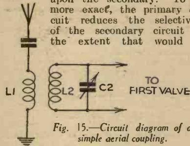
Fig. 15.—Circuit diagram of a simple aerial coupling.
