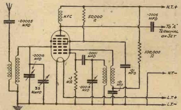
Fig. 3.—A converter circuit using a pentagrid frequency-changer.
