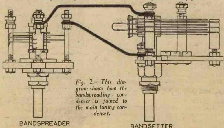
Fig. 2.—This diagram shows how the bandspreading condenser is joined to the main tuning condenser.
