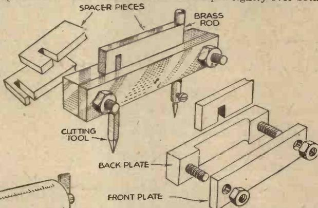
A handy tool for cutting circular holes in speaker baffles or chassis.
