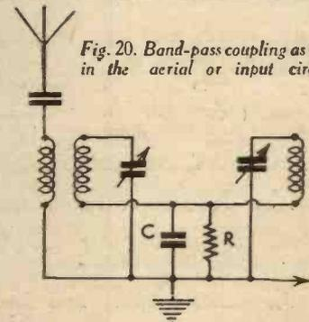
Fig. 20. Band-pass coupling as used in the aerial or input circuit.
