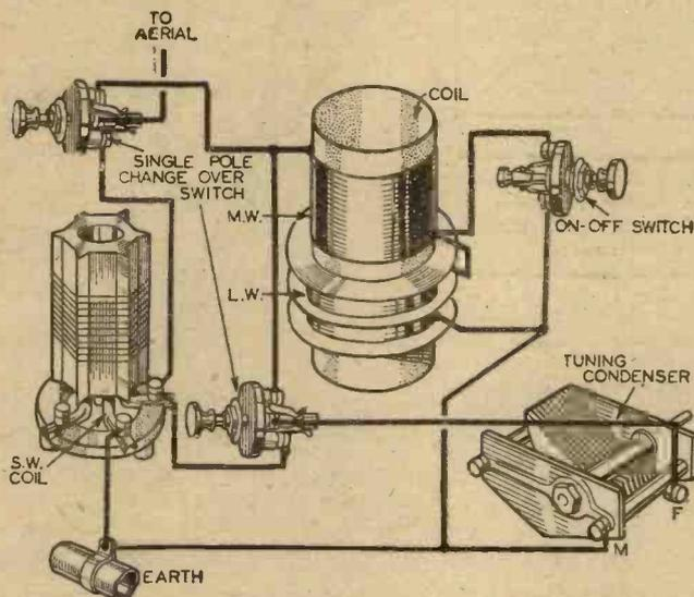
Fig. 1.—The basic arrangement for an all-wave tuning circuit, utilising separate standard components.
