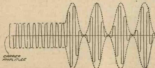
Fig. 3.—Indicating the wave-form when 100% modulation is applied. Note the well-defined maximum and minimum.
