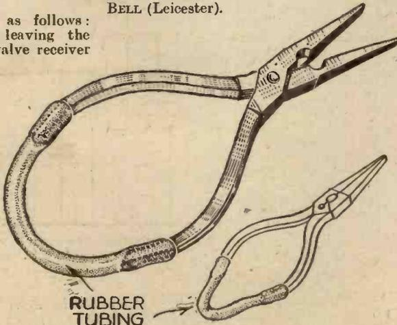
An ordinary pair of pliers can easily be adapted for self-opening by the simple method illustrated.
