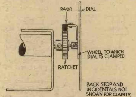
Fig. 3.—The ratchet device which provides the "locator."
