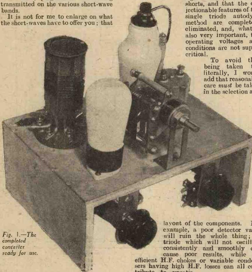
Fig. 1.—The completed converter ready for use.
