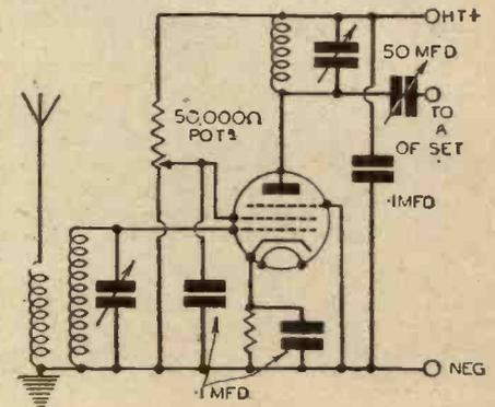
Fig. 3.—Circuit of a pre-H.F. amplifier for a short-wave superhet.
