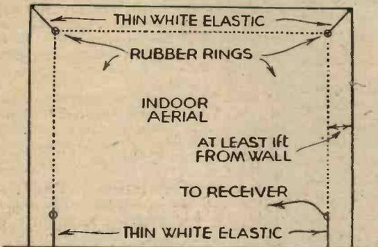
Fig. 1.—An efficient indoor aerial should be arranged as shown here.
