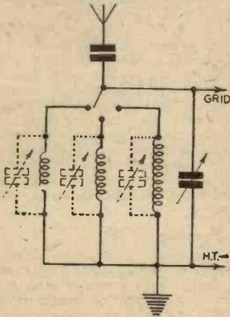
Fig. 7.—A simple method of all-wave tuning by using three separate coils with a three-way switch.
