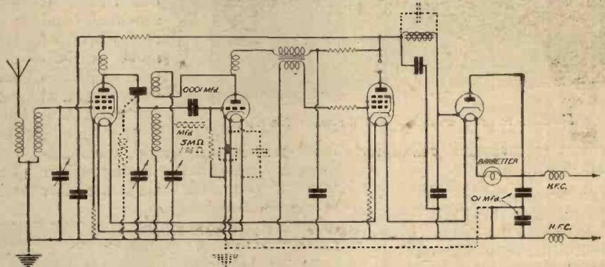
Skeleton diagram of the A.C./D.C. set with which various experiments were carried out with a view to preventing modulation and background hum. Broken lines and figures show the principal changes that proved to be most successful.
