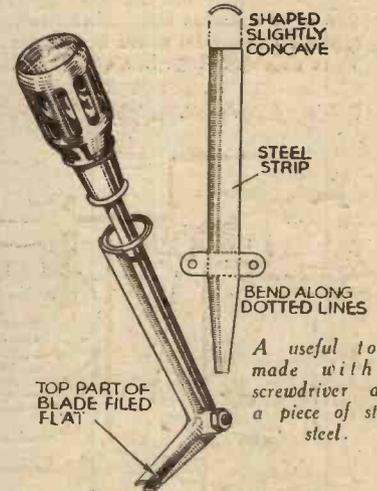
small nut and bolt. This tool will be found useful for such jobs as holding small nuts in place, picking up blobs of solder, etc. With the steel jaw removed the bent driver is handy for removing stubborn valves from their sockets, adjusting trimming condensers, and many other little jobs where an ordinary screwdriver would be useless.—G. H. HUNTER (Ashington).
