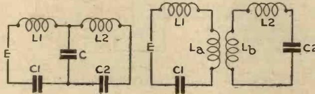
Fig. 12 (left) Two circuits with common coupling impedance.
