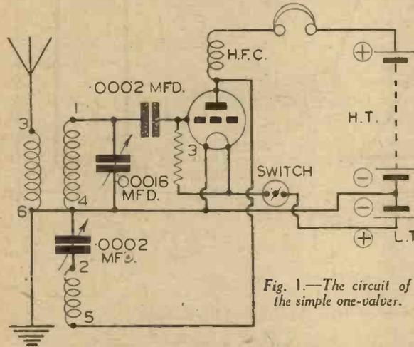
Fig. 1.—The circuit of the simple one-valve.
