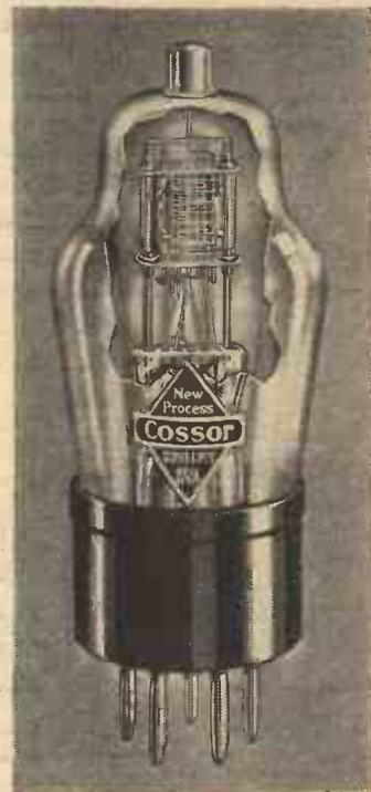
The new Cossor 220 I.P.T. is a special Pentode Detector Valve designed for use in Battery Receivers. Due to its indirectly heated cathode it has remarkable anti-microphonic properties even under very adverse conditions. It is, therefore, particularly suitable for use in Portable Receivers where high L.F. gain is usually provided. The base used on the 220 I.P.T. is of the 7-pin type with standard H.F. Pentode connections.
