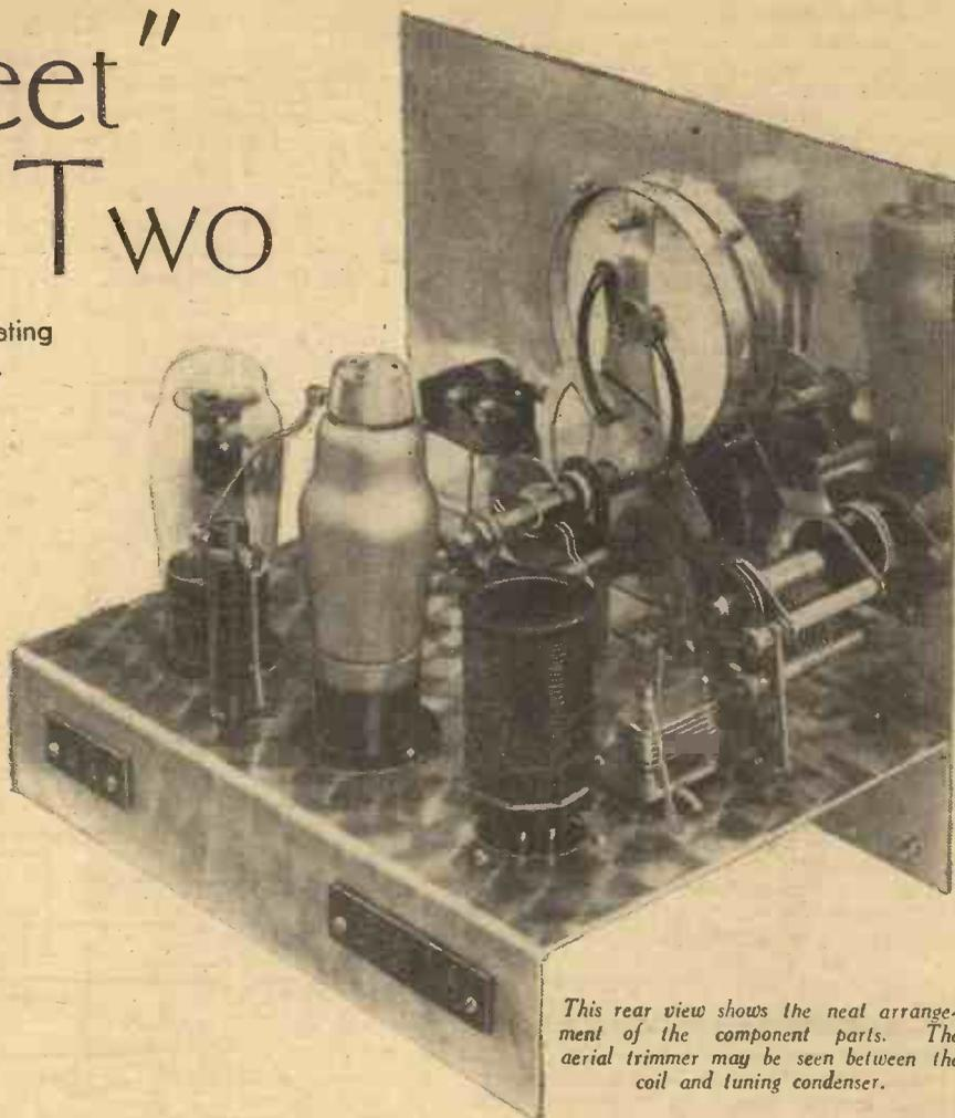
This rear view shows the neat arrangement of the component parts. The aerial trimmer may be seen between the coil and tuning condenser.
