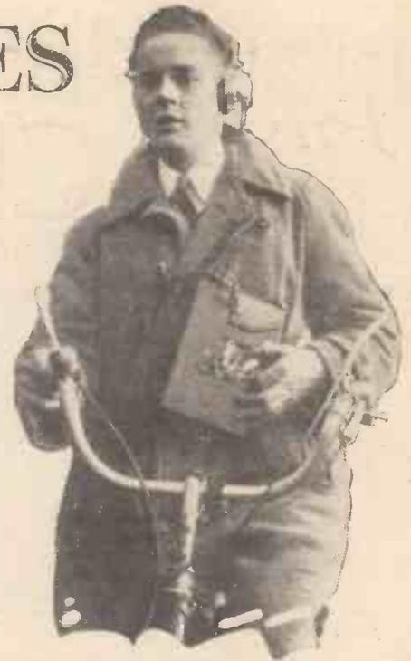
A self-contained two-valve headphone receiver, built by Mr. C. R. Pritchard.
