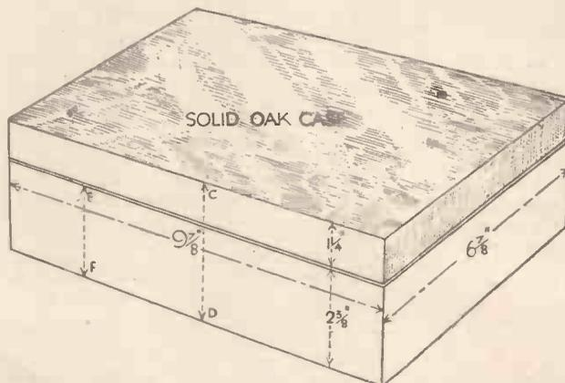
Fig. 4.—The meter may be housed in a simple wooden case, and a suitable design may be made up as shown here.
