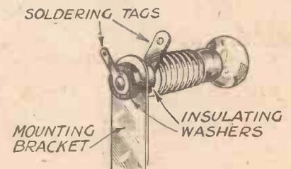
Fig. 3.—A pilot or dial lamp-holder is often the cause of crackling noises.
