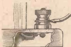
Fig. 2.—If a terminal is tightened too severely the bolt may be loosened causing crackles by the loose internal connection.
