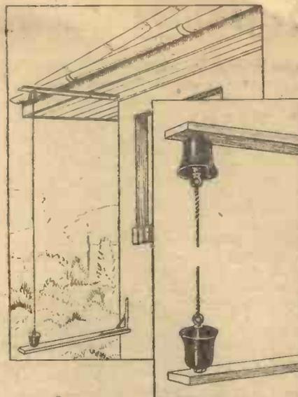
Fig. 5.—A useful short-wave aerial may be erected as shown here. Ideal where there is limited garden space.
