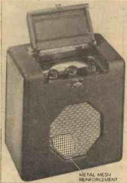
Fig. 1.—The Roberts portable, in which the complete receiver unit is removable.
