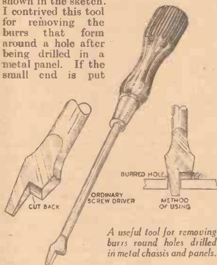
A useful tool for removing burrs round holes drilled in metal chassis and panels.
