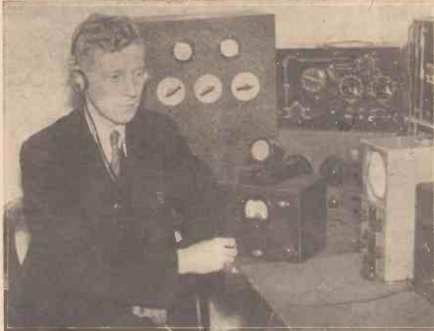
A well-known Welsh radio amateur, G. R. Silverthorne, of Abertillery, has made a transmitter suitable for working in a car for Air Raid Precaution exercises. It is only nine inches by eight by eight, and has been used in conjunction with the Abertillery A.R.P. tests. It was demonstrated to a Home Office expert in Cardiff recently. Our illustration shows Mr. Silverthorne testing his set.
