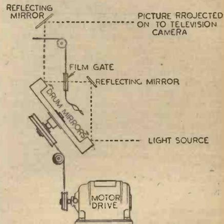
Fig. 2.—The light and picture paths shown simply for the film projector used in television transmission.
