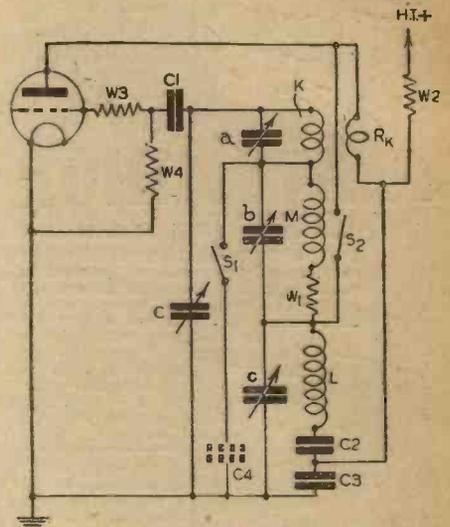
Fig. 1.—The oscillator circuit of a superhet receiver.
