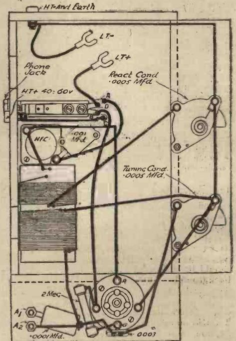
Fig. 3.—Wiring diagram of this compact little portable.
