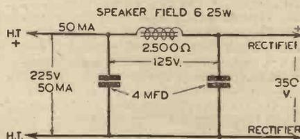
Fig. 3.—How a speaker field winding can be energised in an A.C. receiver.
