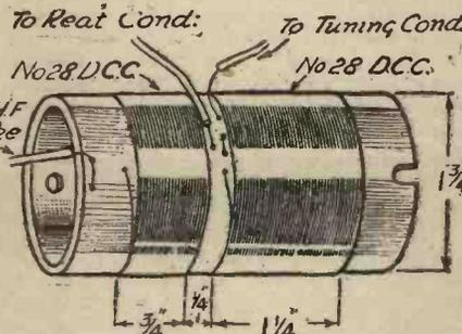
Fig. 1.—Winding details and connections for the coil.
