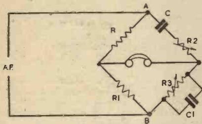
Fig. 1.—Original bridge circuit.
