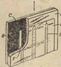
front or rear surface and is secured to the back-plate B of glass, metal, synthetic material, etc., by a raised border C, for example, of Chatterton's compound. The back-plate, if of glass, is rendered opaque or translucent except along strips F lying behind the wave-band scales E through which a luminous tuning spot or pointer moving behind the rear plate may be seen. The several wave-band scales E and lists of station names D may be differentially coloured.
