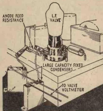
Fig. 2.—The output of a stage, or the audio voltage developed across the load resistance may be measured as shown here.
