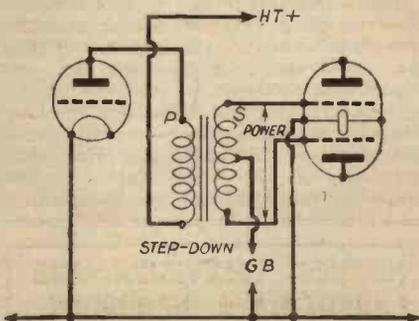
*A class B transformer steps down, because the valve is power operated;*
