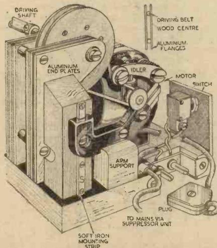
A coil-winding machine utilising an electric motor as fitted to a domestic sewing machine.
