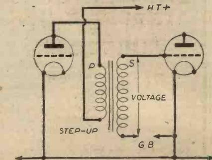
*an ordinary L.F. valve is voltage operated.*
