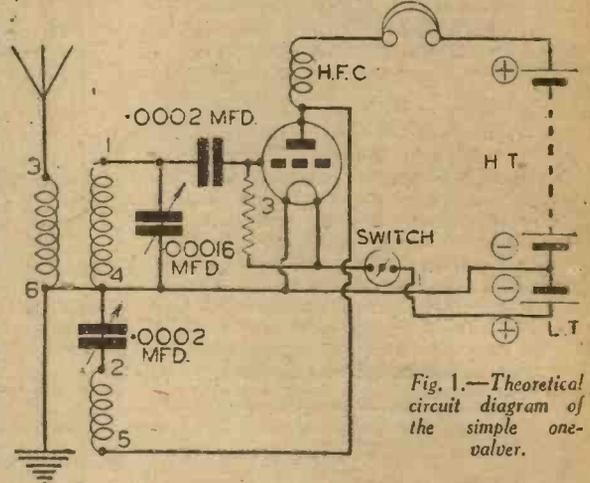
Fig. 1.—Theoretical circuit diagram of the simple one-valver.
