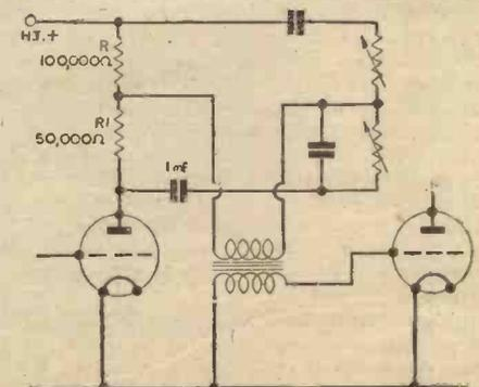
Fig. 5.—The filter used for intervalve coupling.
