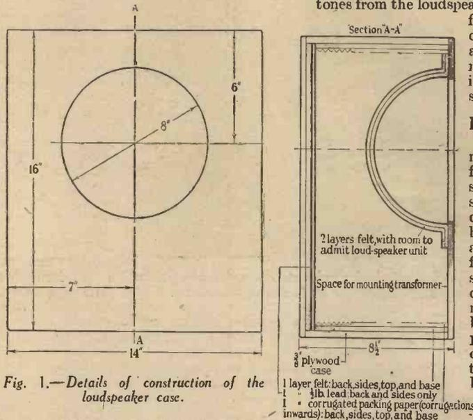
Fig. 1.—Details of construction of the loudspeaker case.
