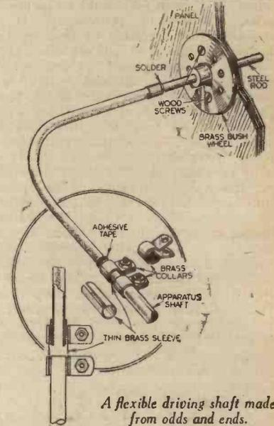
A flexible driving shaft made from odds and ends.
