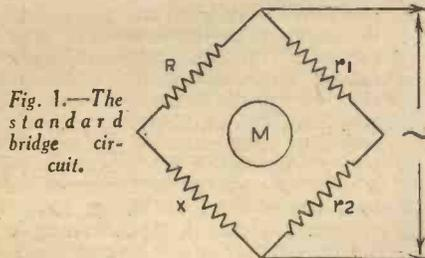
Fig. 1.—The standard bridge circuit.
