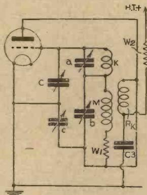
omitted for the sake of simplicity. It will be seen that an inductive feedback occurs between the feedback coil  $R_k$  and the grid circuit coil  $K$ . The circuit elements  $M, W, L$  and  $C_2$  of Fig. 1 are in parallel with the condenser  $C_3$  in the S.W. setting, and are, therefore, in effect inoperative and not shown in Fig. 2.
