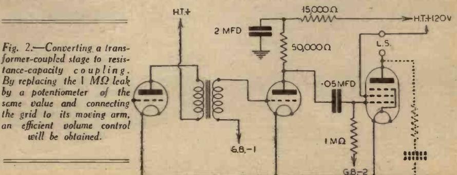
Fig. 2.—Converting a transformer-coupled stage to resistance-capacity coupling. By replacing the 1 MΩ leak by a potentiometer of the same value and connecting the grid to its moving arm, an efficient volume control will be obtained.
