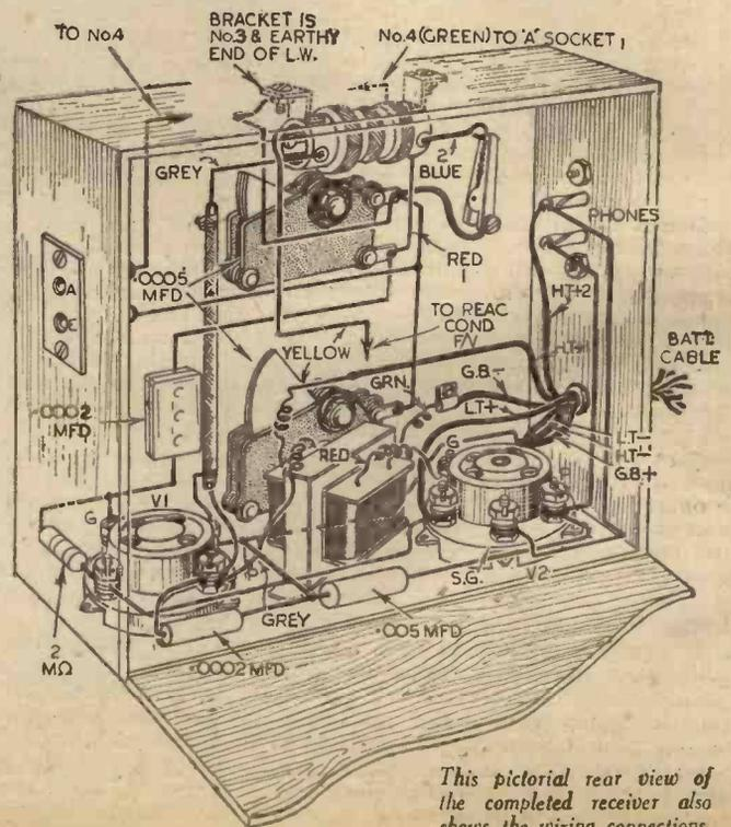
This pictorial rear view of the completed receiver also shows the wiring connections.
