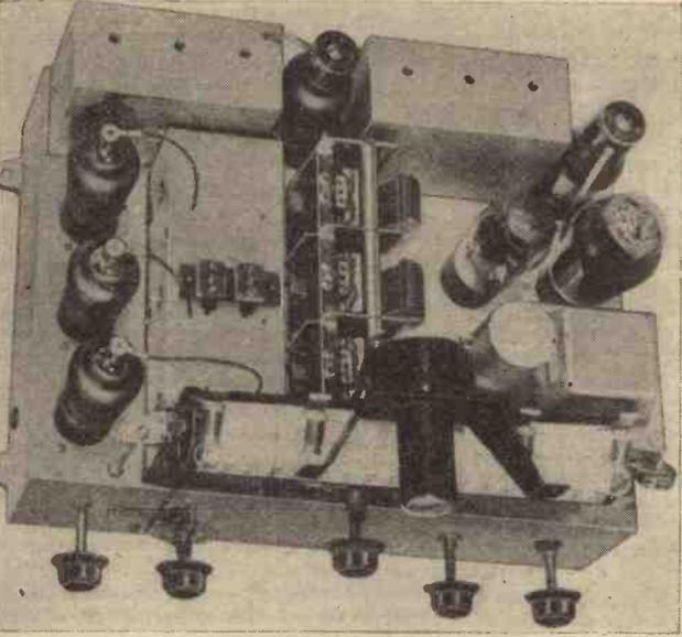
A "bird's-eye" view of the complete E.R.A.7 chassis, with the tuning indicator in position. This picture gives an idea of the screening.
