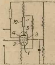
variable resistance or impedance 19 is connected in the circuit of electrode 5 to modify as regards frequency or shift as a whole the level of the curve relating output to input. Specification 508038 is referred to.
