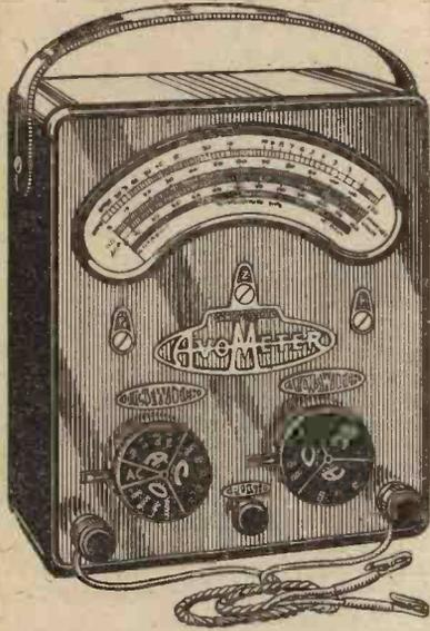
The Avo Test Meter, which has several separate ranges, easily selected by rotary switches.
