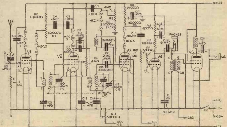
Fig. 1.—Theoretical circuit diagram of the Short-Wave Five.
