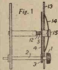
In a remote-control device for a wireless receiver, wherein the tuning element is driven through a flexible shaft from a shaft 2 (Fig. 1) actuated by the tuning knob 1, the tuning indicia are carried on a scale
