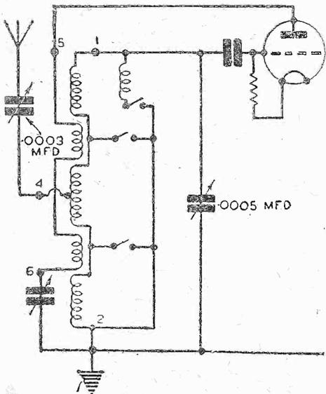
Fig. 1.—Circuit of the Lissen 4-range tuner.
