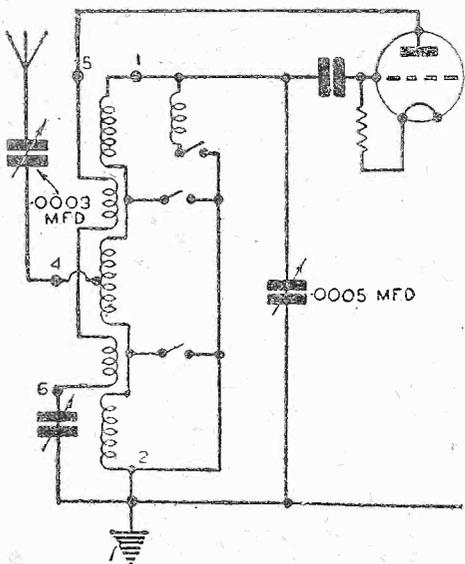
Fig. 1.—Circuit of the Lissen 4-range tuner.
