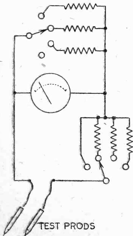
Fig. 1.—Basic principles of a general-purpose test meter.
