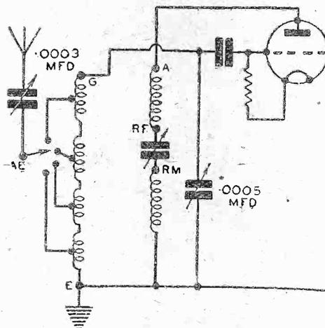
Fig. 2.—This is the original British general tuner.
