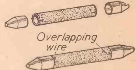
of their compact size. Being a Sunday I could not buy any, so looking in the junk box I picked out a couple of old type grid leaks with holders. I dismantled the leaks by taking off the two metal caps. Inside the tube was a carbon resistance which I took out and replaced with fuse wire overlapping slightly, so that when the caps were replaced they secured the fuse wire. I have since used this type for many different purposes.—K. ARCHER (North Harrow).
