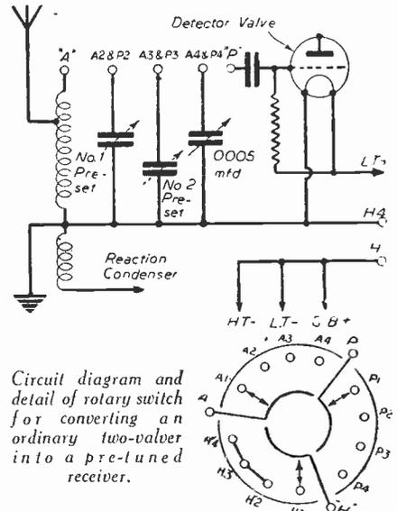
Circuit diagram and detail of rotary switch for converting an ordinary two-valver into a pre-tuned receiver.
