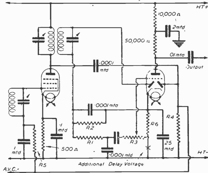
Fig. 6.—An arrangement similar in principle to that shown in Fig. 5, but using mains valves and a double-diode-valve for second detection, A.V.C. and L.F. amplification.
