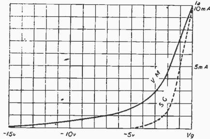
Fig. 1.—A representative  $I_a-V_g$  curve for a variable-mu valve. It shows that the "slope" is reduced with increasing negative bias. A broken line shows a corresponding curve for a "plain" S.G. type of valve.
