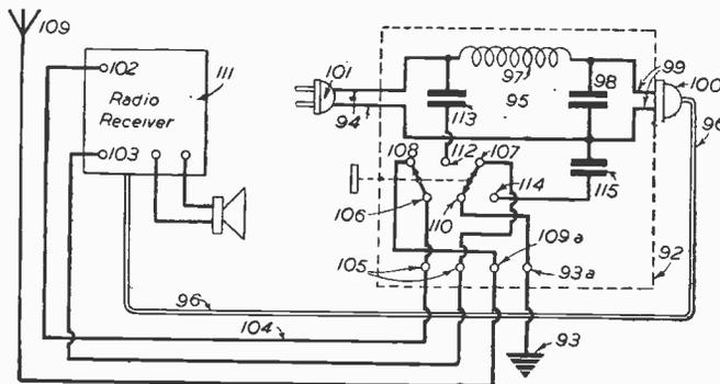
valve serves as output valve and oscillator valve, no switching of the control grid circuit is required, and since in the case of the screen-grid output valve the oscillatory tuned circuit may be maintained in circuit for audio-frequency amplification, the switching is simplified.
