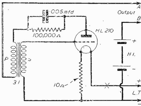
Fig. 1.—The oscillator circuit.
