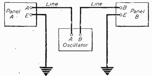
Fig. 3.—Two-way send/receive working connections.
