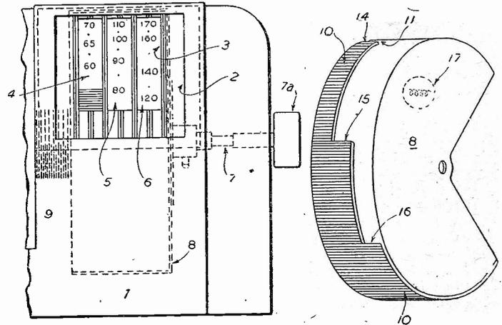
Fig. 1.—A corner of a cabinet, showing the new tuning indicator. Fig. 2.—(Right) A hollow drum segment.
