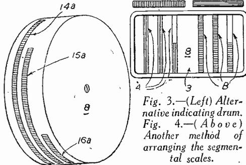
Fig. 3.—(Left) Alternative indicating drum. Fig. 4.—(Above) Another method of arranging the segmental scales.
