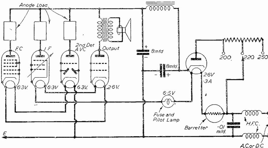
Fig. 4.—This skeleton circuit shows the arrangement of the heater wiring and rectifier connections in a typical superhet receiver of the AC/DC type. The tapped resistor in the anode circuit of the rectifier is not always necessary, and the combined break-circuit fuse and pilot lamp is an optional fitting.
