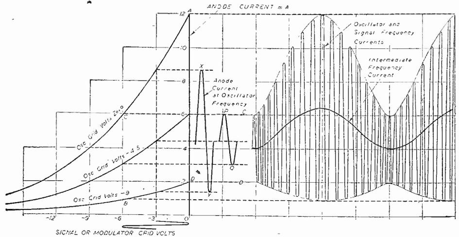
Fig. 2.—Graphical representation of action of octode frequency changer.
