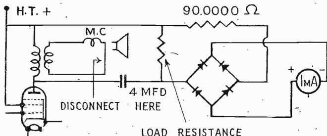
Westinghouse instrument-type rectifiers may be used up to frequencies of more than 100 kCs, and enable a simple and robust output meter to be constructed for such purposes as assisting trimming, measuring frequency response, etc. Full details for constructing such a meter are given in descriptive pamphlet No. 11b/1.
