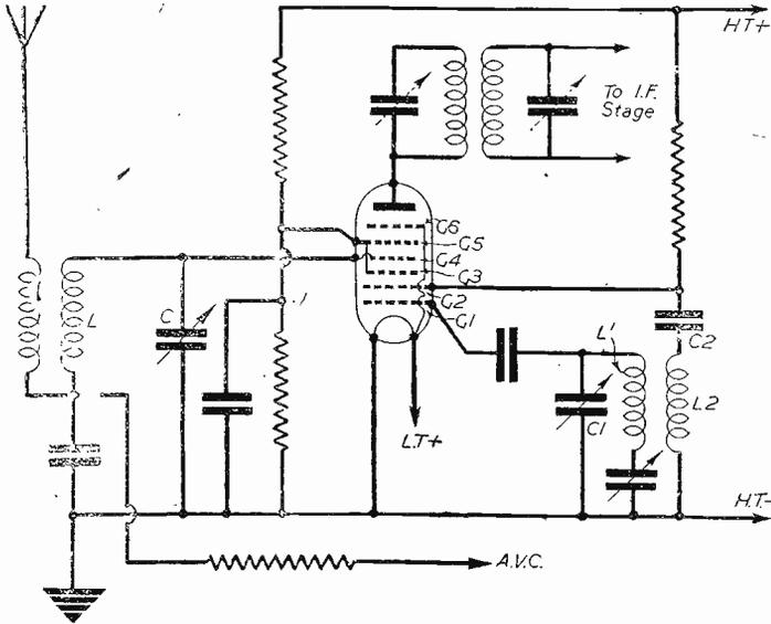
Fig. 1.—Circuit of octode frequency changer.
