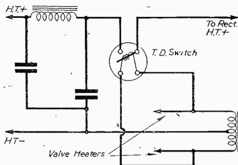
Fig. 1.—Connections for a thermal-delay H.T. switch. The heating resistance may be fed from the valve-heater winding of the transformer, as shown, or from the rectifier-heater winding, when this is provided.
