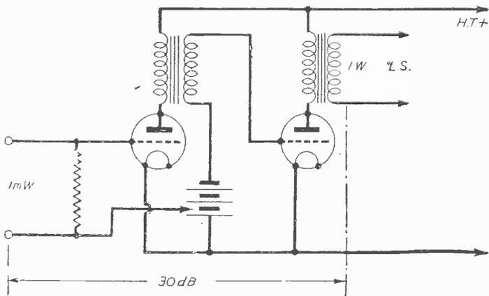
Fig. 1.—This outline diagram of a simple amplifier shows the relationship between power amplification and decibel gain.
