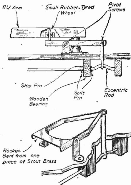
Details of an efficient pick-up lifting device.
