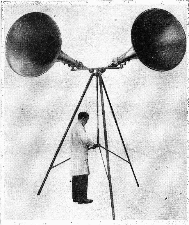
Fig. 1.—Large projector loudspeaker mounted on a tripod in order to "cover" a very large crowd.
