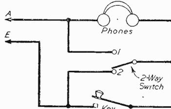
Fig. 2.—Extension panel circuit.
