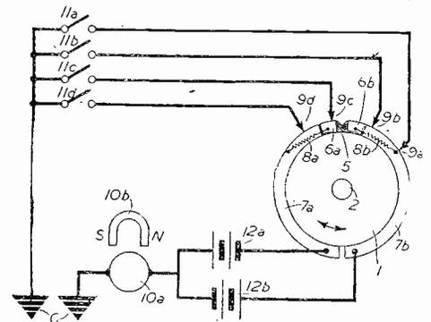
Fig. 2.—A selector system incorporating a reversible electric motor.
