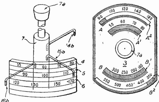
Fig. 5.—Cursors mounted on the control shaft.
