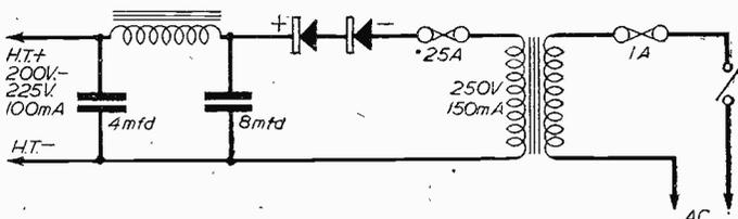
Fig. 2.—Connections for a half-wave metal rectifier, such as the Westinghouse type H.T. 17, which has an unsmoothed output of 225 volts, 100 mA.
