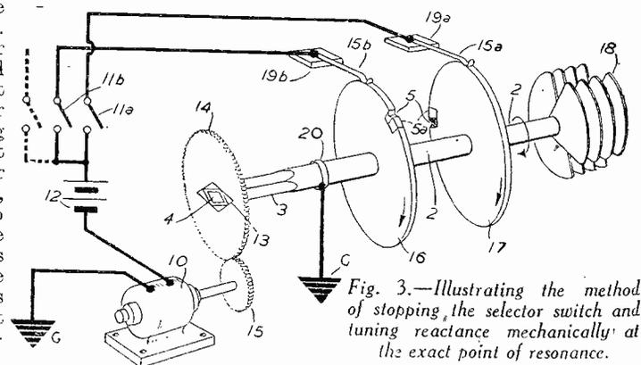
Fig. 3.—Illustrating the method of stopping the selector switch and tuning reactance mechanically at the exact point of resonance.
