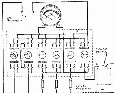
Method of using a push-button unit in connection with a universal meter.
