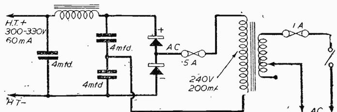
than that which is required as D.C. output. In the example shown in Fig. 2, the output is taken as being in the region of 225 volts (before smoothing) at 100 mA, whilst the required output from the transformer is 250 volts at 150 mA. These figures are those given by the makers for the Type H.T.17.
