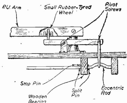
Details of an efficient pick-up lifting device.
