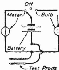
meter. To test the wiring of sets use the bulb by switching to the bulb on the panel. The battery is of the flat type 4.5 volts.—A. G. S. COBB (Tamworth).
