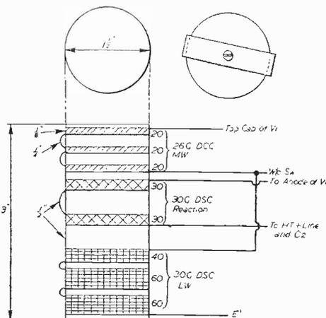
Fig. 2.—Coil former and windings.
