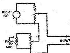
Fig. 4 (Left).—Shows how the mixer circuit was wired.
