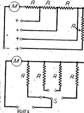
Fig. 4.—How to arrange the separate resistances to provide alternative readings.
