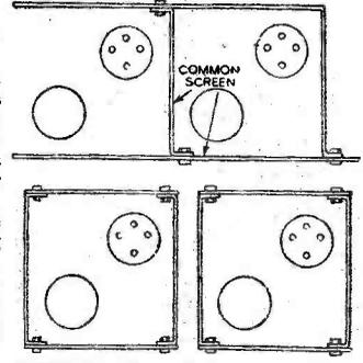
Fig. 7.—Correct and incorrect methods of screening sections of a highly sensitive receiver.
