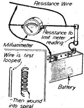
Fig. 3.—Method of making accurate shunts from resistance wire.
