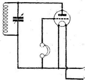
Fig. 2.—A simple form of diode-grid detector circuit.
