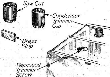
A method of making adjusting knobs for trimming condensers.
