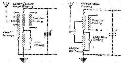
Figs. 7 and 8.—Showing alternative methods of improving selectivity by tapping into the aerial coil.
