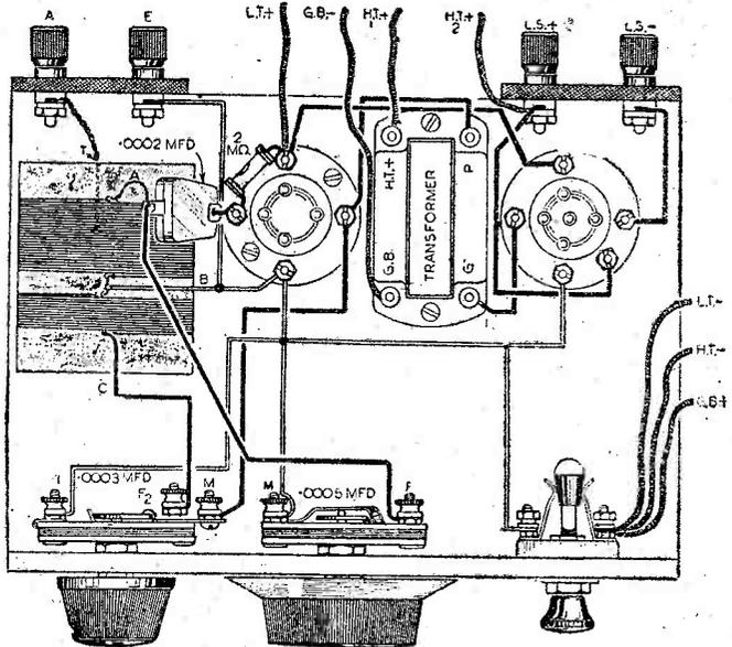
Fig. 3.—Wiring diagram of the Rapid Two.
