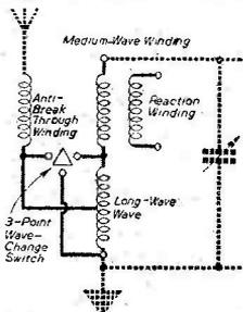
Fig. 11.—One method of connecting the anti-breakthrough choke.
