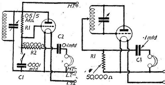
Figs. 3 and 4.—Modifications of the diode-grid detector circuit shown in Fig. 2.
