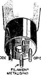
Fig. 6.—(Right) In wiring a battery receiver it is wise to ensure that the filament pin to which the metallising is joined is earth-connected.
