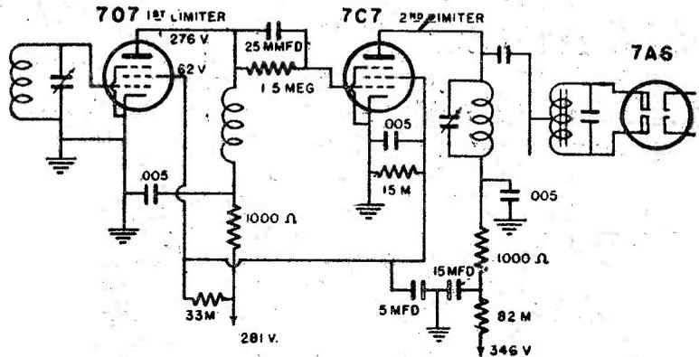
Two pentodes, capacity coupled, are used in the double limiter circuit of the Zenith models. The 7A double-diode discriminator-demodulator is shown on right.
