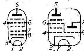
Fig. 5.—Diagrams of a pentagrid or heptode (left) and a triode-hexode (right). The electrodes are: 1 and 2, heater; 3, cathode; 4, signal grid; 5, main anode; 6, screening grids; 7, oscillator anode; 8, oscillator grid.
