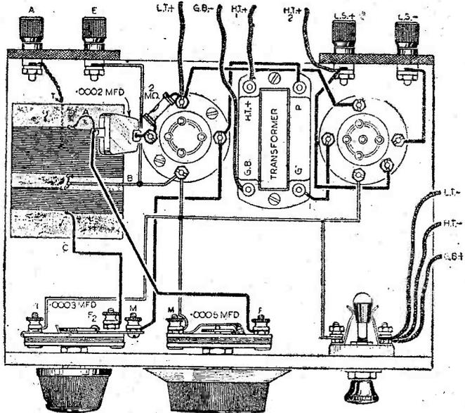
Fig. 3.—Wiring diagram of the Rapid Two.
