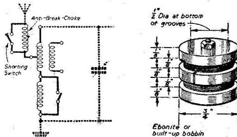
Figs. 12 and 13.—The choke is cut out on medium waves when it is wired as shown by diagram on left. The constructional details of the choke are shown on right.
