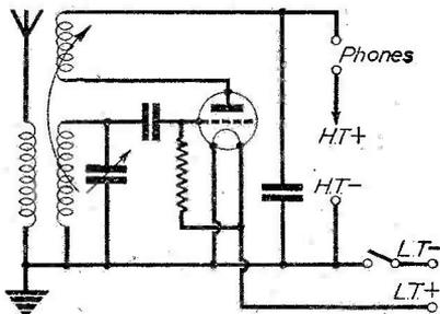
Fig. 1.—The earliest form of inductively-coupled reaction circuit. Its advantages were neutralised by its inherent defects.
