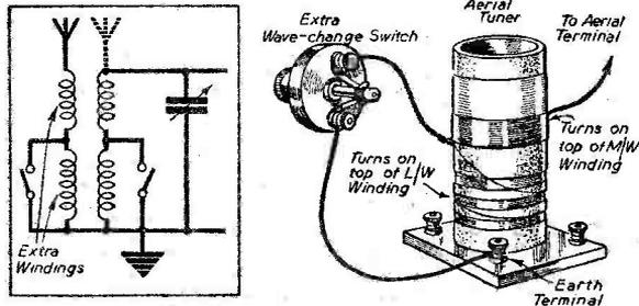
Fig. 9.—Adding aerial coupling coils, as shown here, also improves matters, especially when separate windings are used for M. and L. waves.]
