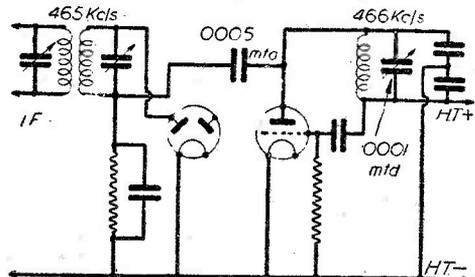
Fig. 5.—A method of using a triode heterodyne oscillator in conjunction with a diode or double-diode second detector in a superhet. The diode circuit is shown in skeleton form only in the interests of simplicity.
