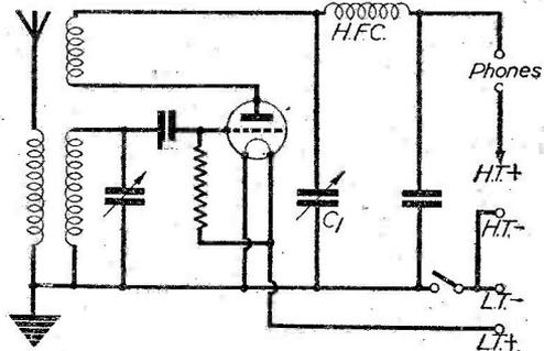
Fig. 3.—Here is a circuit favoured by many S.W. enthusiasts. It uses what is known as "throttle control."
