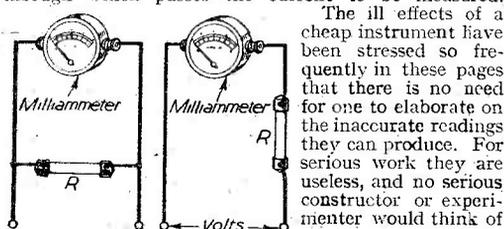
Figs. 1 and 2 show the method of connecting shunts and series resistances for multiplying the range.
