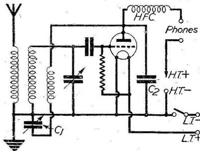
Fig. 2.—The standard Reinartz circuit in which the reaction coil is fixed and the control obtained by the variable condenser C.1.
