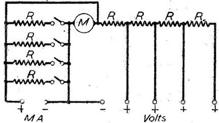
Fig. 5.—Complete circuit of the all-purpose meter as described.
