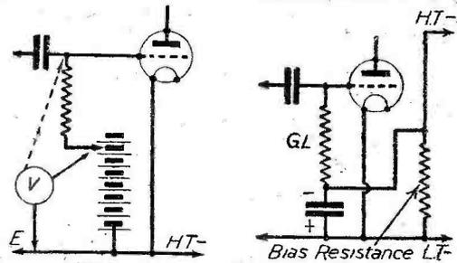
Fig. 3.—Full lines indicate the voltmeter leads when measuring the bias voltage in a battery set. There may not be any reading when the meter is connected as shown by the broken line.
