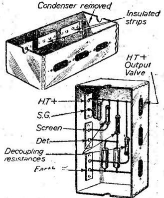
A H.T. distributor unit devised from an old ganged-condenser case.
