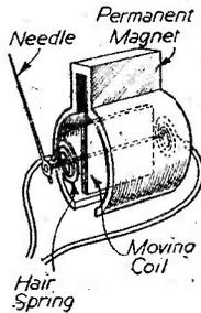
Fig. 1.—The basic moving-coil meter movement, using a specially shaped magnet.
