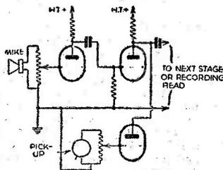
Fig. 5.—This is how the amplifier circuit was modified when the moving-coil "mike" was used. This arrangement provides a very satisfactory method of levelling up the amplification of the two inputs.
