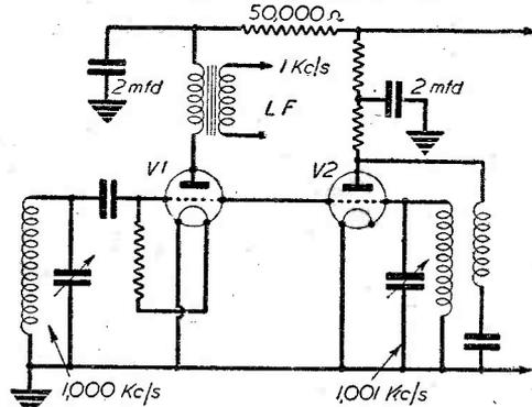
Fig. 4.—A separate oscillator (V.2) used in conjunction with a triode detector or second detector (V.1) to produce a C.W. note at audio-frequency.
