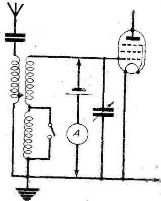
Fig. 5.—A simple method of measuring the resistance of a tuning coil set to medium and long waves.
