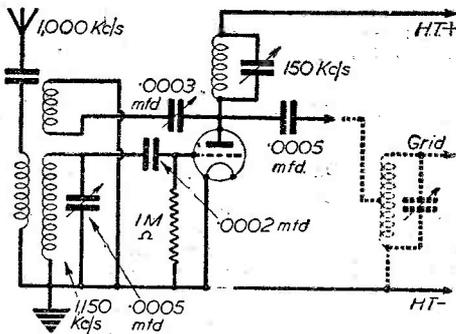
Fig. 3.—A form of oscillating first detector of the type at one time fairly widely used as a superhet converter in conjunction with a "straight" receiver.
