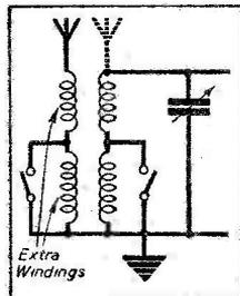
Fig. 9.—Adding aerial coupling coils, as shown here, also improves matters, especially when separate windings are used for M. and L. waves.]
