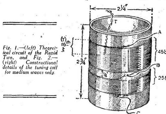
Fig. 1.—(left) Theoretical circuit of the Rapid Two, and Fig. 2.—(right) Constructional details of the tuning coil for medium waves only.
