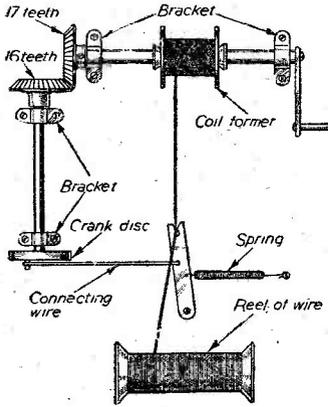
An improved winder for honeycomb coils.
