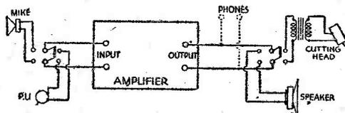
Fig. 3. (Top).—The switching used for the recording amplifier.
