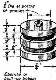
Figs. 12 and 13.—The choke is cut out on medium waves when it is wired as shown by diagram on left. The constructional details of the choke are shown on right.
