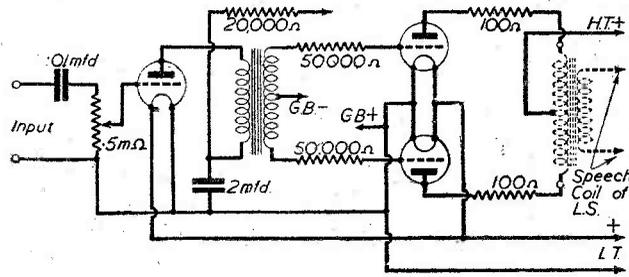
Fig. 2.—The Class A push-pull amplifier circuit, which is intended for good quality reproduction rather than high gain.
