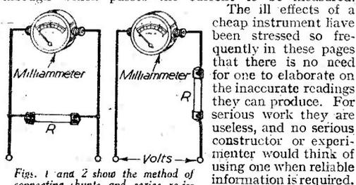
Figs. 1 and 2 show the method of connecting shunts and series resistances for multiplying the range.
