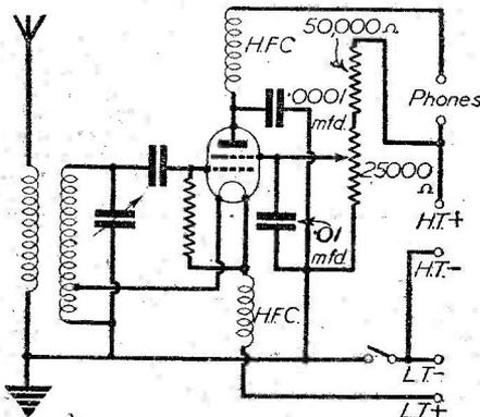
Fig. 4.—One of the most efficient reaction circuits for S.W. work, using the "electron-coupled" system.
