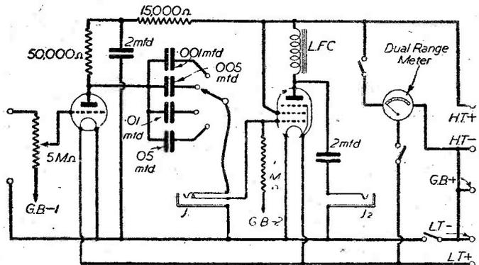
Fig. 2.—The battery-operated amplifier which 2CHW is building to complete his Rx. Note the tone control arrangement.
