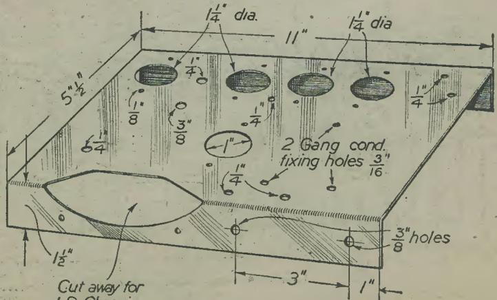
Fig. 2.—Chassis diagram showing positions of holes for valveholders, etc.
