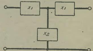
Fig. 5.—A “T” section filter in which *X*<sub>1</sub> and *X*<sub>2</sub> represent reactors of opposite kind.
