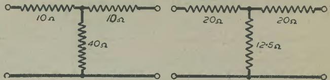
Fig. 3.—Both of these arrangements will match into a 30 ohm load, but the one will give greater attenuation.
