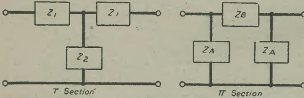
Fig. 1.—“T” and “π” section filters or attenuators. These form the most widely used arrangements.
