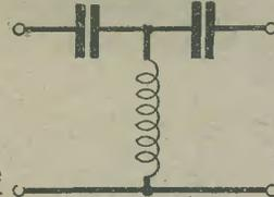
Fig. 9.—A high-pass filter arrangement.
