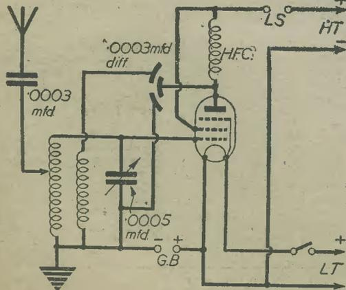
Fig. 2.—An anode-bend detector arrangement, which utilises a steep-slope pentode.
