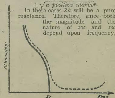
Fig. 10.—The curve produced by a well designed high-pass filter.
