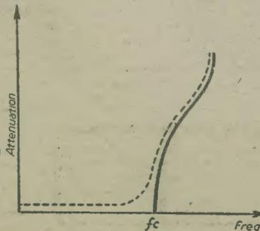
Fig. 8.—The behaviour of the low-pass filter shown in graphical form.
