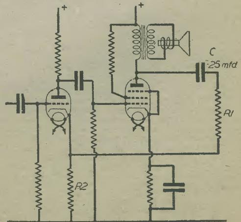
Fig. 2.—A suitable method when R.C. coupling is in use.
