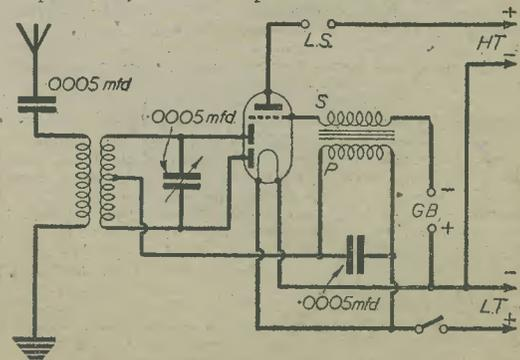
Fig. 3.—Using a D.D.T. valve as diode detector and triode L.F. amplifier.
