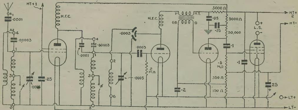
Fig. 14.—The theo. of the £5.5s. Battery Four, blueprint No. W.M. 381. This is a good general purpose dual-range receiver.
