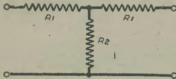
Fig. 2.—A “T” section attenuator in which  $R_k = \sqrt{R_1^2 + 2R_1Z}$ .
