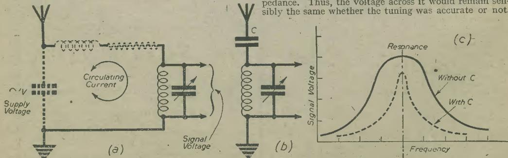
Fig. 1.—Diagrams used to explain the effect of a series aerial condenser on selectivity. (a) Shows the capacity, inductance and resistance of the aerial-earth circuit in parallel with the tuning coil; (b) shows the series aerial condenser, and (c) shows corresponding tuning curves without a series condenser (full line) and with it (broken line).
