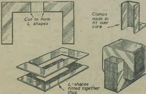
An easily constructed microphone transformer.
