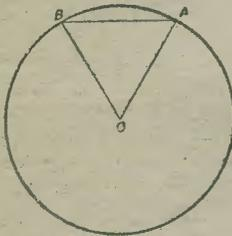
Fig. 1.—Diagram explaining radian.
