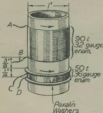
Fig. 3.—Diagram of windings for the coil.
