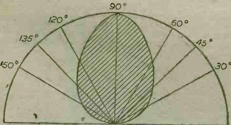
Fig. 8.—Horizontal polar diagram of the broadside array, showing that directivity has been achieved.
