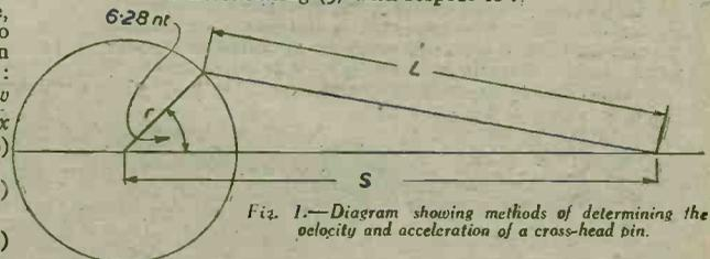
Fig. 1.—Diagram showing methods of determining the velocity and acceleration of a cross-head pin.
