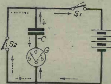
Fig. 1.—Circuit showing the charging and discharging of a fixed condenser.
