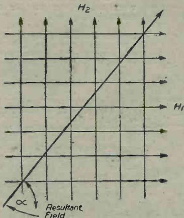
Fig. 18.—Fields produced in the goniometer stator coils and the resultant picked up by the rotor.
