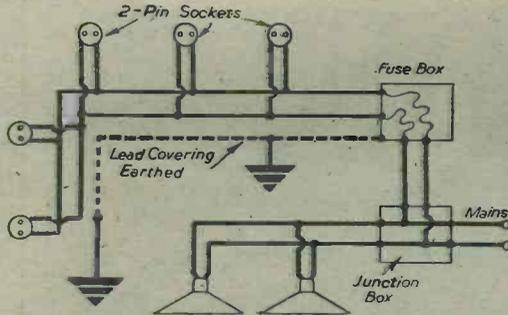
Fig. 4.—The circuits for the supply points and lighting. Note the position of the fuses.
