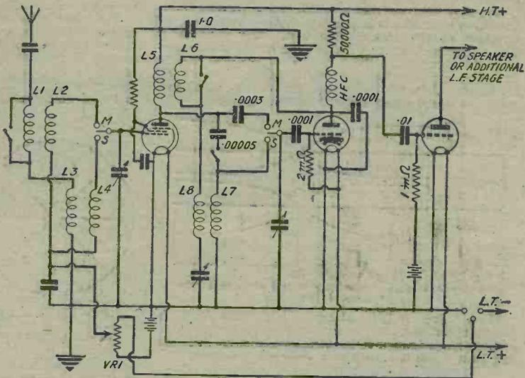
Fig. 4.—If suitable switches are available, this circuit has certain advantages which make it worthy of trial.
