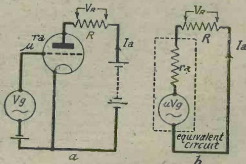
Fig. 2 (a).—The valve circuit with external anode load, and (b) its electrical representation.
