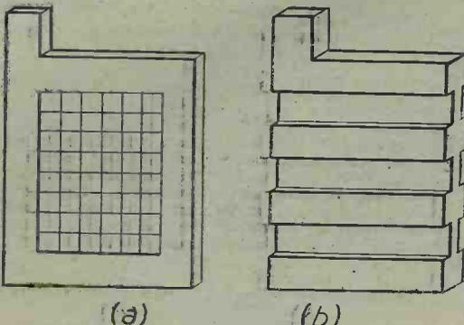
Fig. 2.—Two types of plate formation: (a) Four, or "pasted," and (b) "plated or formed."
