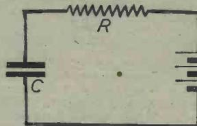
Fig. 2.—In a circuit such as this the time taken for the condenser  $C$  to charge is proportional to the product of the capacity and the series resistance.
