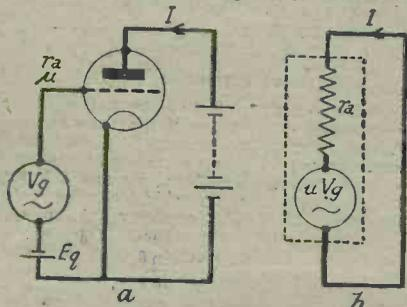
Fig. 1 (a).—A triode without load resistance, (b) its equivalent electrical circuit.
