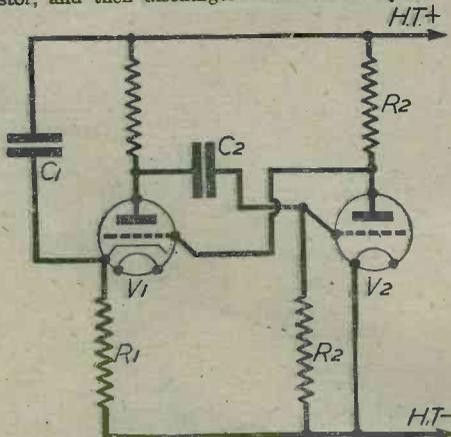
Fig. 5.—A time-base circuit, where the frequency of the "saw-tooth" wave is governed by the condenser C1 and the resistor R1.
