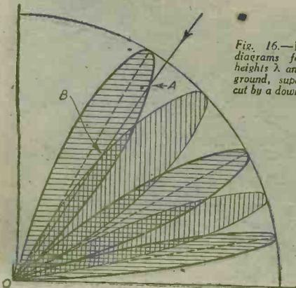
Fig. 16.—Vertical polar diagrams for aerials of heights  $\lambda$  and  $3\lambda/2$  above ground, superimposed and cut by a downcoming signal.
