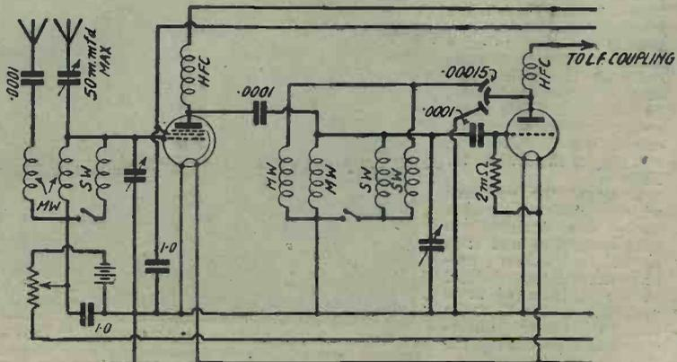
Fig. 2.—The H.F. and detector portion of a similar circuit, but in this arrangement the S.W. coils are connected in parallel with the M.W. sections.
