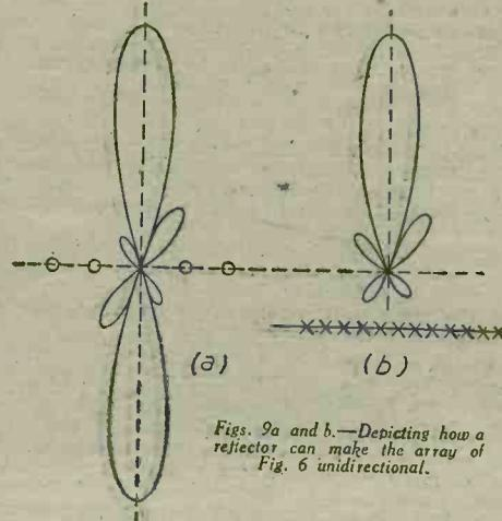
Figs. 9a and b.—Depicting how a reflector can make the array of Fig. 6 unidirectional.
