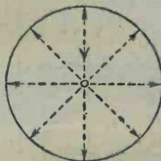
Fig. 3.—Circular polar diagram of a vertical dipole far removed from earth.
