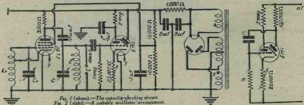
Fig. 1 (above).—The capacity-checking circuit.
