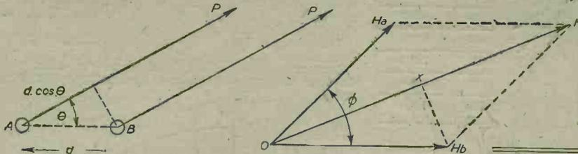
Fig. 6 (left).—Excitation of a two-member broadside array, used to calculate the resultant polar diagram.
