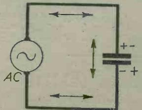
Fig. 3.—When A.C. is applied to a fixed condenser current flows backward and forward round the circuit, as indicated by arrows.
