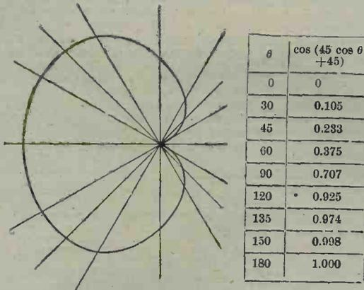
Fig. 10.—Polar diagram (spacing  $\lambda/4$ ) of the end fire aerial array.
