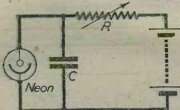
Fig. 4.—A neon oscillator. The neon "strikes" when the voltage on C reaches the "striking" voltage of the neon. The frequency of the "striking" may be governed by adjustment of the variable resistor marked R.
