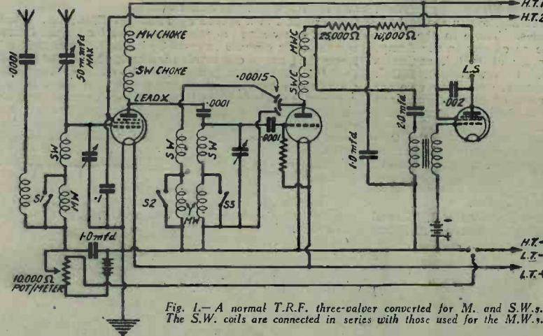
Fig. 1.—A normal T.R.F. three-valve converted for M. and S.W.s. The S.W. coils are connected in series with those used for the M.W.s.
