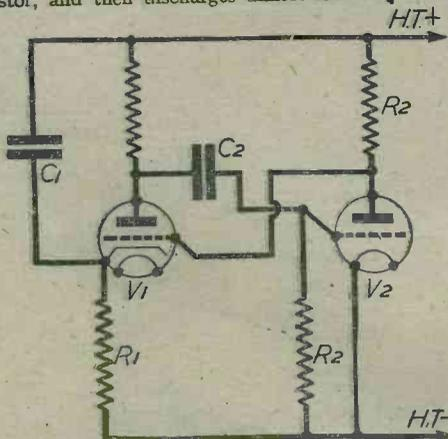
Fig. 5.—A time-base circuit, where the frequency of the "saw-tooth" wave is governed by the condenser C1 and the resistor R1.
