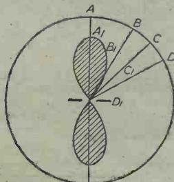
Fig. 4.—Production of the polar diagram of the horizontal dipole, showing the "figure of eight."
