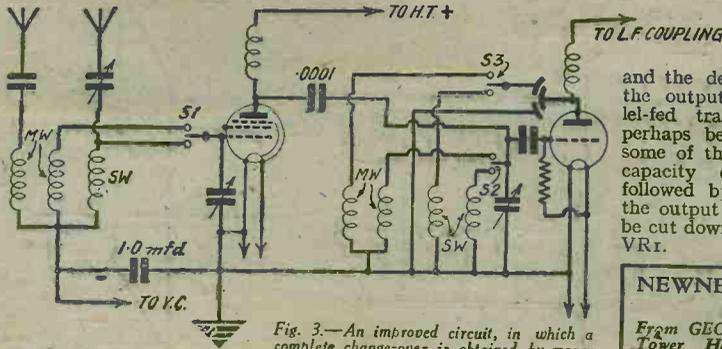
Fig. 3.—An improved circuit, in which a complete change-over is obtained by means of double-throw switches.
