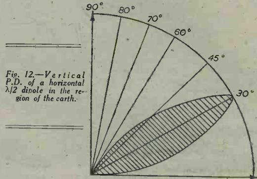
Fig. 12.—Vertical P.D. of a horizontal  $\lambda/2$  dipole in the region of the earth.
