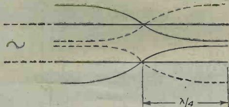
Fig. 1.—Distribution of voltage and current waves on an open circuited line.
