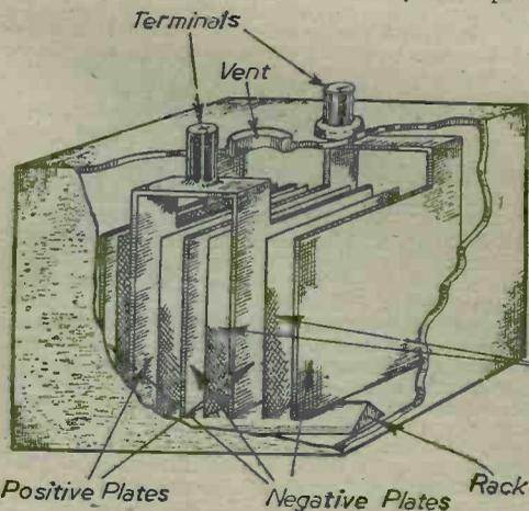
Fig. 3.—The fundamental assembly features of a lead-acid type accumulator.
