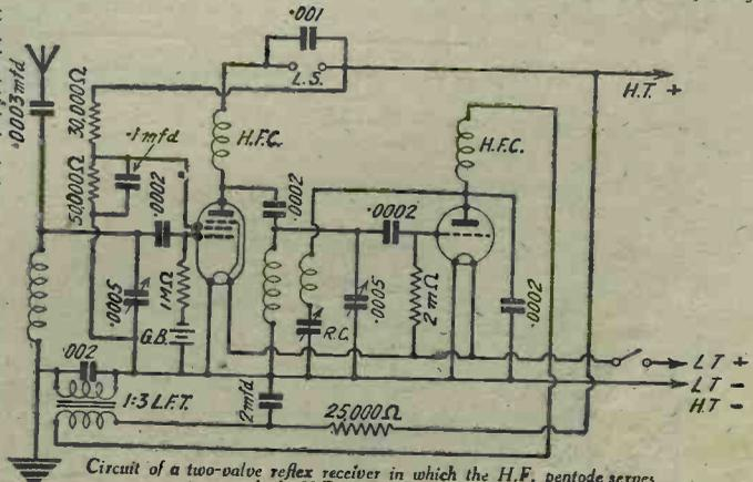
Circuit of a two-valve reflex receiver in which the H.F. pentode serves as both H.F. and L.F. amplifier.
