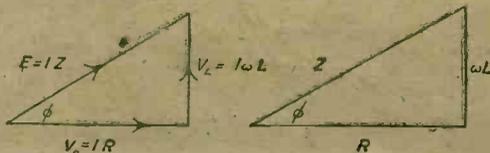
Fig. 12.—Production of the impedance triangle from which is obtained the expression  $Z^2 = R^2 + \omega^2 L^2$ .
