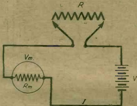
Fig. 1.—The basic circuit illustrating the principle of the ohm/volt meter.
