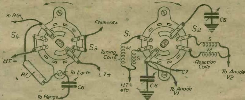
Fig. 6.—Connections to power and wavechange switches.
