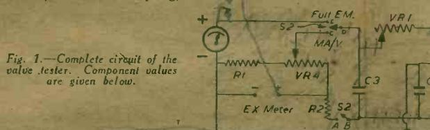
Fig. 1.—Complete circuit of the valve tester. Component values are given below.
