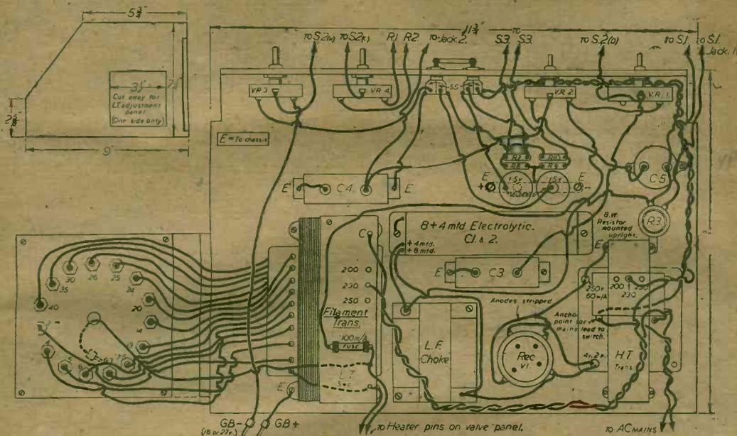
Fig. 4.—Layout and wiring of power unit. The L.T. voltage adjustment panel is accessible from side of panel as shown by the inset.
