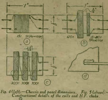
Fig. 4 (left).—Chassis and panel dimensions. Fig. 5 (above).—Constructional details of the coils and H.F. choke.
