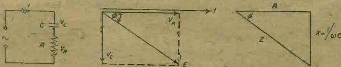
Fig. 13.—Phase relations of  $E$  and  $I$  and the impedance triangle for a resistance-capacity arrangement.
