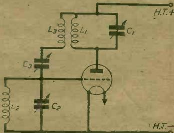
Fig. 27.—A typical neutralising circuit.
