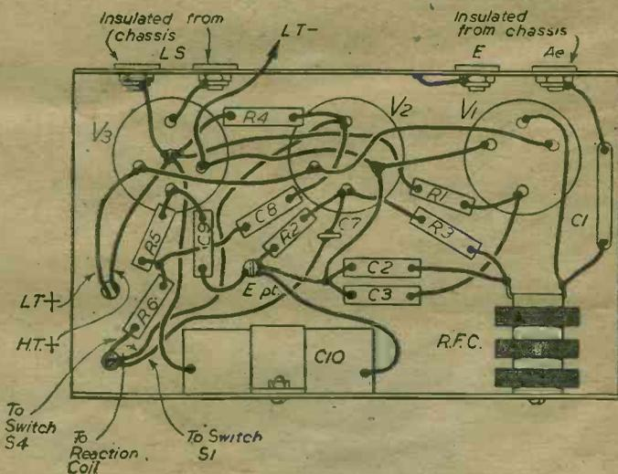
Fig. 2.—Underside of chassis showing wiring, etc.
