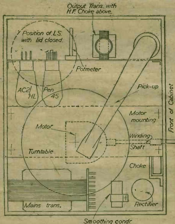
Fig. 2.—Plan view of the record amplifier, showing layout of components.
