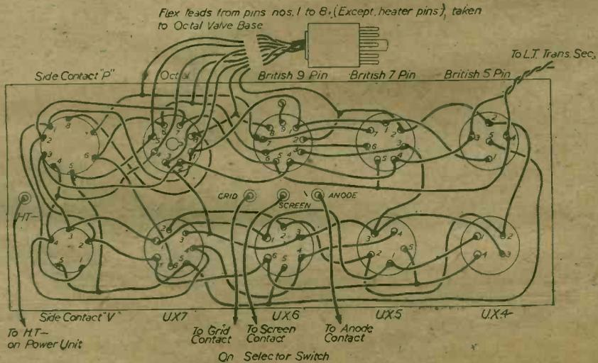
Figs. 2 and 3.—Plan and underside views of the valve panel.
