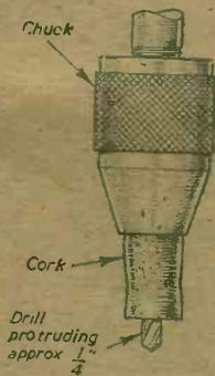
A drill stop for use when drilling holes in thin metal.
