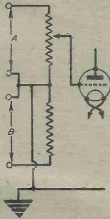
Fig. 2.—No switching required as use is made of a "fader" type volume control. This allows fading from one input to another but no mixing.
