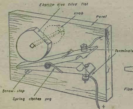
A simple L.T. switch made from odds and ends.
