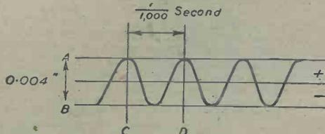
Fig. 2.—Diagram illustrating the amplitude waveform of a single note.
