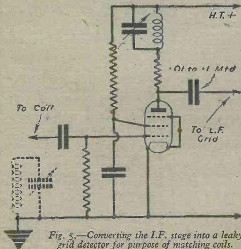
Fig. 5.—Converting the I.F. stage into a leaky grid detector for purpose of matching coils.
