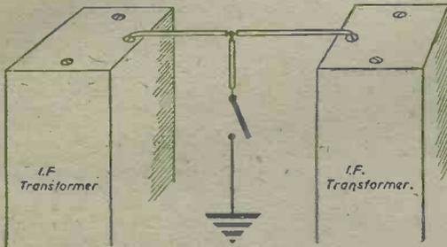
Coupling two I.F. transformers for receiving C.W. signals on a superhet.
