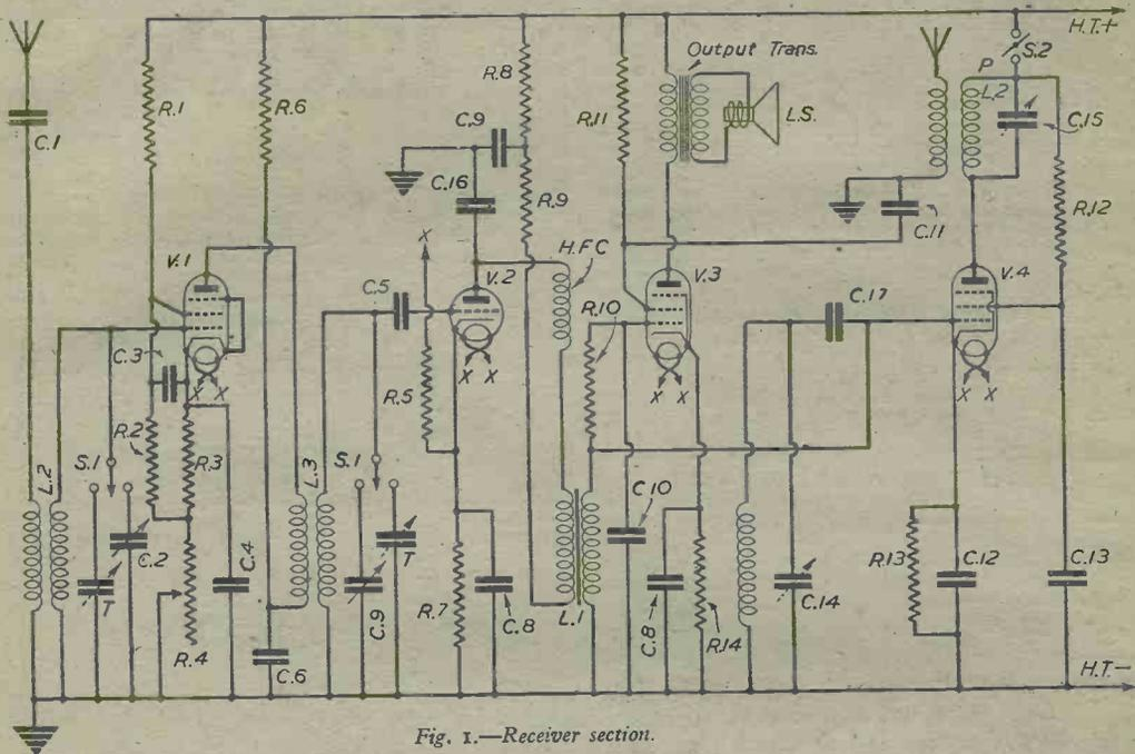
Fig. 1.—Receiver section.
