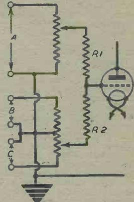
Fig. 4.—A three input arrangement mixer on two and fader on two. Better than that shown in Fig. 3.
