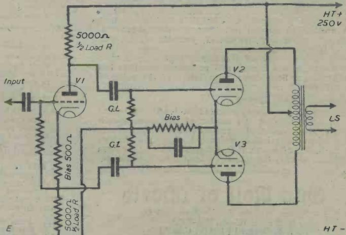
**Fig. 2.**—Skeleton circuit of a paraphase amplifier of the type suggested for fidelity reproduction. High-quality amplifiers were described in the January, February and March, 1944, issues of PRACTICAL WIRELESS. A paraphase amplifier with negative feed-back was described in the last-mentioned issue.
