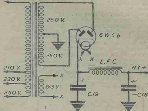
Fig. 3.—Power circuit.
