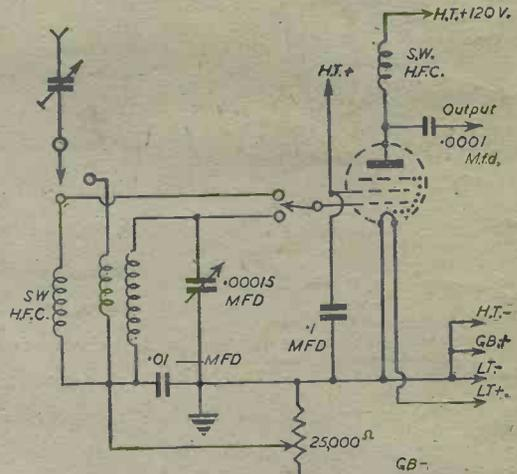
The circuit of the variable Mu H.F. amplifier, showing how a tuned or untuned aerial circuit is obtained by switching.
