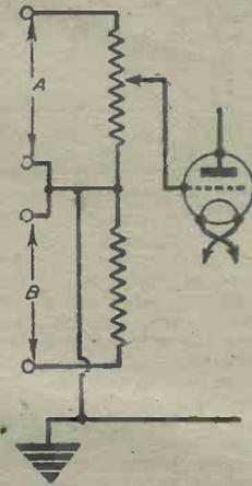
Fig. 2.—No switching required as use is made of a "fader" type volume control. This allows fading from one input to another but no mixing.
