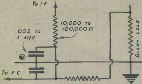
Fig. 3.—Decoupling the A.V.C. circuit.
