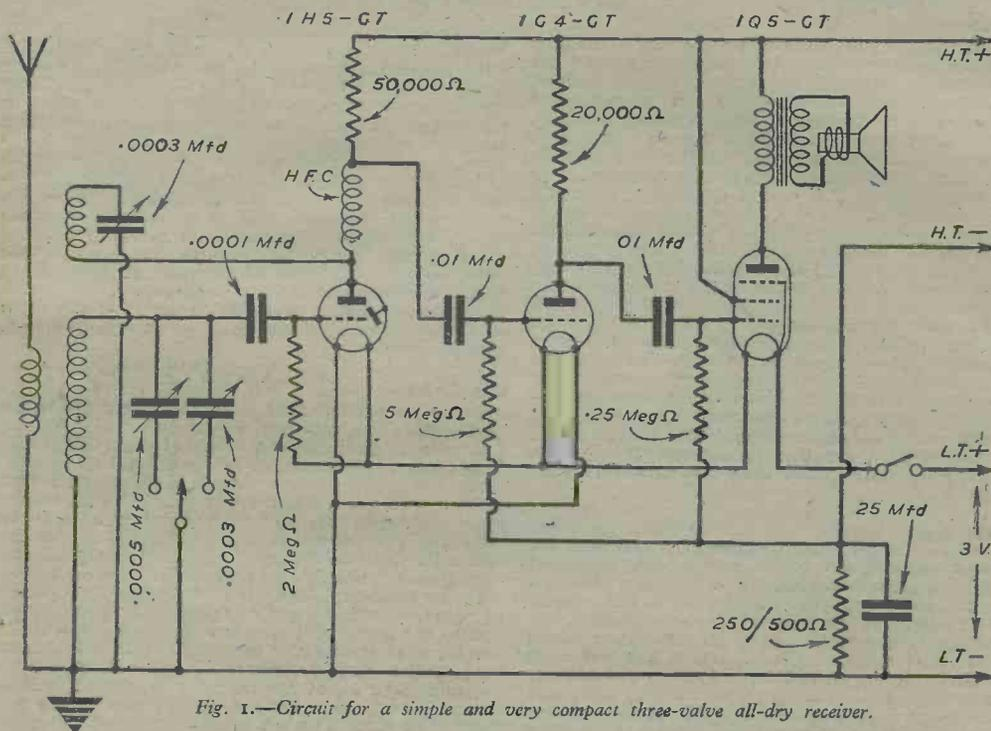
Fig. 1.—Circuit for a simple and very compact three-valve all-dry receiver.
