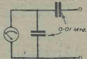
Fig. 4.—Method of doubling the range of an electrostatic voltmeter.
