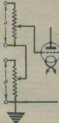
Fig. 3.—The simplest form of mixer circuit, suitable for two inputs. Provides volume control, fading and mixing.
