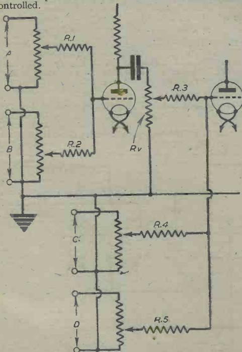
Fig. 7.—A four input system suitable for use with low and high inputs, and good mixing.
