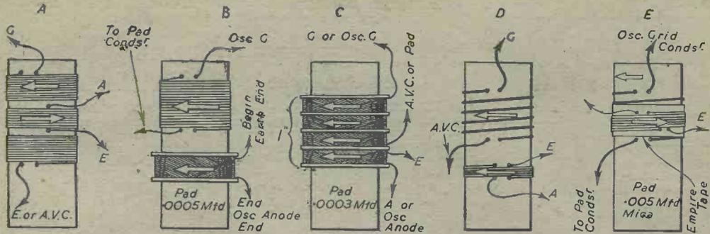
Fig. 7.—Coil details (see table). A, medium-wave aerial coil; B, medium-wave oscillator coil; C, long-wave aerial and oscillator coil; D, s.w. aerial coil; E, oscillator as aerial coil.
