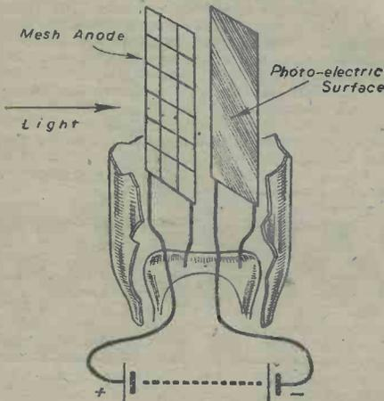
Fig. 2.—The construction of a simple photo-electric cell.
