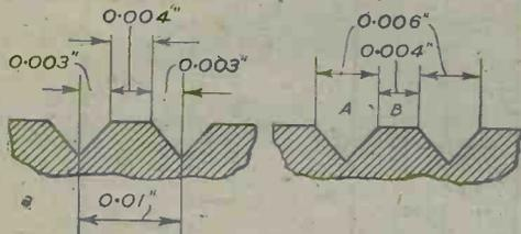
Fig 5 (a).—See text; (b) Normal cut for 96/100 cuts/inch. Known as a 60/40 cut.
