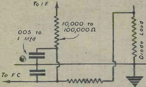
Fig. 3.—Decoupling the A.V.C. circuit.
