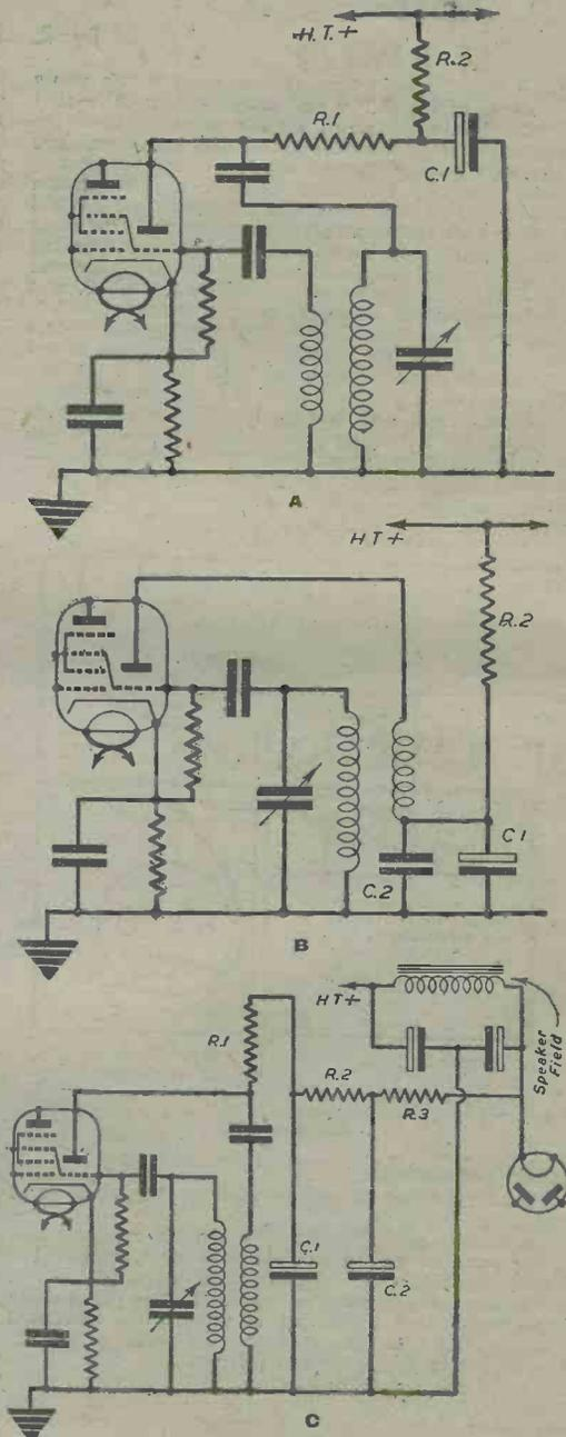
Fig. 2.—Three methods of eliminating L.F. hum.
