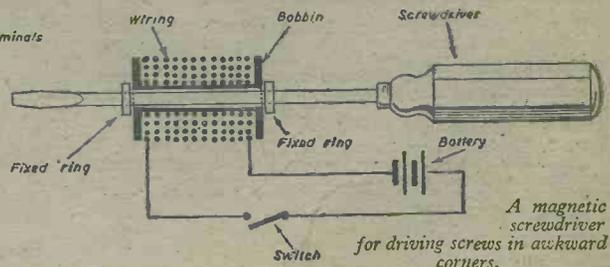
A magnetic screwdriver for driving screws in awkward corners.
