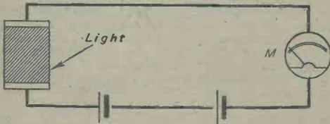
Fig. 1.—A simple selenium cell causing current changes in accordance with the intensity of incident light.
