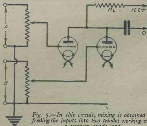
Fig. 5.—In this circuit, mixing is obtained by feeding the inputs into two triodes working into a common anode load.
