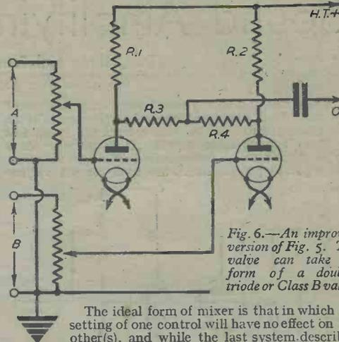
Fig. 6.—An improved version of Fig. 5. The valve can take the form of a double-triode or Class B valve.
