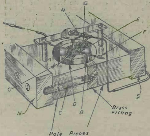
Fig. 1.—Moving coil meter movement.
