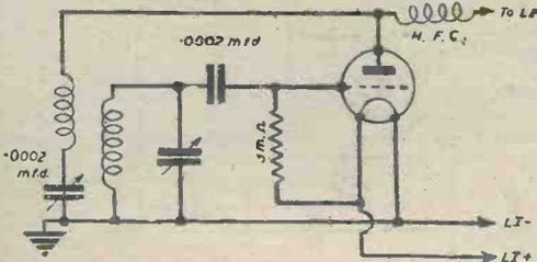
Fig. 1.—The simplest reaction arrangement.
