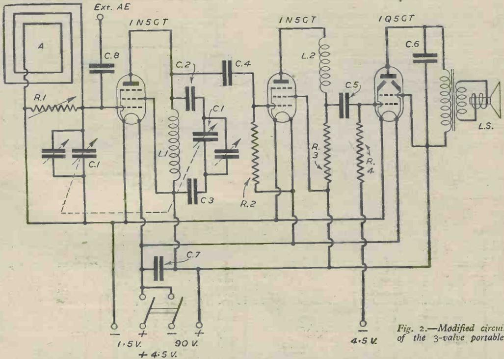
Fig. 2.—Modified circuit of the 3-valve portable.
