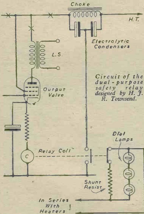
Circuit of the dual-purpose safety relay designed by H. J. R. Townsend.
