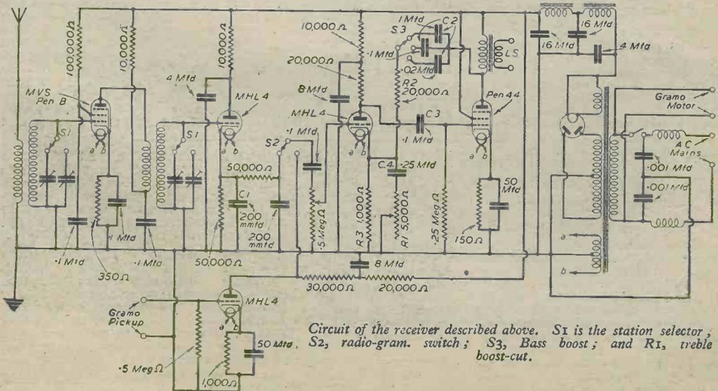
Circuit of the receiver described above. S1 is the station selector; S2, radio-gram. switch; S3, Bass boost; and R1, treble boost-cut.
