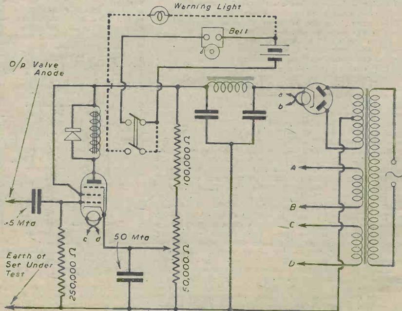
Circuit of the fault detector.
