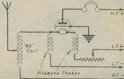
Fig. 6.—This Filadlyne circuit receives the local station without tuning.
