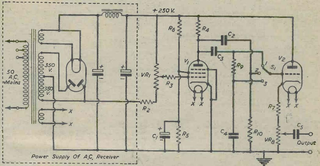
Fig. 12.—Pulse generator. Note: Switch S1 in position (1) gives square wave output; in position (2), sharp pulse output; and in position (3), triangular wave output.
