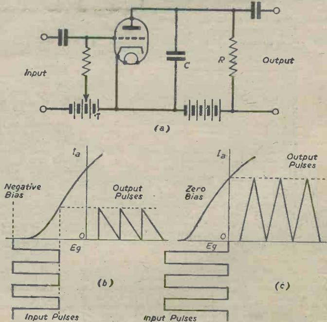
Fig. 11.—Another type of wave-shaping circuit for triangular pulses.
