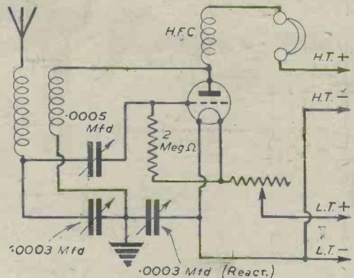
Fig. 2.—A modified Chitos circuit.
