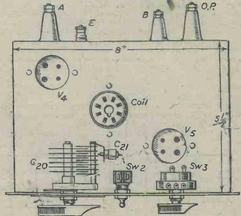
Fig. 2.—Layout of chassis and components for the Preselector.
