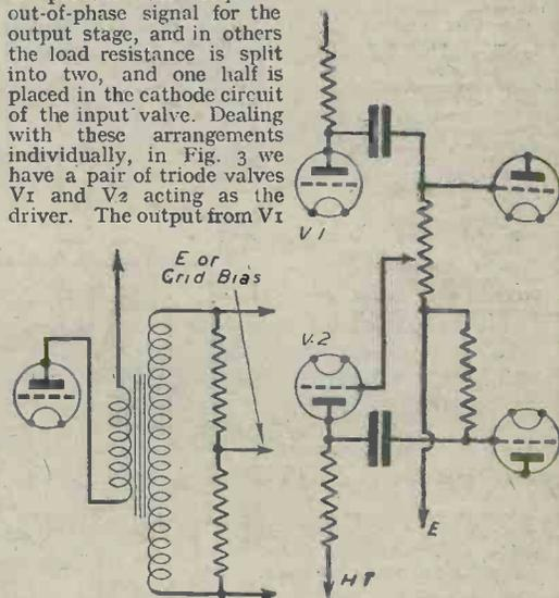
Fig. 2.—Improvising a centre-tap on an ordinary transformer by means of two resistors.
