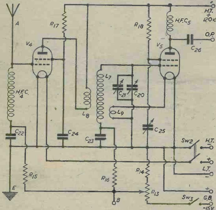
Fig. 1—Circuit of the Preselector.
