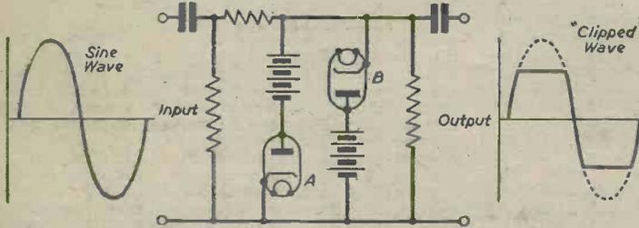
Fig. 10.—A "peak clipping" circuit and its effects shown diagrammatically.
