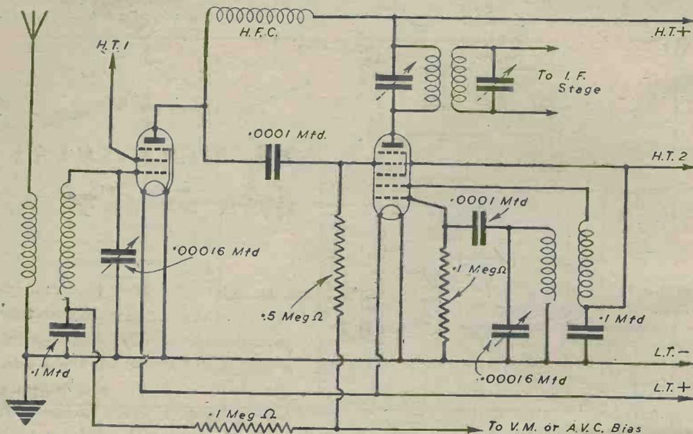
Fig. 4.—A heptode valve is used in this circuit, with the addition of an H.F. stage.
