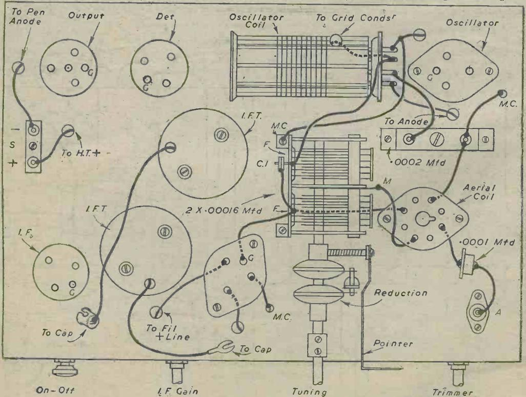
Fig. 3.—Top of chassis wiring diagram. Use this in conjunction with the photo above.
