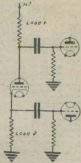
Fig. 4.—A single valve acting as a phase inverter stage.
