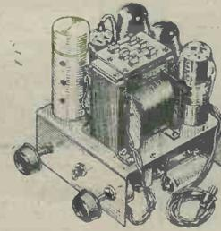
**UNIT No. 7 :** High Fidelity Output and Power Stages—two L.F. valves feeding two PX4 valves in push-pull (triodes). Controls: Volume, Mains on/off, radio-gram, switch and Tone.
