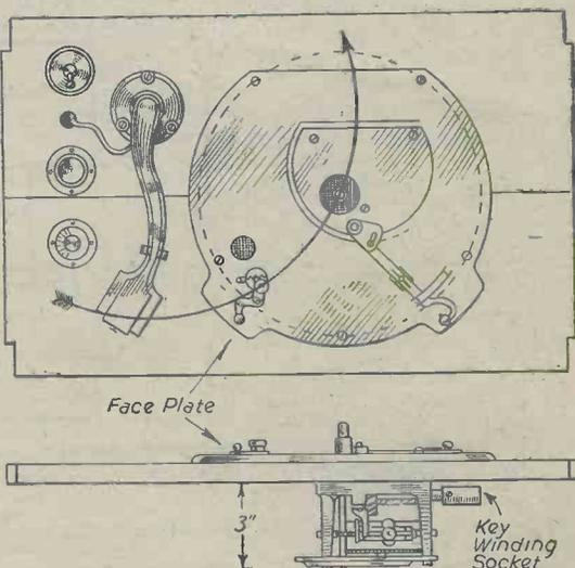
Fig. 8.—How the gramophone motor face-plate is mounted on its board, with approximate position of pick-up, switch and needle holder cups.
