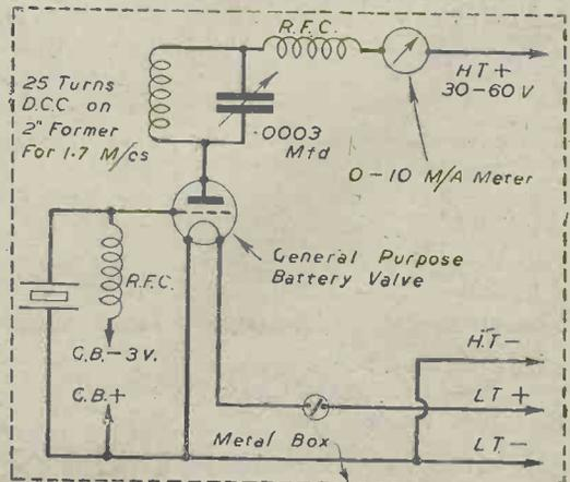
Fig. 2.—Test oscillator for the crystals.
