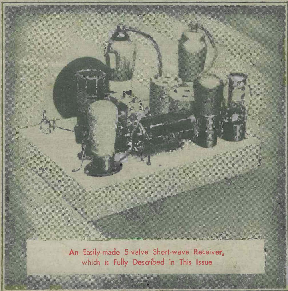
An Easily-made 5-valve Short-wave Receiver,
