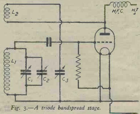
Fig. 3.—A triode bandspread stage.
