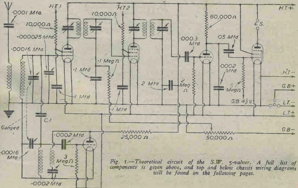
Fig. 1.—Theoretical circuit of the S.W. 5-valver. A full list of components is given above, and top and below chassis wiring diagrams will be found on the following pages.
