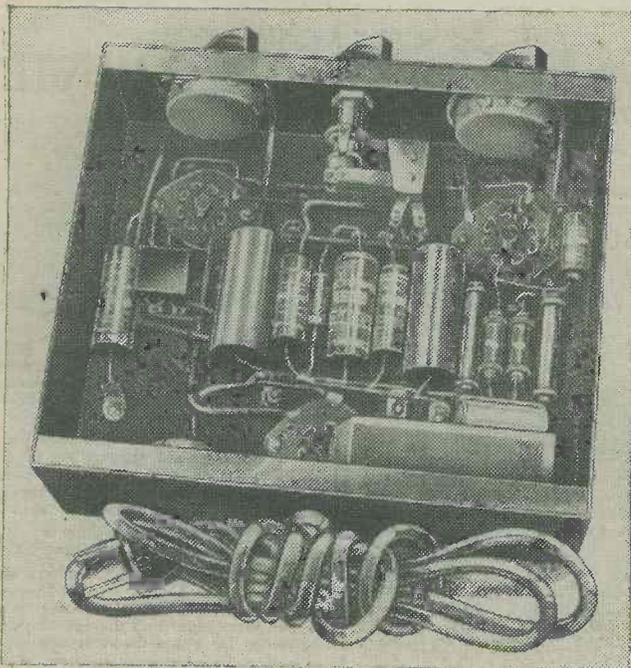
Fig. 3.—An under-chassis view of the instrument. Control in centre is the D.P.D.T. switch. Terminal strips help make a systematic layout and a neat wiring job.
