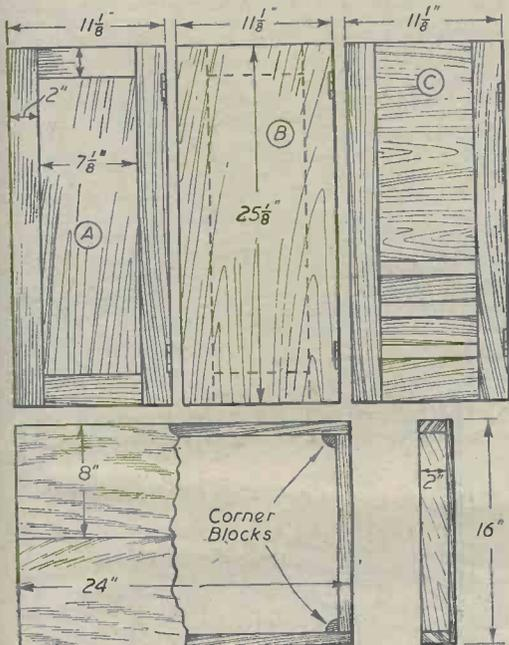
Fig. 7.—The doors and top plan of lid.
