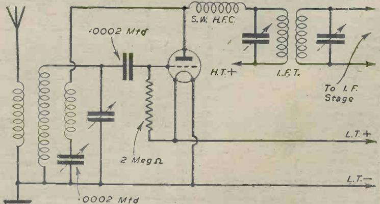
Fig. 1.—The simplest form of frequency-changer—in other words a simple Superhet. converter.
