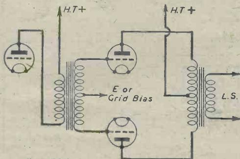
Fig. 1.—Skeleton circuit of the push-pull arrangement.
