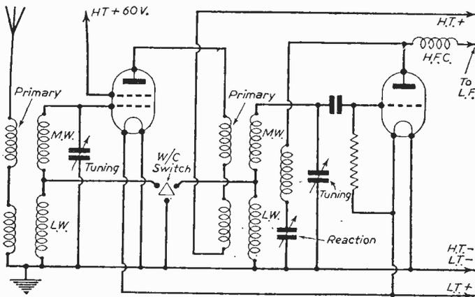
Fig. 4.—This circuit uses two of the coils of Fig. 2.
