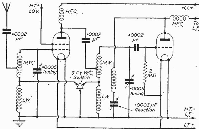
Fig. 3.—Simple circuit incorporating a pair of the coils of Fig. 1.
