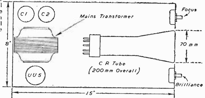
Fig. 5. Layout of the complete instrument.
