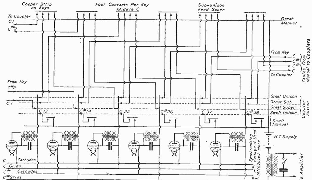
Fig. 1.—General scheme of the organ, illustrated by three octaves of the notes C and C sharp. All other notes are, of course, treated the same.
