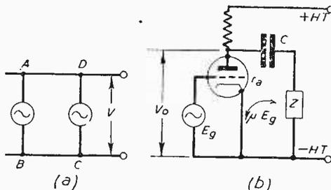
Fig. 2.—The E.M.F.s of two alternators in parallel are virtually in series opposition in the closed mesh ABCD. In the shunt-fed valve circuit (b), *Z* and *ra* are in parallel relative to *Vo*, but  $\mu E_g$  still acts upon *Z*, *ra* and *C* regarded as a closed series mesh.
