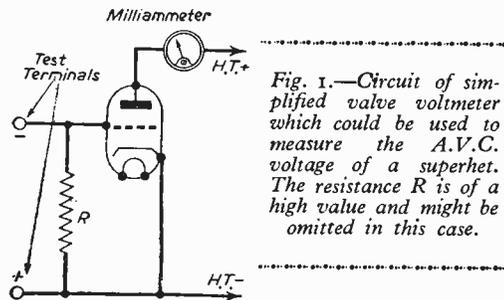
Fig. 1.—Circuit of simplified valve voltmeter which could be used to measure the A.V.C. voltage of a superhet. The resistance R is of a high value and might be omitted in this case.
