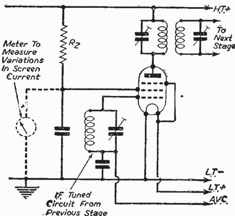
Fig. 3.—Battery version of Fig. 2, showing how "trimming meter" is this time connected between screen grid of the valve and earth.
