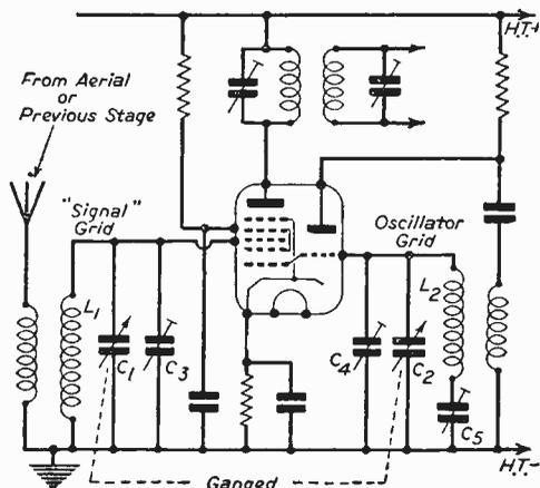
Fig. 7.—Circuit of typical frequency-changer, illustrating various condensers used for tuning, trimming and padding.
