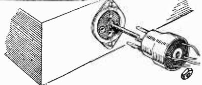
A plug which cannot be knocked out of its socket.
