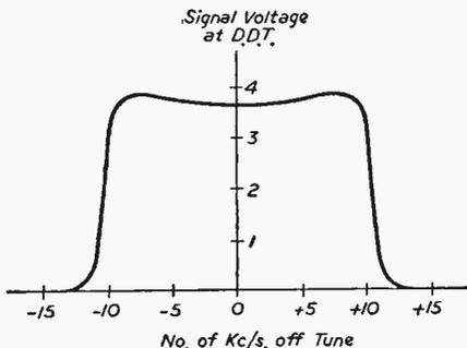
Fig. 4.—Example of “bandwidth curve” of I.F. transformers. The signal cuts off sharply after 10 kc/s off-tune on either side and remains substantially flat for  $\pm 7.5$  kc/s.
