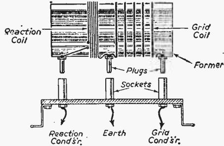
Fig. 8.—Plug-in short-wave coils with reaction windings.
