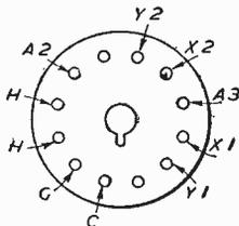
Fig. 4. Connections to the tube base.
