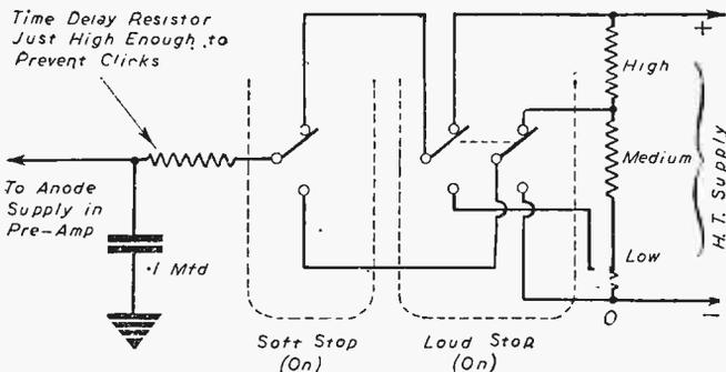
Fig. 2.—Gaskell's two-stop, three intensity circuit. With Soft off and loud off output is 0
