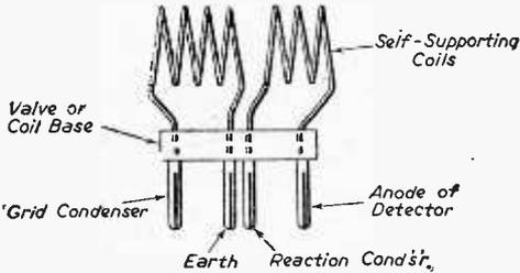
Fig. 7.—Another form of interchangeable U.S.W. coil.
