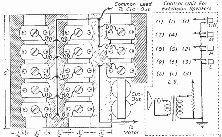
Fig. 5.—Details of assembly of the complete relay bank, and, on the right, the control unit wiring for the extension speakers.
