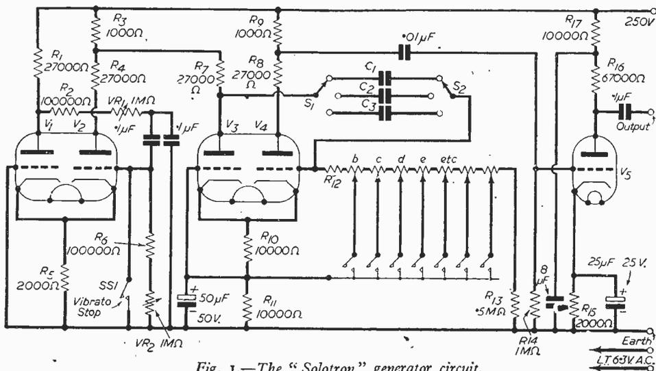
Fig. 1.—The "Solotron" generator circuit.
