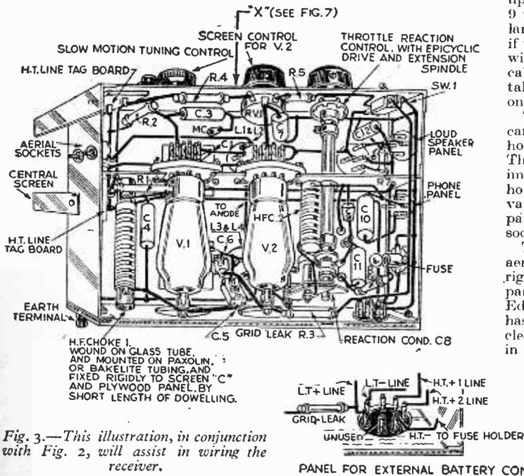
Fig. 3.—This illustration, in conjunction with Fig. 2, will assist in wiring the receiver.
