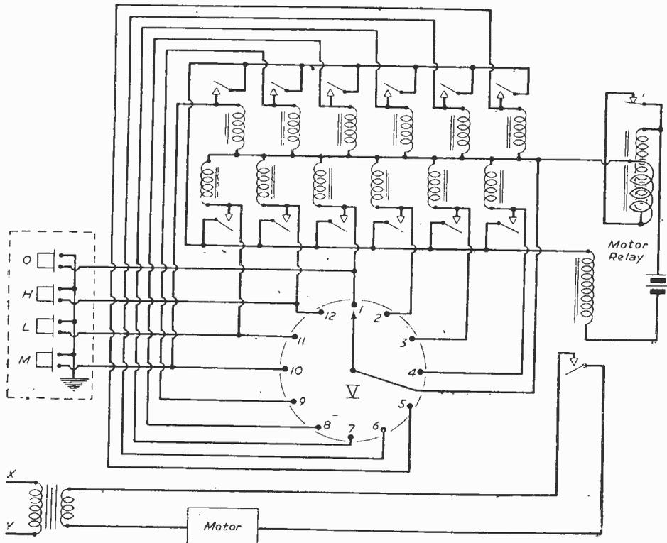
Fig. 2.—Circuit of the main switching mechanism. This is mains operated, and the input transformer at points X and Y is joined to the similarly marked points on Fig. 1 opposite.
