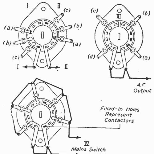
Fig. 3.—Connections of the switch wafers.
