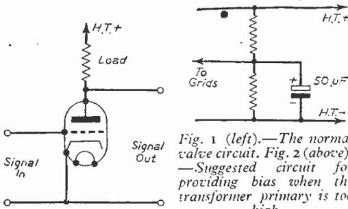
Fig. 1 (left).—The normal valve circuit. Fig. 2 (above).—Suggested circuit for providing bias when the transformer primary is too high.
