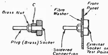
Method of making insulated sockets.
