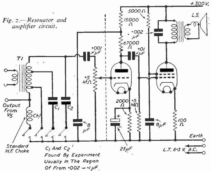
Fig. 2.—Resonator and amplifier circuit.
