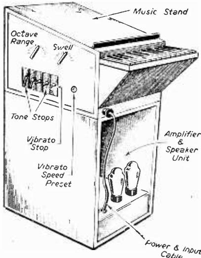
Fig. 3.—The completed instrument.
