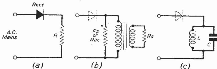
Fig. 5.—Three types of "load." (a) An ordinary D.C. resistance; (b) an "A.C." aperiodic, or non-resonant resistance; (c) resonant load, or dynamic resistance of a tuned-circuit. What effects would occur in each case if the current was of the form shown in Fig. 1(a) last month?
