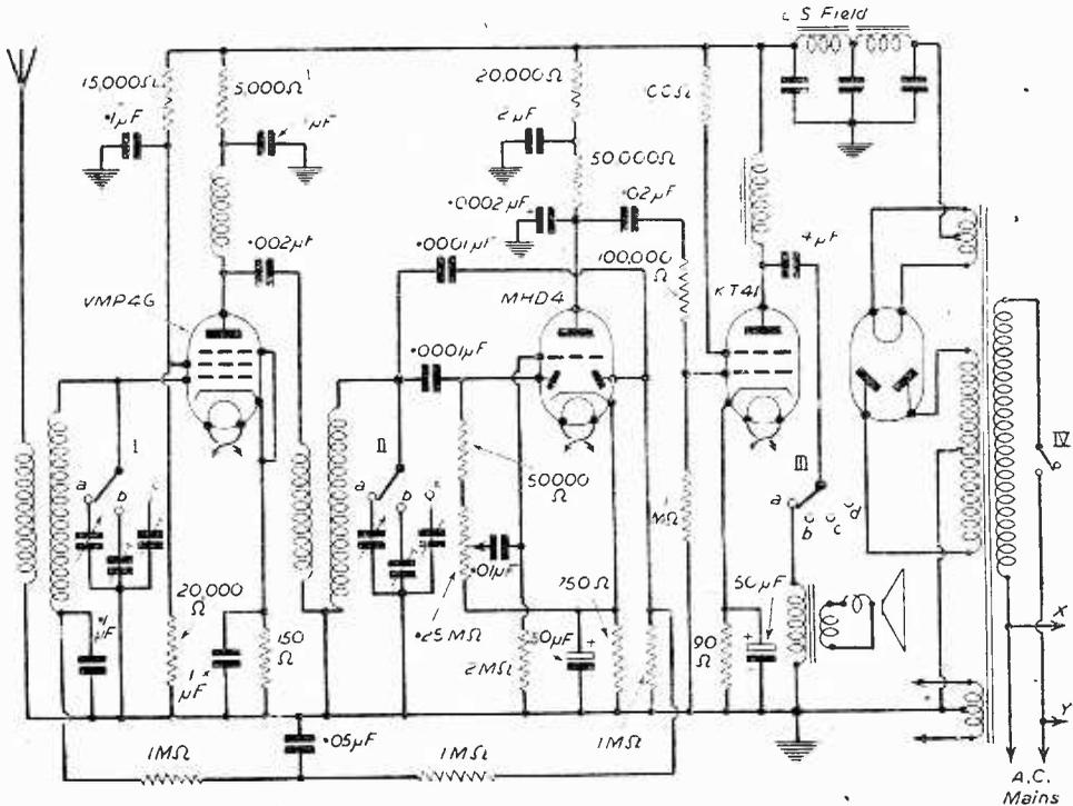
Fig. 1.—Circuit of the radio receiver, which follows more or less standard lines. The two points X and Y on the primary of the mains transformer are connected to similarly marked points on Fig. 2 opposite.
