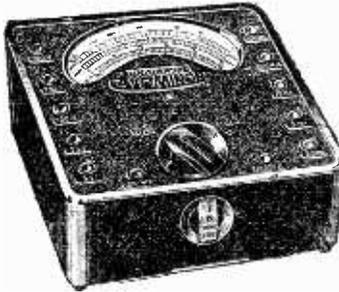
A small but highly accurate instrument for measuring A.C. and D.C. voltage, D.C. current, and also resistance. It provides 22 ranges of readings on a 3-inch scale, the required range being selected by plugging the leads supplied into appropriately marked sockets. An accurate moving-coil movement is employed, and the total resistance of the meter is 200,000 ohms.
