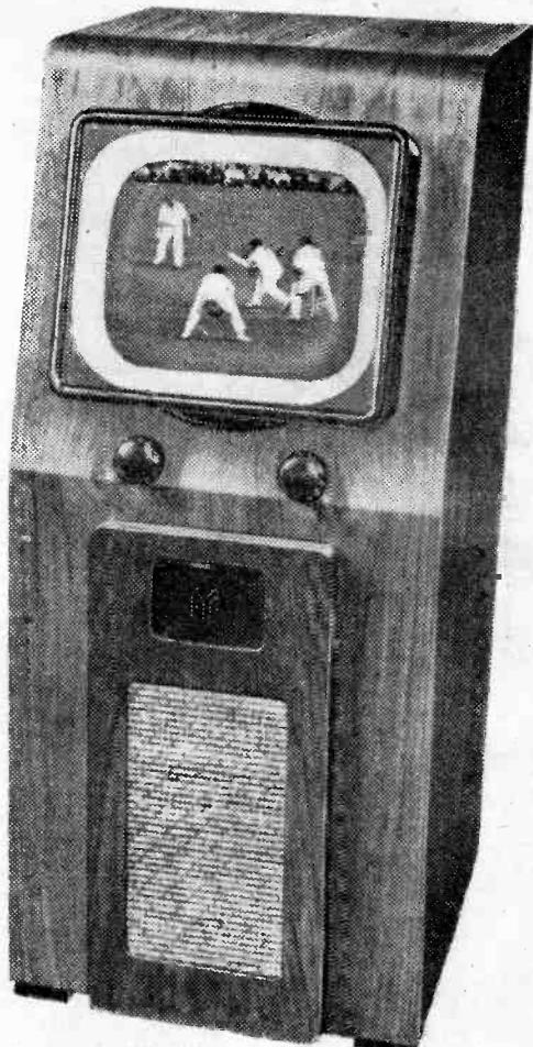
*A Pye television receiver of the console type. Although having only two controls (Brightness and Volume) the remaining controls, such as Contrast, Line Hold, etc., are accessible, being mounted immediately behind the small panel seen below the two control knobs. Thus it is a simple matter to make adjustments as and when required. This model gives a black-and-white picture.*
