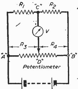
Fig. 1.—Circuit of Wheatstone Bridge.
