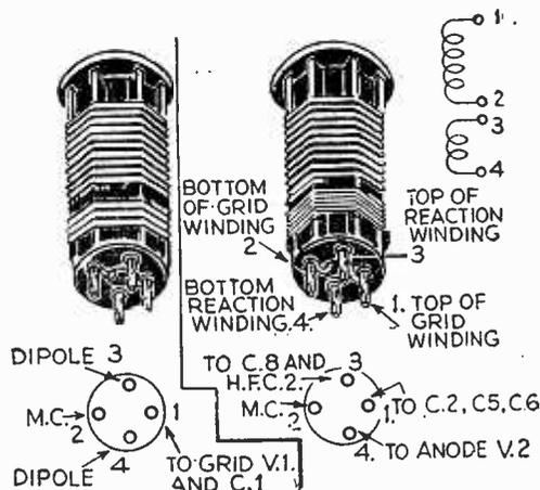
Fig. 9.—Constructional and connection data for the two types of coil used in the Short-wave Battery Three.
