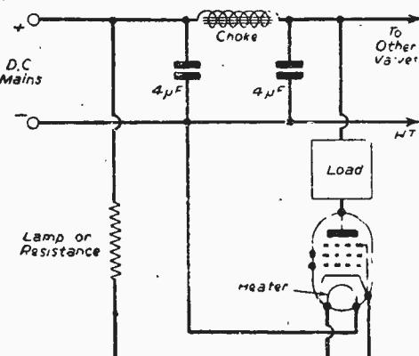
Fig. 3.—An eliminator supplying both H.T. and heater voltages and currents.
