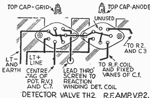
Fig. 7.—Wiring details for valve holders of V.1 and V.2, as viewed from Point "X" in Fig. 3.
