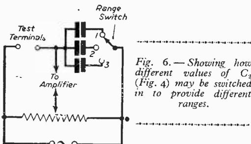
Fig. 6. — Showing how different values of  $C_2$  (Fig. 4) may be switched in to provide different ranges.
