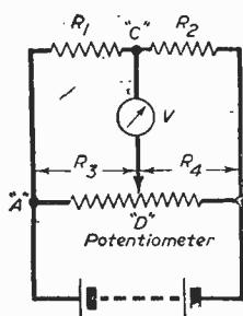
Fig. 1.—Circuit of Wheatstone Bridge.
