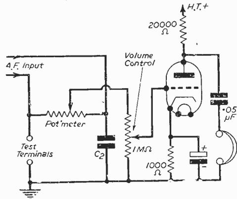
Fig. 5.—Modified version of Fig. 4. Point "C<sub>2</sub>" of Fig. 4, is now connected to earth, and the A.F. input has both leads isolated from earth. Any L.F. amplifier type triode may be used.
