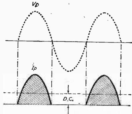
Fig. 7.—If an "average D.C." is multiplied by an alternating voltage, what sort of "power" does the answer give? The D.C. in the diagram is the mean value of a half-wave current. The sine-wave voltage is the mains voltage.
