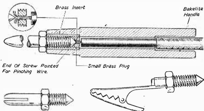
Making test prods with interchangeable points.
