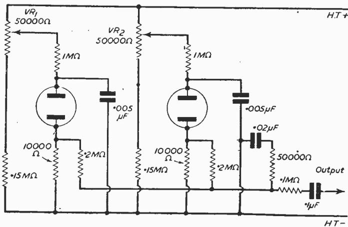
Fig. 3.—For an aircraft engine effect this circuit should be used.
