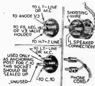
Fig. 8.—Loud speaker and phone panels, showing wiring details.
