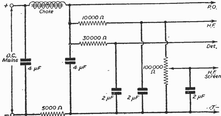
Fig. 1.—An old type of D.C. eliminator for use with a set not employing decoupling.
