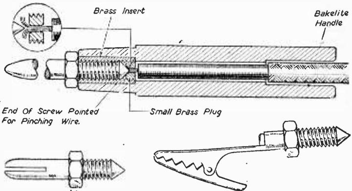
Making test prods with interchangeable points.
