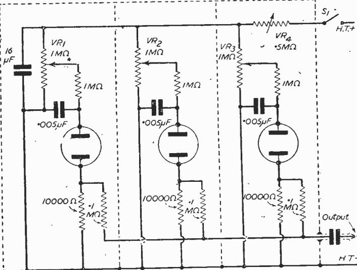
Fig. 1.—Circuit for producing a siren effect.
