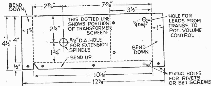
Fig. 6.—Cutting, bending and drilling details for the central screening panel.
