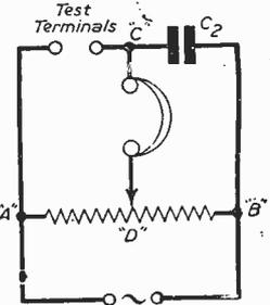
Fig. 4.—Circuit of simple capacity bridge.
