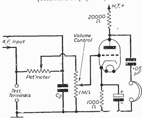
Fig. 5.—Modified version of Fig. 4. Point "C," of Fig. 4, is now connected to earth, and the A.F. input has both leads isolated from earth. Any L.F. amplifier type triode may be used.
