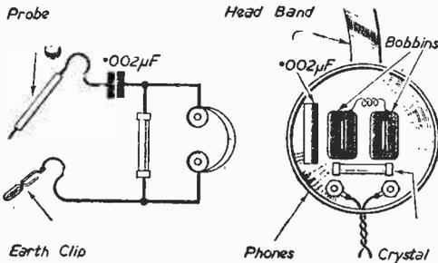
The simplest form of signal tracer
