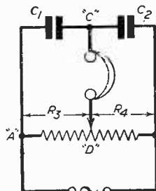
Fig. 3.—Showing how condensers may be connected in the bridge circuit instead of resistances  $R_1$  and  $R_2$  (Fig. 2).
