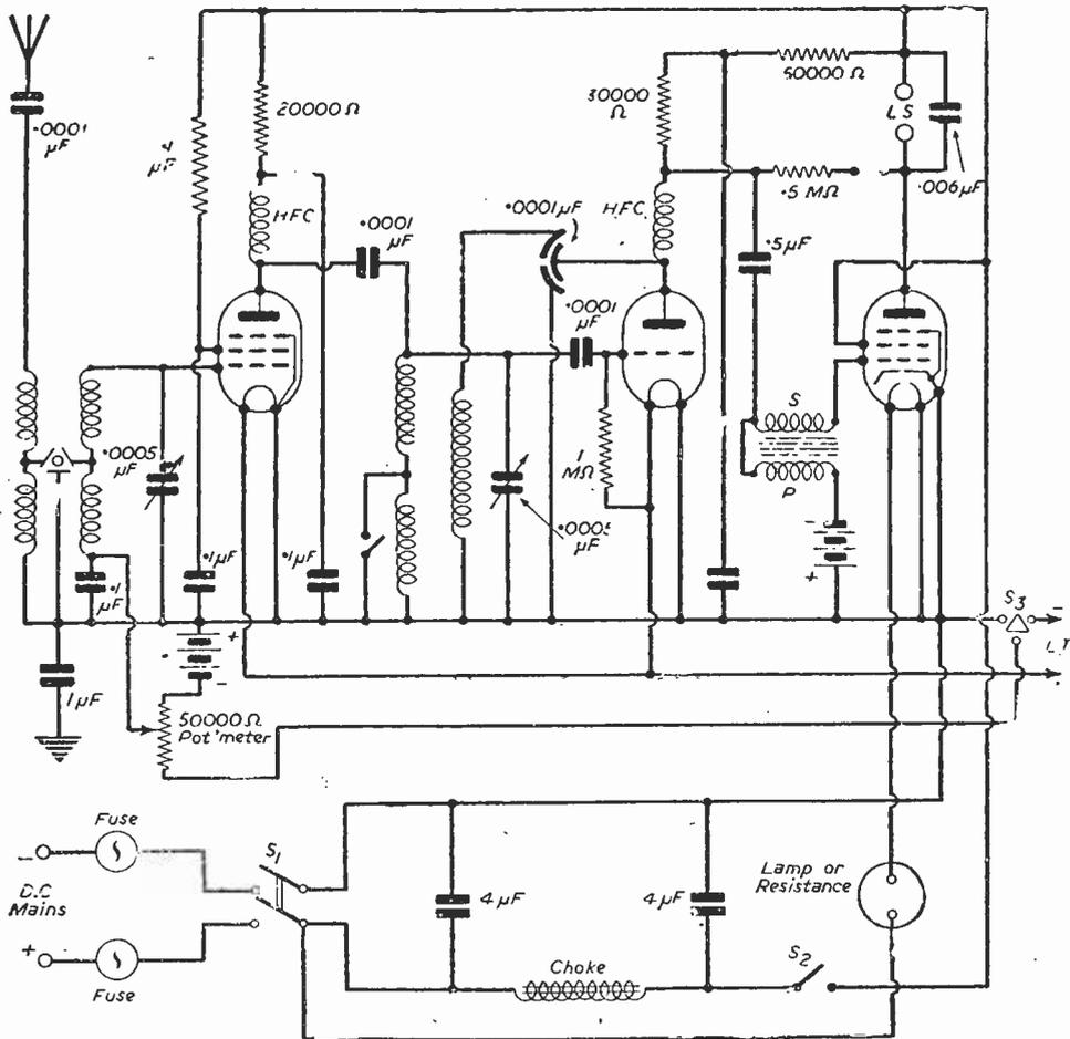
Fig. 4.—This diagram shows how a mains pentode may be used in conjunction with battery valves and a D.C. mains eliminator.
