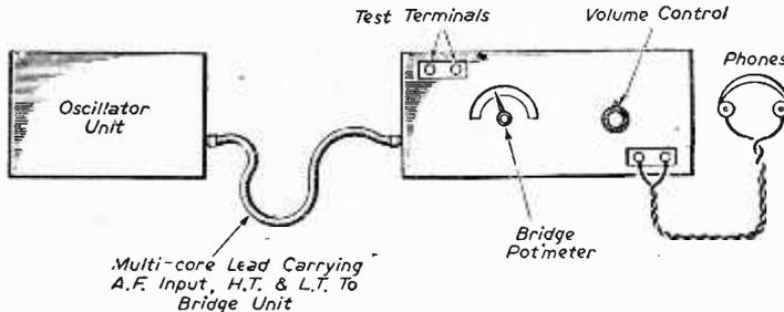
Fig. 9.—How the capacity meter was finally arranged.
