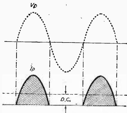
Fig. 7.—If an "average D.C." is multiplied by an alternating voltage, what sort of "power" does the answer give? The D.C. in the diagram is the mean value of a half-wave current. The sine-wave voltage is the mains voltage.
