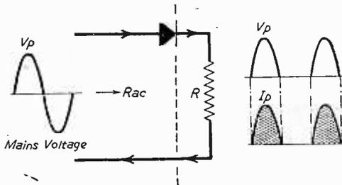
Fig. 8.—On the right of the dotted line, current and voltage are pulsating. To the left, the current is still of pulsating waveform, but the mains voltage is a sine-wave. "Fundamental power" will be taken from the mains, equal to the sum of the various power components in R. The A.C. mains will see a load  $R_{ac}=2R$ .
