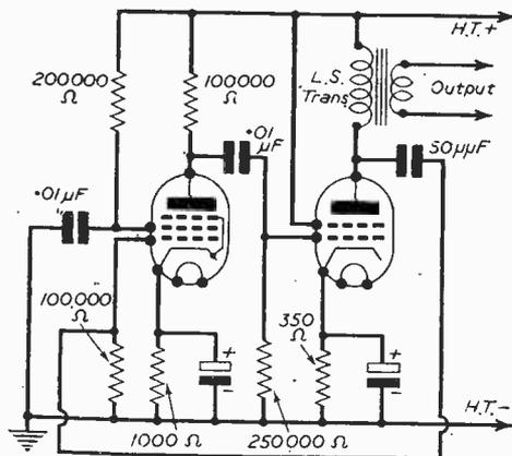
Fig. 7. — Circuit of A.F. oscillator used with bridge. Any R.F. pentode followed by any output pentode or tetrode will suffice. Some individual adjustment of values may be required to produce the hiss component required (see text). Output is at low impedance.
