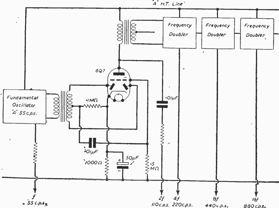
Fig. 4.—A frequency doubler circuit.
