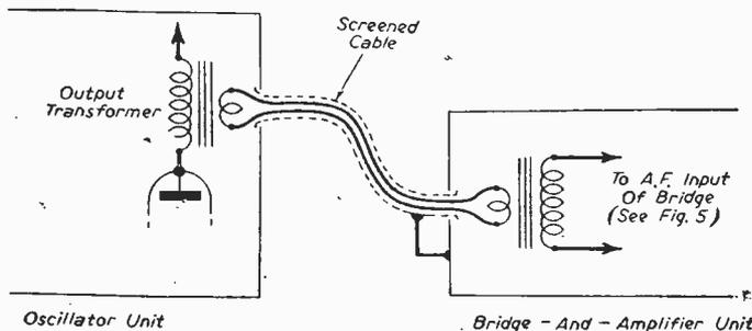
Fig. 8. — Showing method of connecting A.F. oscillator to bridge unit.
