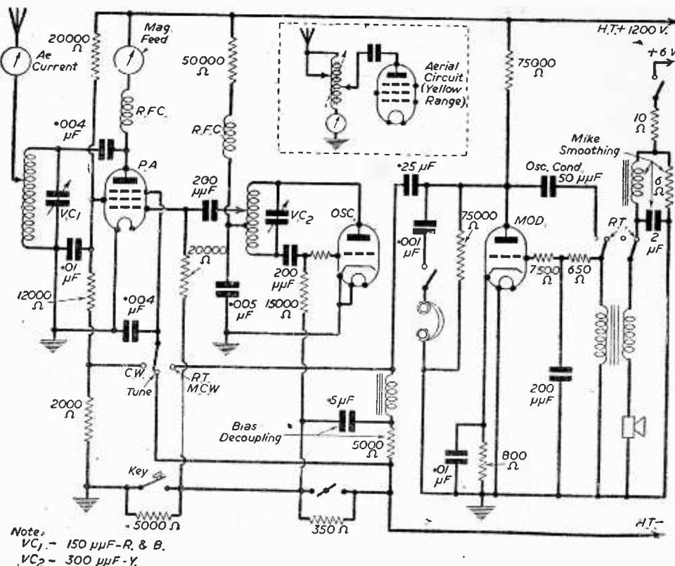
Fig. 1.—Skeleton theoretical circuit of the T.1154 R.A.F. receiver referred to in these notes.
