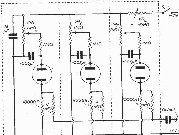
Fig. 1.—Circuit for producing a siren effect.
