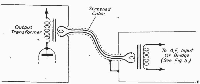
Fig. 8.—Showing method of connecting A.F. oscillator to bridge unit.
