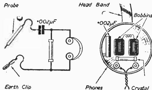
The simplest form of signal tracer
