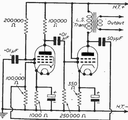
Fig. 7.—Circuit of A.F. oscillator used with bridge. Any R.F. pentode followed by any output pentode or tetrode will suffice. Some individual adjustment of values may be required to produce the hiss component required (see text). Output is at low impedance.
