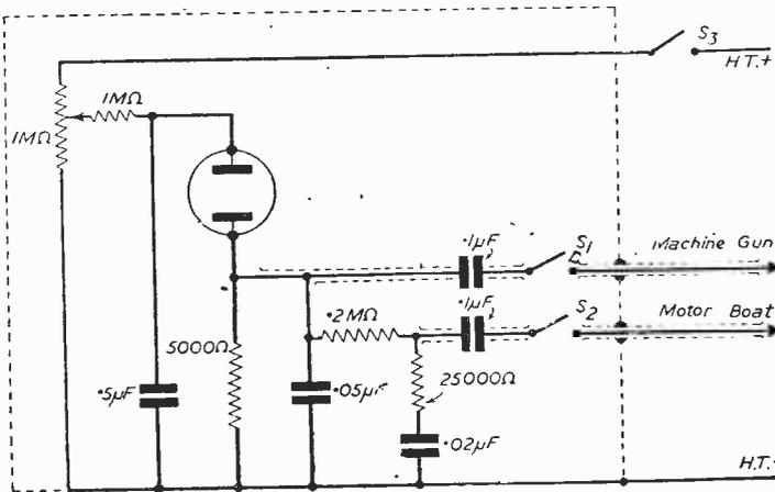
Fig. 2.—This circuit will simulate a machine gun or motor boat.
