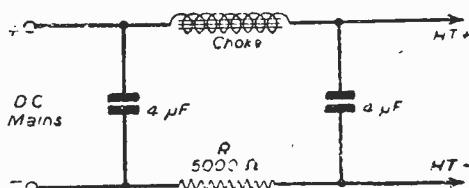
Fig. 2.—In this circuit the current through the eliminator is limited by 'R.'
