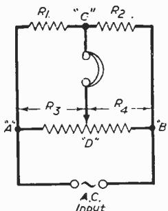
Fig. 2.—Showing modification of Fig. 1. The A.C. input may be conveniently supplied by an A.F. oscillator.
