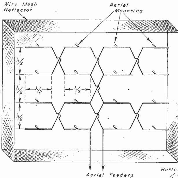
Fig. 7.—A representative form of stacked dipole aerial array, with wire mesh back reflector. The whole array is arranged to rotate for direction-finding.
