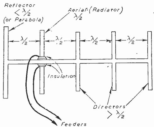
Fig. 8.—The Yagi type of directional aerial has a reflector, which is slightly longer than the aerial itself, or which consists of a parabola and any number of directors, which are slightly shorter than the aerial. The narrowness of the beam angle is governed by the number of directors. All elements are spaced by one-half wavelength.
