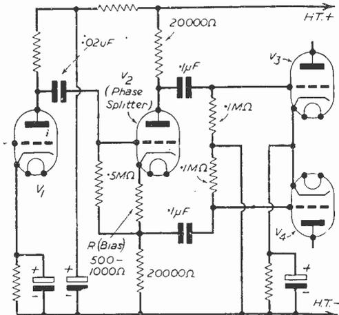
Fig. 5.—Phase-splitting valve with principal component values.
