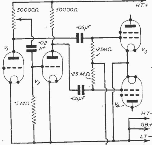
Fig. 7.—The "paraphase" circuit.
