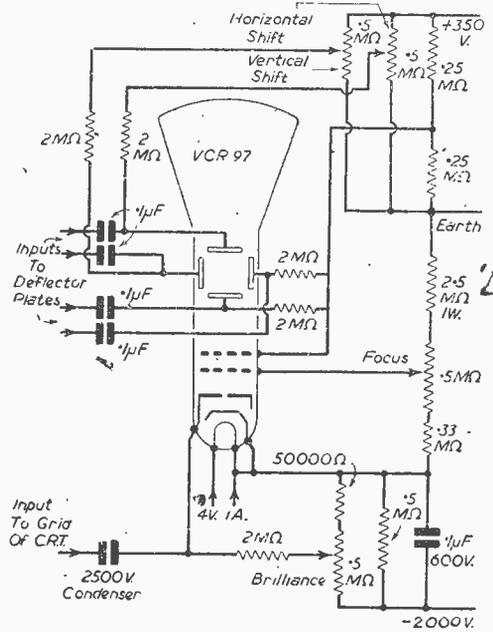
Fig. 1.—Typical circuit for the VCR97 and its equivalents.
