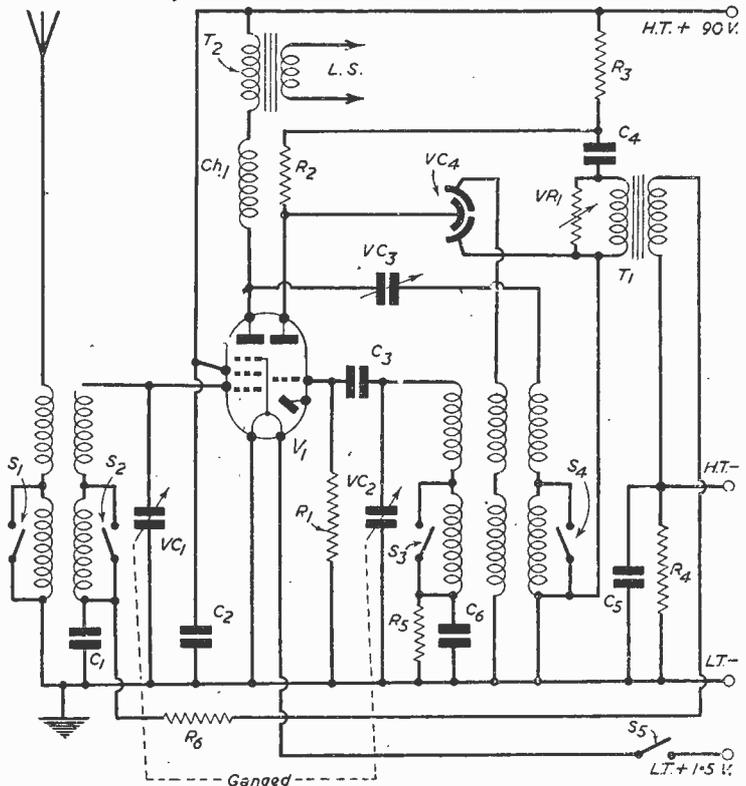
Fig. 1.—An efficient one-valve reflex receiver.
