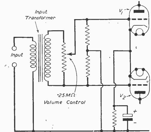
Fig. 9.—Connections for input transformer and volume control.
