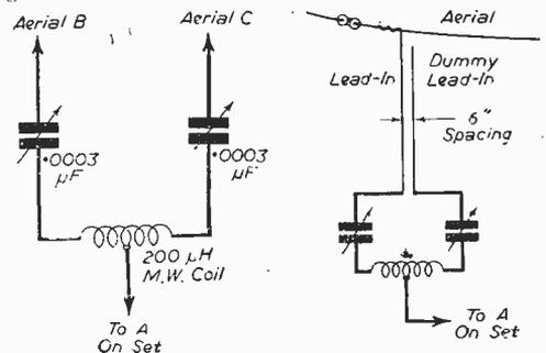
Fig. 3.—Coupling arrangement for the two aerials.
