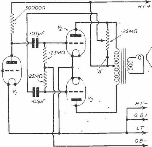
Fig. 6.—"Phase splitting" for push-pull, when the required input for V3 is taken from the output of V2.
