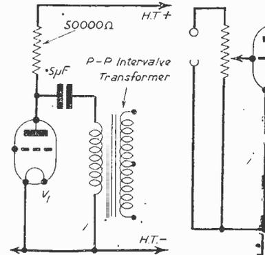
Fig. 2.—Connections for valve and transformer, using parallel feed.
