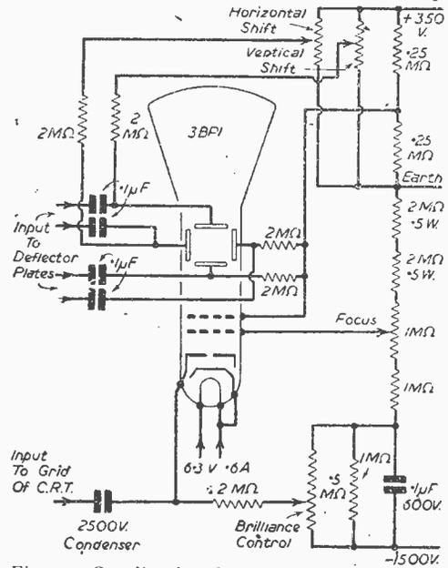
Fig. 2.—Supplies for the 3BP1 are shown here.
