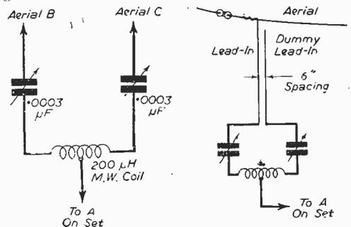
Fig. 3.—Coupling arrangement for the two aerials.
