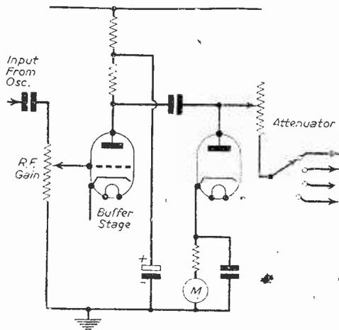
Fig. 2.—An R.F. meter and rectifier circuit showing modification of buffer stage for R.F. gain control.
