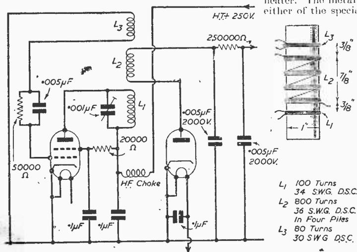
Fig. 4.—Another scheme for obtaining E.H.T. by means of an oscillator.
