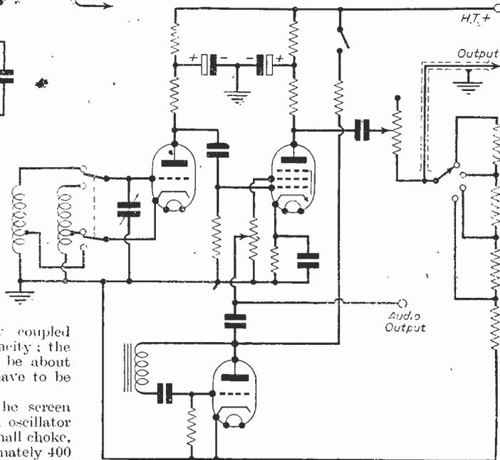
Fig. 1.—A signal generator using an E.C. oscillator.
