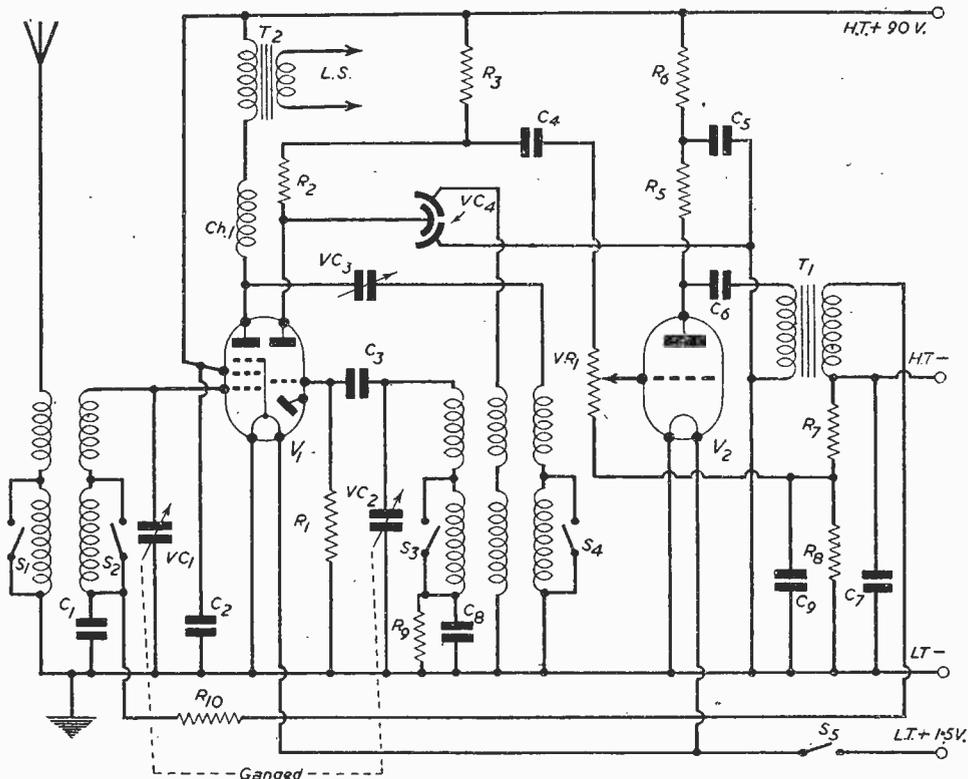
Fig. 2.—The arrangement of Fig. 1 with an additional stage and auto-bias.
