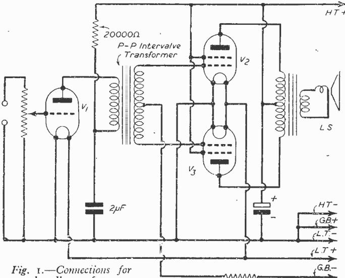
Fig. 1.—Connections for push-pull transformer.
