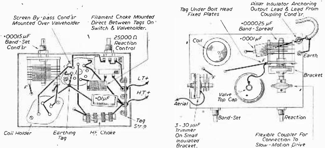
Fig. 2.—Top and below chassis wiring diagrams for the pre-selector.
