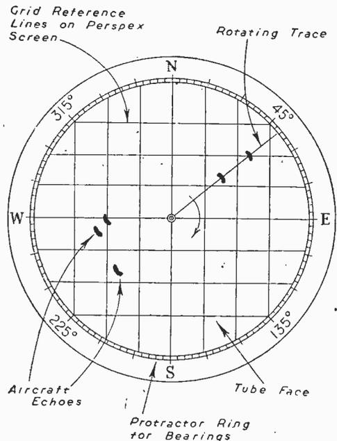
Fig. 10.—This illustration gives a good impression of the type of presentation obtained on a P.P.I. (plan position indicator) tube.
