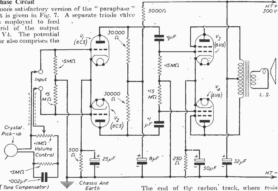
Fig. 8.—Twin-channel amplifier circuit, using "strapped" tetrodes as output triodes. Typical circuit for crystal pick-up is also shown.
