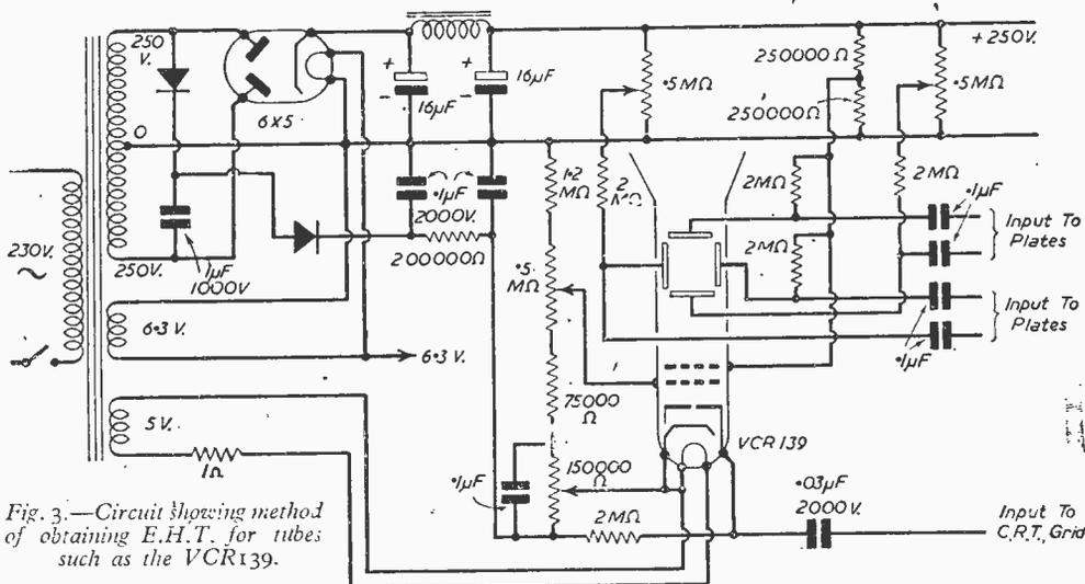
Fig. 3.—Circuit showing method of obtaining E.H.T. for tubes such as the VCR139.
