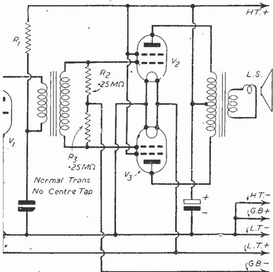
Alternative circuit, using normal inter-valve transformer.
