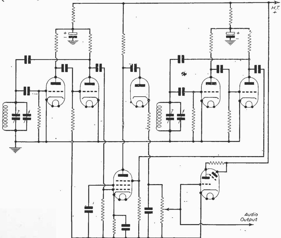
Fig. 3.—This circuit shows a Beat Frequency Oscillator with Franklin oscillators, and a cathode-ray zero indicator.
