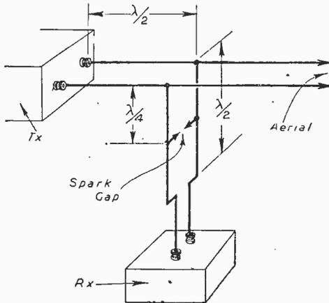
Fig. 9.—The method of connecting both transmitter and receiver to the same aerial is shown here. The spark gap (normally of the vapour-tube type) arcs over when the transmitter emits a pulse and so completes the quarter-wave "metallic insulator."
