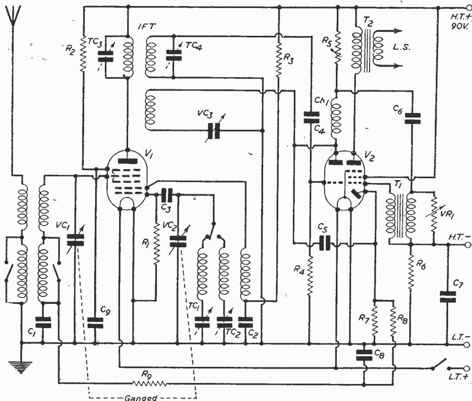
Fig. 3.—A superhet circuit with only two valves.
