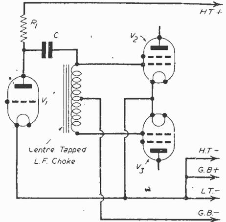
Fig. 4.—Basic circuit for inclusion of a centre-tapped L.F. choke.
